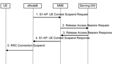
Figure 5.3.4A-1: eNodeB initiated Connection Suspend procedure
