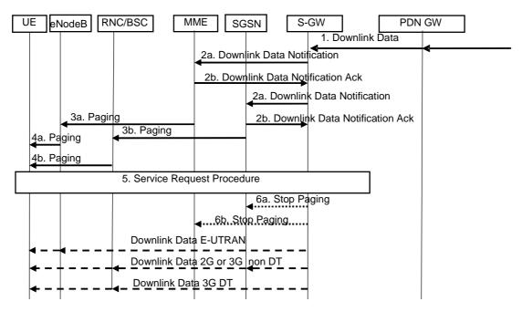
Figure 5.3.4.3-1: Network triggered Service Request procedure
