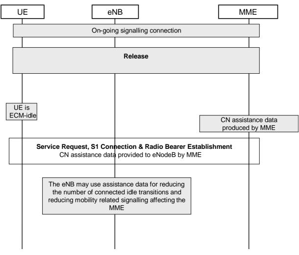
Figure 4.3.21.3-1: Core Network assisted eNodeB parameters tuning
