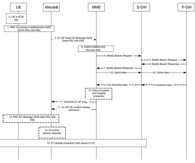
Figure 5.3.4B.2-1: MO Data transport in NAS PDU
