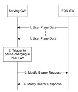
Figure 5.3.6A: PDN GW Pause of charging procedure
