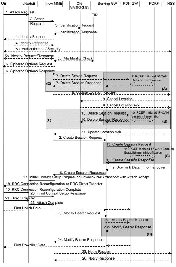
Figure 5.3.2.1-1: Attach procedure
