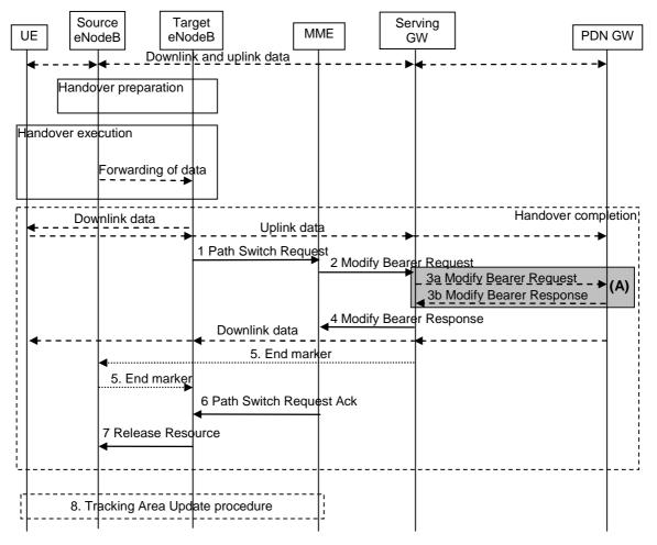
Figure 5.5.1.1.2-1: X2-based handover without Serving GW relocation
