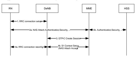
Figure 4.3.20.2-1: RN attach procedure
