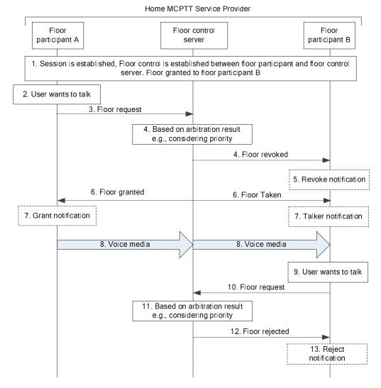
Figure 10.9.1.3.2.1-1: Floor override using floor revoked (also floor rejected) during an MCPTT session
