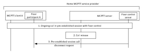
Figure 10.5.3.2.2-1: Disconnect procedure
