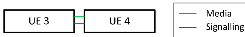
Figure 9.3.1-1: Off-network architectural model for inter-UE communication where no relay function is used
