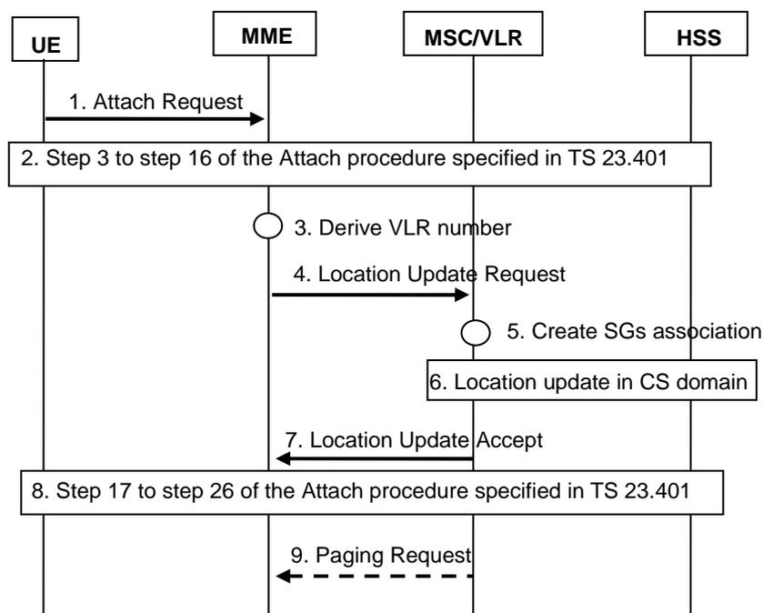
**Figure 5.2-1: Attach Procedure**
