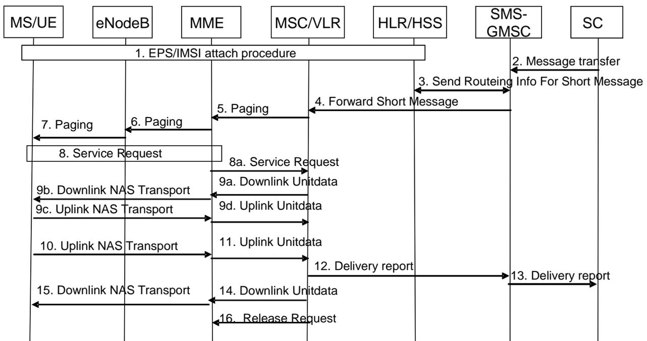
**Figure 8.2.4-1: Mobile terminating SMS in idle mode**
