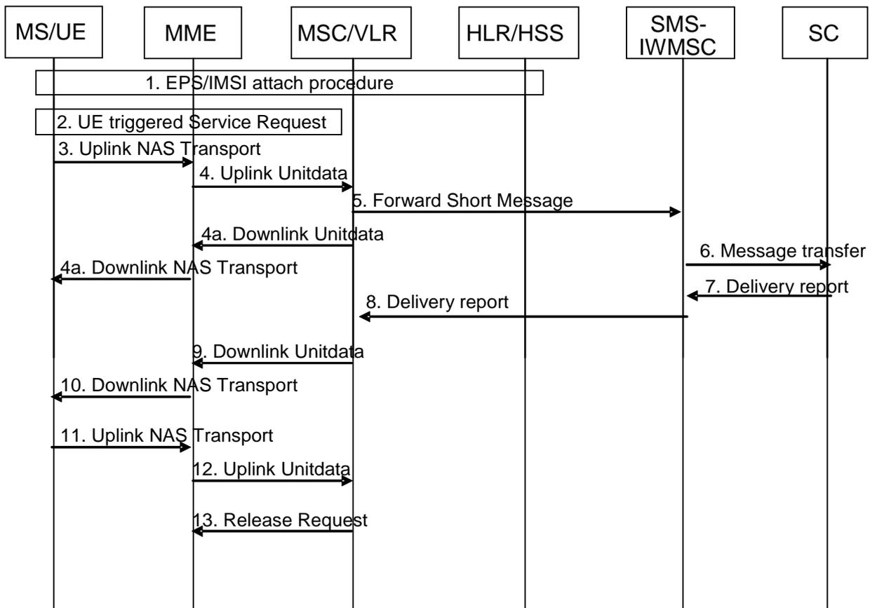
**Figure 8.2.2-1: Mobile originating SMS in idle mode**
