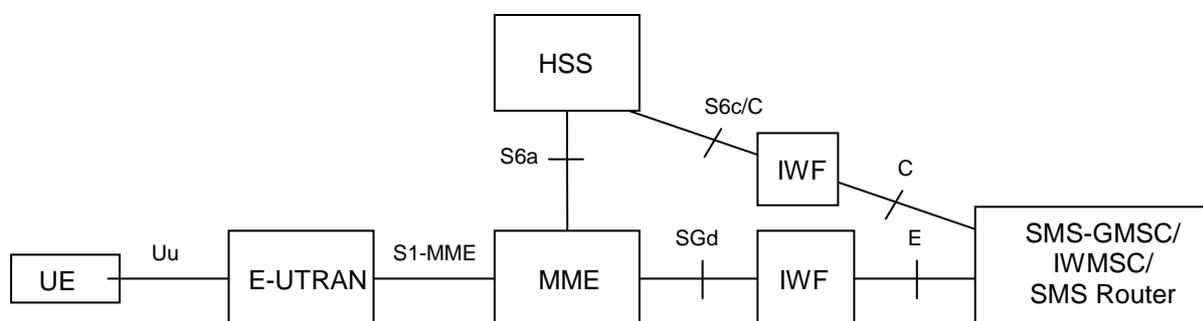
**Figure C.2-2: SMS in MME architecture using IWF**
