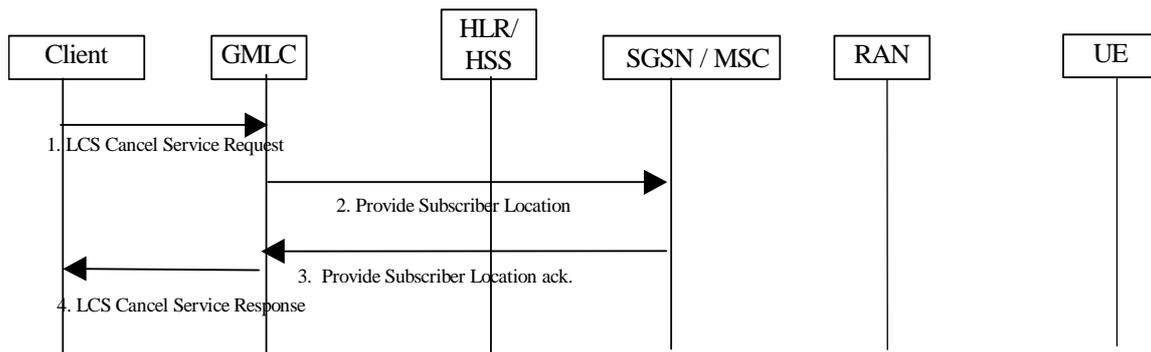
**Figure 9.6c: Cancellation of a Deferred MT-LR procedure**
