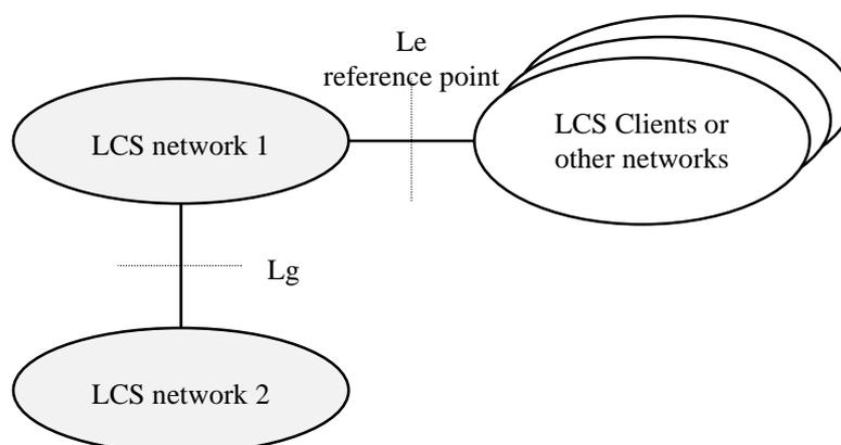
**Figure 5.1: LCS Access Interfaces and Reference Points**
