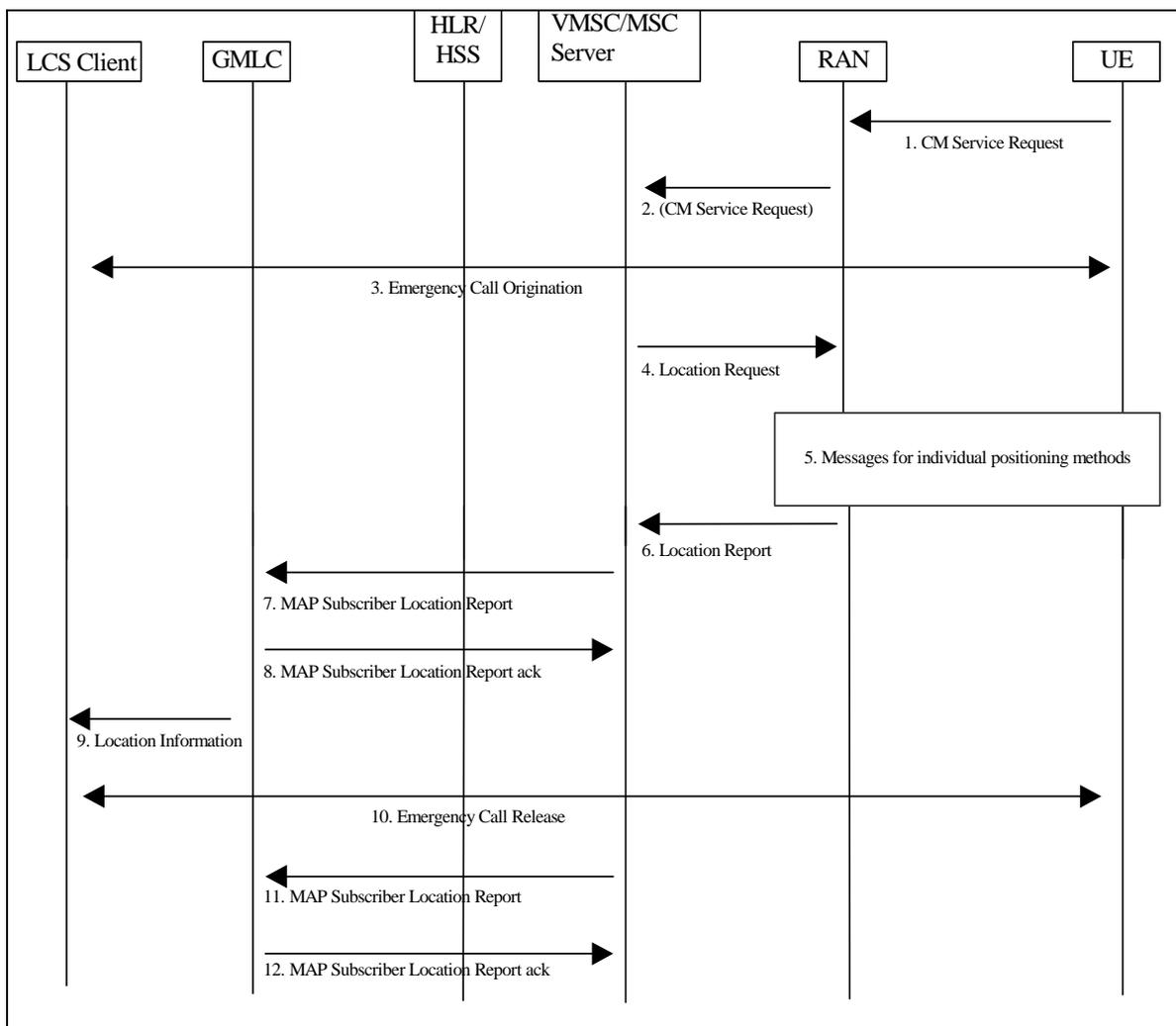
Figure 9.4: Positioning for a NI-LR Emergency Service Call
