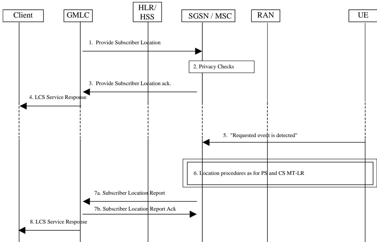
Figure 9.6a: General Network Positioning for a Deferred MT-LR
