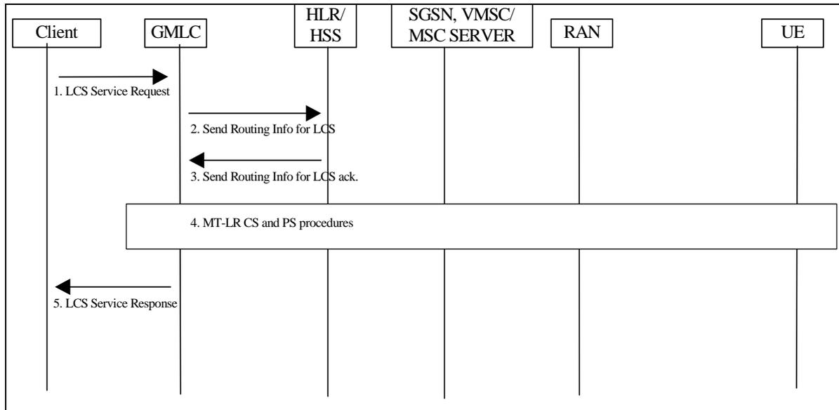
**Figure 9.1: General Network Positioning for a MT-LR**
