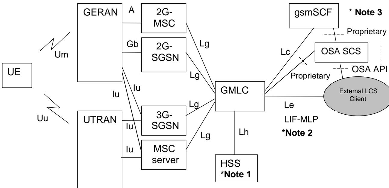
NOTE 1: HSS includes both 2G-HLR and 3G-HLR functionality. LCS is included in the overall network architecture in TS 23.002 [20].
