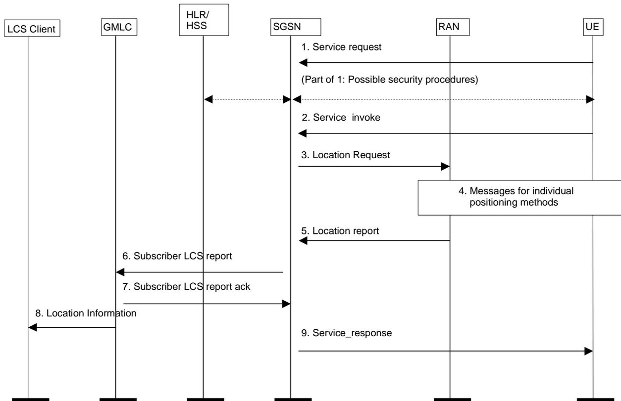
Figure 9.8: General Network Positioning for packet switched MO-LR
