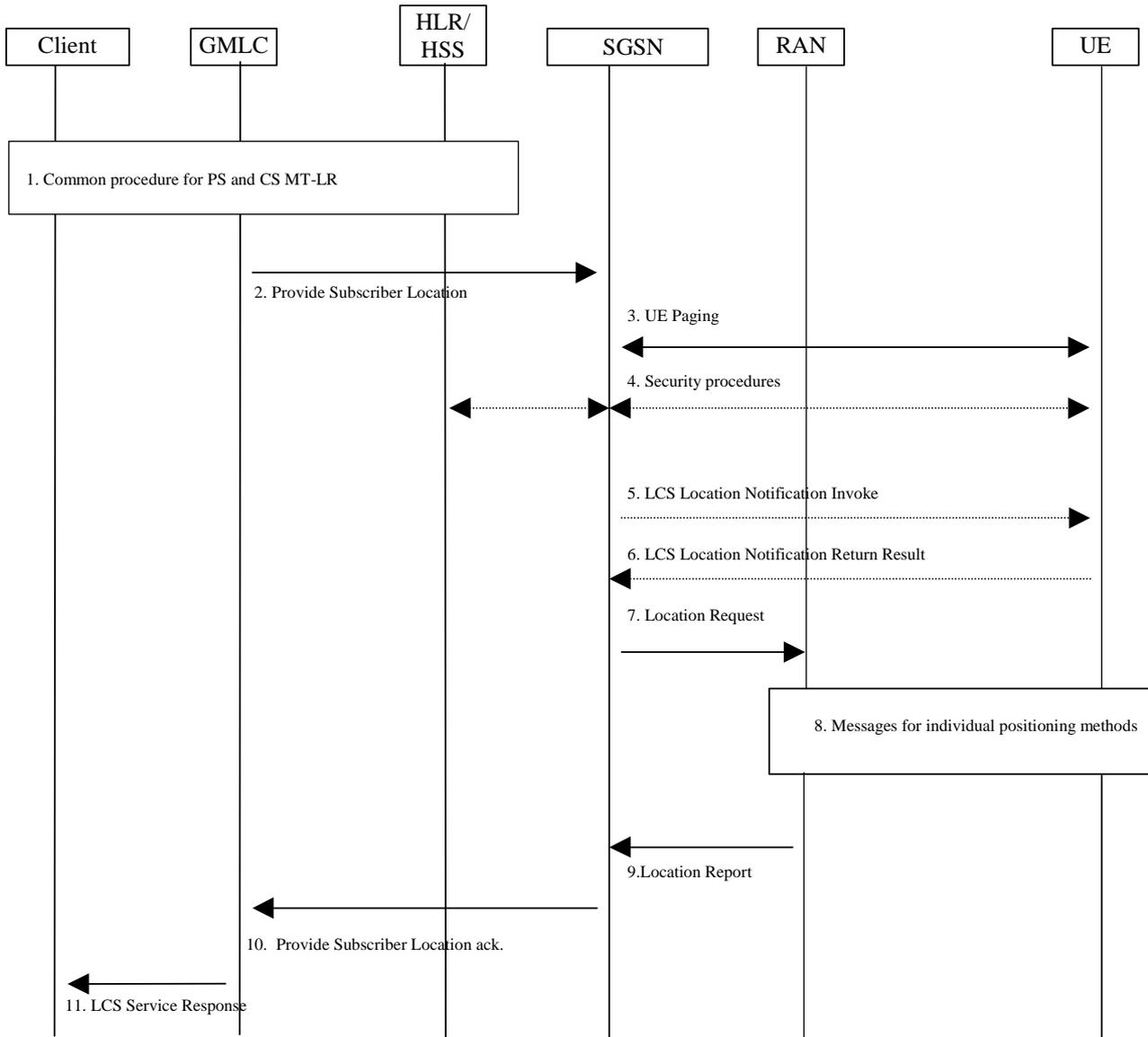
**Figure 9.5: General Network Positioning for Packet Switched MT-LR**
