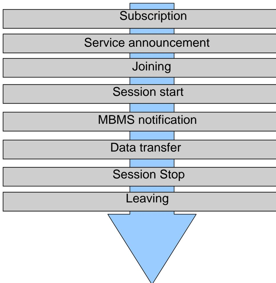
**Figure 2: Phases of MBMS Multicast service provision**
