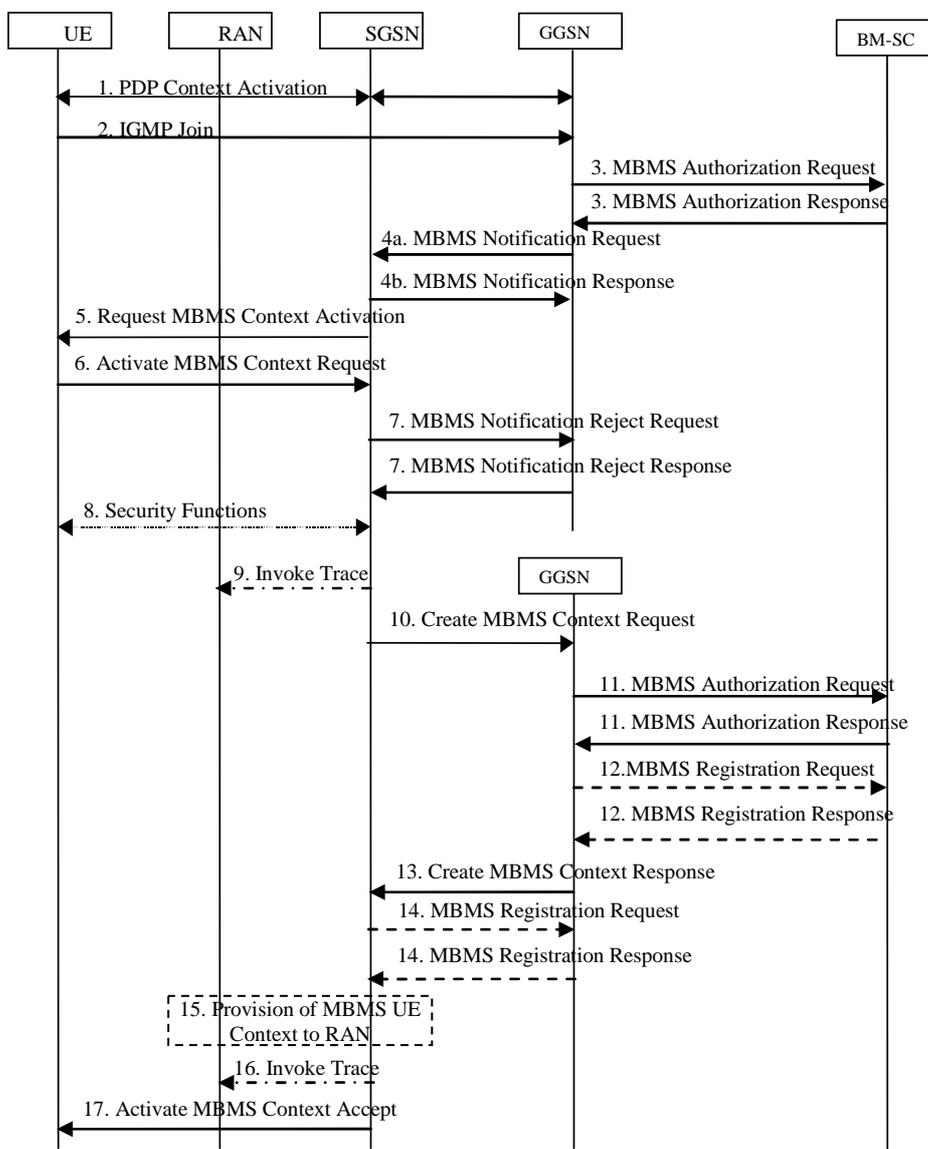
Figure 7: The activation of an MBMS multicast service
