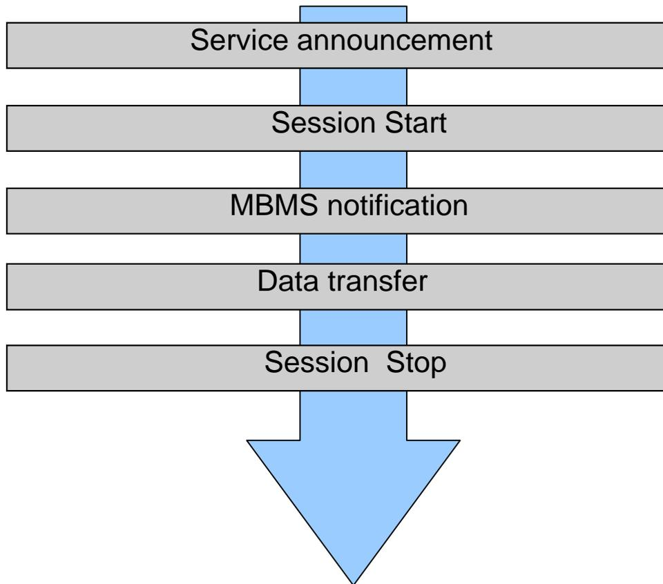
**Figure 4: Phases of MBMS broadcast service provision**
