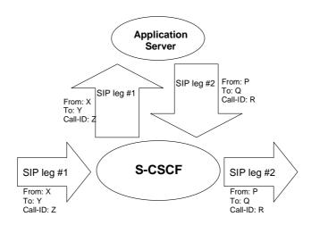
Figure 4.3d: Application Server performing 3<sup>rd</sup> party call control
