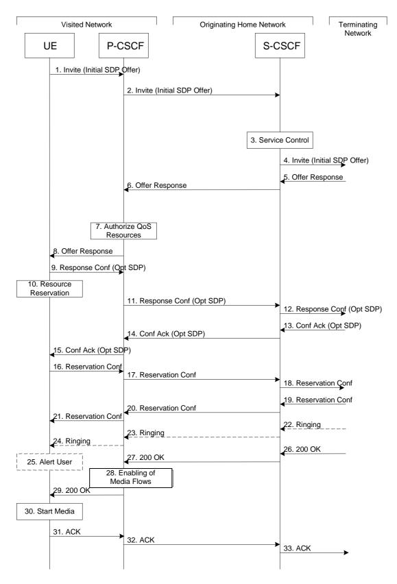
Figure 5.14: Mobile origination procedure - roaming
