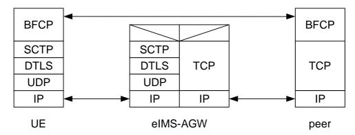
Figure U.1.5.2-1: Protocol architecture for BFCP
