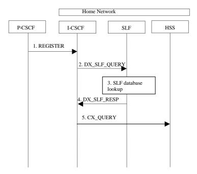
Figure 5.20: SLF on register (1st case)
