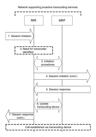
Figure P.1.3.2-1: Proactive transcoding triggering logic
