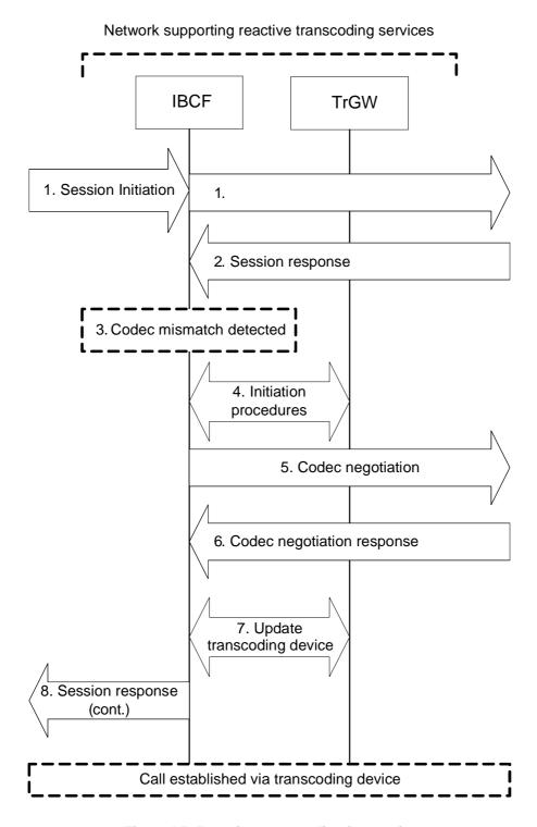
Figure I.5: Reactive transcoding invocation
