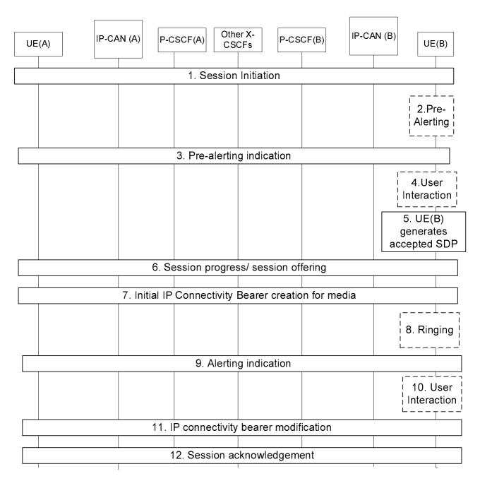
Figure 5.7: Bearer establishment showing optional pre-alerting
