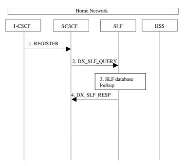
Figure 5.20a: SLF on register (2<sup>nd</sup> case)
