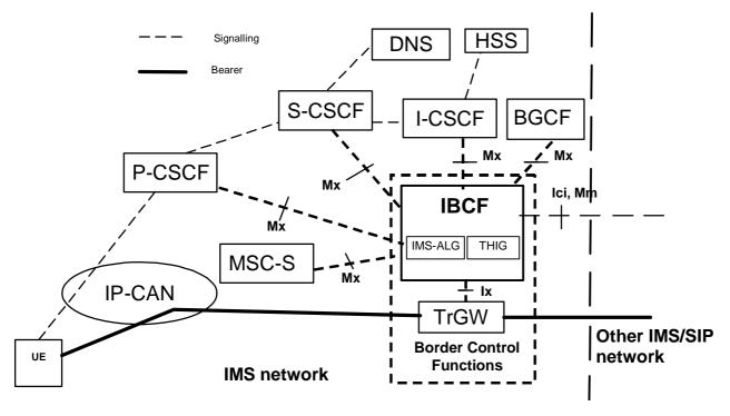
**Figure I.1: Border Control Functions**
