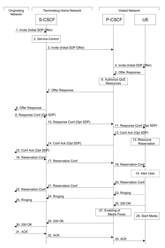
Figure 5.17: Mobile termination procedure - roaming
