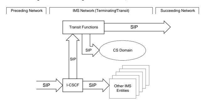
Figure 5.50b: Terminating/Transit IMS network, I-CSCF first
