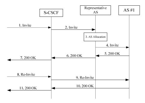
Figure J.2.2: Bypassing Representative AS procedure
