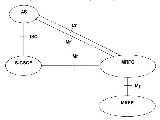
Figure 4.7: Architecture of MRF
