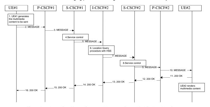
Figure 5.47: Immediate Messaging procedure to registered Public User Identity
