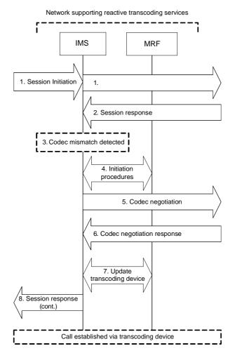
Figure P.1.3.3-1: Reactive transcoding triggering logic
