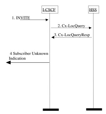
Figure 5.45: HSS determination of unknown user
