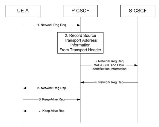
Figure G.7: Flow Establishment Procedures for Outbound
