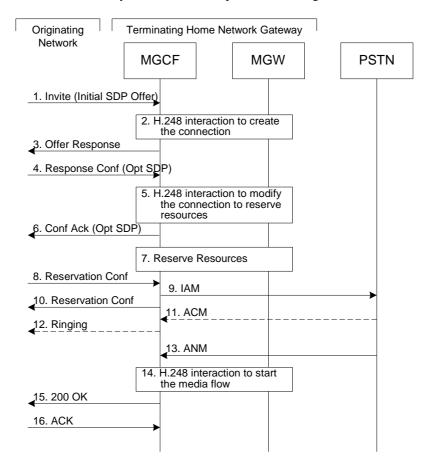
Figure 5.19: PSTN termination procedure
