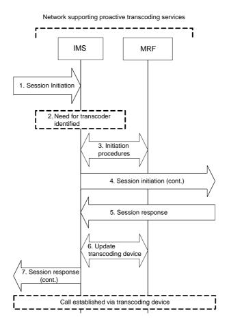
Figure P.1.3.2-1: Proactive transcoding triggering logic
