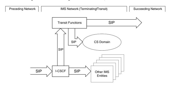
Figure 5.50b: Terminating/Transit IMS network, I-CSCF first
