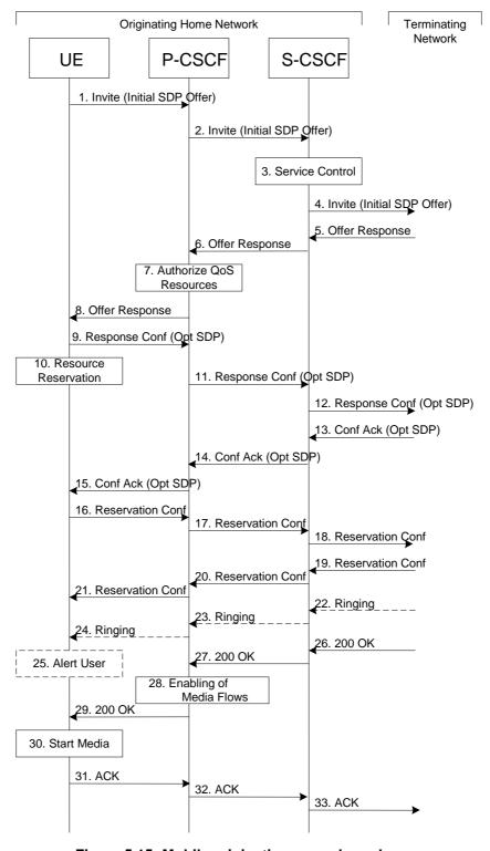
Figure 5.15: Mobile origination procedure - home
