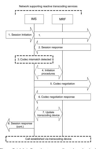
Figure P.1.3.3-1: Reactive transcoding triggering logic
