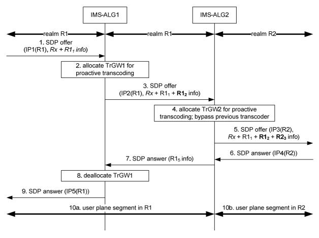
Figure Q.8: IMS-ALG replaces prior proactive transcoder
