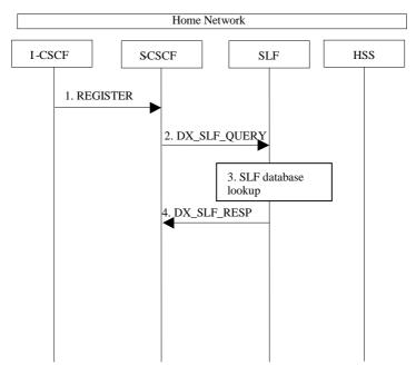
Figure 5.20a: SLF on register (2<sup>nd</sup> case)
