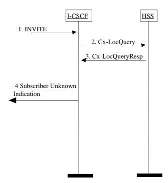
Figure 5.45: HSS determination of unknown user
