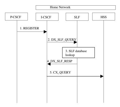
Figure 5.20: SLF on register (1st case)
