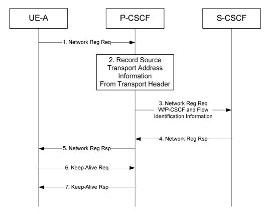
Figure G.7: Flow Establishment Procedures for Outbound
