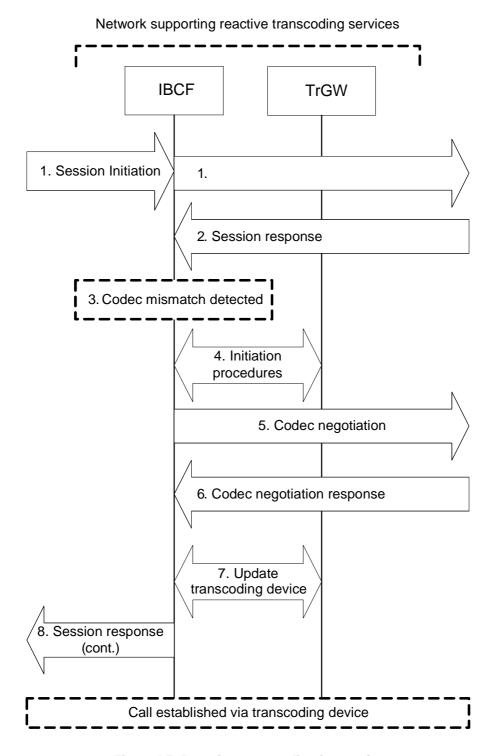
Figure I.5: Reactive transcoding invocation
