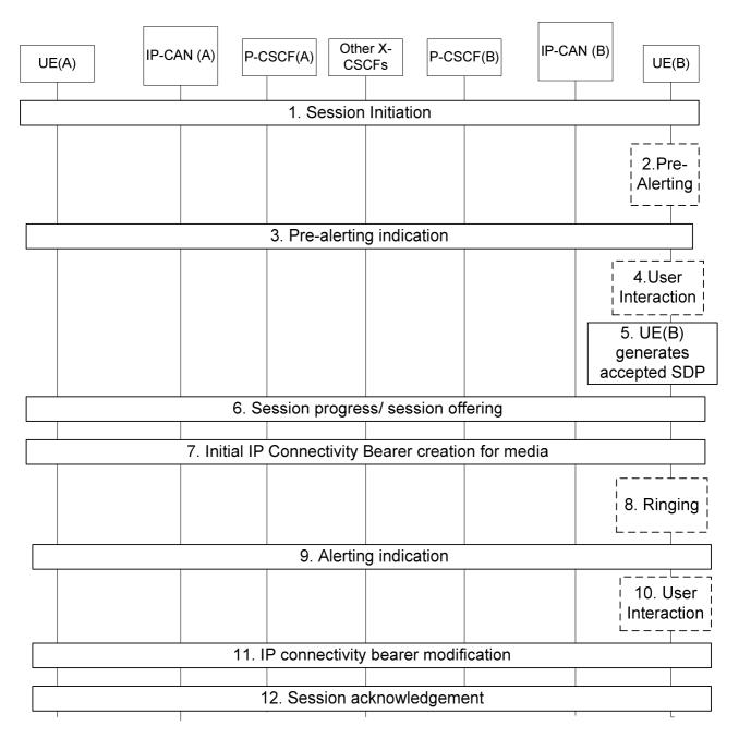
Figure 5.7: Bearer establishment showing optional pre-alerting
