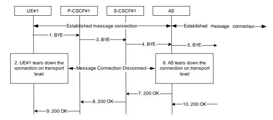
Figure 5.48e: Message session release procedure with intermediate node
