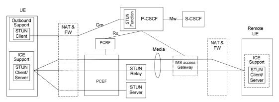
Figure G.2a: Reference model for ICE and Outbound Methodology
