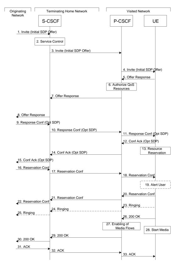
Figure 5.17: Mobile termination procedure - roaming
