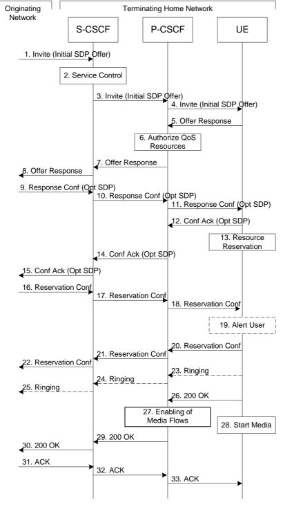
Figure 5.18: Mobile termination procedure - home
