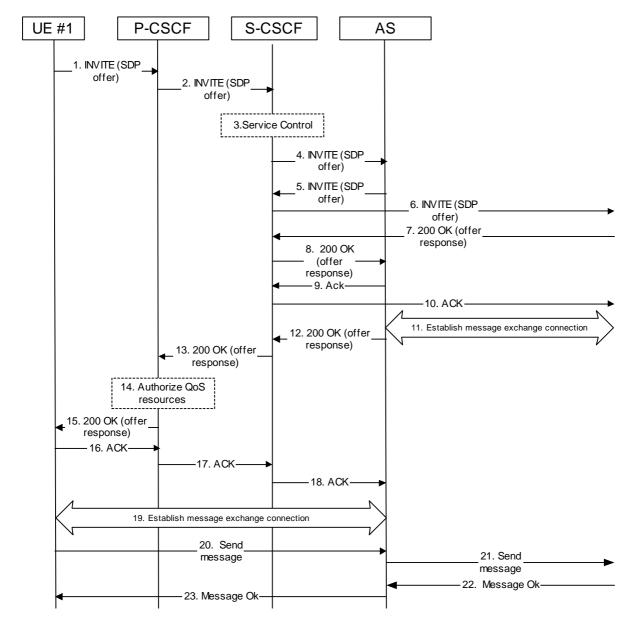
Figure 5.48c: Session based messaging with an intermediate node
