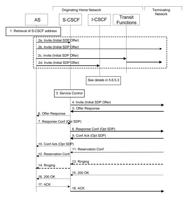
Figure 5.16b: Application Server origination procedure
