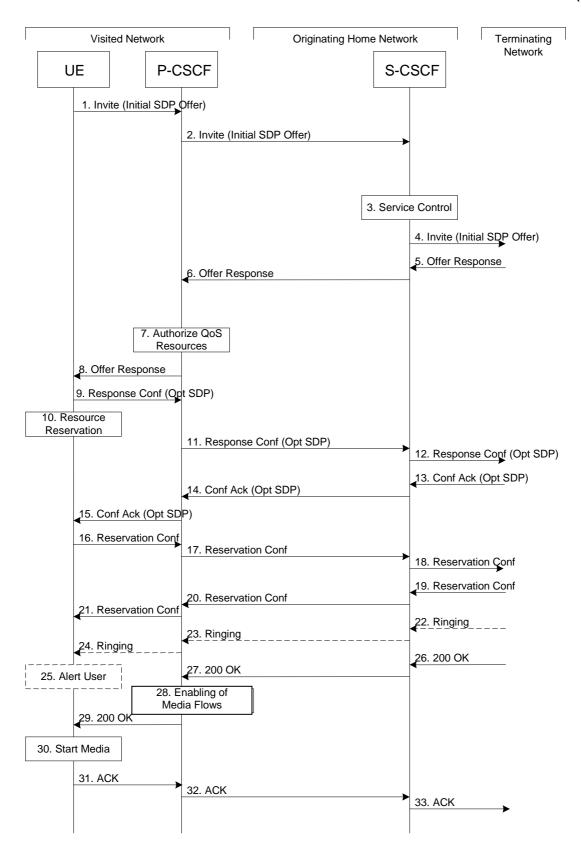
Figure 5.14: Mobile origination procedure - roaming
