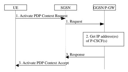
Figure E.1: P-CSCF discovery using PDP Context Activation signalling
