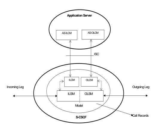
Figure 4.3f: Service Control Model with Incoming Leg Control and Outgoing Leg Control
