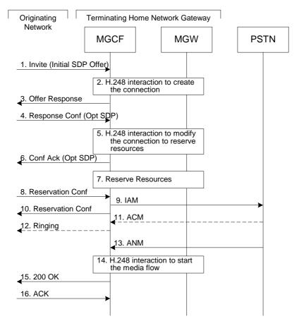
Figure 5.19: PSTN termination procedure
