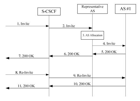
Figure J.2.2: Bypassing Representative AS procedure
