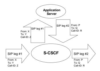
Figure 4.3d: Application Server performing 3<sup>rd</sup> party call control
