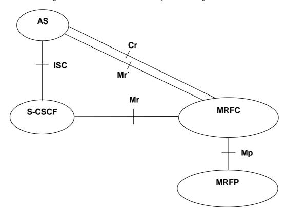
Figure 4.7: Architecture of MRF
