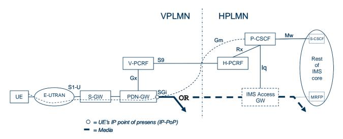
Figure M.2.1.1: Overall architecture for IMS Local breakout with P-CSCF located in home network
