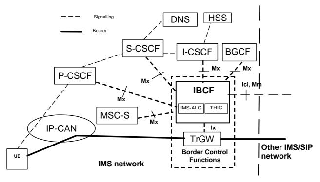
**Figure I.1: Border Control Functions**
