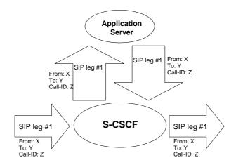
Figure 4.3c: Application Server acting as a SIP proxy
