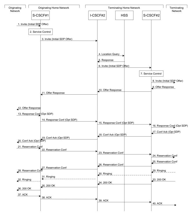
Figure 5.10: Serving to serving procedure - different operators
