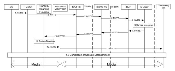
Figure M.3.1.3: Example scenario with P-CSCF located in visited network and with VPLMN routing
