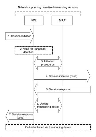
Figure P.1.3.2-1: Proactive transcoding triggering logic
