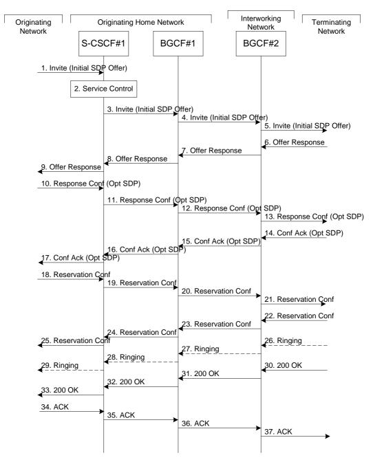
Figure 5.13: Serving to PSTN procedure - different operator
