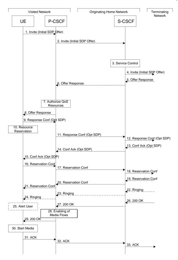
Figure 5.14: Mobile origination procedure - roaming
