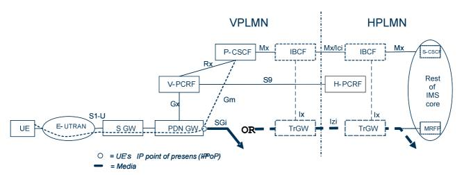
Figure M.1.1.1: Overall architecture for IMS Local Breakout with P-CSCF located in visited network
