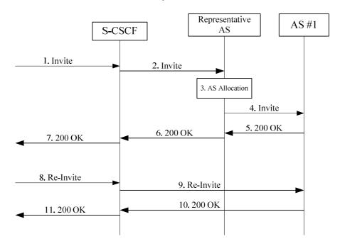
Figure J.2.2: Bypassing Representative AS procedure
