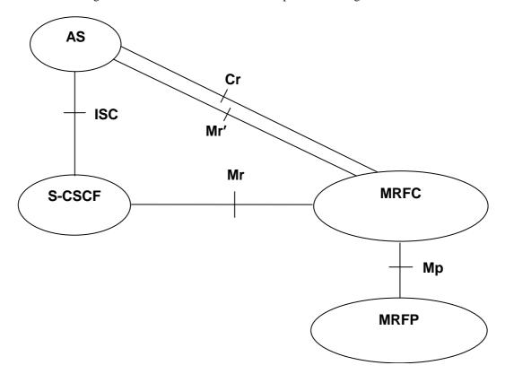
Figure 4.7: Architecture of MRF
