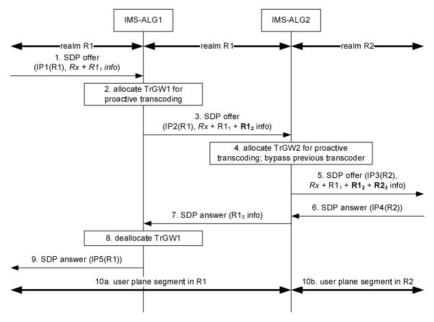
Figure Q.8: IMS-ALG replaces prior proactive transcoder
