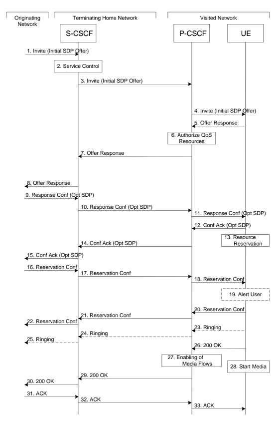
Figure 5.17: Mobile termination procedure - roaming
