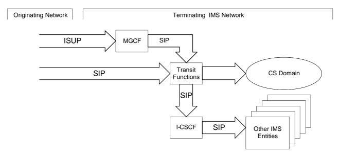
Figure 5.50: Terminating IMS network with transit support, Transit Functions first
