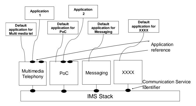
Figure 4.13-1: IMS applications on top of an IMS communication service
