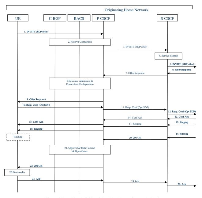
Figure N.1.1: Fixed xDSL originating - home (example flow)
