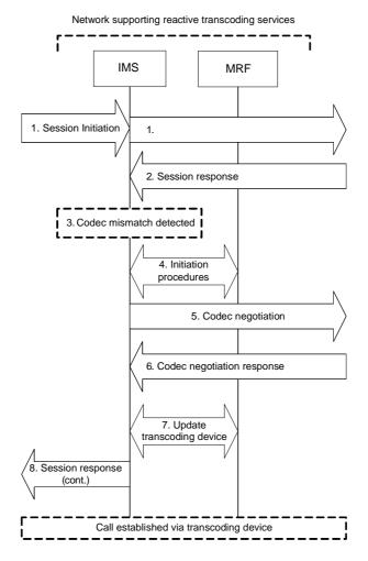
Figure P.1.3.3-1: Reactive transcoding triggering logic
