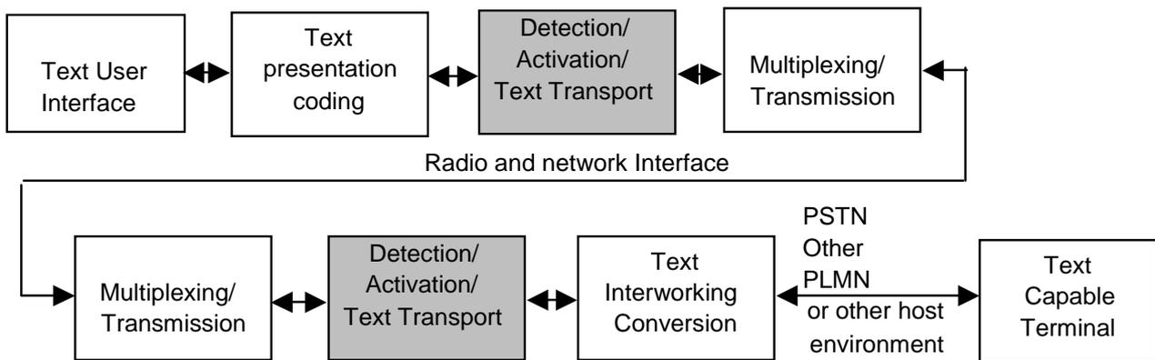
**Figure 3: GTT general text transmission functions showing interworking**
