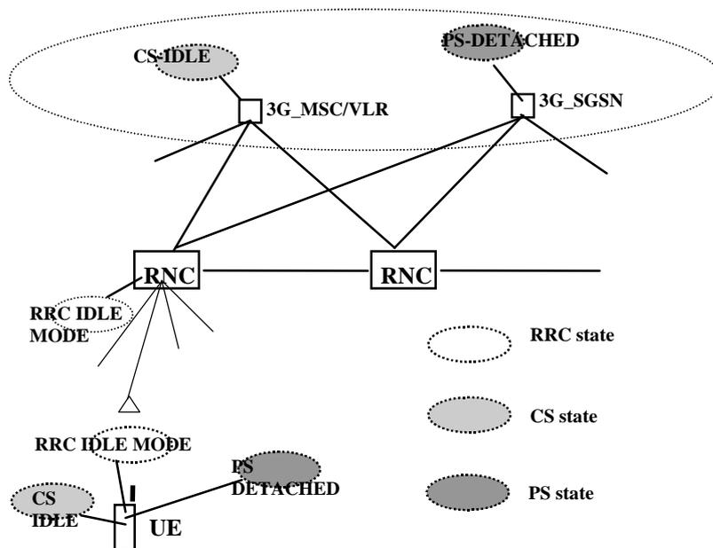
Figure 6.6: UE in CS-IDLE state and PS-DETACHED state
