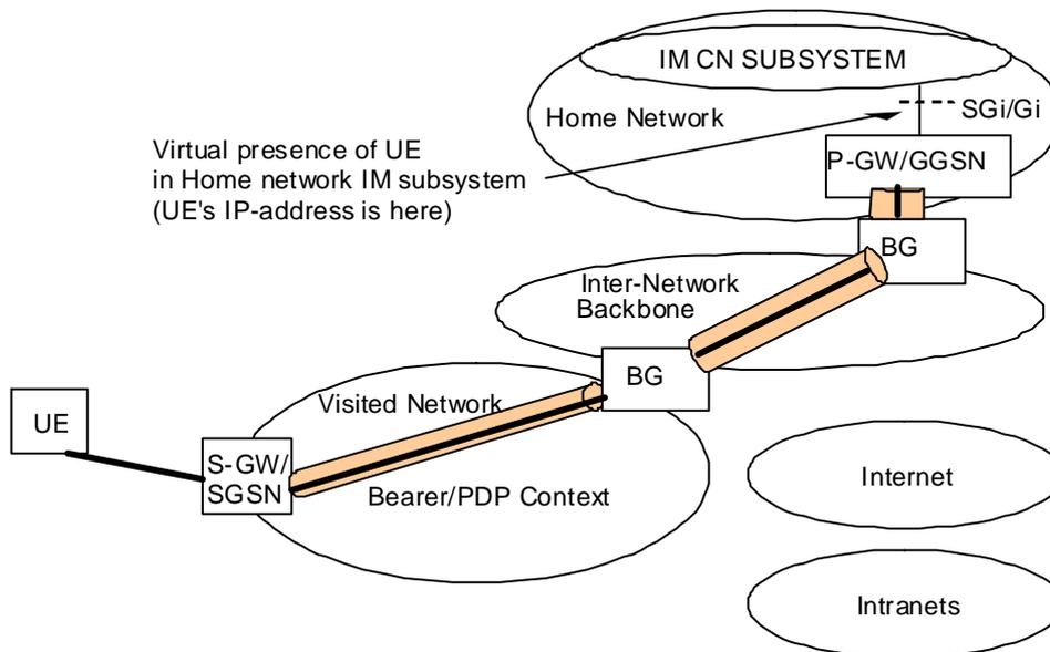
**Figure 5-5a: UE Accessing IM CN subsystem Services with P-GW/GGSN in the Home network**
