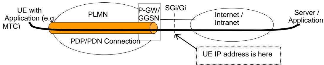
**Figure 5.7-1: UE accessing server/application outside of the PLMN**
