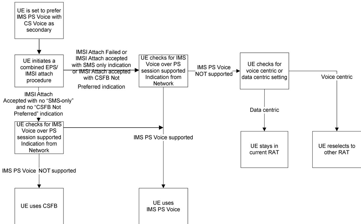
**Figure A.2.2-1: UE behaviour for IMS PS Voice preferred with CS Voice as secondary, combined EPS/IMS attach**
