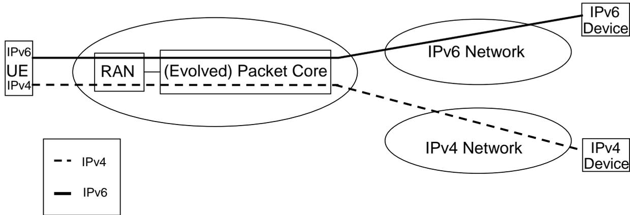
Figure 5-1: UE with IPv4 and IPv6 capability connecting to IPv4 and IPv6 networks
