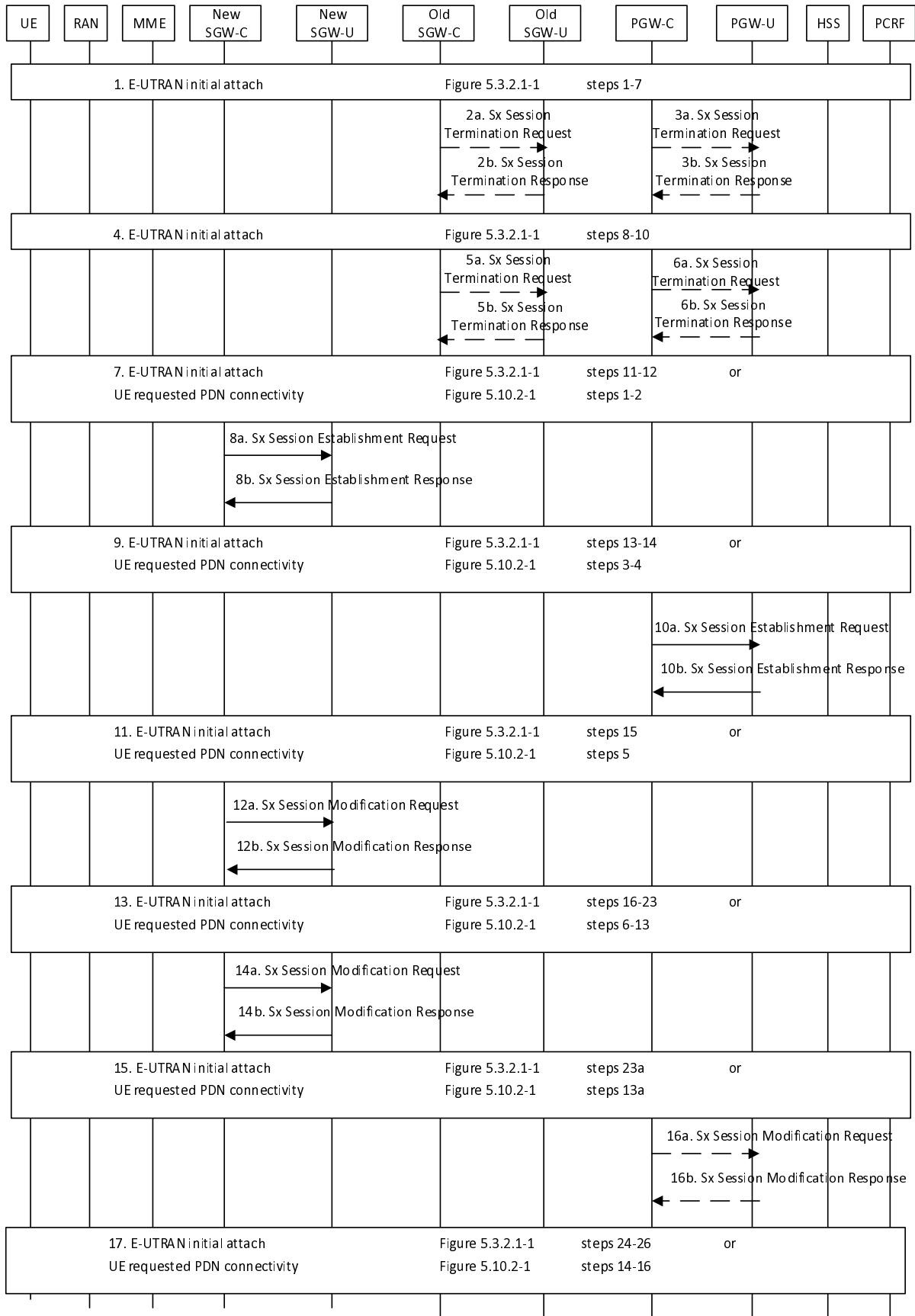
Figure 6.3.1.1-1: Interaction between CP and UP function during PDN connection establishment
