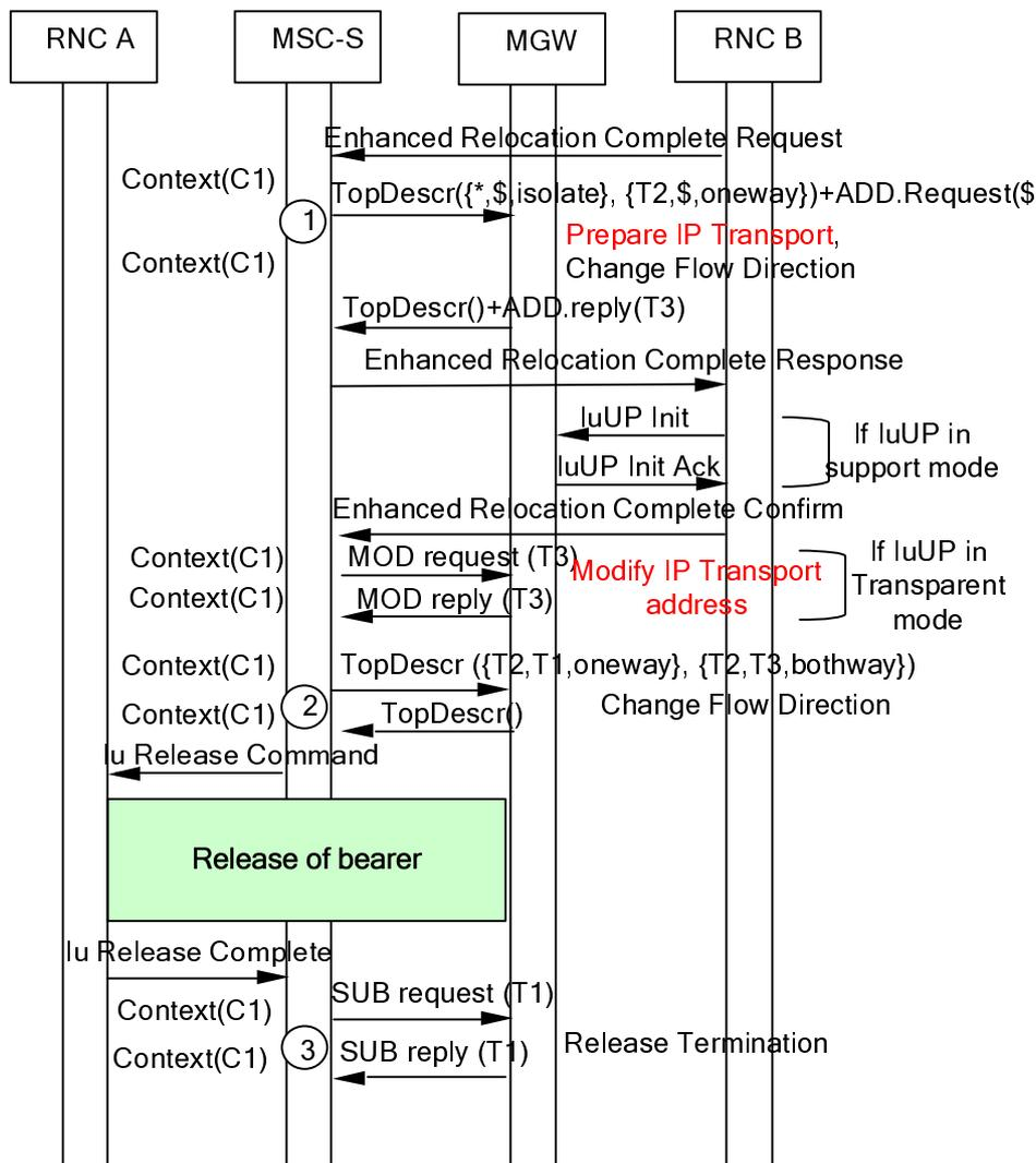
Figure 8.1.7/1 Enhanced SRNS Relocation with Iu on IP
