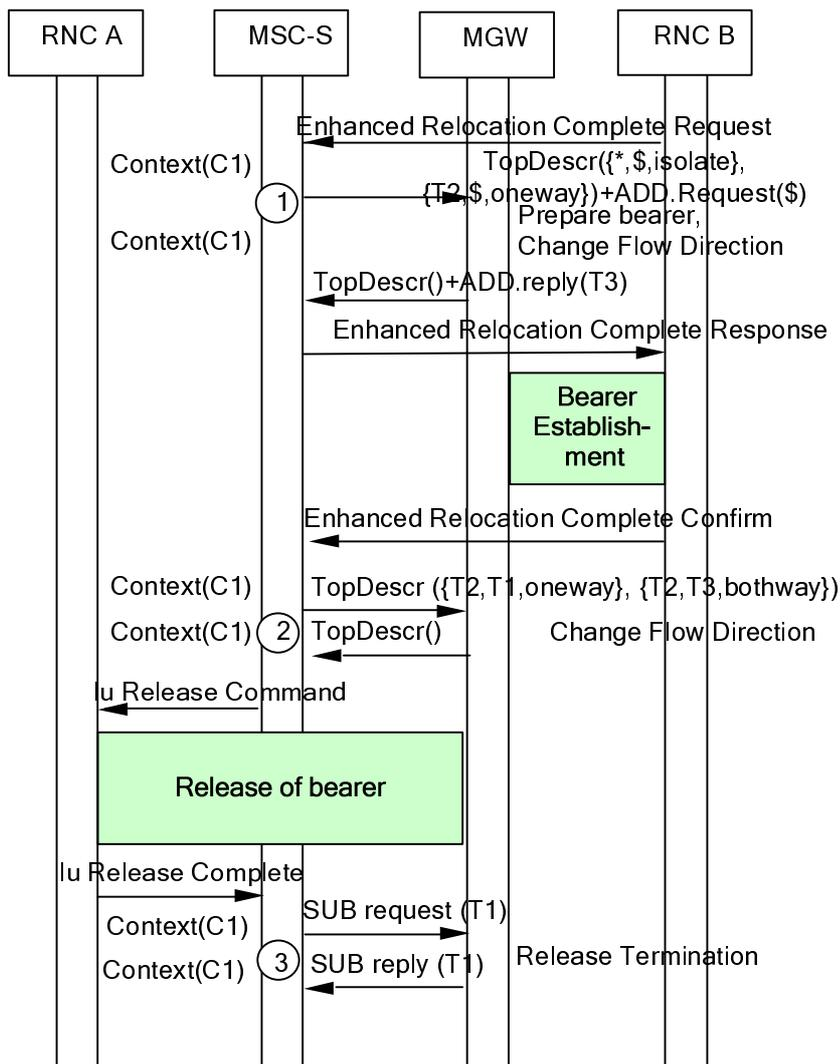
Figure 8.1.6/2: Intra-MSC Enhanced SRNS Relocation (message sequence chart)
