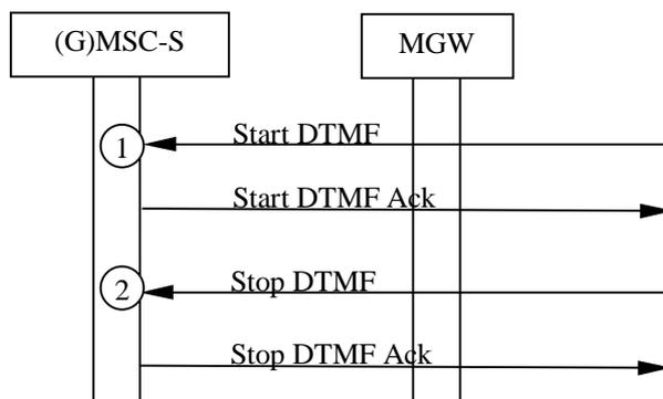
**Figure 14.6: Out-of-Band DTMF detection (message sequence chart)**
