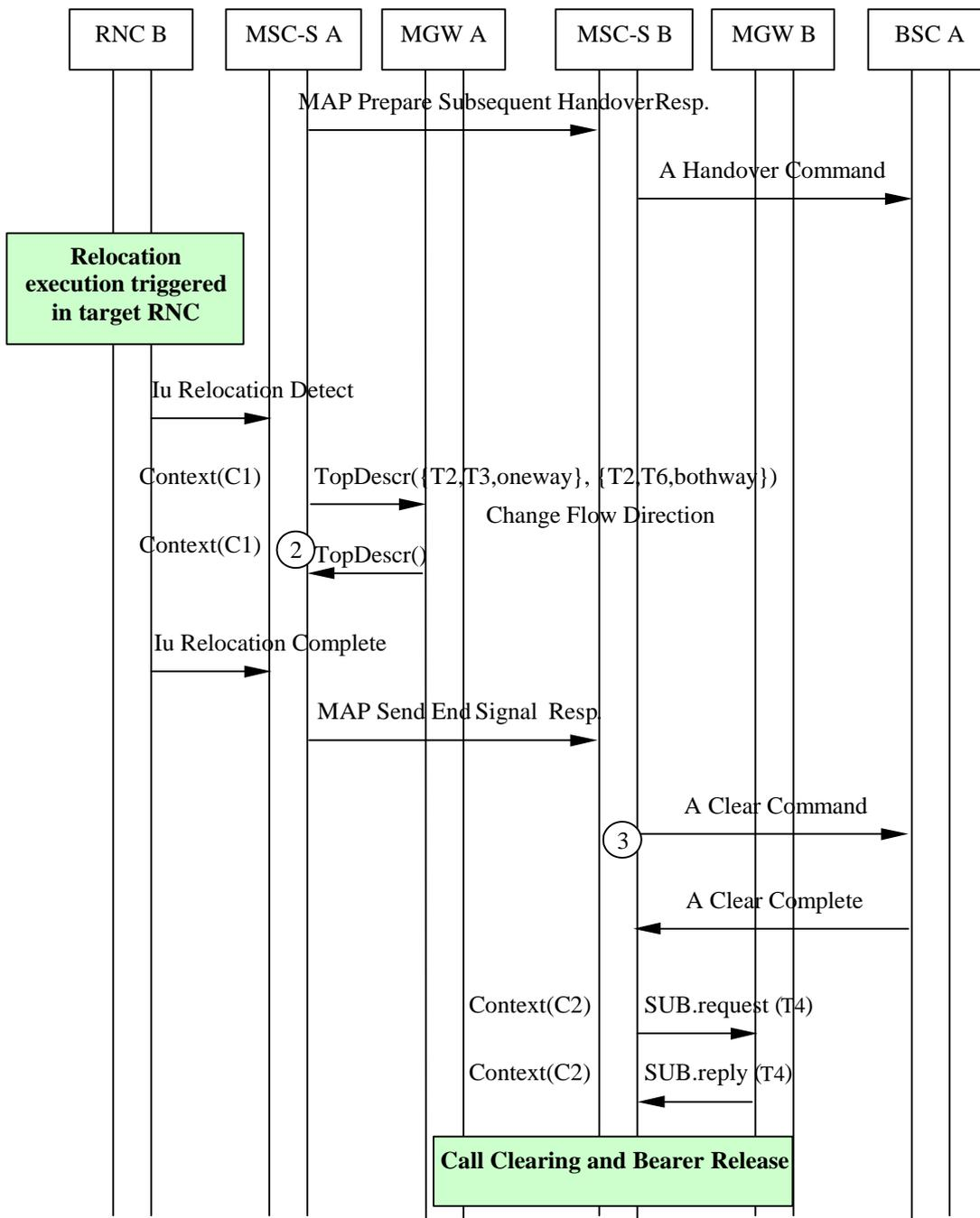
Figure 8.18/2: Subsequent Inter-MSC GSM to UMTS Handover back to the Anchor MSC (message sequence chart)
