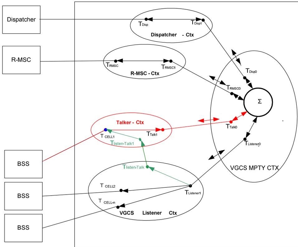
**Figure 13.20.5/3: VGCS call (termination overview for Talker on one channel model)**
