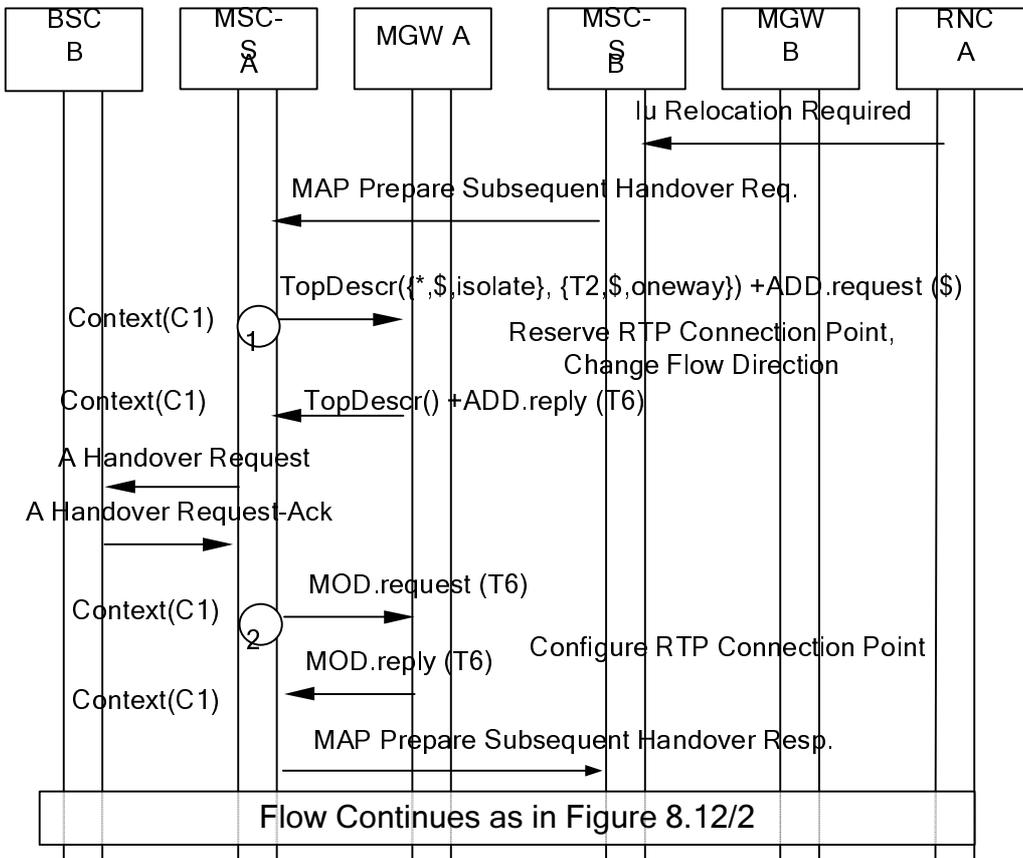
**Figure 8.2.3.c.1: Subsequent Inter-MSC UMTS to GSM Handover back to the anchor MSC for AoIP (message sequence chart)**
