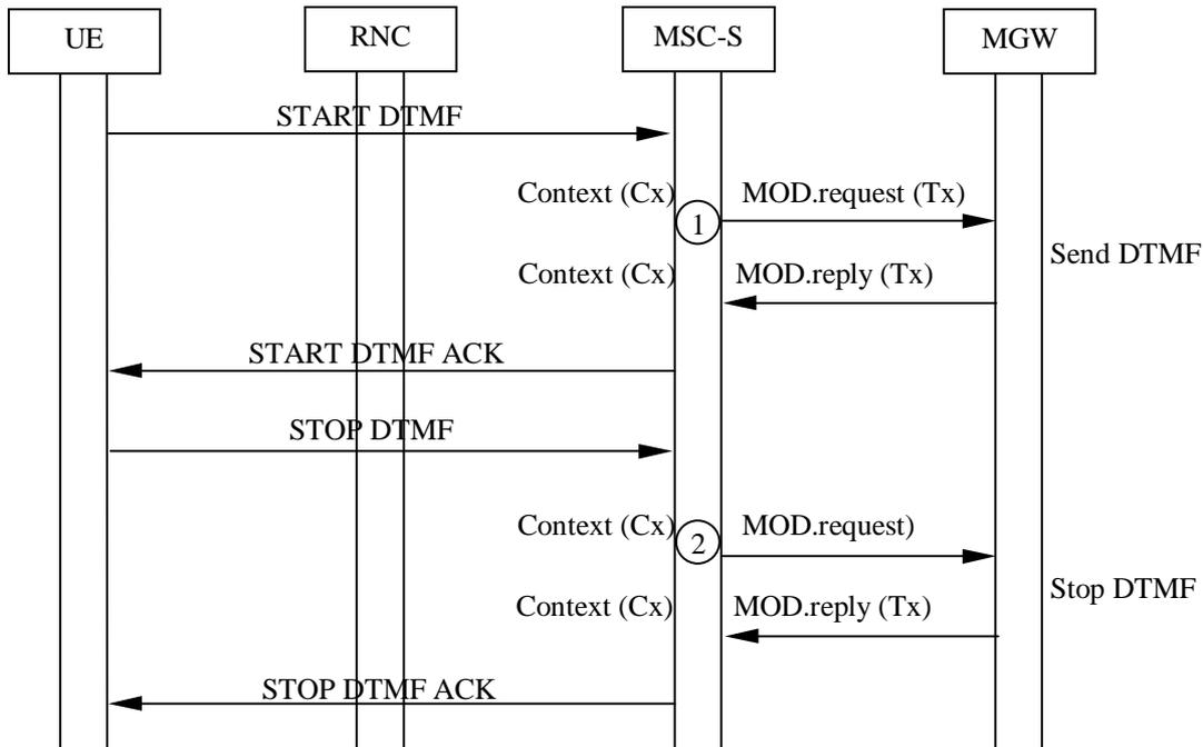
Figure 14.3: Inband DTMF generation (message sequence chart)
