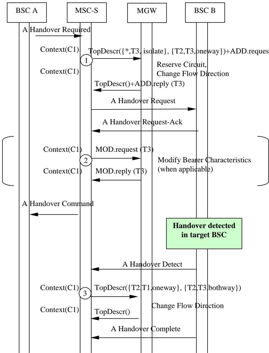
Figure 8.20/1: Intra-MSC GSM to GSM Handover (message sequence chart)
