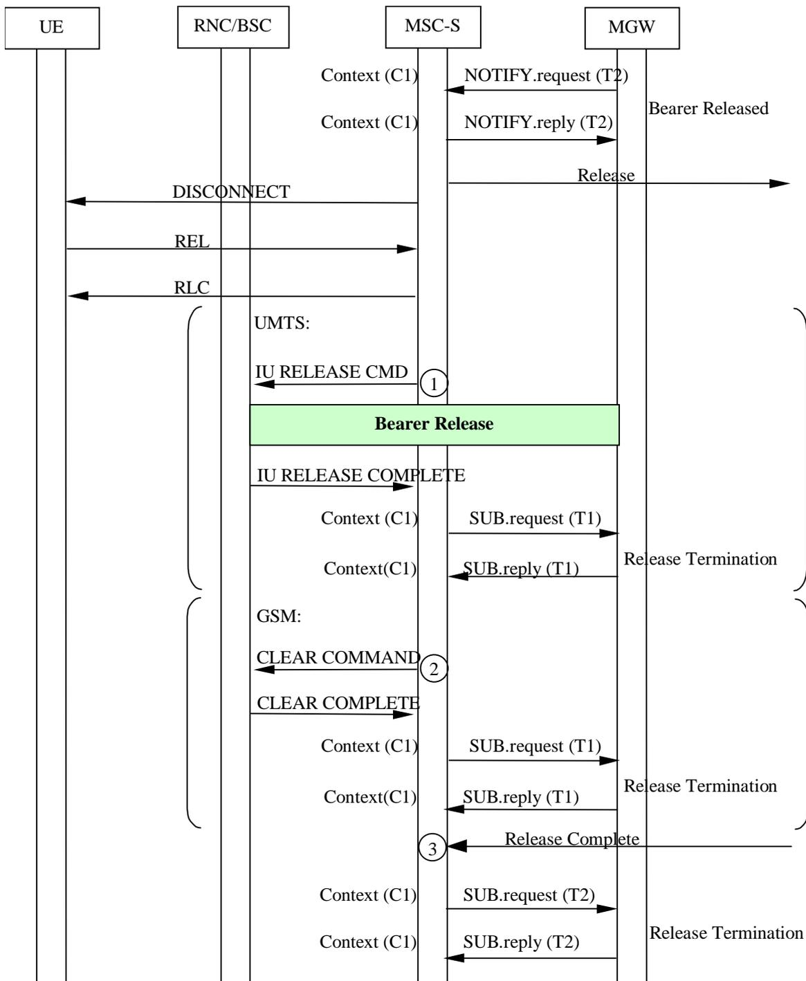
Figure 7.8: MGW Initiated Call Clearing (message sequence chart)
