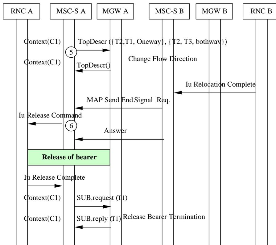
Figure 8.4/2: Basic Inter-MSC SRNS Relocation (message sequence chart)
