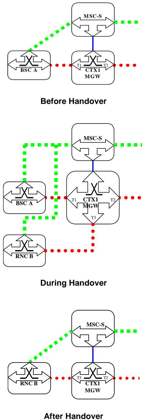
**Figure 8.13: Intra-3G\_MSC GSM to UMTS Handover (network model)**
