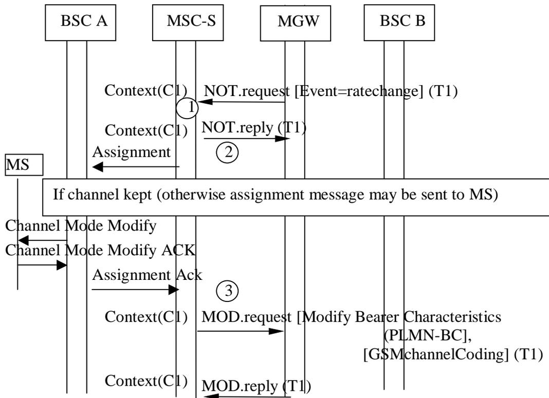
**Figure 13.19/1: GSM access Channel Mode Modify message**
