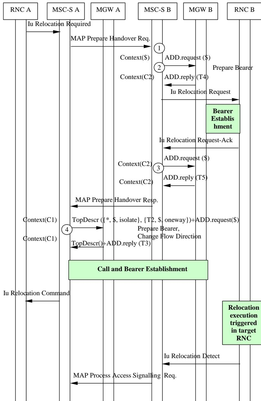
Figure 8.4/1: Basic Inter-MSC SRNS Relocation (message sequence chart)
