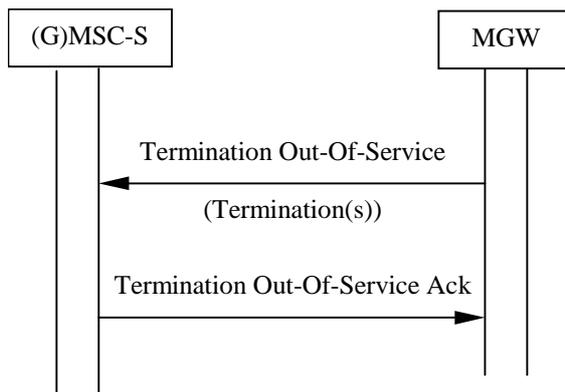
**Figure 10.9: Removal from service of a Physical Termination**
