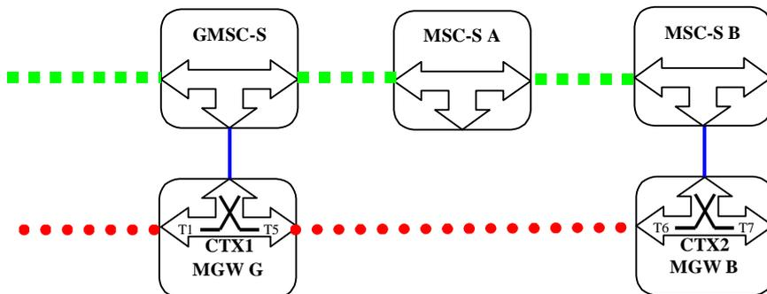
**Figure 17.1B: CFNRy and Bearer Redirect (Network model)**
