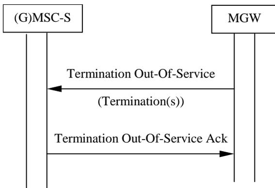
**Figure 10.9: Removal from service of a Physical Termination**
