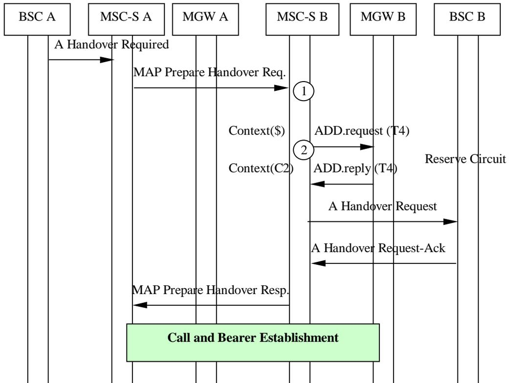
Figure 8.22/1: Basic Inter-MSC GSM to GSM Handover (message sequence chart)
