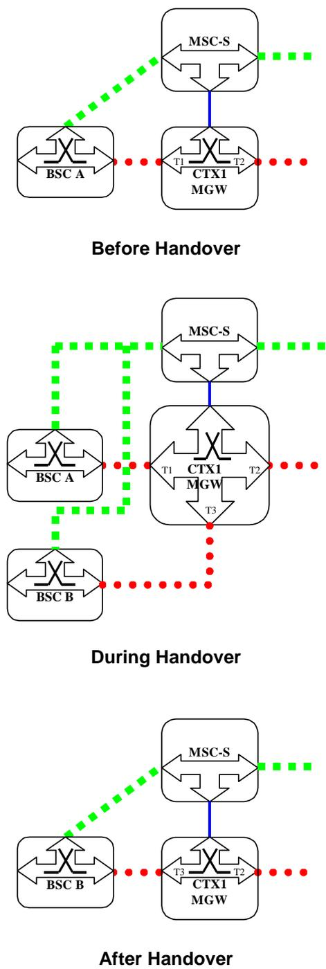
Figure 8.19: Intra-MSC GSM to GSM Handover (network model)
