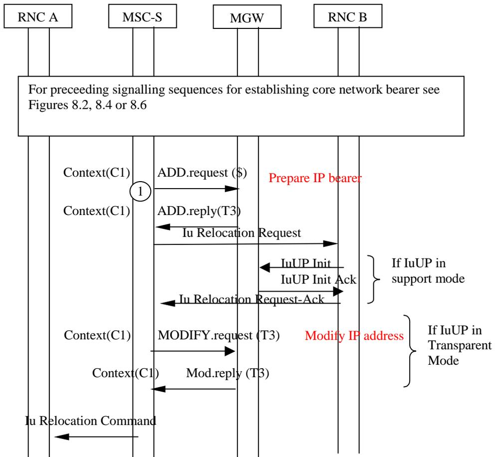
Figure 8.1.5/1 SRNS Relocation with Iu on IP
