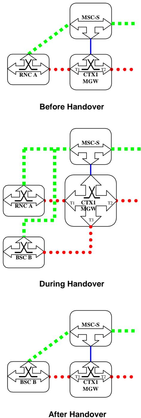
**Figure 8.7: Intra-MSC UMTS to GSM Handover (network model)**
