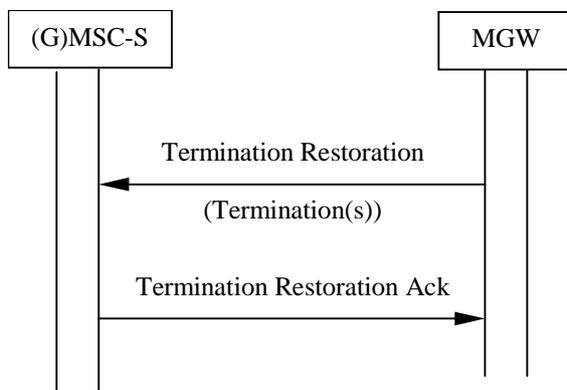
**Figure 10.10: Restoration to service of a Physical Termination**
