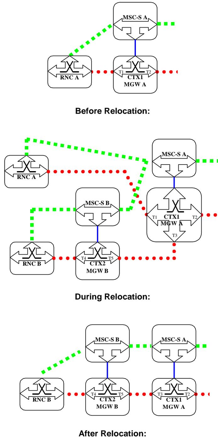
Figure 8.3: Basic Inter-MSC SRNS Relocation (network model)
