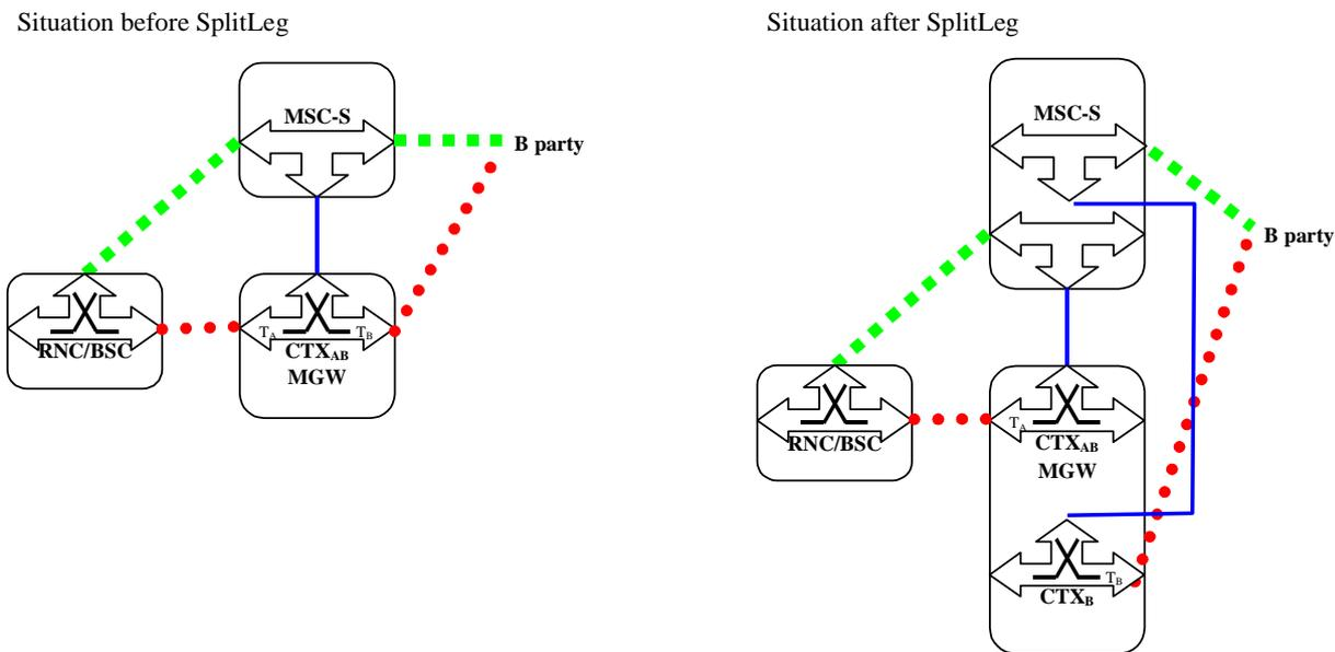
Figure 14. 1.3/5 Split Leg procedure (Network model)
