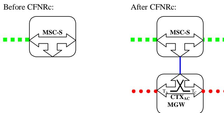
**Figure 13.11: CFNRc; Rerouting by VLR (Network model)**
