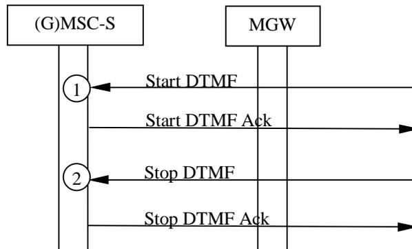
**Figure 14.6: Out-of-Band DTMF detection
