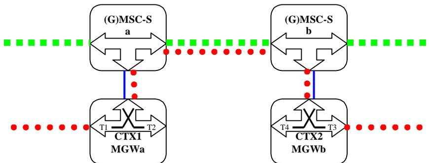
**Figure 15.3: Delayed Backward Tunnelling Transport Mechanism (network model)**
