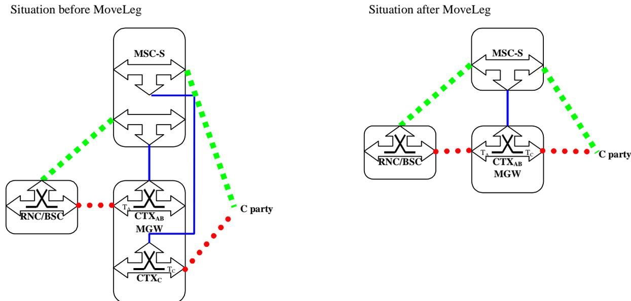
Figure 14. 1.3/3 Move Leg procedure (Network model)
