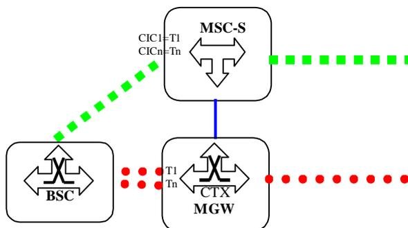
**Figure 9.1 TDM circuits used for A-interface (network model)**
