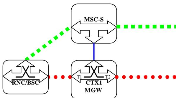
**Figure 7.5: MSC Server Initiated Call Clearing (Network model)**
