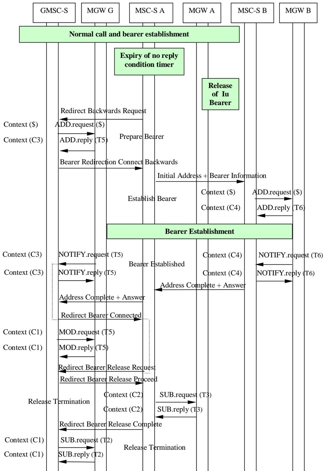
Figure 17.2: Information flow for CFNRy with Bearer Redirect (message sequence chart)
