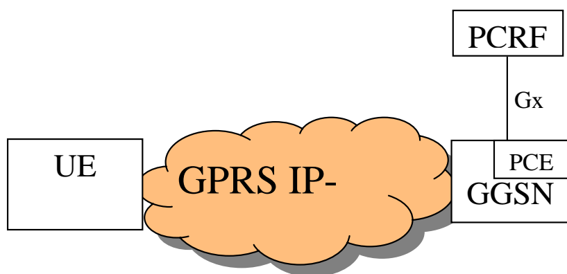
Figure A.1: The GPRS IP-CAN
