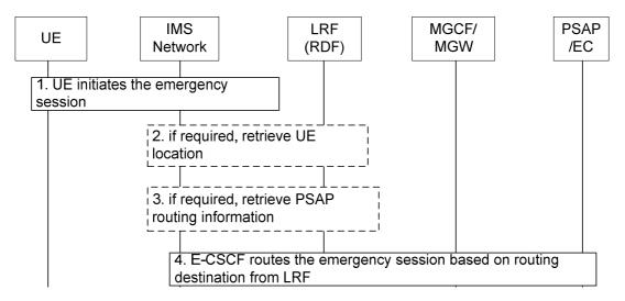
Figure 7.2: Emergency Session Establishment procedure with using LRF/RDF
