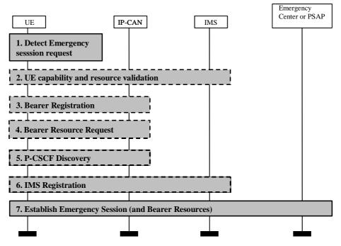
Figure 7.1: Terminal Detected Emergency Calls
