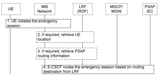
Figure 7.2: Emergency Session Establishment procedure with using LRF/RDF
