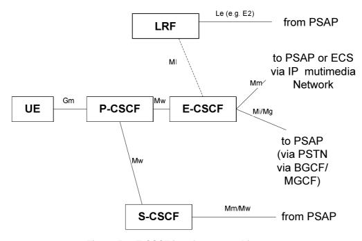
Figure 5.1: E-CSCF in reference architecture
