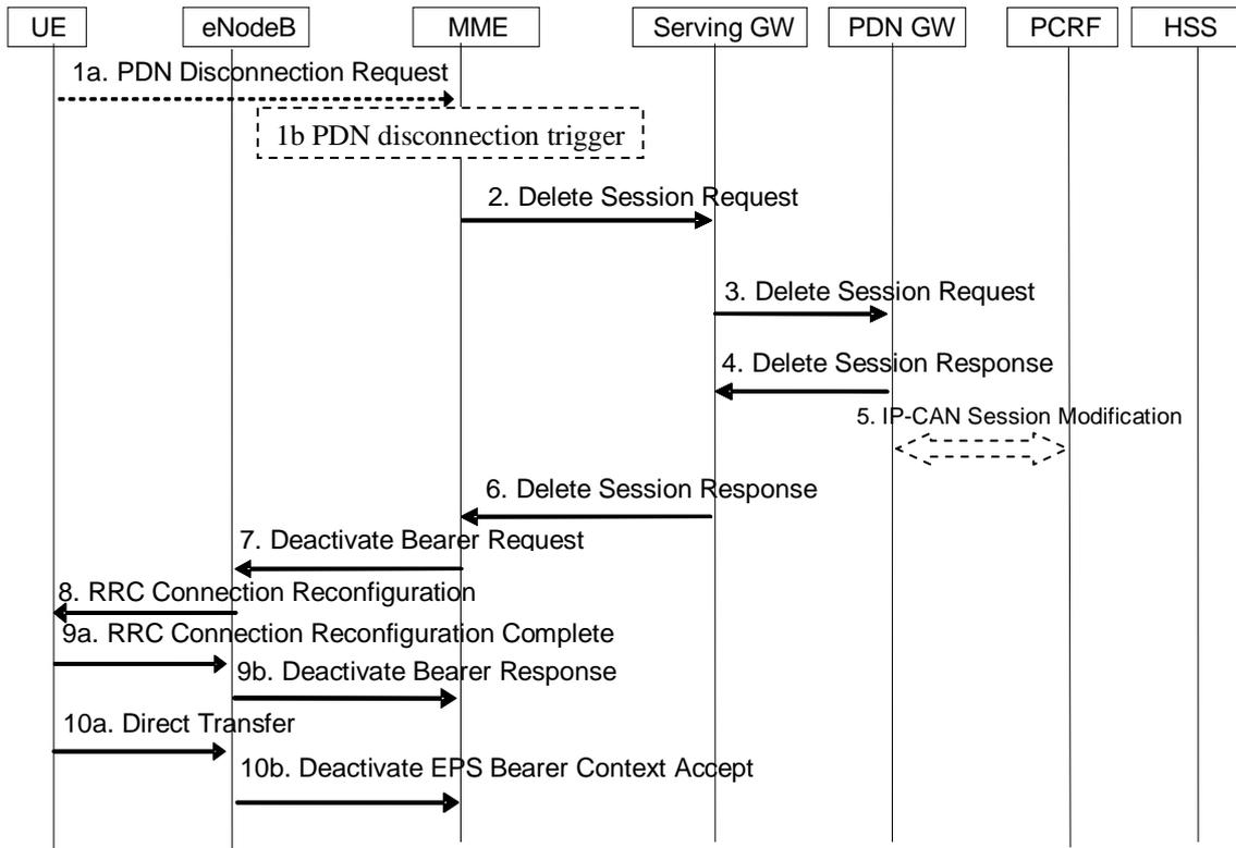
**Figure 6.5.1.1-1: UE-Initiated Removal of 3GPP access via E-UTRAN**
