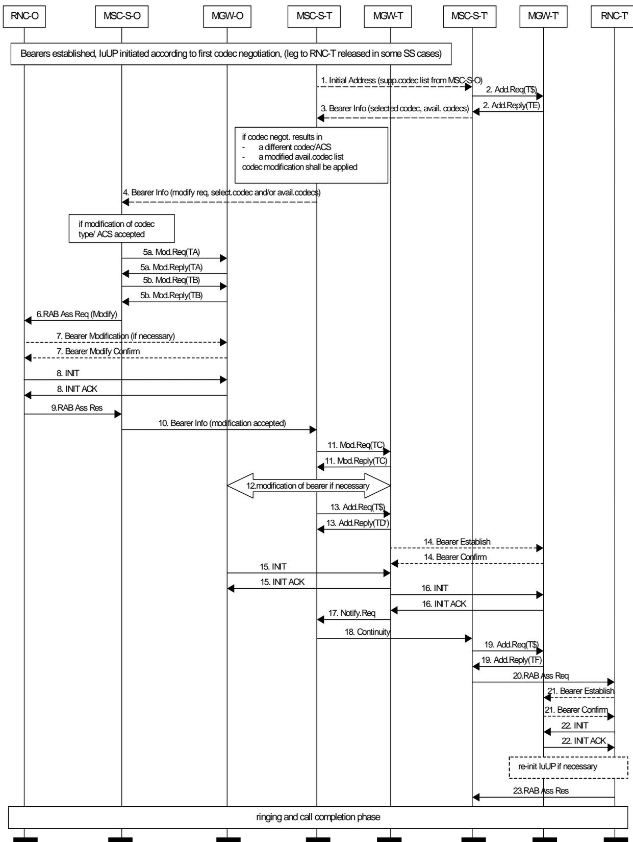
Figure 6.3.1/2: Codec Modification for SS-interworking & UP re-initialisation
