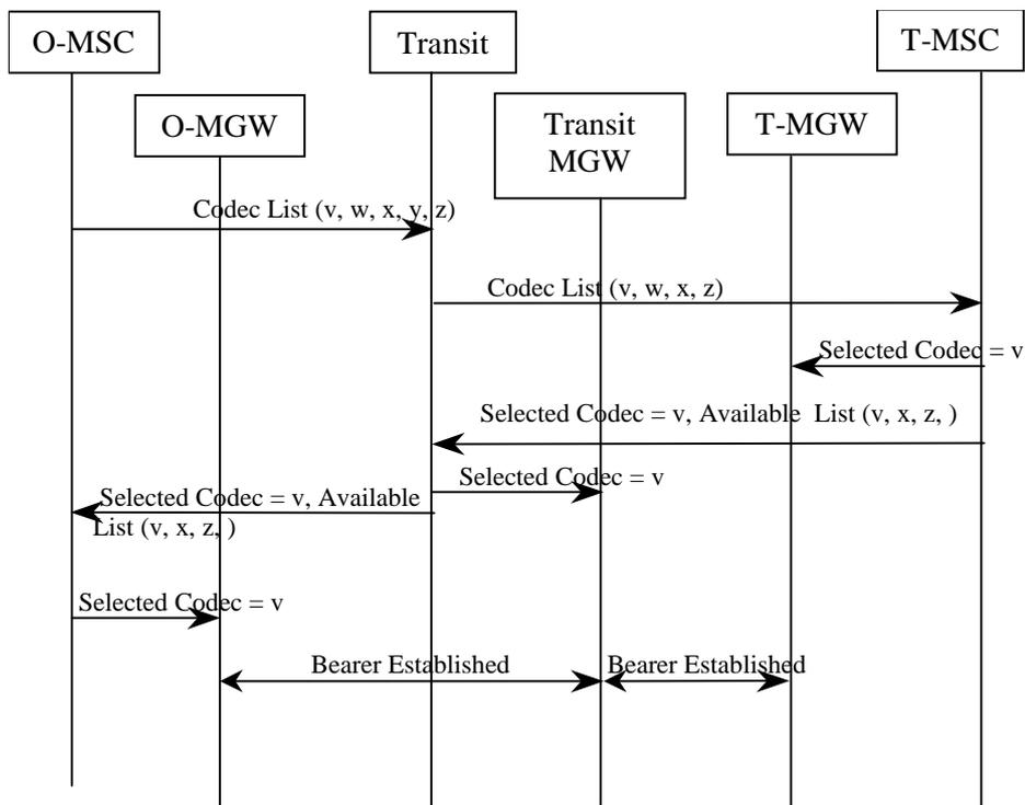
Figure 5.2/1. Basic Codec Negotiation Sequence
