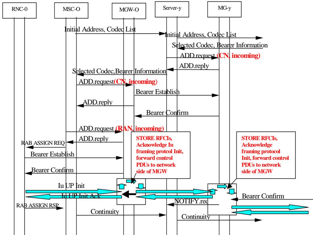
Figure 5.4.1/1: Iu Framing Protocol Establishment, Forward Bearer
