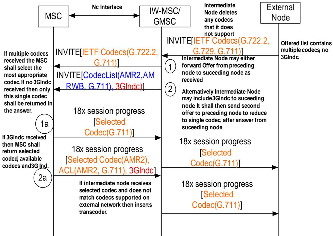
Figure 9.6.7: Mobile Terminating Codec Negotiation with specific codec examples
