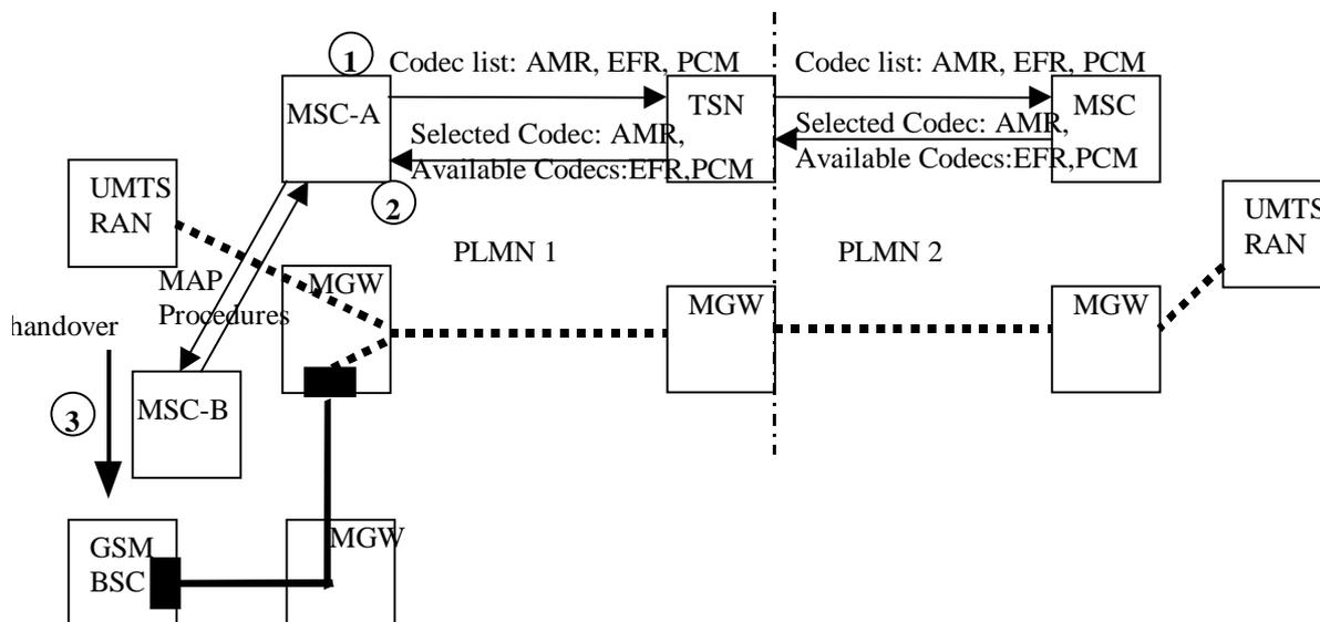
Figure 6.5/2: Inter-MSC, UMTS to GSM handover
