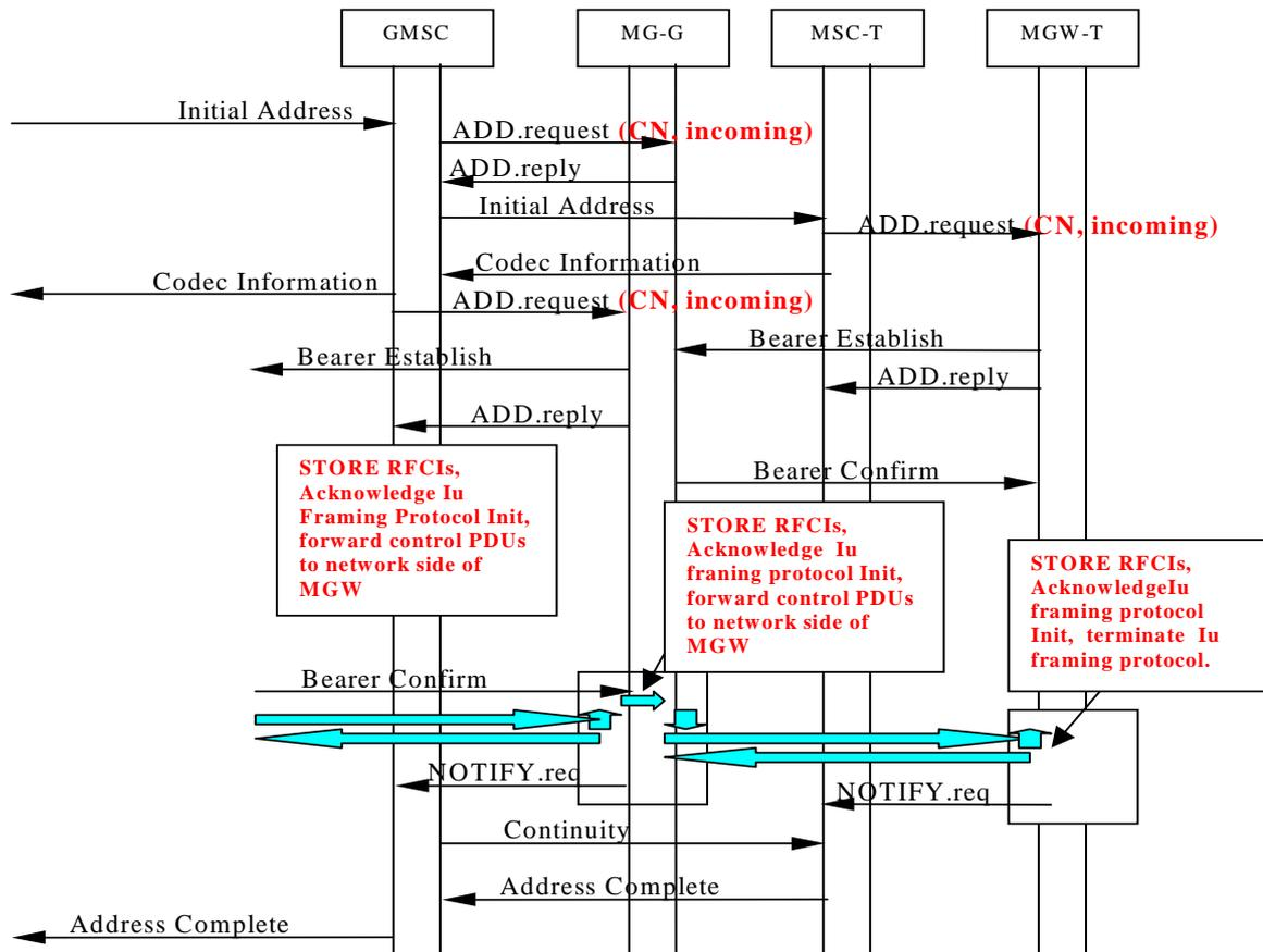
Figure 5.4.1/2: Iu Framing Protocol Establishment, backward bearer.
