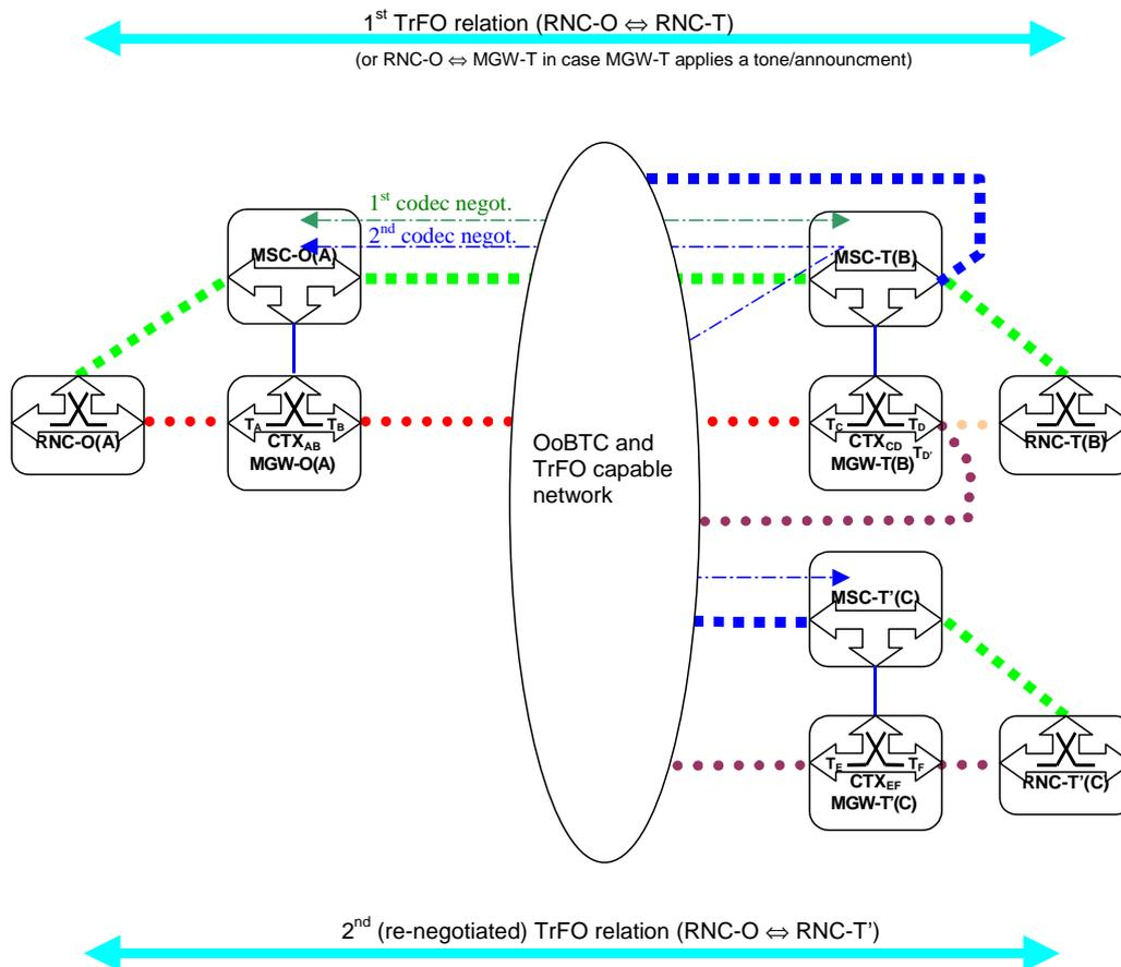
**Figure 6.3.1/1. Codec Modification in case of SS interworking**
