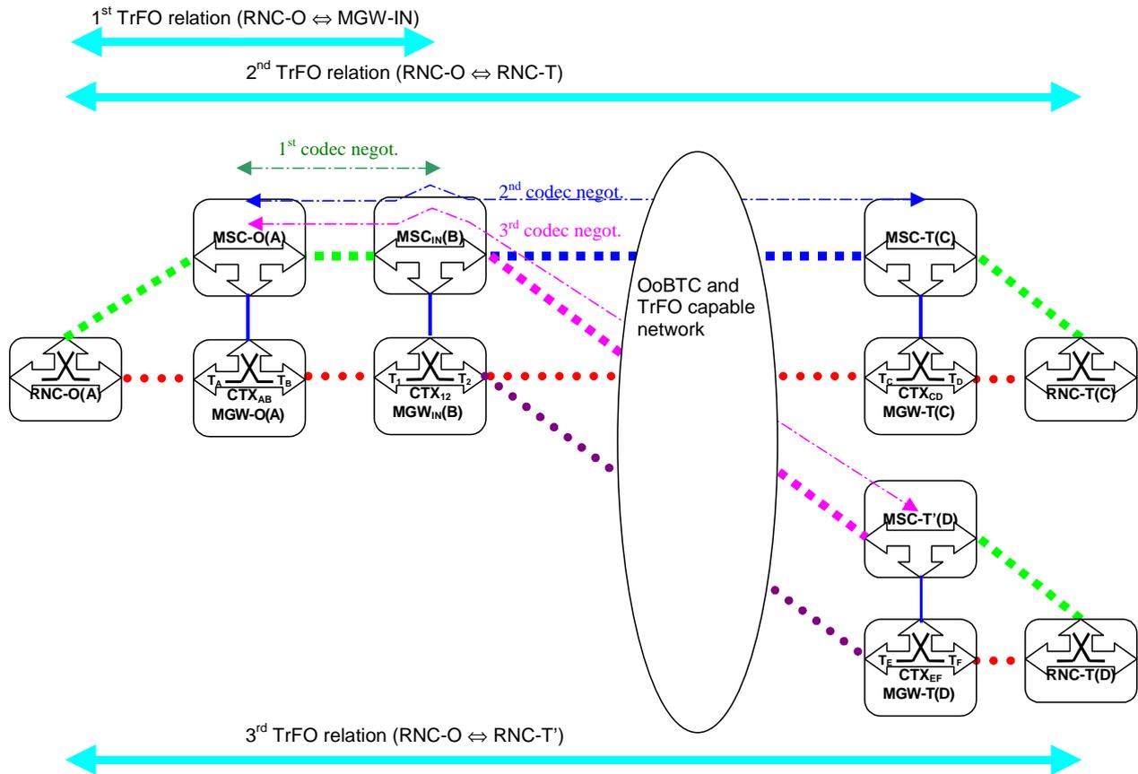
**Figure 6.3.2/1. Codec Modification in case of IN interworking**
