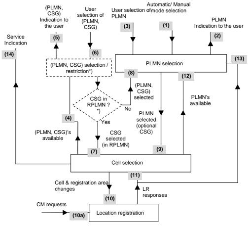
\*) dashed parts apply only for MEs supporting CSGs and are executed for manual CSG selection
