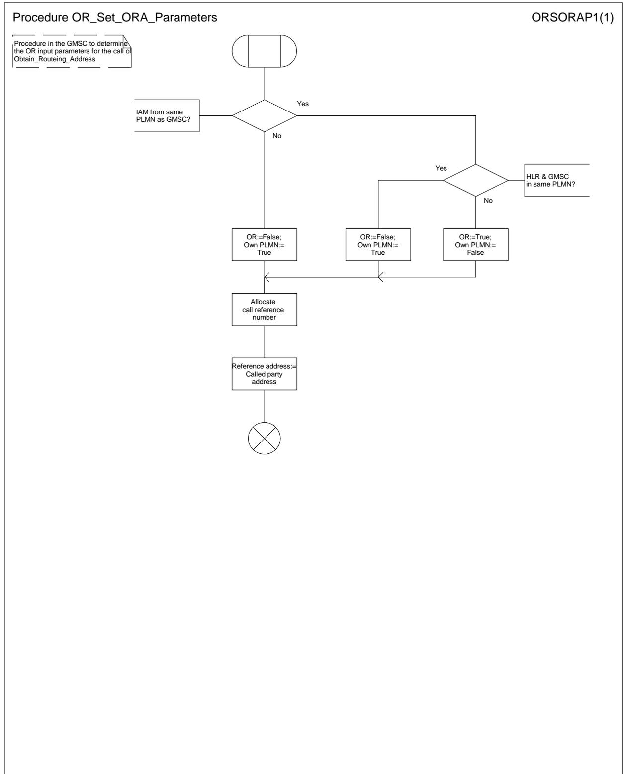
Figure 6: Procedure OR\_Set\_OR\_A\_Parameters
