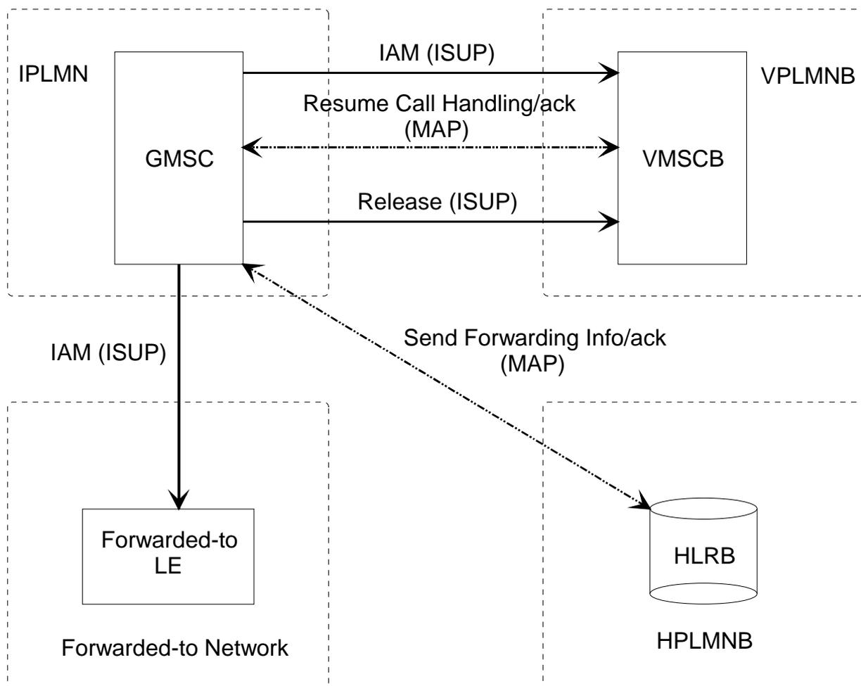
**Figure 2: Architecture for optimal routeing of late call forwarding**
