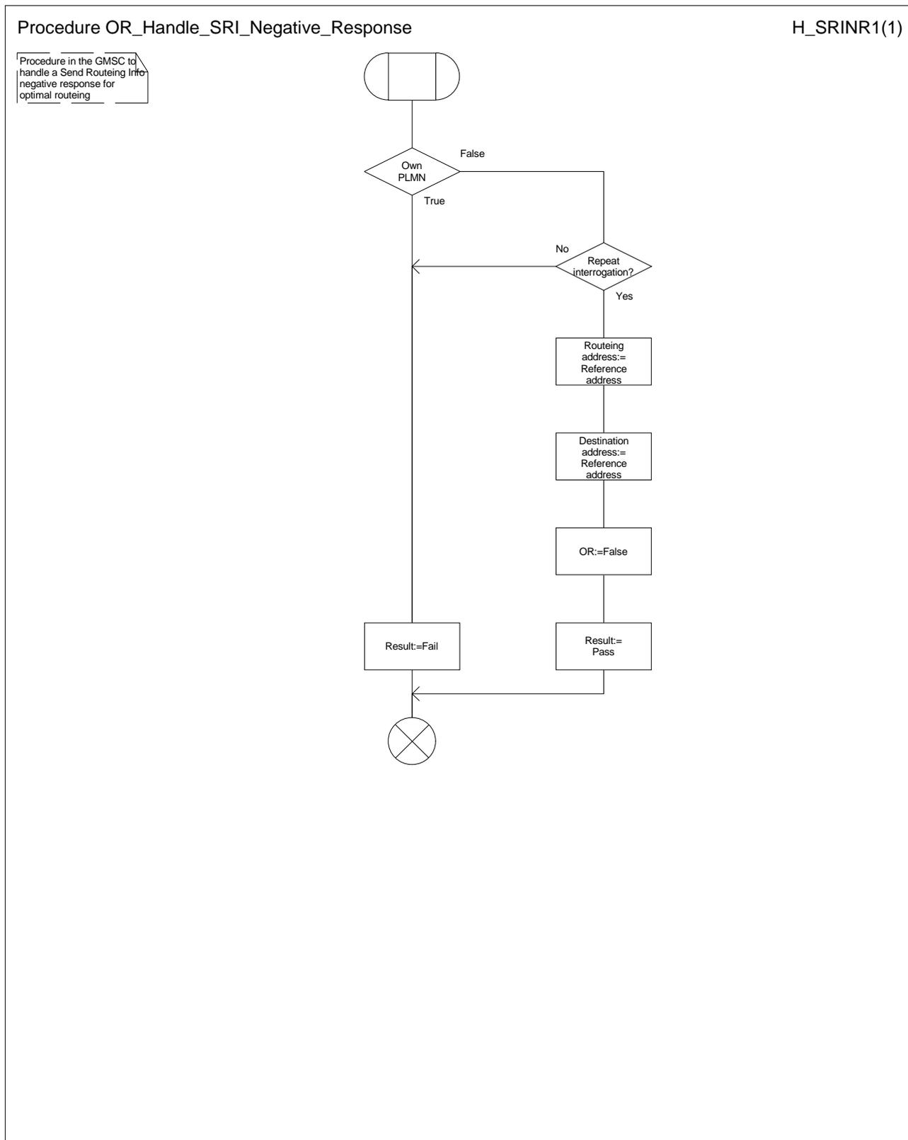
Figure 9: Procedure OR\_Handle\_SRI\_Negative\_Response
