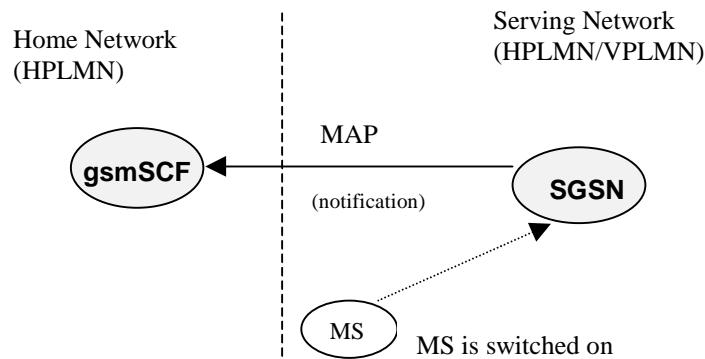
**Figure 9.4-4: Attach of MS**
