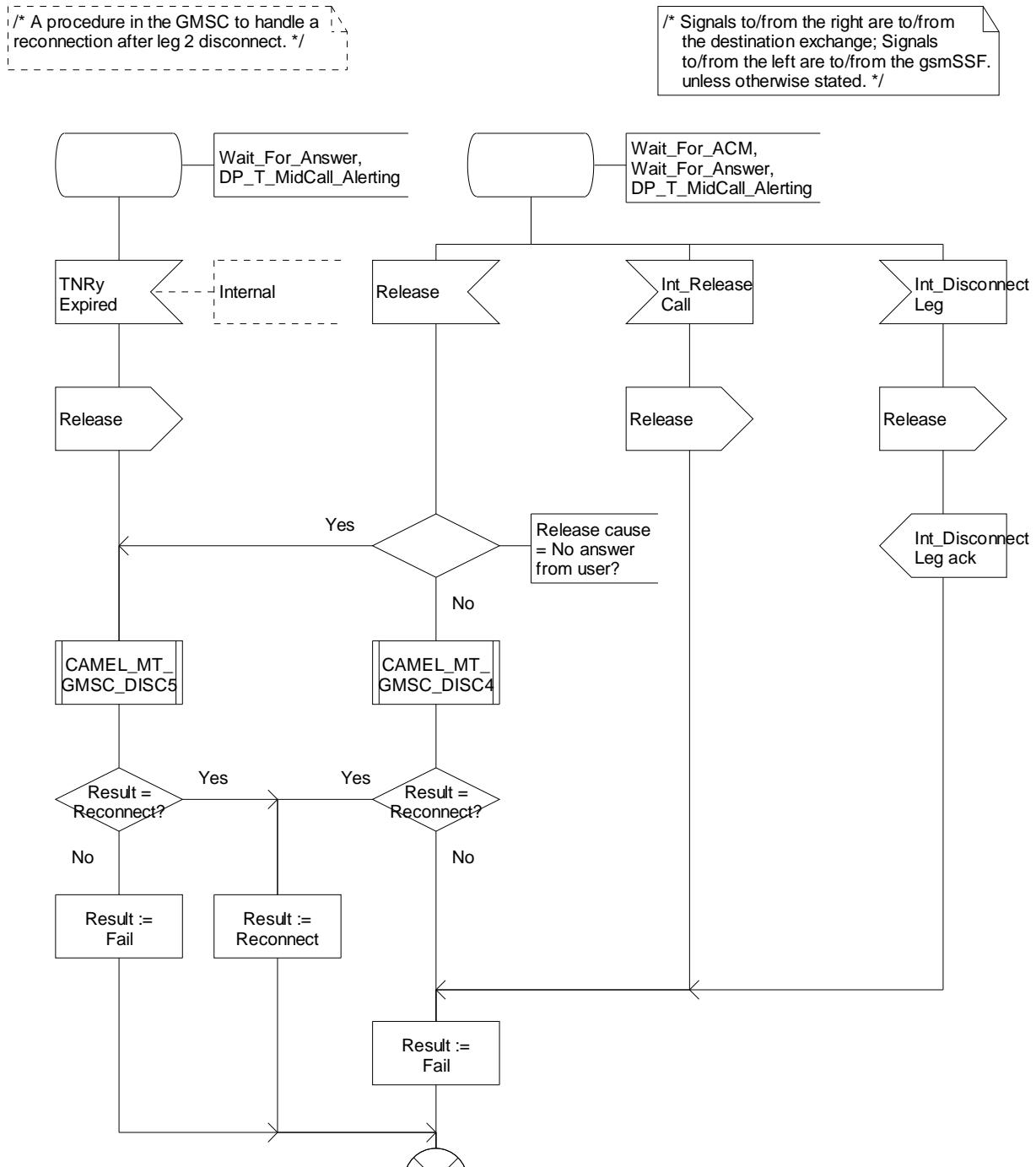
Figure 4.56-4: Procedure CAMEL\_MT\_RECONNECT\_GMSC (sheet 4)
