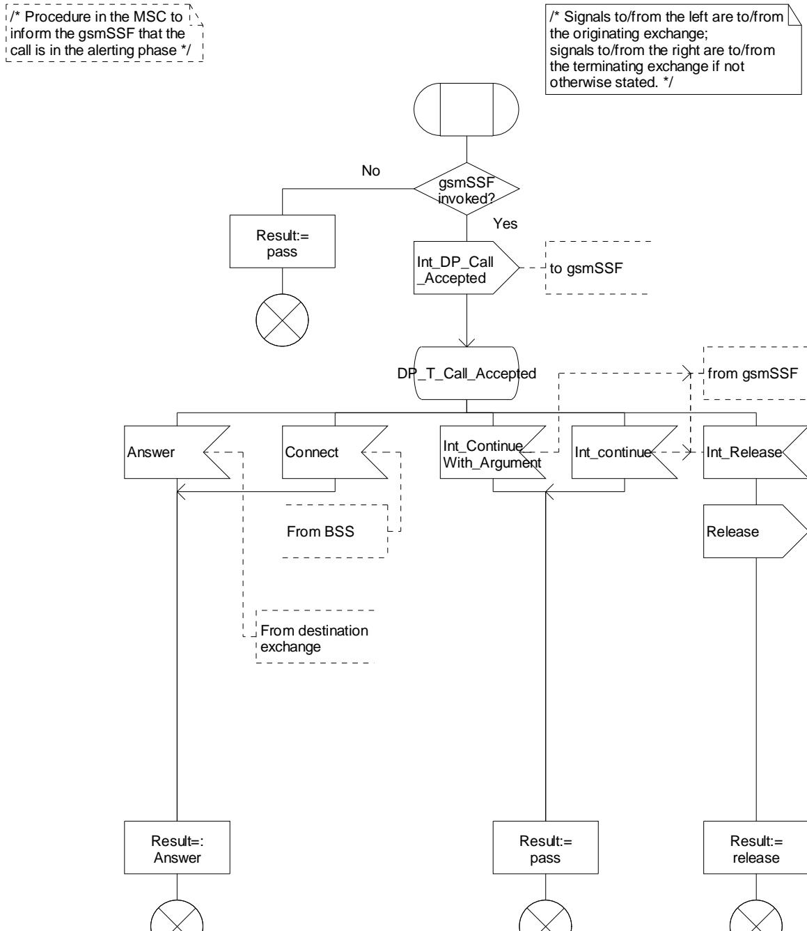
Figure 4.43-1: Procedure CAMEL\_MT\_MSC\_ALERTING (sheet 1)
