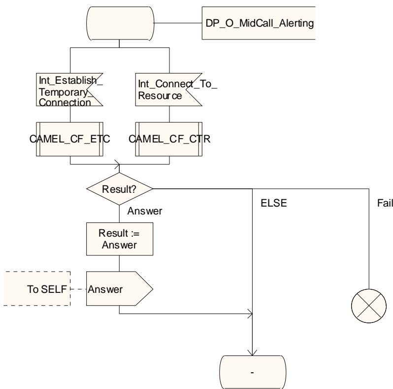
Figure 4.119D-5: Procedure CAMEL\_TOC\_LEG1\_MSC (sheet 5)
