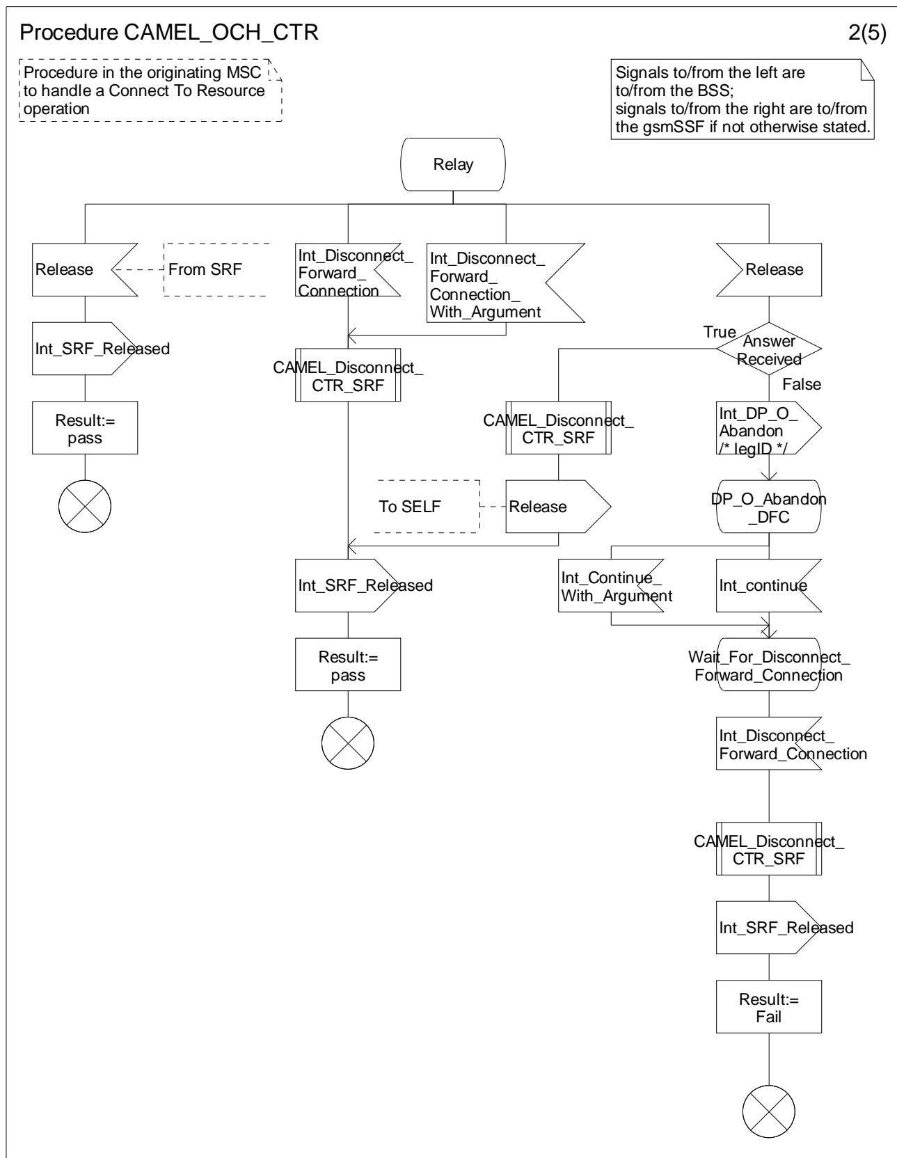
Figure 4.24-2: Procedure CAMEL\_OCH\_CTR (sheet 2)
