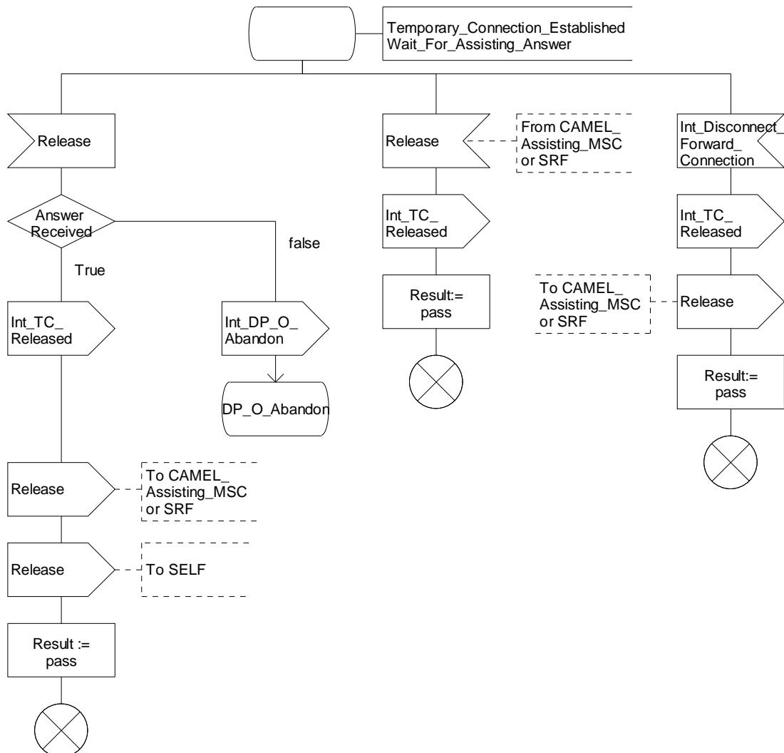
**Figure 4.84-3: Procedure CAMEL\_CF\_ETC (sheet 3)**
