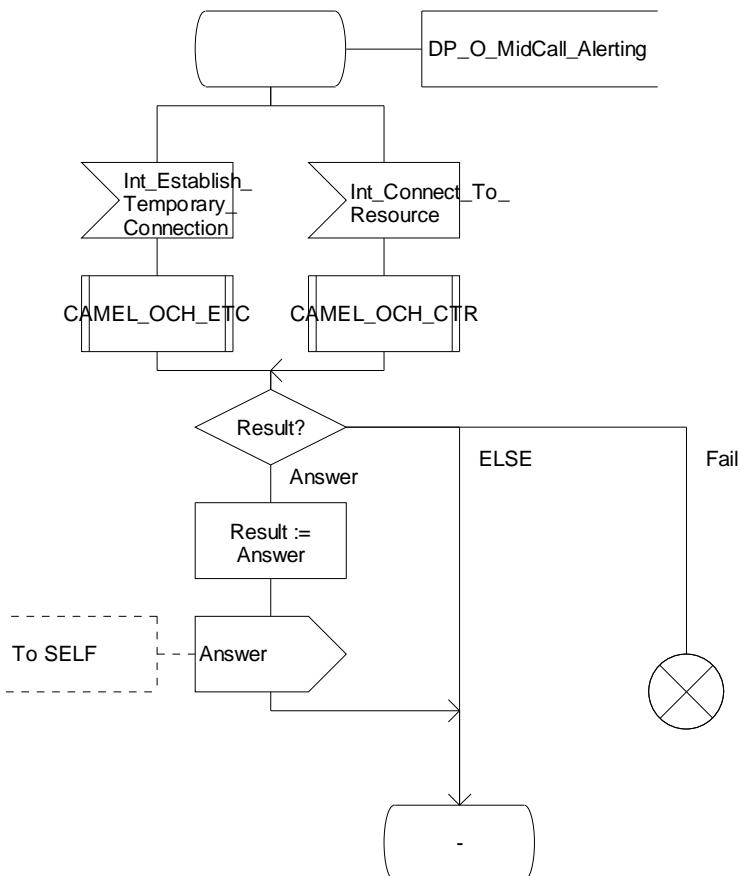
Figure 4.33-8: Procedure CAMEL\_OCH\_RECONNECT\_MSC (sheet 8)
