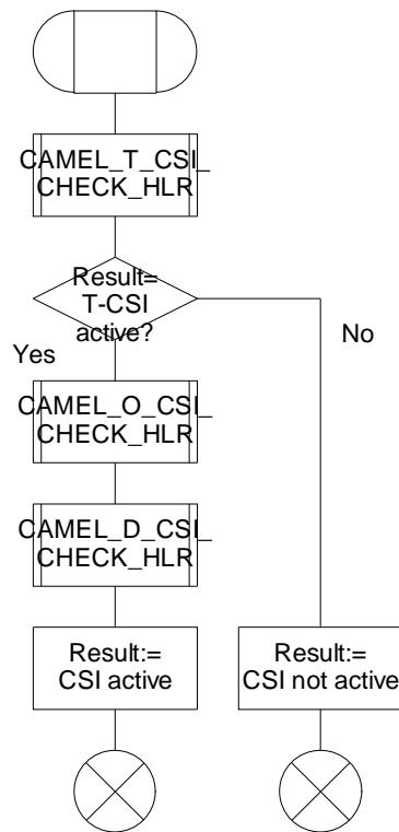
Figure 4.59-1: Procedure CAMEL\_CSI\_Check\_HLR (sheet 1)
