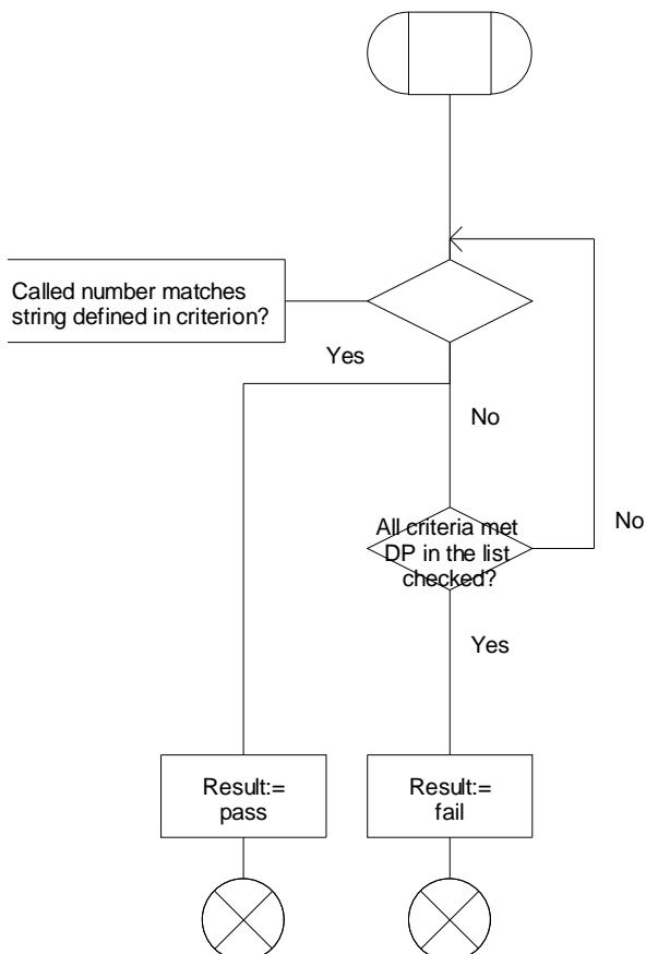
Figure 4.101-1: Procedure Check\_Criteria\_Analysed\_Info (sheet 1)
