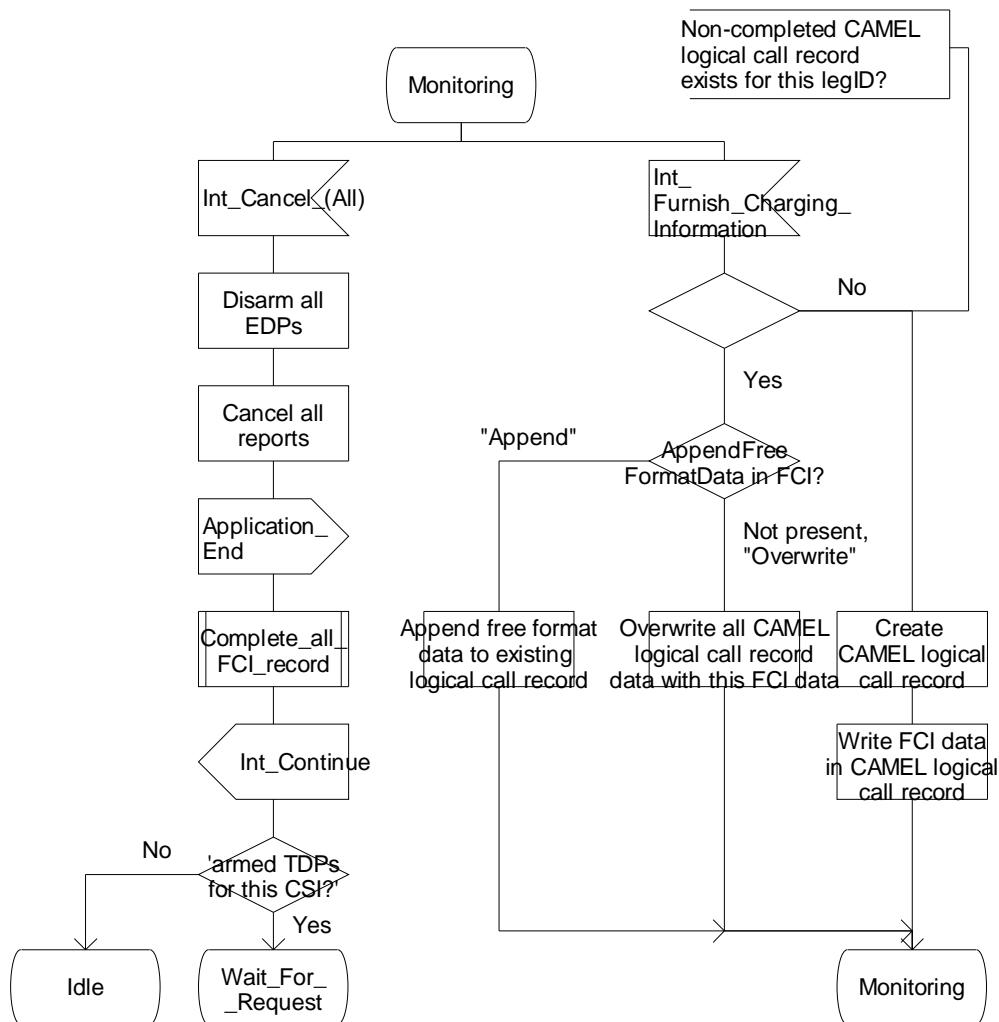
Figure 4.99-33: Process CS\_gsmSSF (sheet 33)
