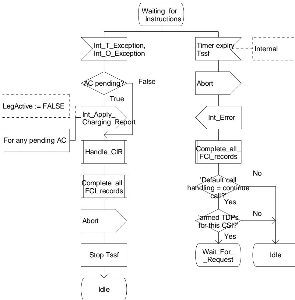
Figure 4.99-23: Process CS\_gsmSSF (sheet 23)
