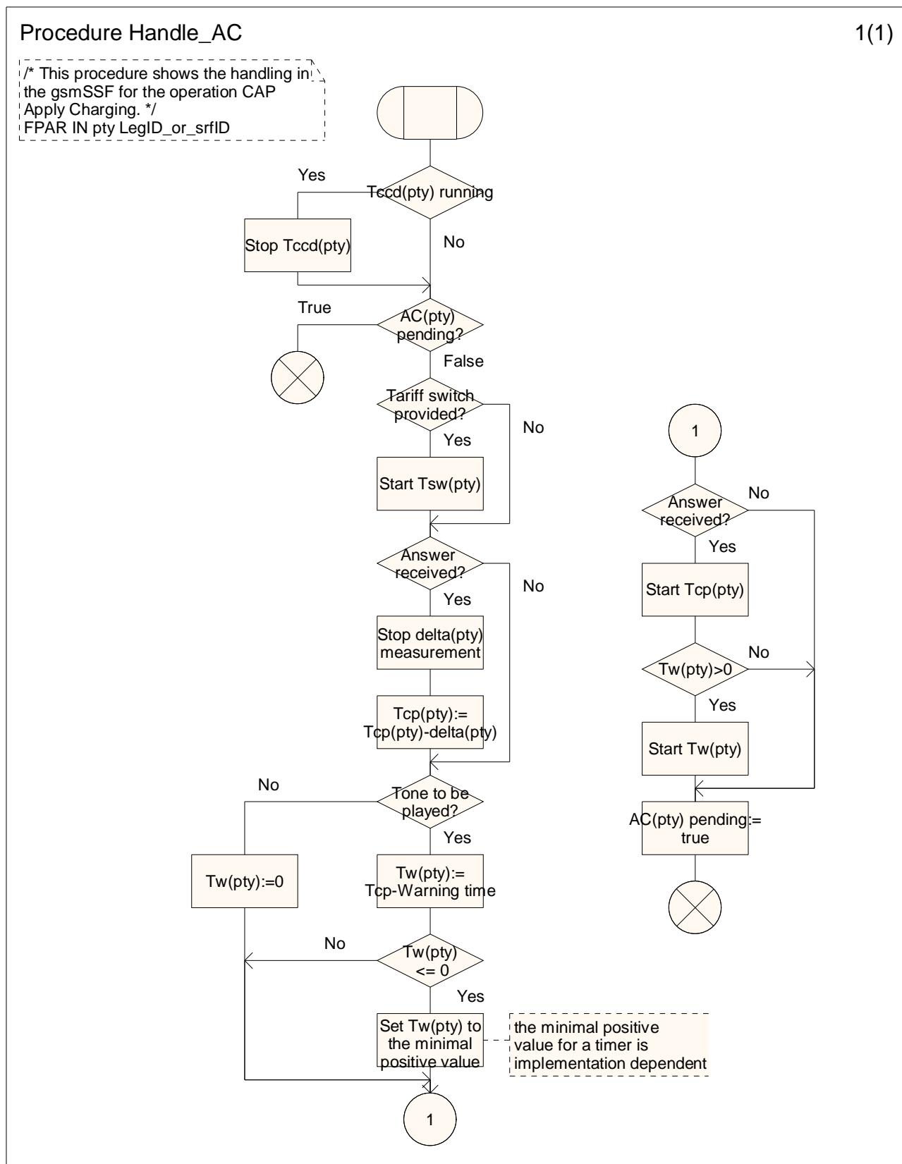
Figure 4.104-1: Procedure Handle\_AC (sheet 1)
