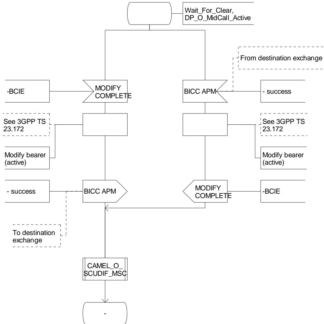
Figure 4.30-8: Procedure CAMEL\_OCH\_LEG1\_MSC (sheet 8)
