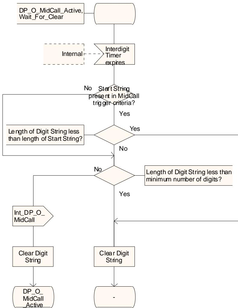
Figure 4.119B-7: Procedure CAMEL\_TOC\_MSC\_INIT (sheet 7)
