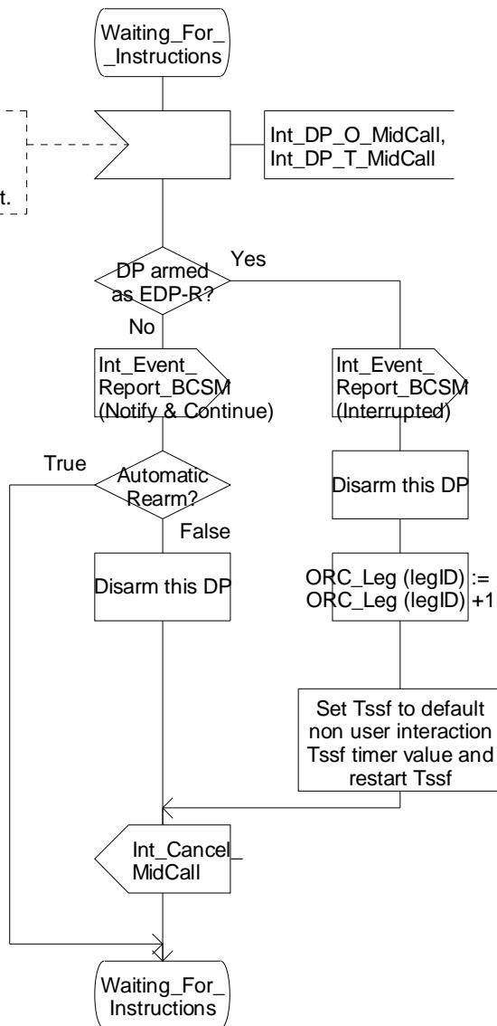
Figure 4.99-14: Process CS\_gsmSSF (sheet 14)
