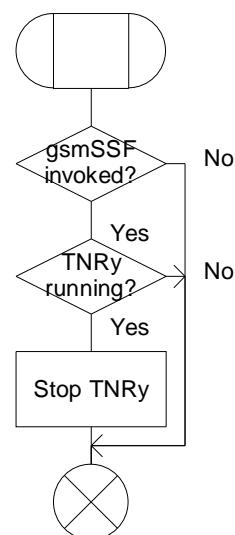
Figure 4.26-1: Procedure CAMEL\_Stop\_TNRy (sheet 1)
