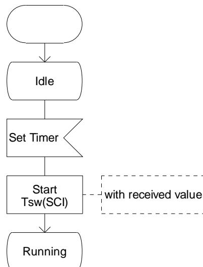
Figure 4.98-1: Process Tsw\_For\_SCI (sheet 1)
