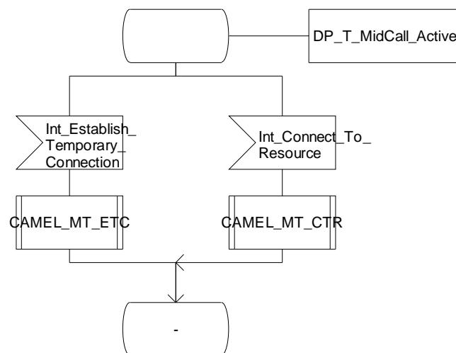
Figure 4.56-7: Procedure CAMEL\_MT\_RECONNECT\_GMSC (sheet 7)
