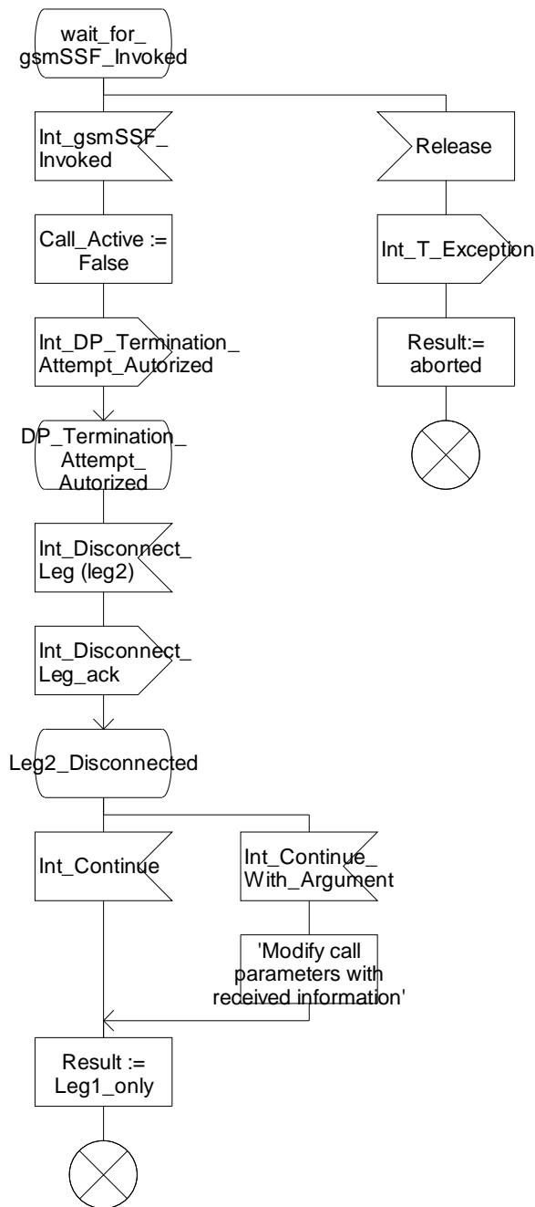
Figure 4.69-2: Procedure CAMEL\_ICH\_MSC\_INIT (sheet 2)
