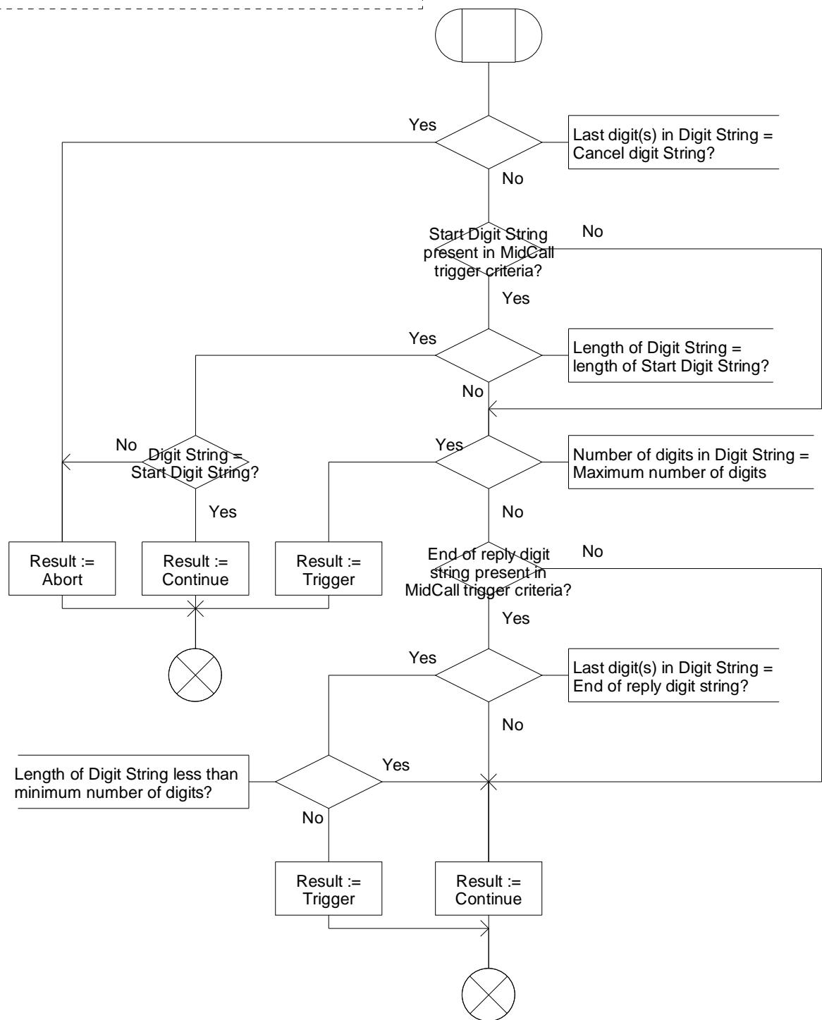
Figure 4.31-1: Procedure CHECK\_DIGIT\_STRING\_MSC (sheet 1)
