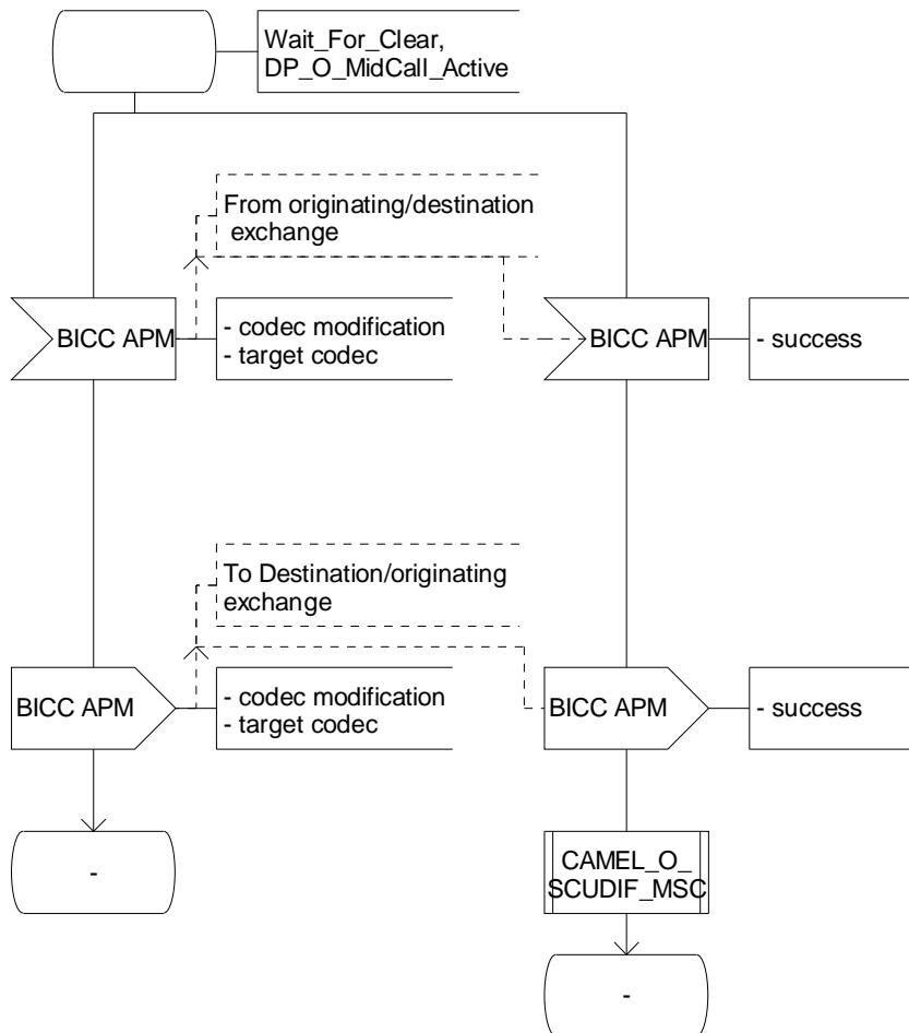
Figure 4.86-7: Procedure CAMEL\_MT\_CF\_LEG1\_MSC (sheet 7)
