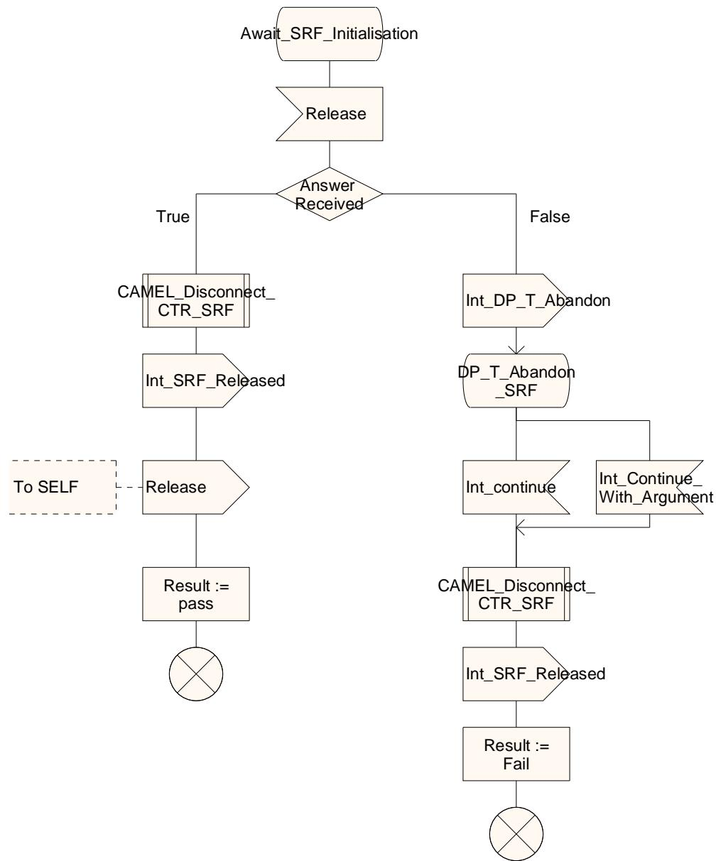
Figure 4.52-4: Procedure CAMEL\_MT\_CTR (sheet 4)
