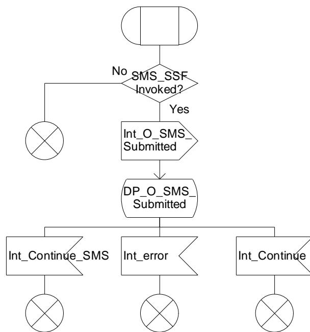
**Figure 7.6-1: Procedure CAMEL\_O\_SMS\_SUBMITTED (sheet 1)**
