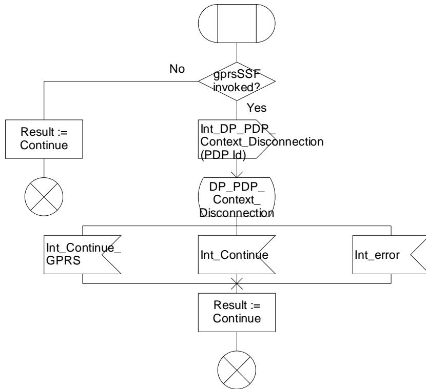
Figure 6.15-1: Procedure CAMEL\_GPRS\_PDP\_Context\_Disconnection (sheet 1)
