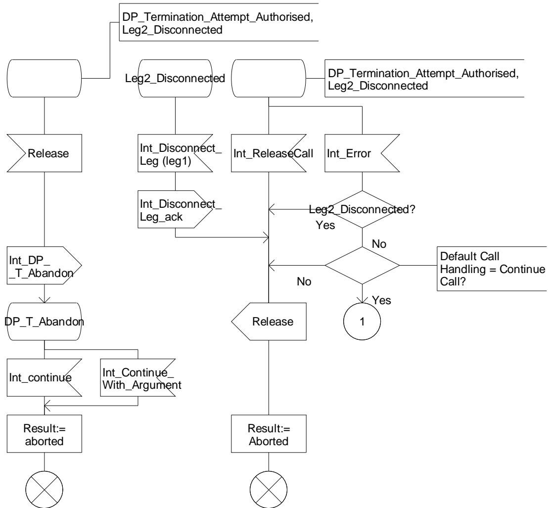
Figure 4.69-4: Procedure CAMEL\_ICH\_MSC\_INIT (sheet 4)
