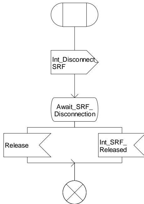
**Figure 4.22-1: Procedure CAMEL\_Disconnect\_CTR\_SRF (sheet 1)**
