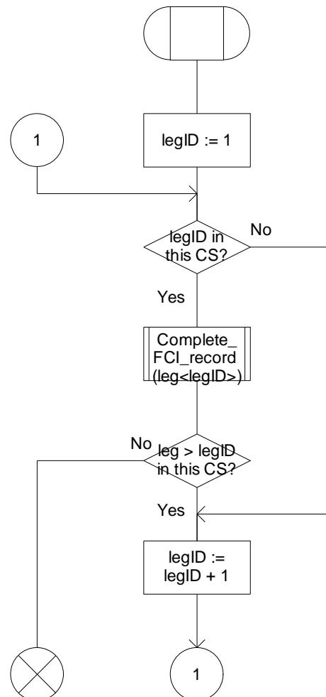
Figure 4.109-1: Procedure Complete\_all\_FCI\_records (sheet 1)
