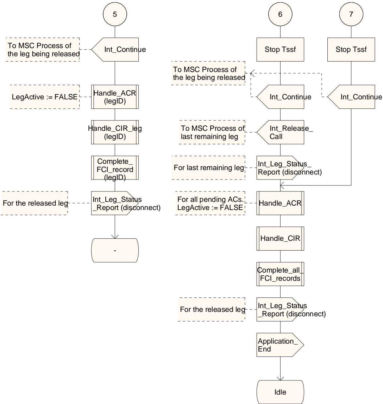
Figure 4.99-48: Process CS\_gsmSSF (sheet 48)
