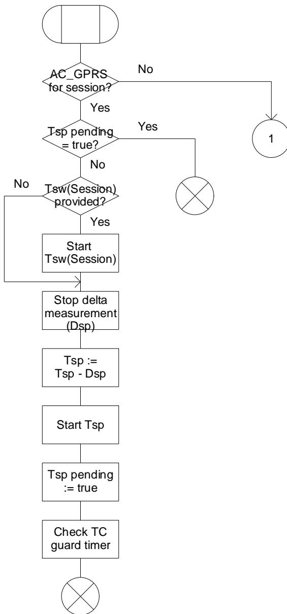
Figure 6.19-1: Procedure Handle\_AC\_GPRS (sheet 1)
