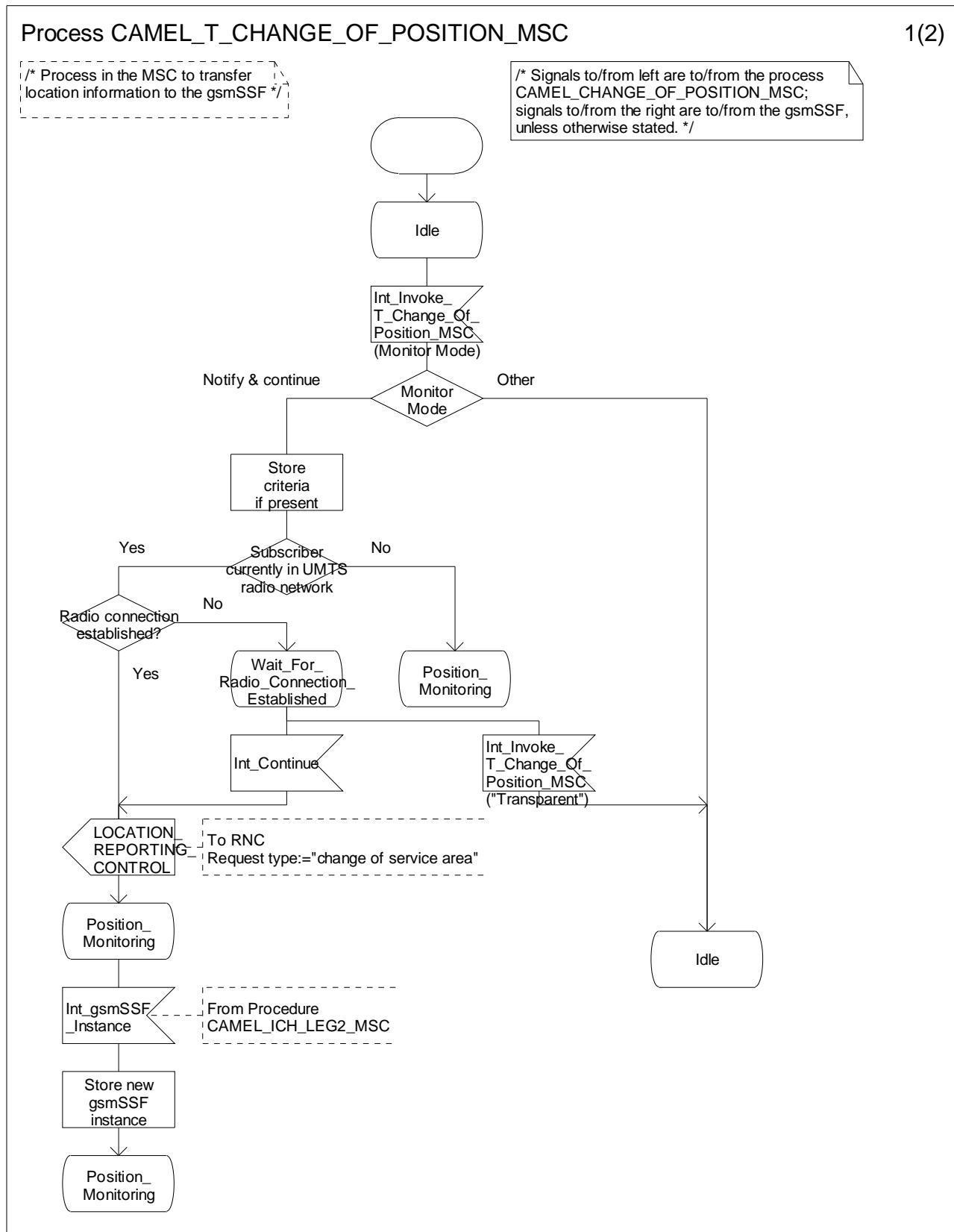
Figure 4.75-1: Process CAMEL\_T\_CHANGE\_OF\_POSITION\_MSC (sheet 1)
