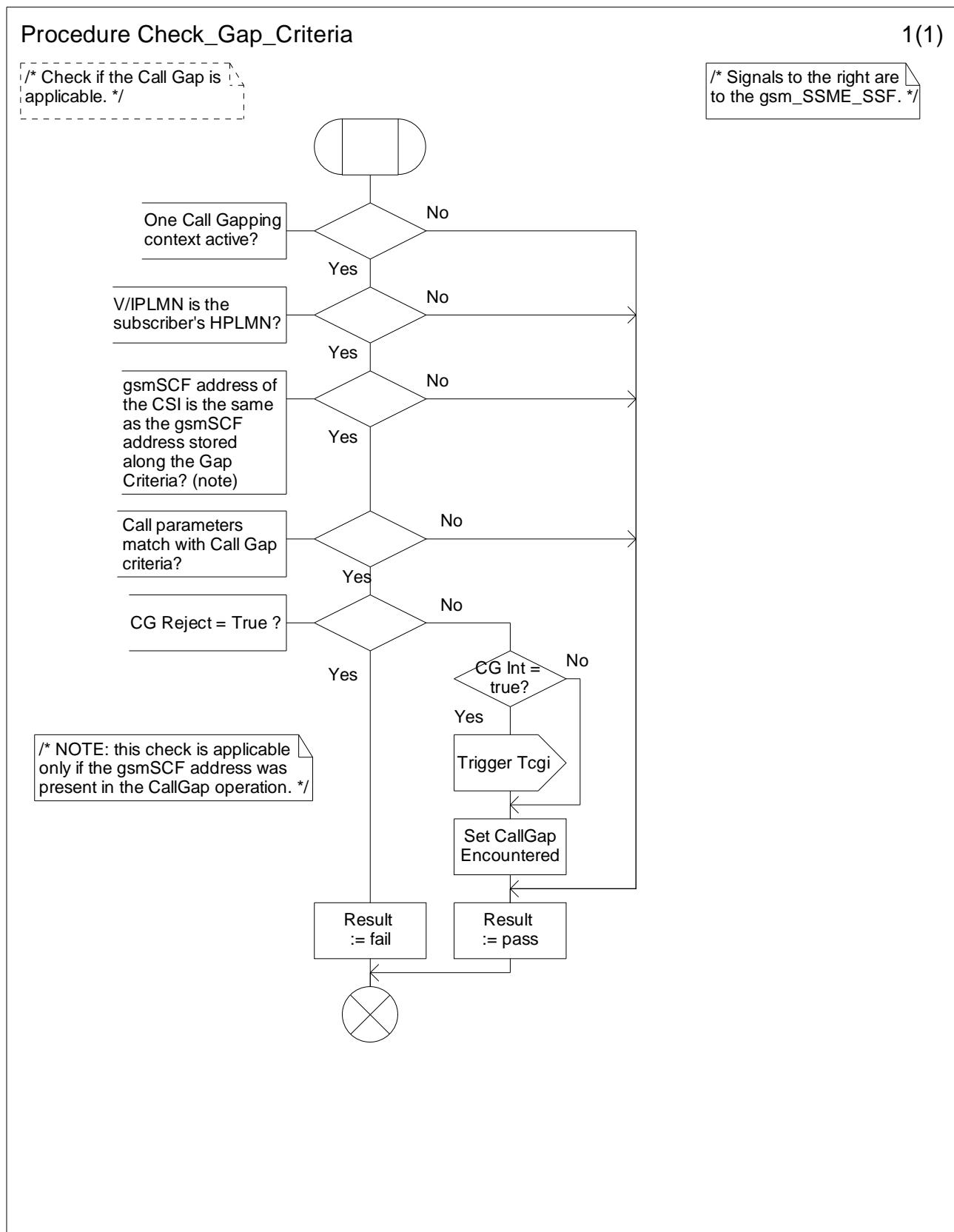
Figure 4.115-1: Procedure Check\_Gap\_Criteria (sheet 1)
