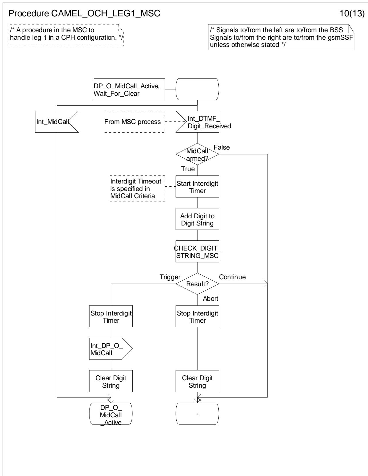
**Figure 4.30-10: Procedure CAMEL\_OCH\_LEG1\_MSC (sheet 10)**
