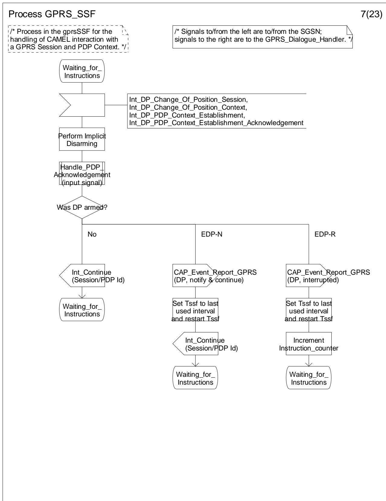
Figure 6.17-7: Process GPRS\_SSF (sheet 7)
