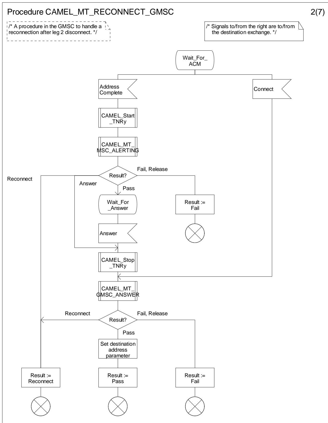
Figure 4.56-2: Procedure CAMEL\_MT\_RECONNECT\_GMSC (sheet 2)
