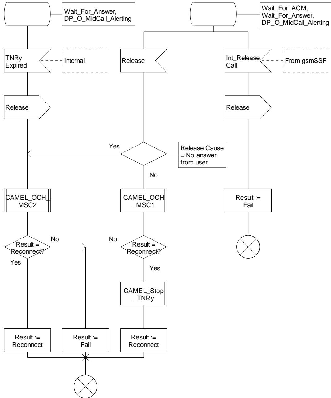
Figure 4.88-3: Procedure CAMEL\_MF\_RECONNECT\_MSC (sheet 3)
