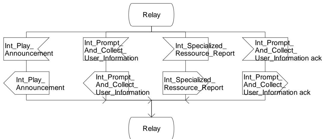
Figure 4.24-3: Procedure CAMEL\_OCH\_CTR (sheet 3)
