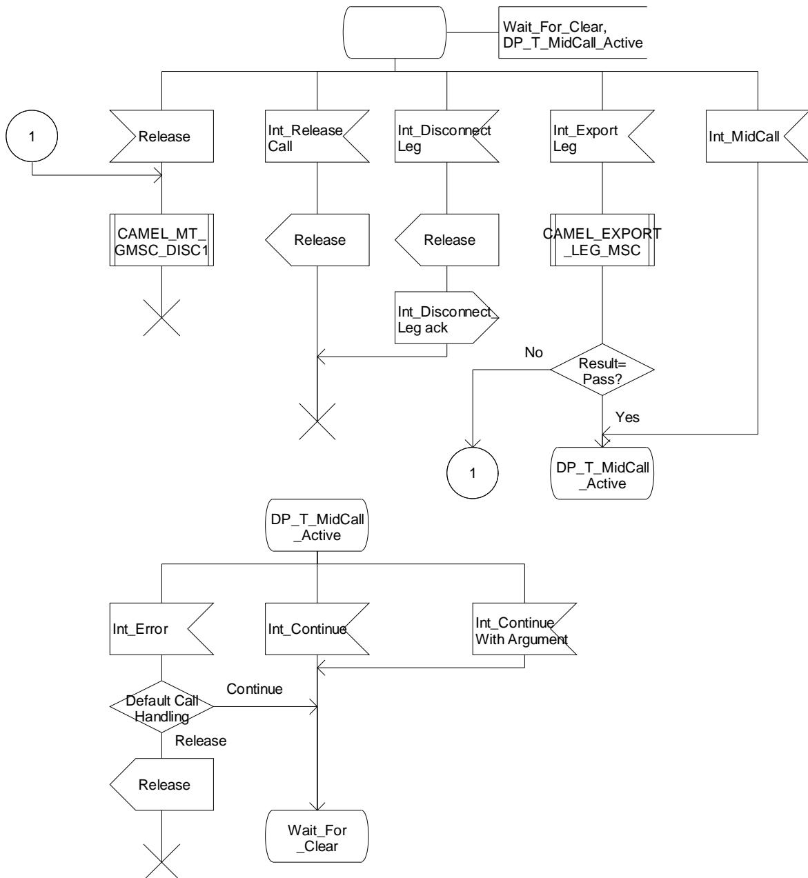
Figure 4.55-3: Process CAMEL\_MT\_LEG1\_GMSC (sheet 3)
