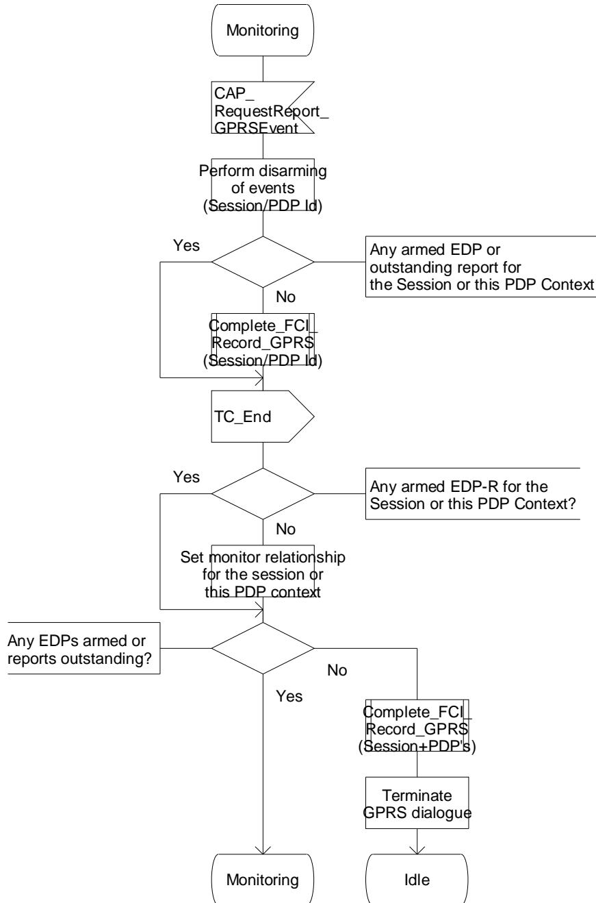
Figure 6.17-15: Process GPRS\_SSF (sheet 15)
