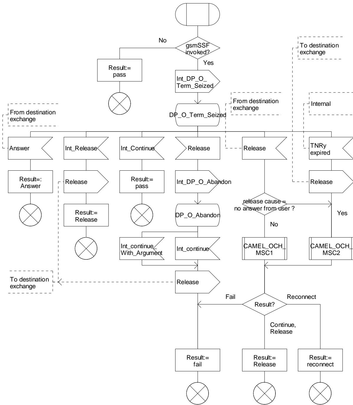
**Figure 4.14-1: Procedure CAMEL\_OCH\_MSC\_ALERTING (sheet 1)**
