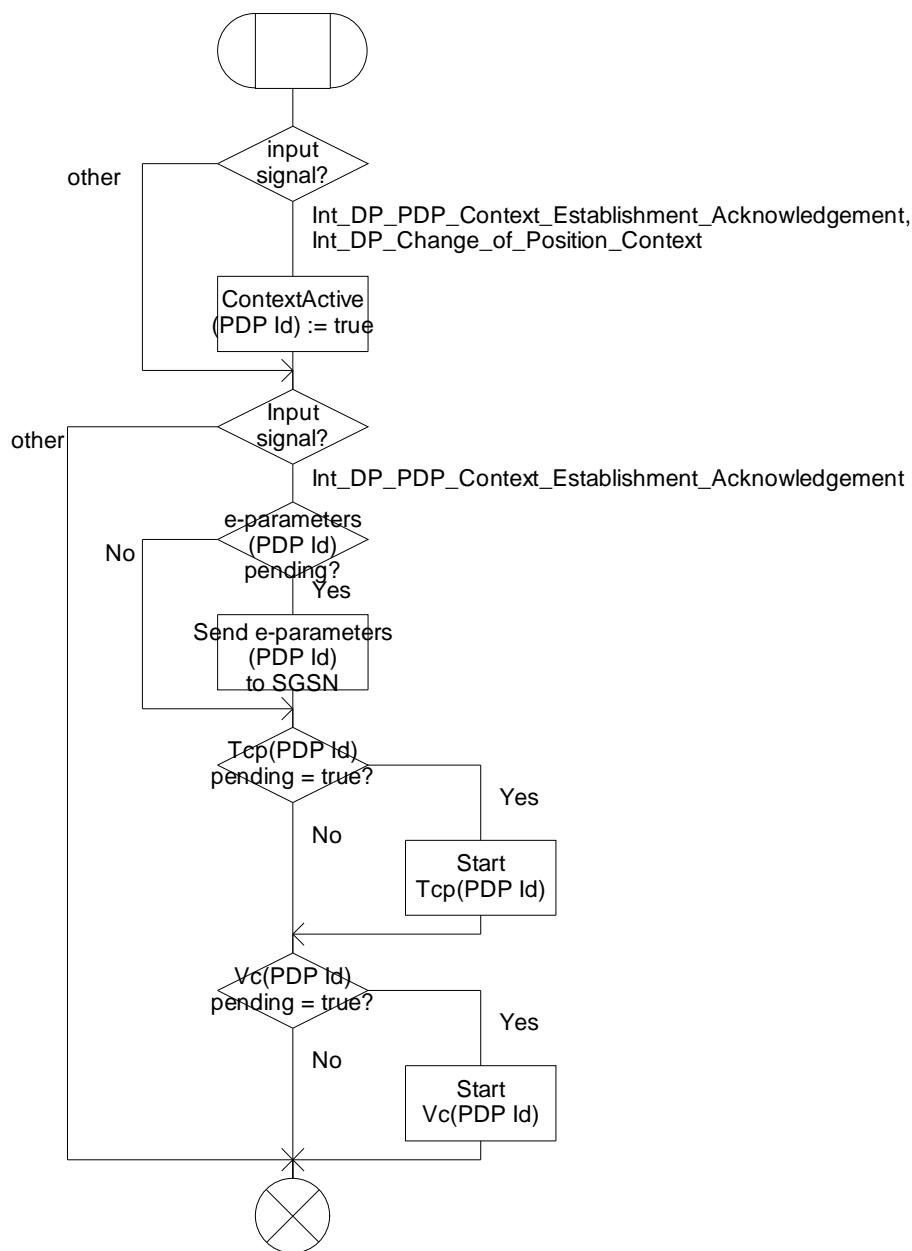
**Figure 6.24-1: Procedure Handle\_PDP\_Acknowledgement (sheet 1)**
