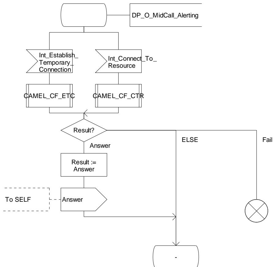
Figure 4.88-5: Procedure CAMEL\_MF\_RECONNECT\_MSC (sheet 5)
