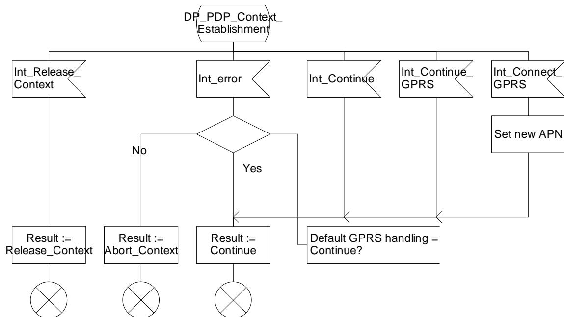
Figure 6.12-2: Procedure CAMEL\_GPRS\_PDP\_Context\_Establishment (sheet 2)
