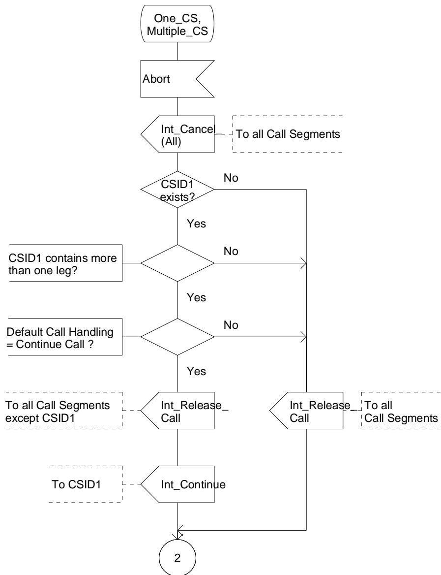
Figure 4.116-15: Process CSA\_gsmSSF (sheet 15)
