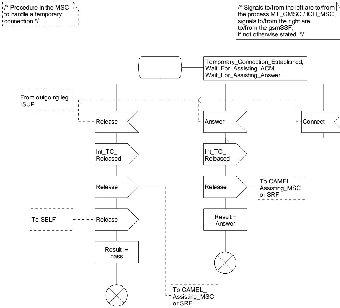
Figure 4.84-4: Procedure CAMEL\_CF\_ETC (sheet 4)
