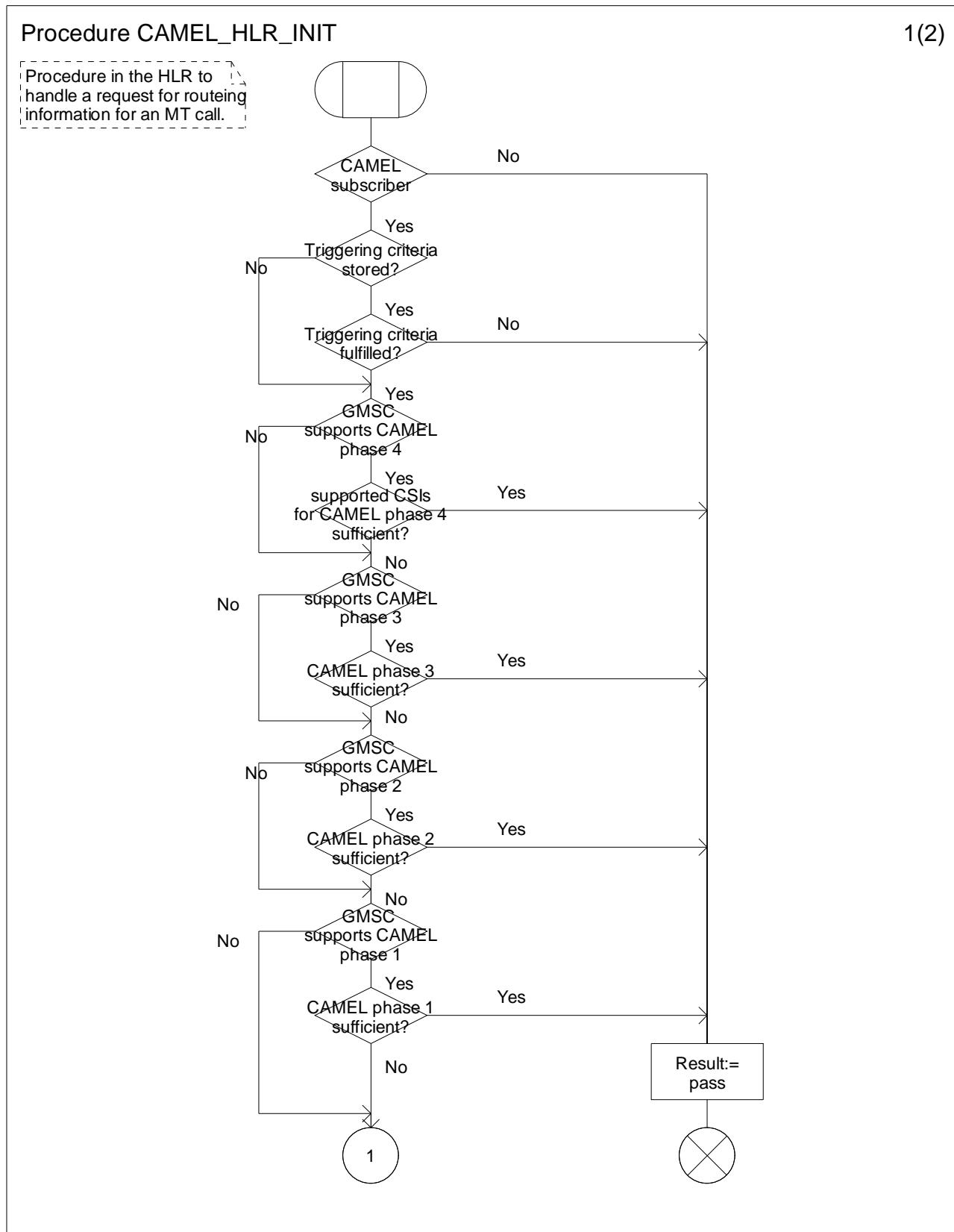
Figure 4.58-1: Procedure CAMEL\_HLR\_INIT (sheet 1)
