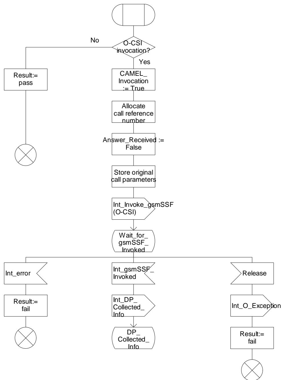
Figure 4.10-1: Procedure CAMEL\_OCH\_MSC\_INIT (sheet 1)
