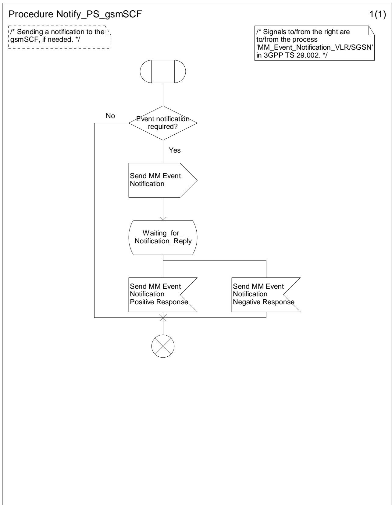
**Figure 9.7-1: Procedure Notify\_PS\_gsmSCF (sheet 1)**
