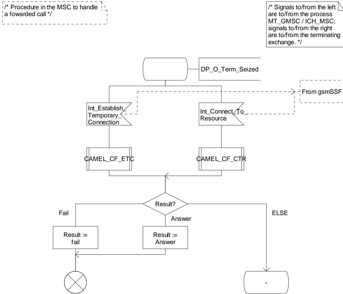
Figure 4.82-3: Procedure CAMEL\_CF\_MSC\_ALERTING (sheet 3)
