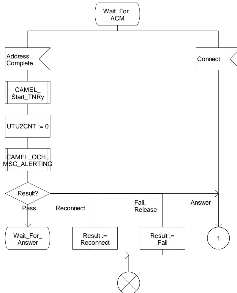
Figure 4.33-2: Procedure CAMEL\_OCH\_RECONNECT\_MSC (sheet 2)
