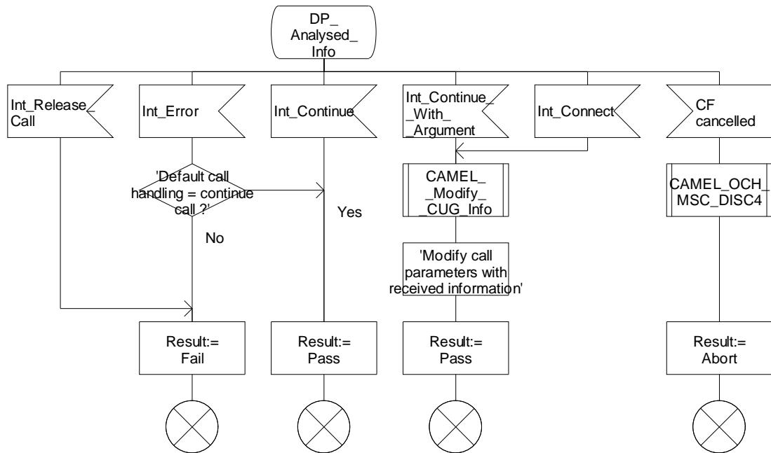
Figure 4.80-2: Procedure CAMEL\_SDS\_CF\_INIT (sheet 2)
