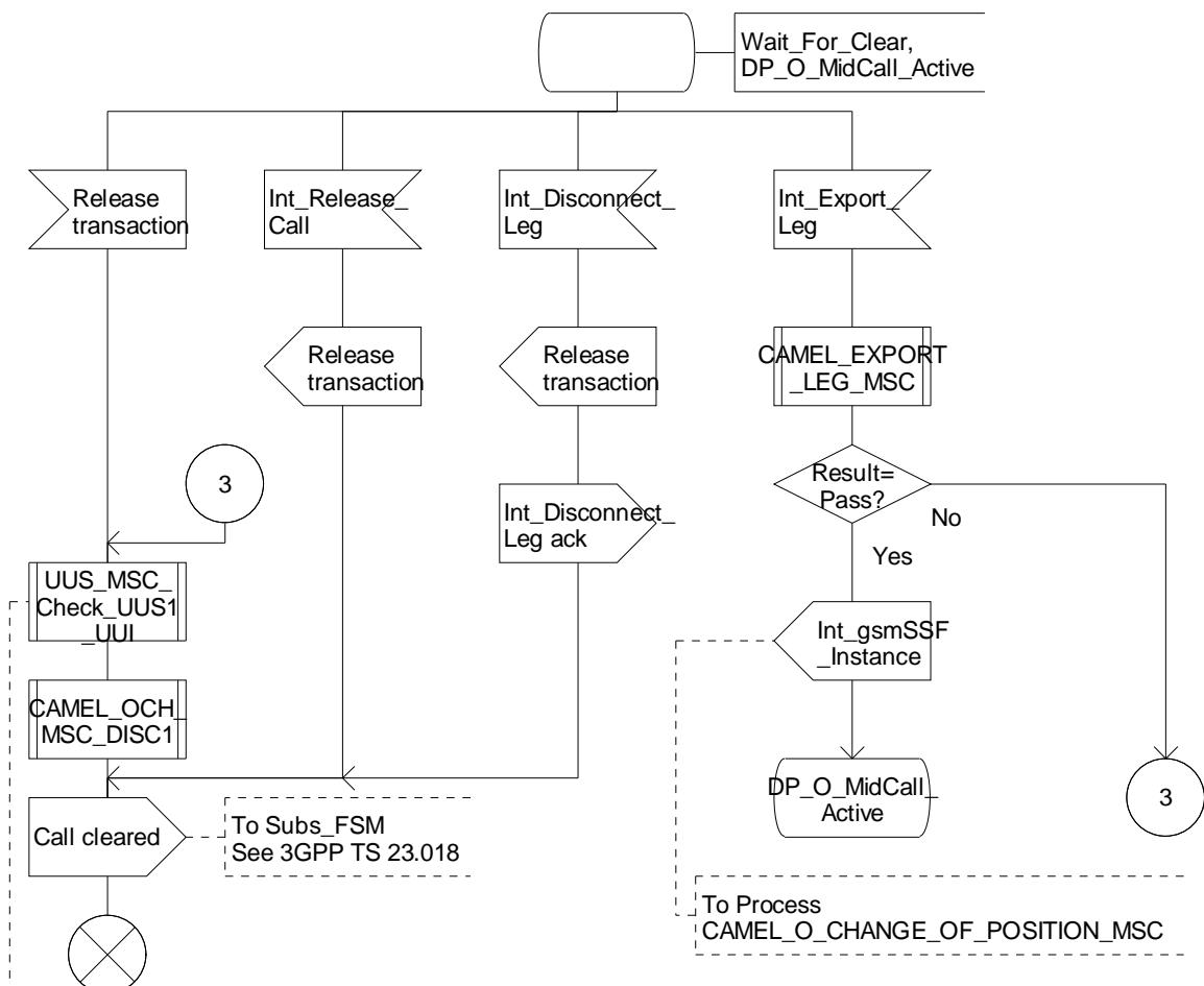
Figure 4.30-5: Procedure CAMEL\_OCH\_LEG1\_MSC (sheet 5)
