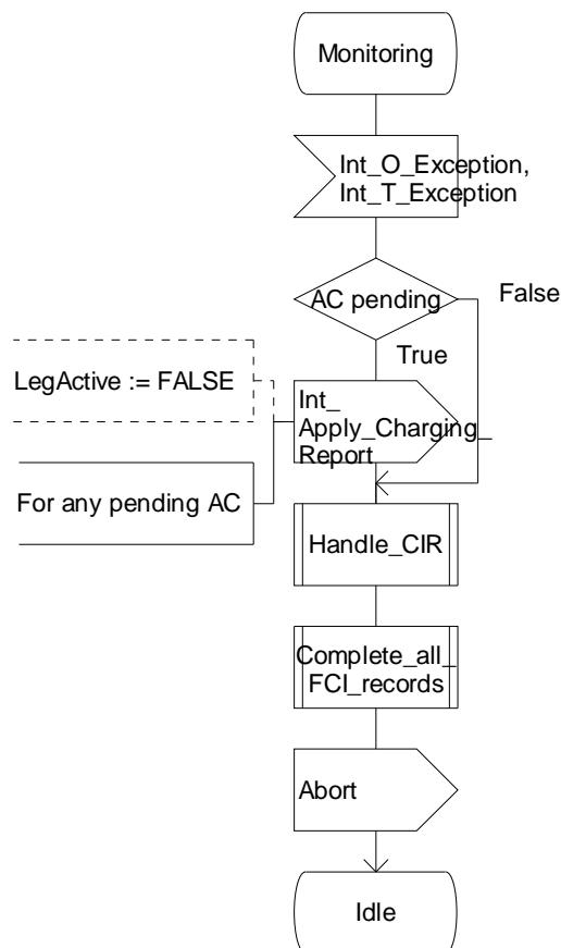
Figure 4.99-31: Process CS\_gsmSSF (sheet 31)
