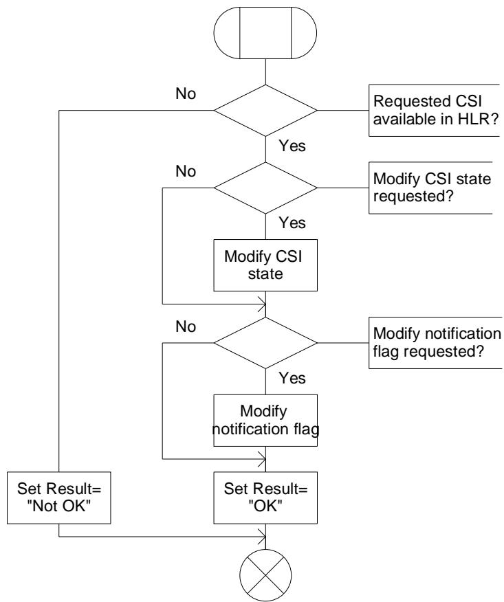
**Figure 10.5-1: Procedure ATM\_Modify\_CSI\_Data (sheet 1)**
