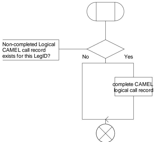
Figure 4.108-1: Procedure Complete\_FCI\_record (sheet 1)
