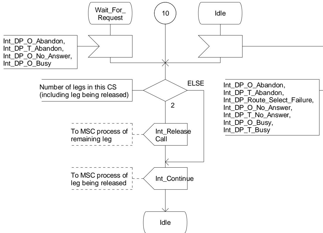
Figure 4.99-8: Process CS\_gsmSSF (sheet 8)
