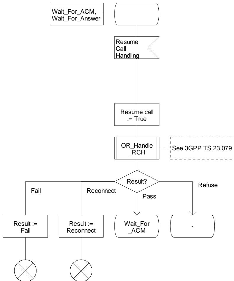
Figure 4.56-3: Procedure CAMEL\_MT\_RECONNECT\_GMSC (sheet 3)
