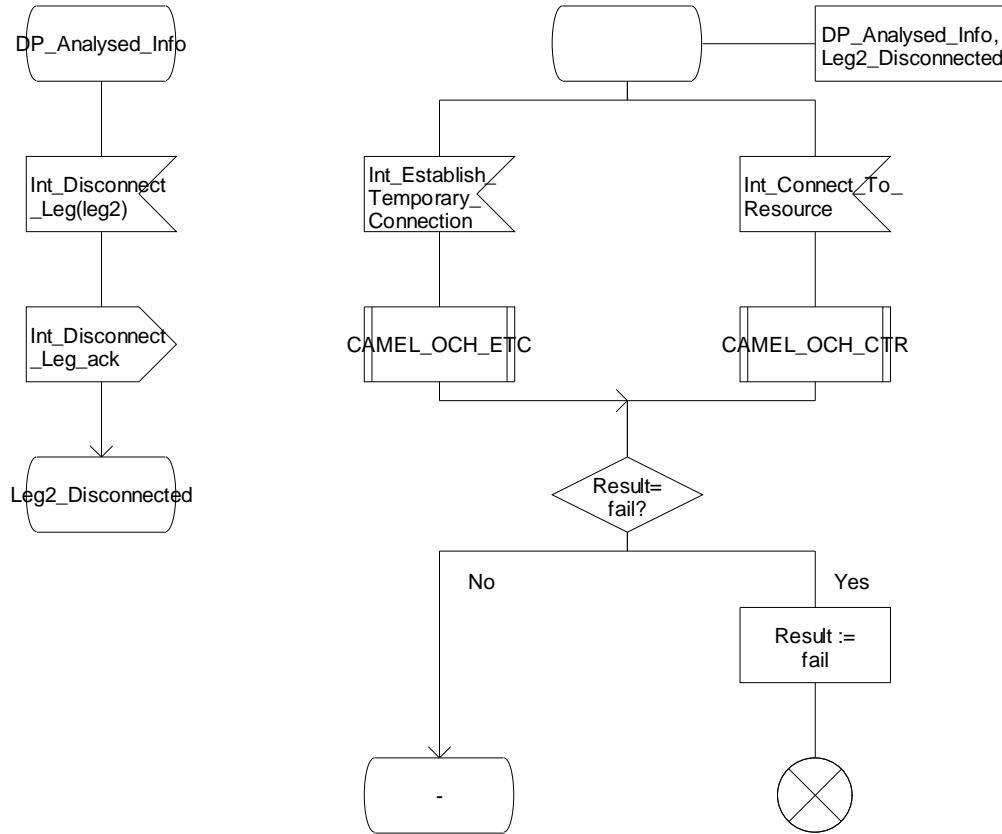
Figure 4.13-3: Procedure CAMEL\_NDS\_MO\_INIT (sheet 3)
