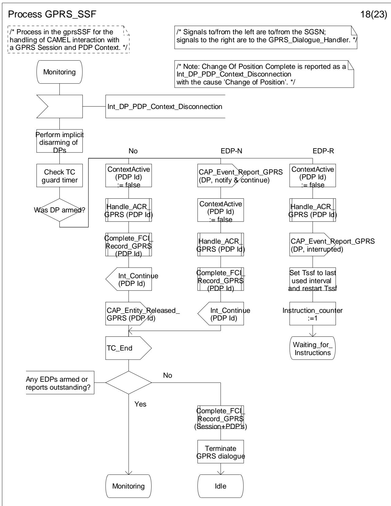
Figure 6.17-18: Process GPRS\_SSF (sheet 18)
