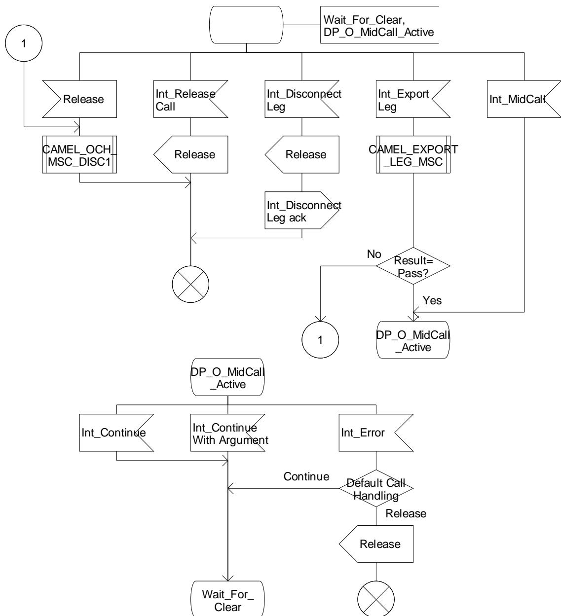
Figure 4.86-4: Procedure CAMEL\_MT\_CF\_LEG1\_MSC (sheet 4)
