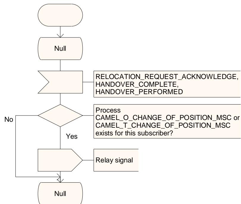
Figure 4.35-1: Process CAMEL\_CHANGE\_OF\_POSITION\_MSC (sheet 1)
