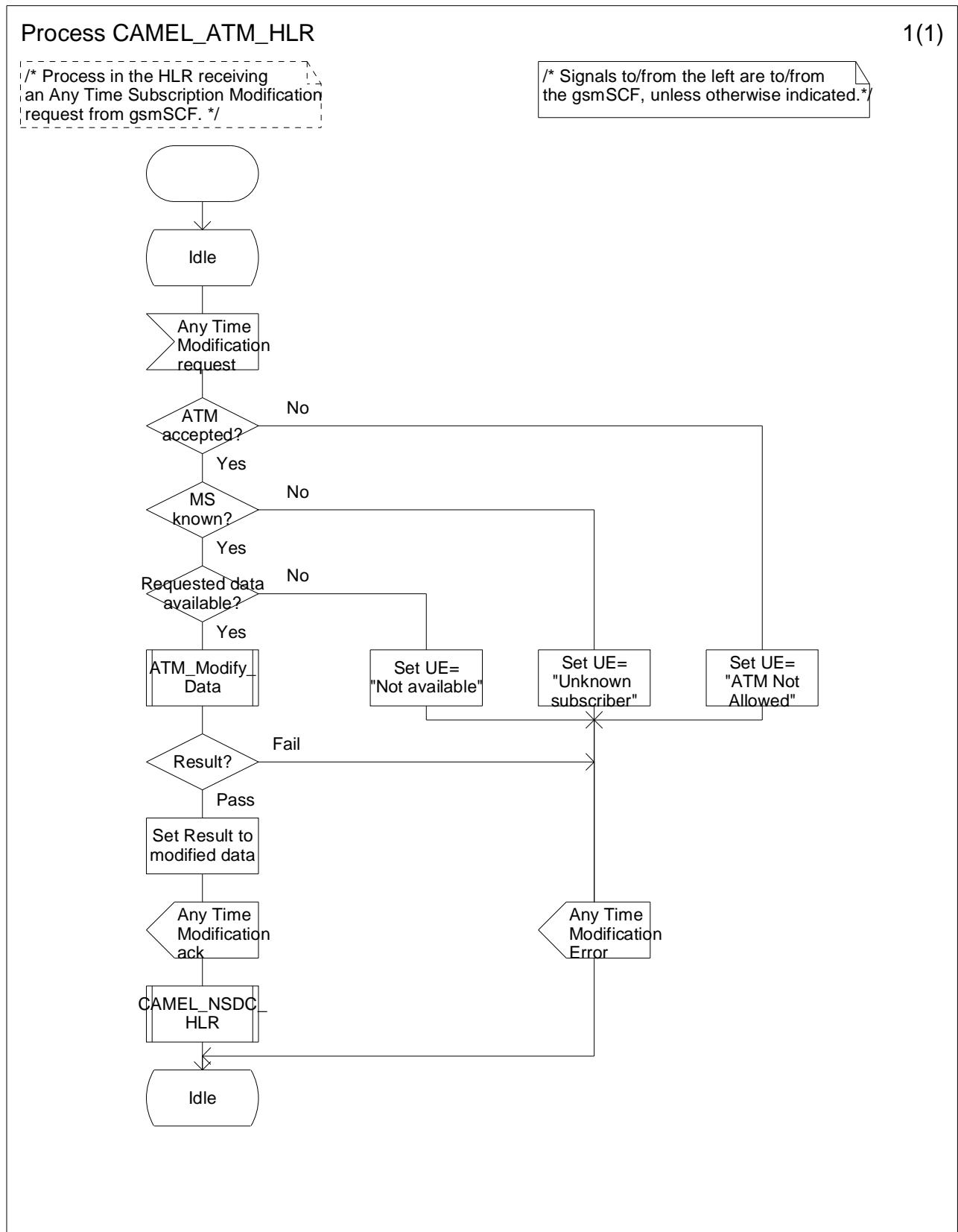
Figure 10.3-1: Process CAMEL\_ATM\_HLR (sheet 1)
