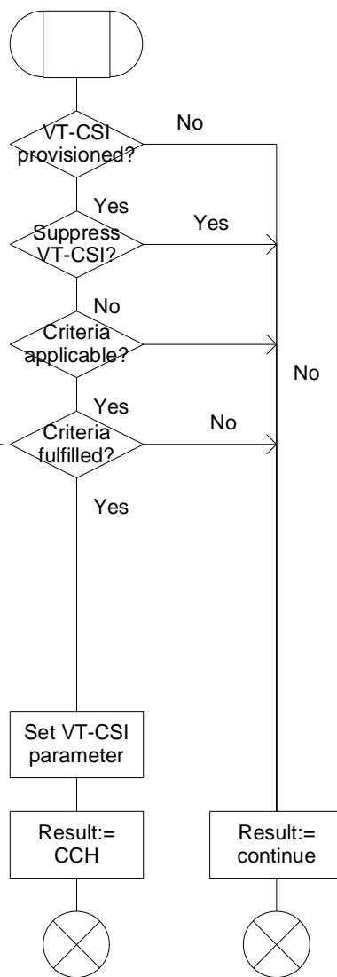
Figure 4.68-1: Procedure CAMEL\_VT\_CSI\_Check\_VLR (sheet 1)
