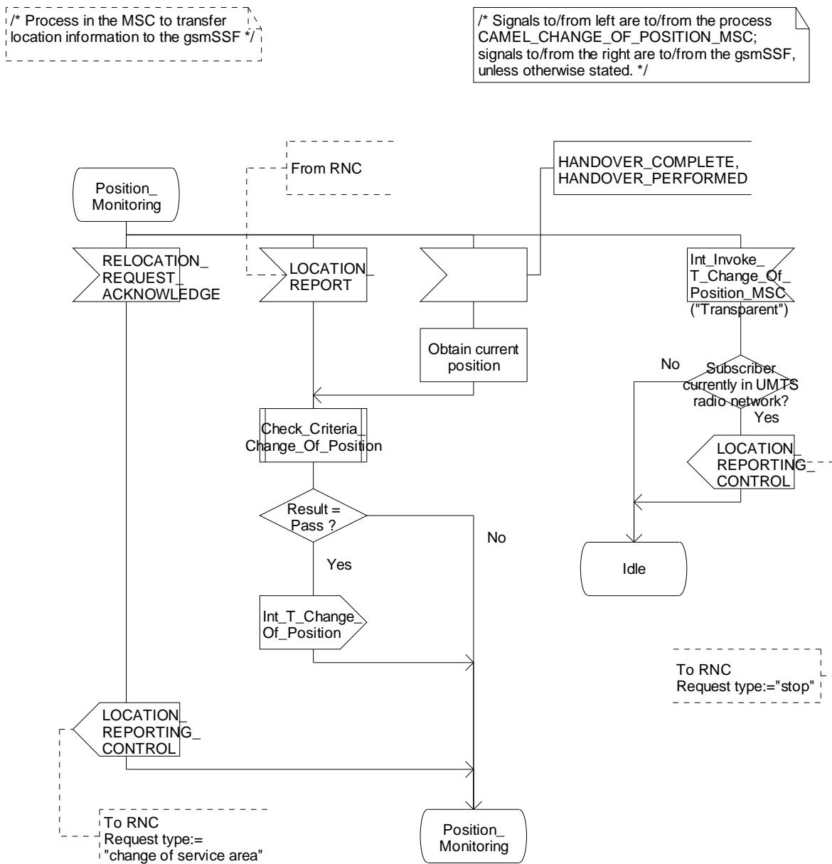
Figure 4.75-2: Procedure CAMEL\_T\_CHANGE\_OF\_POSITION\_MSC (sheet 2)
