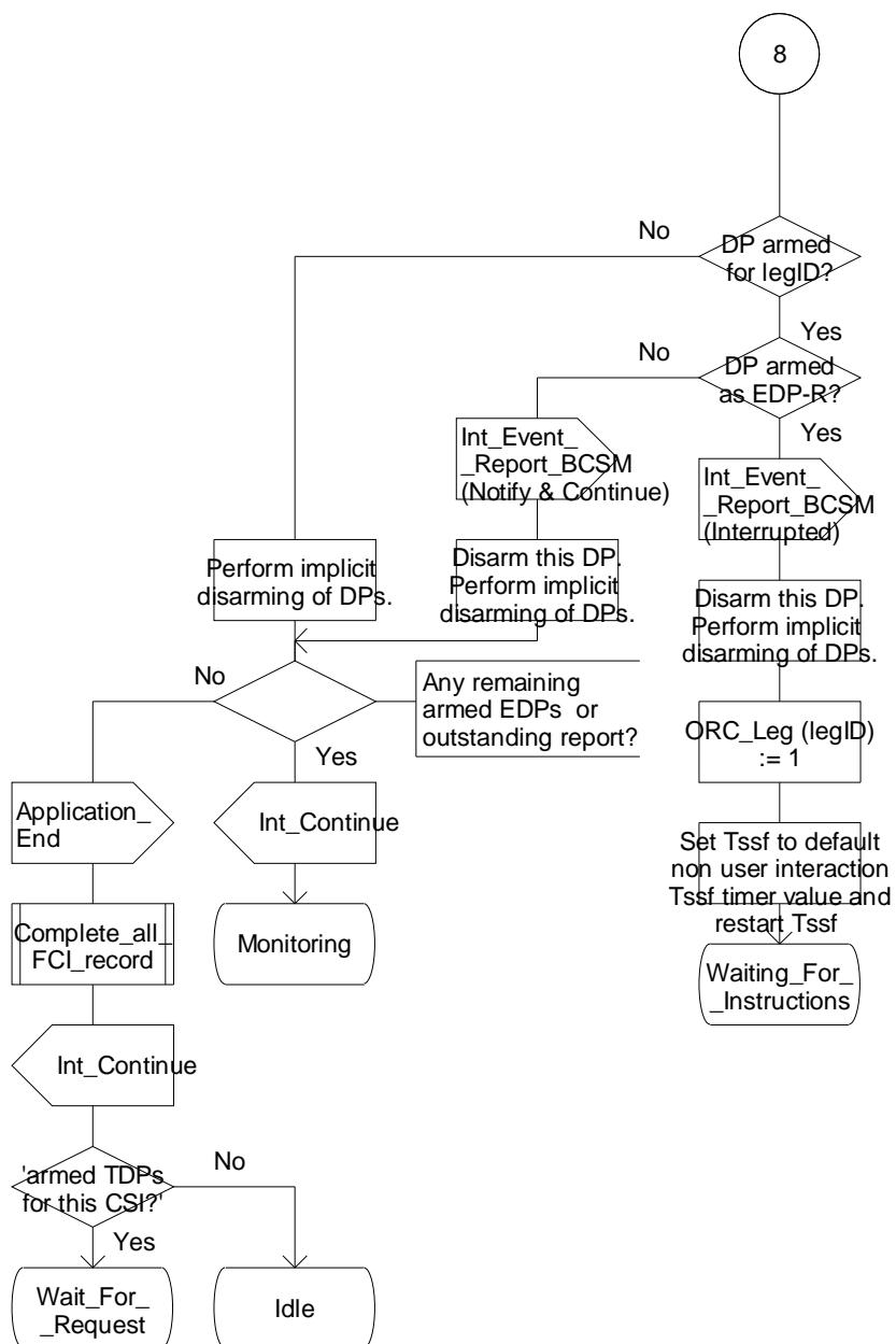
Figure 4.99-26: Process CS\_gsmSSF (sheet 26)
