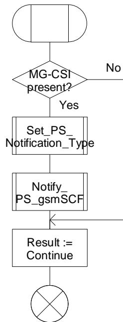
Figure 9.5-1: Procedure CAMEL\_PS\_Notification (sheet 1)
