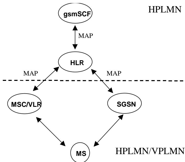
**Figure 11.1-2: Functional architecture for Any Time Interrogation**
