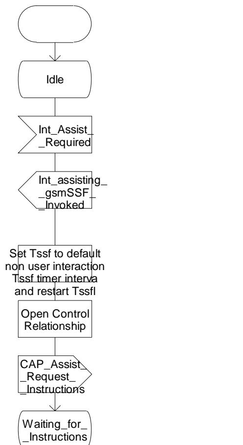
Figure 4.118-1: Process Assisting\_gsmSSF (sheet 1)
