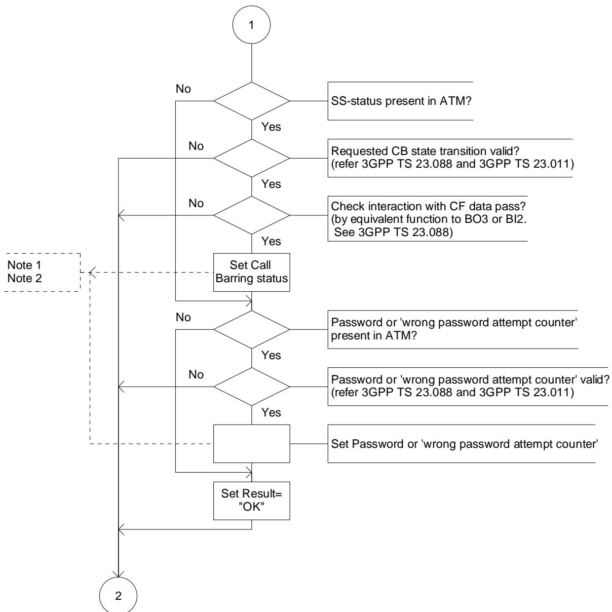
Figure 10.7-2: Procedure ATM\_Modify\_CB\_Data (sheet 2)
