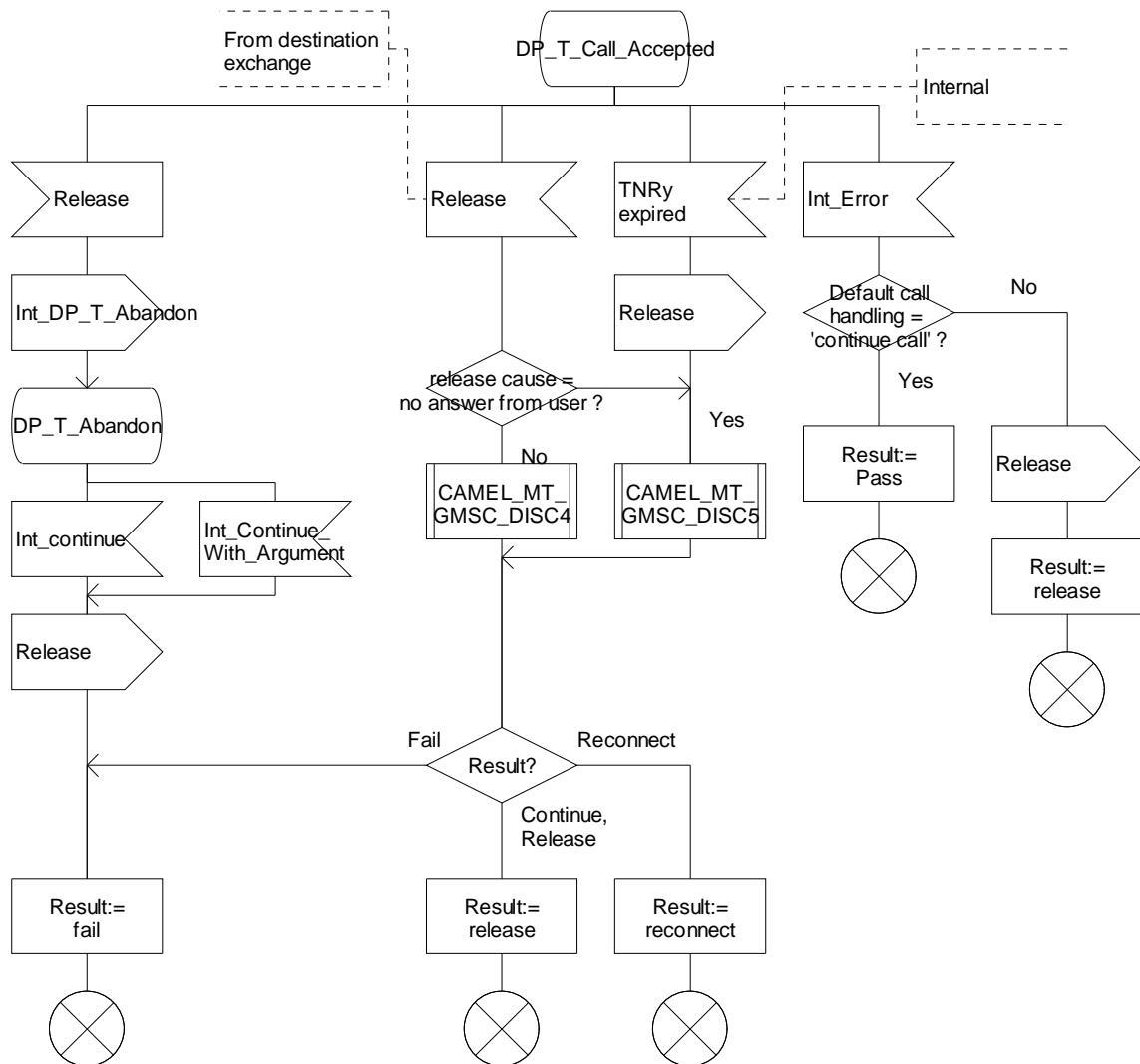
Figure 4.43-2: Procedure CAMEL\_MT\_MSC\_ALERTING (sheet 2)
