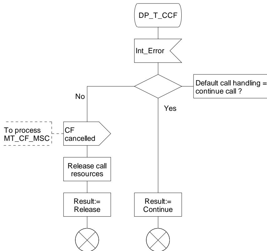
Figure 4.53-2: Procedure CAMEL\_MT\_GMSC\_Notify\_CF (sheet 2)
