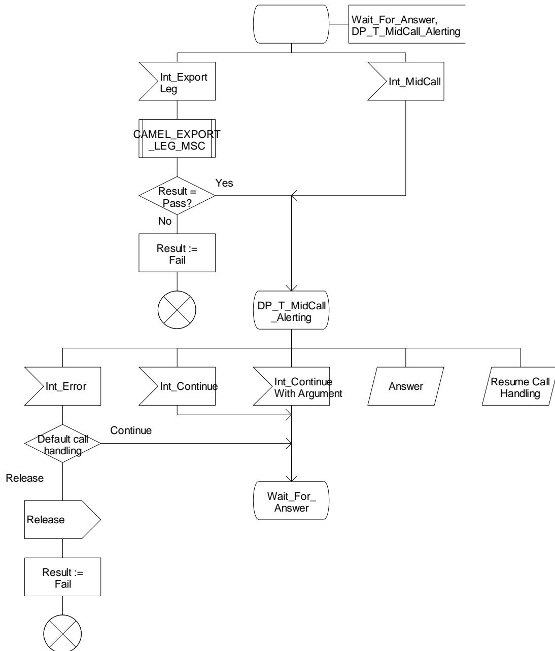
Figure 4.56-5: Procedure CAMEL\_MT\_RECONNECT\_GMSC (sheet 5)
