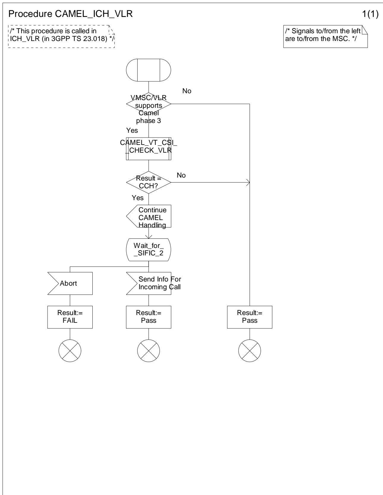
Figure 4.65-1: Procedure CAMEL\_ICH\_VLR (sheet 1)
