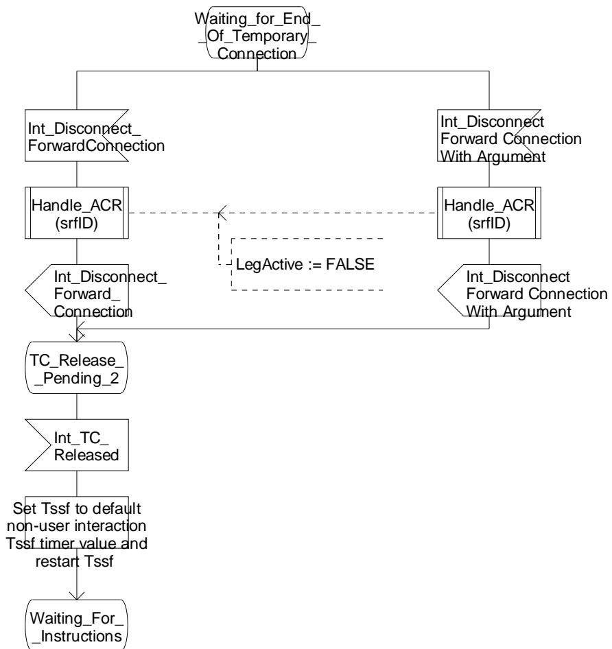
Figure 4.99-39: Process CS\_gsmSSF (sheet 39)
