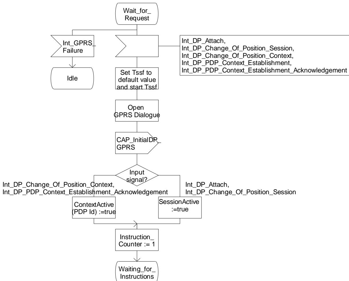
Figure 6.17-2: Process GPRS\_SSF (sheet 2)
