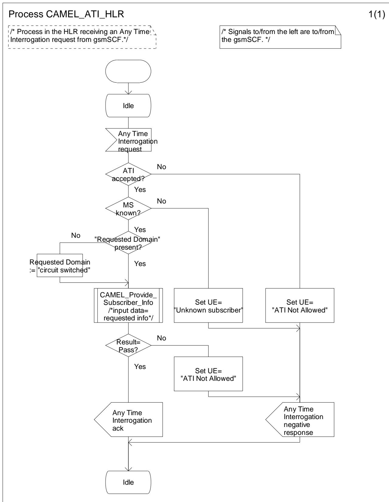
Figure 11.3-1: Process CAMEL\_ATI\_HLR (sheet 1)
