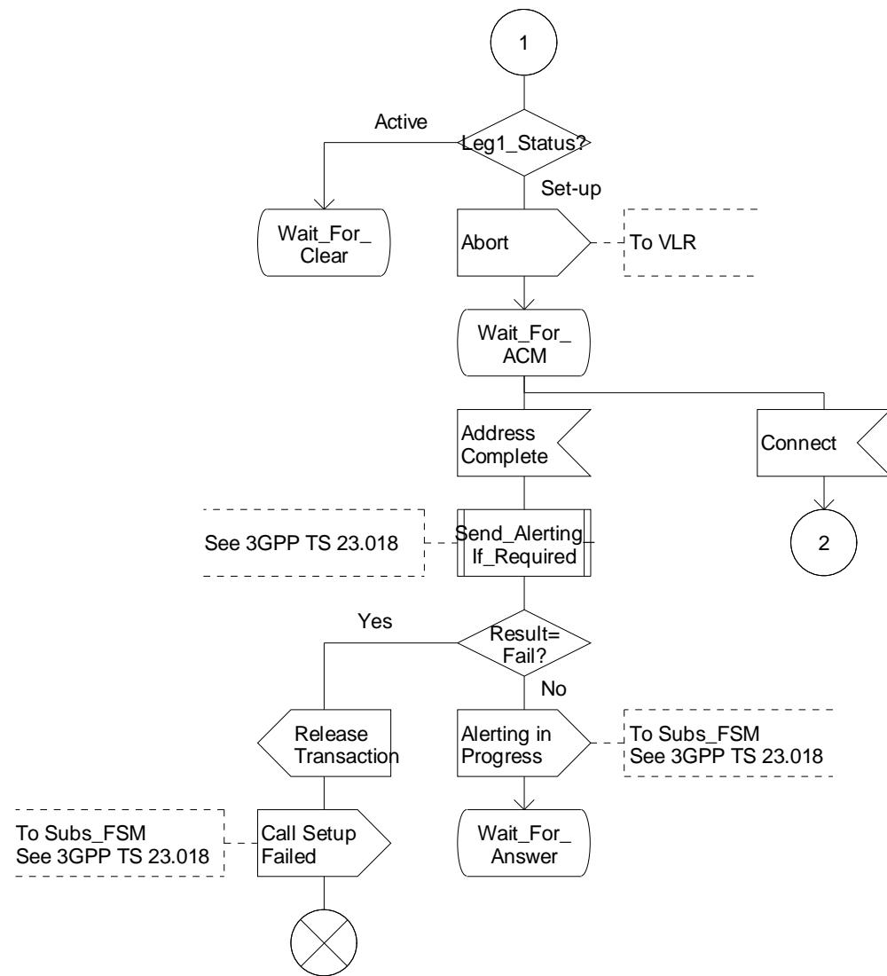
Figure 4.30-2: Procedure CAMEL\_OCH\_LEG1\_MSC (sheet 2)
