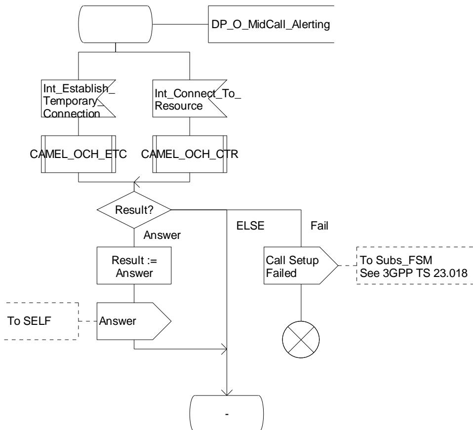
Figure 4.30-12: Procedure CAMEL\_OCH\_LEG1\_MSC (sheet 12)
