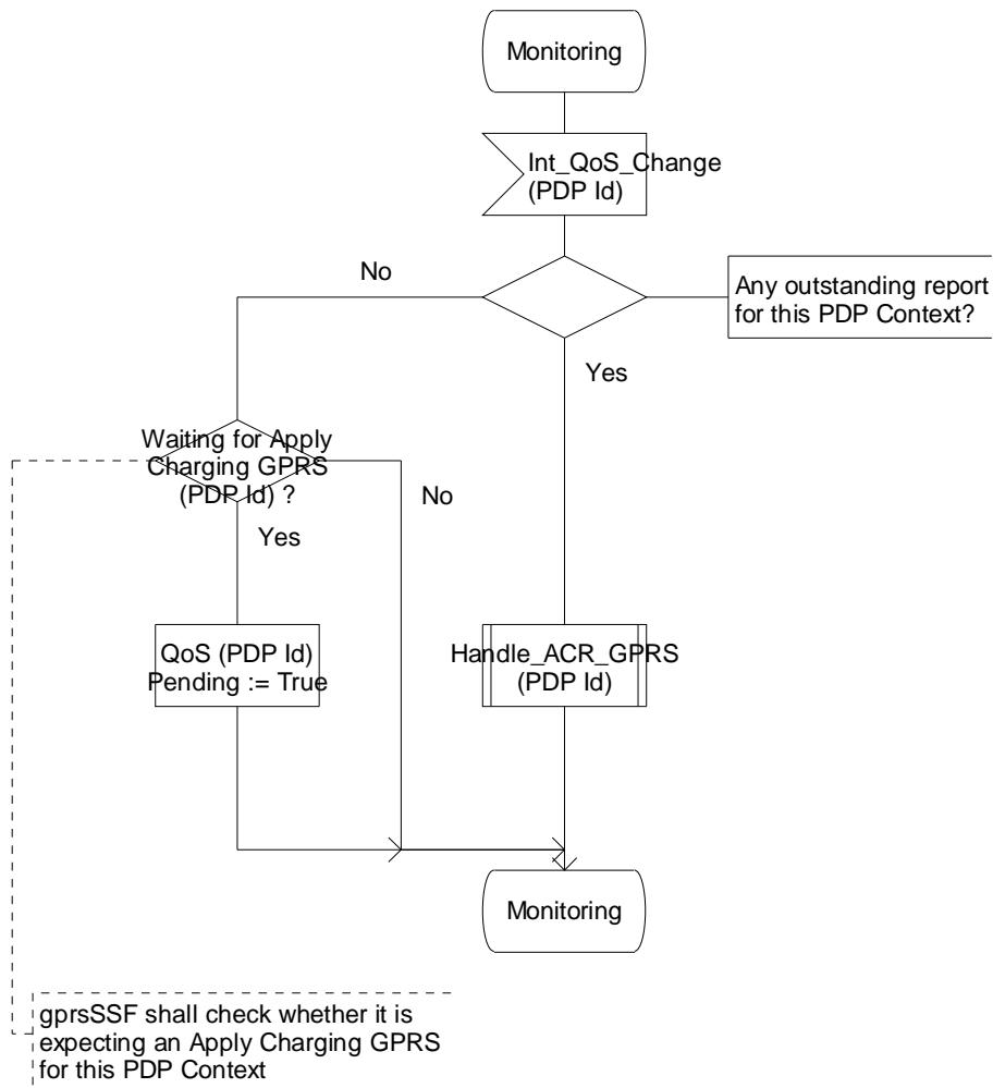
gprsSSF shall check whether it is expecting an Apply Charging GPRS for this PDP Context
