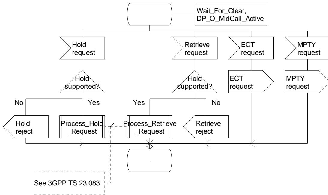
Figure 4.30-6: Procedure CAMEL\_OCH\_LEG1\_MSC (sheet 6)
