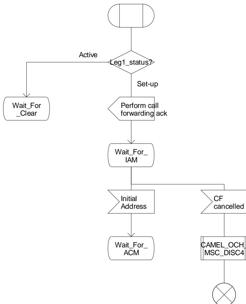
**Figure 4.86-1: Procedure CAMEL\_MT\_CF\_LEG1\_MSC (sheet 1)**
