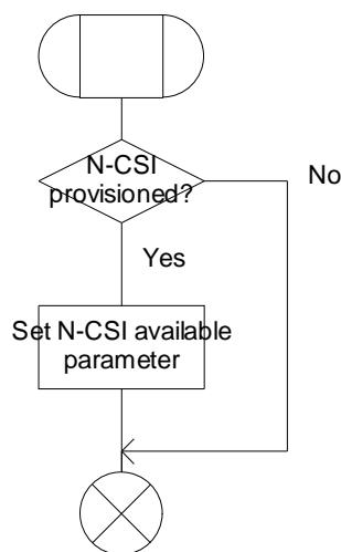
Figure 4.29-1: Procedure CAMEL\_N\_CSI\_CHECK\_MSC (sheet 1)
