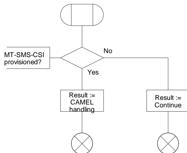
Figure 7.14-1: Procedure CAMEL\_MT\_SMS\_SGSN (sheet 1)
