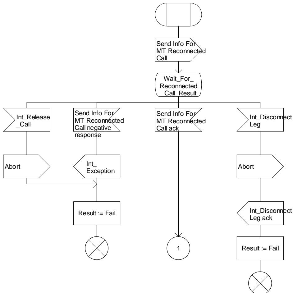
Figure 4.74-1: Procedure CAMEL\_ICH\_RECONNECT\_MSC (sheet 1)
