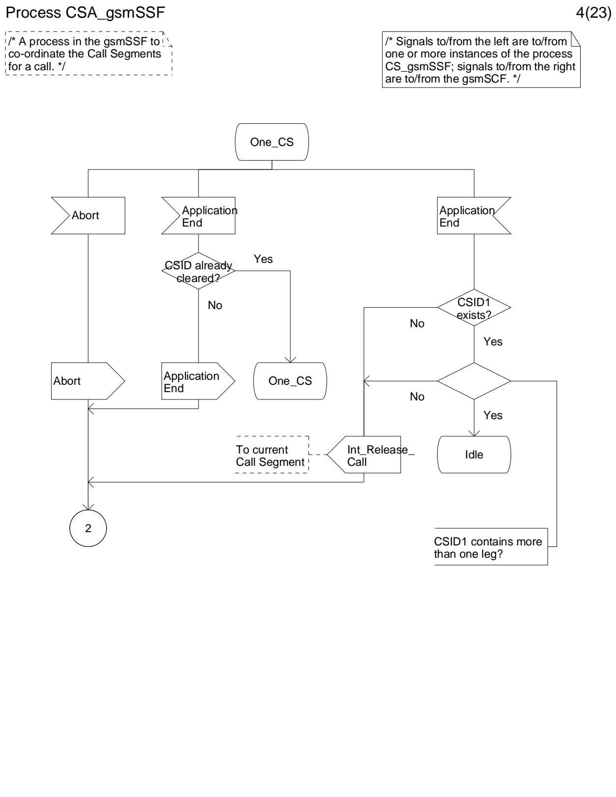
Figure 4.116-4: Process CSA\_gsmSSF (sheet 4)
