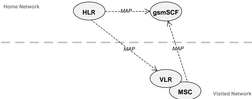
**Figure 8.1: Functional architecture for support of SS Notifications**
