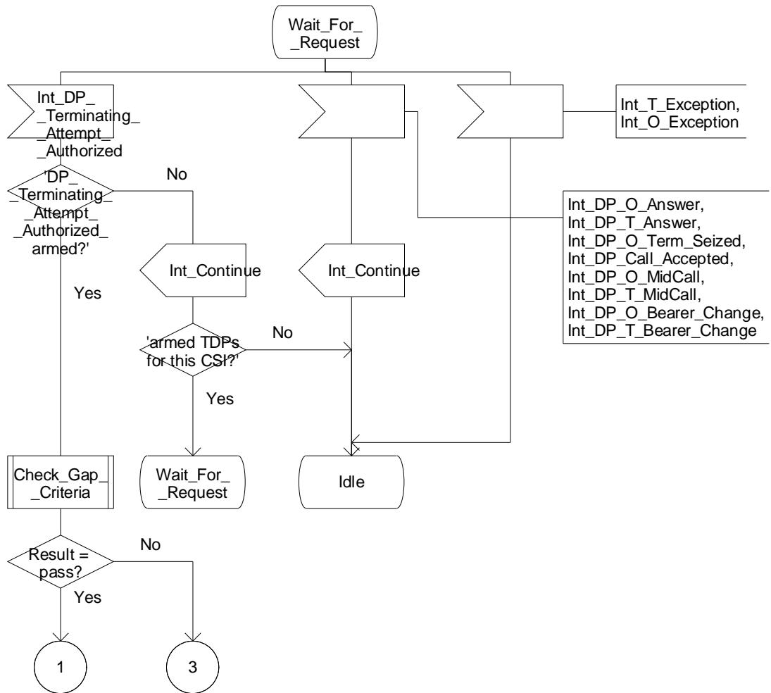
Figure 4.99-6: Process CS\_gsmSSF (sheet 6)
