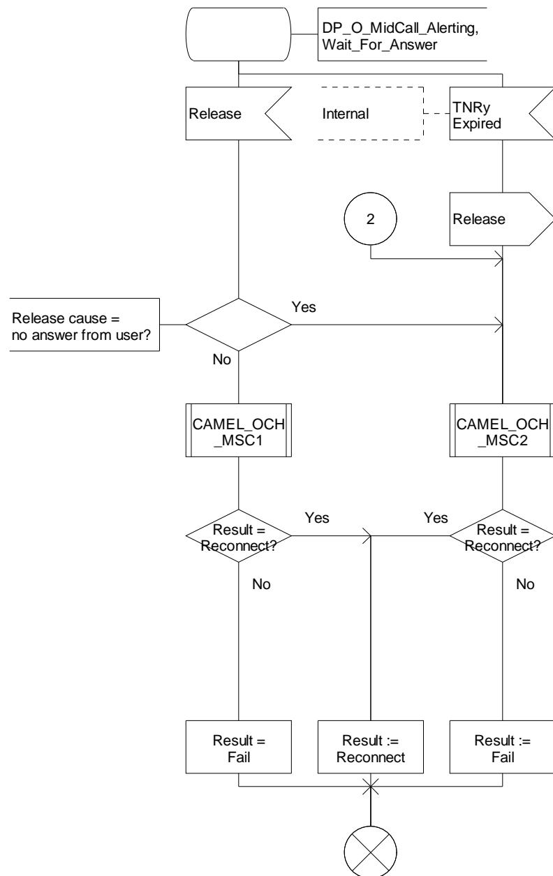
Figure 4.33-5: Procedure CAMEL\_OCH\_RECONNECT\_MSC (sheet 5)
