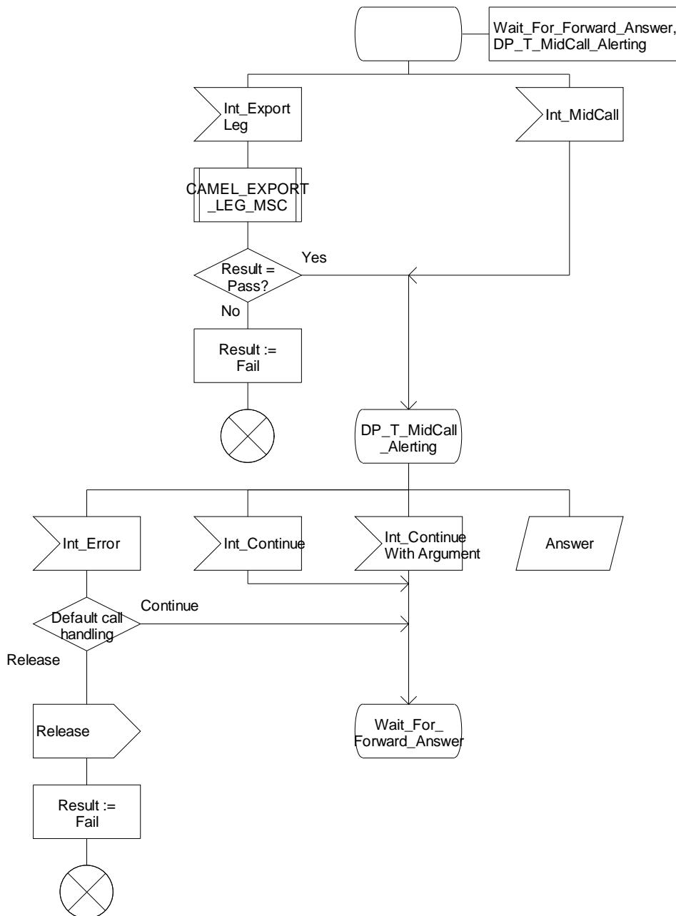
Figure 4.74-5: Procedure CAMEL\_ICH\_RECONNECT\_MSC (sheet 5)
