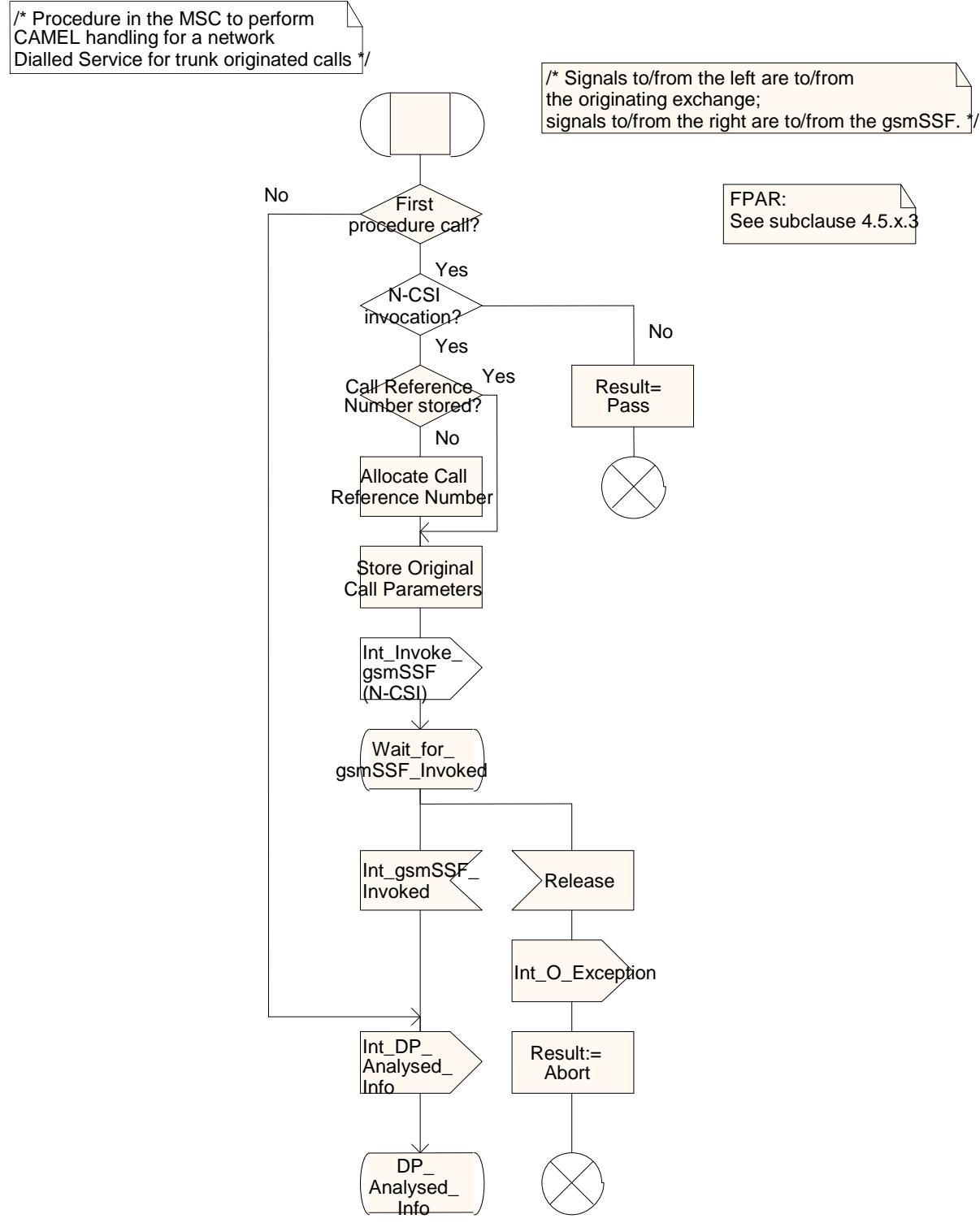
Figure 4.119C-1: Procedure CAMEL\_NDS\_TOC\_INIT (sheet 1)
