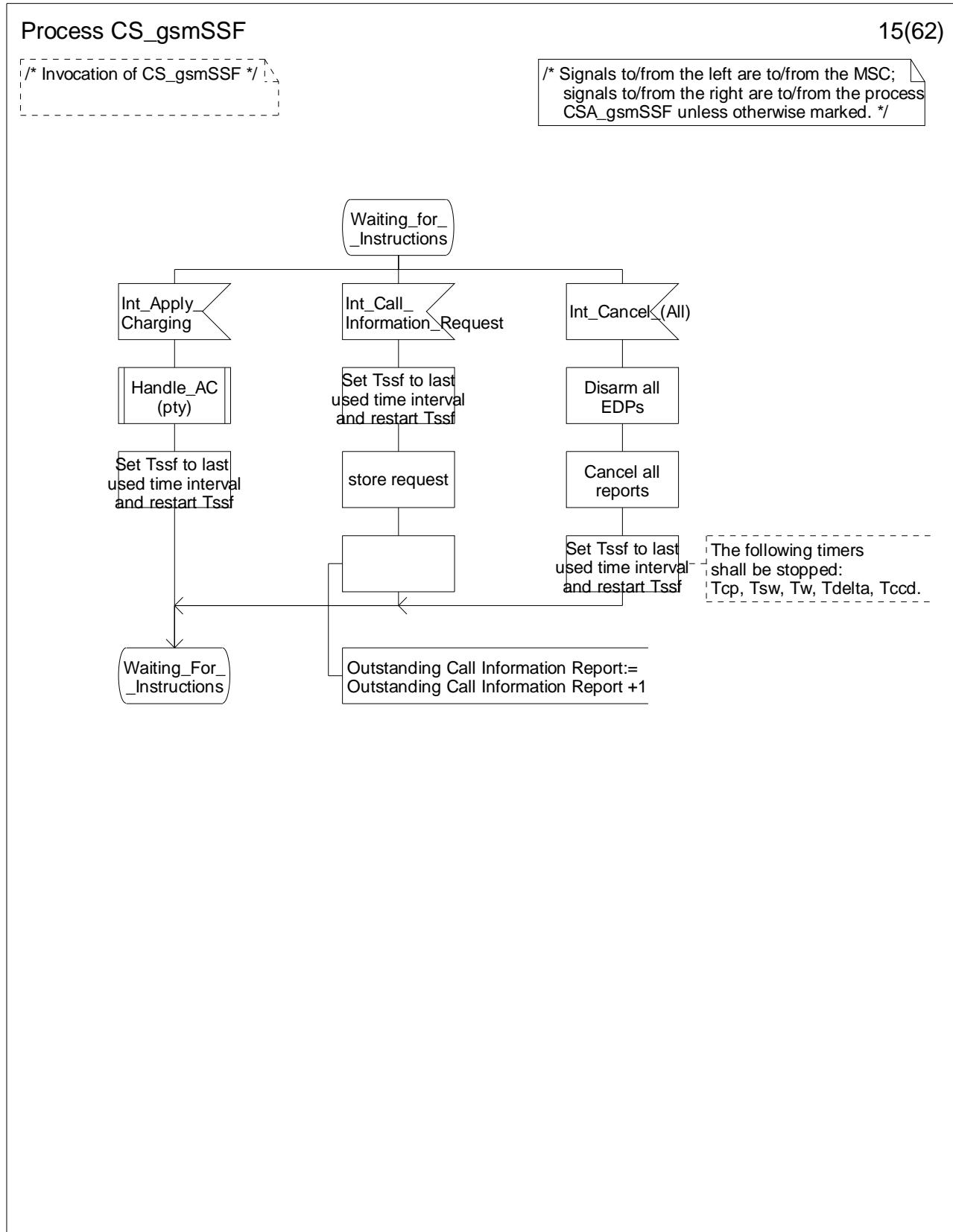
**Figure 4.99-15: Process CS\_gsmSSF (sheet 15)**
