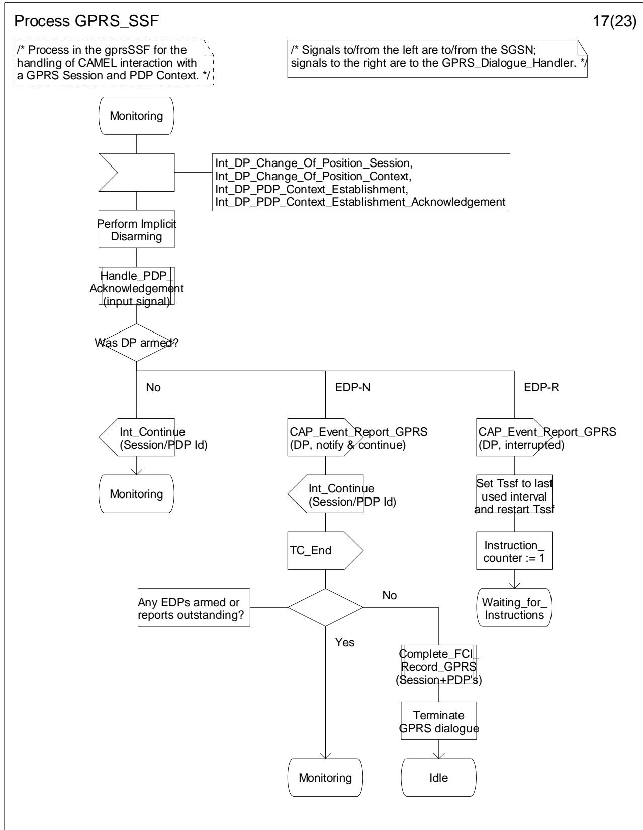
**Figure 6.17-17: Process GPRS\_SSF (sheet 17)**
