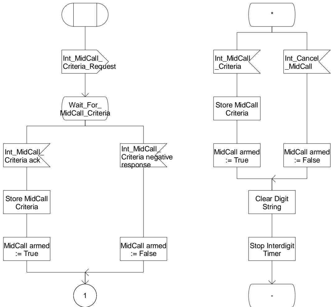
Figure 4.30-1: Procedure CAMEL\_OCH\_LEG1\_MSC (sheet 1)
