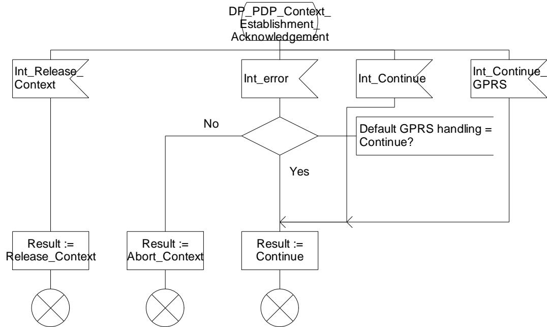
Figure 6.13-2: Procedure CAMEL\_GPRS\_PDP\_Context\_Establishment\_Acknowledgement (sheet 2)
