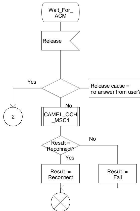
Figure 4.33-3: Procedure CAMEL\_OCH\_RECONNECT\_MSC (sheet 3)
