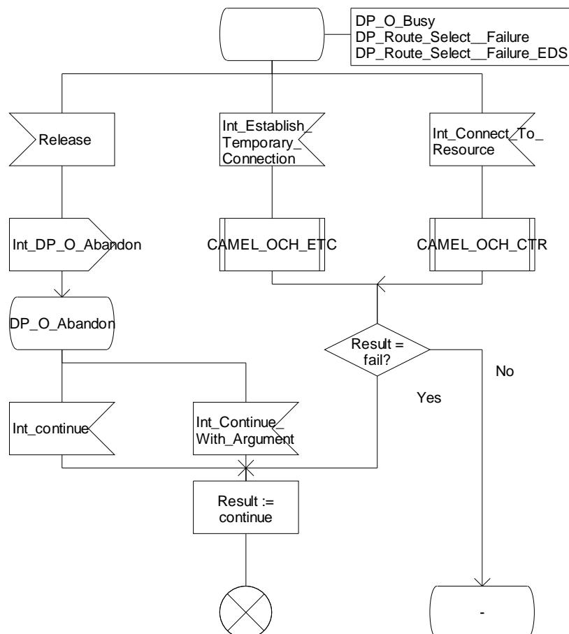
Figure 4.16-3: Procedure CAMEL\_OCH\_MSC1 (sheet 3)
