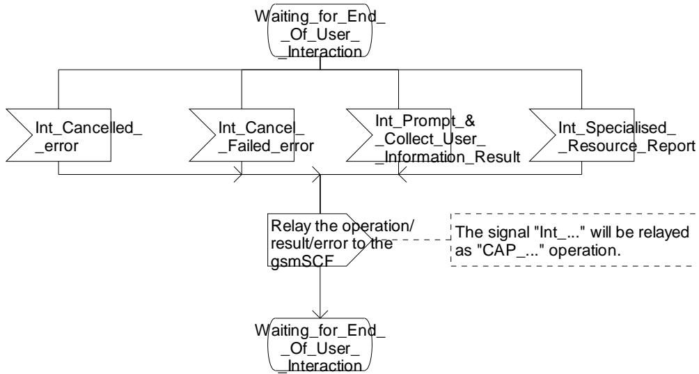
Figure 4.118-4: Process Assisting\_gsmSSF (sheet 4)
