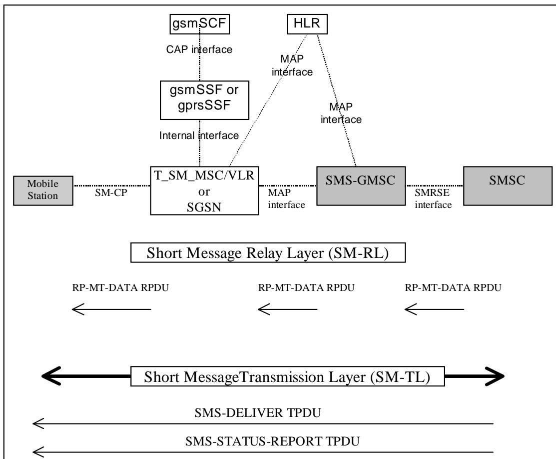
Note 1: The functional entities depicted by means of dark shaded boxes in the figure 7.9 are not affected by CAMEL interaction with MT-SMS.
