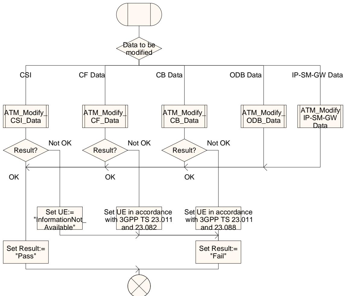
**Figure 10.4-1: Procedure ATM\_Modify\_Data (sheet 1)**
