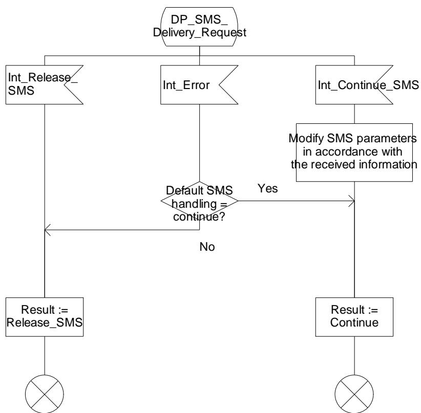
Figure 7.10-2: Procedure CAMEL\_T\_SMS\_INIT (sheet 2)
