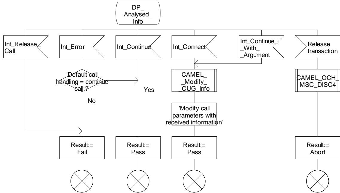
Figure 4.13-2: Procedure CAMEL\_NDS\_MO\_INIT (sheet 2)
