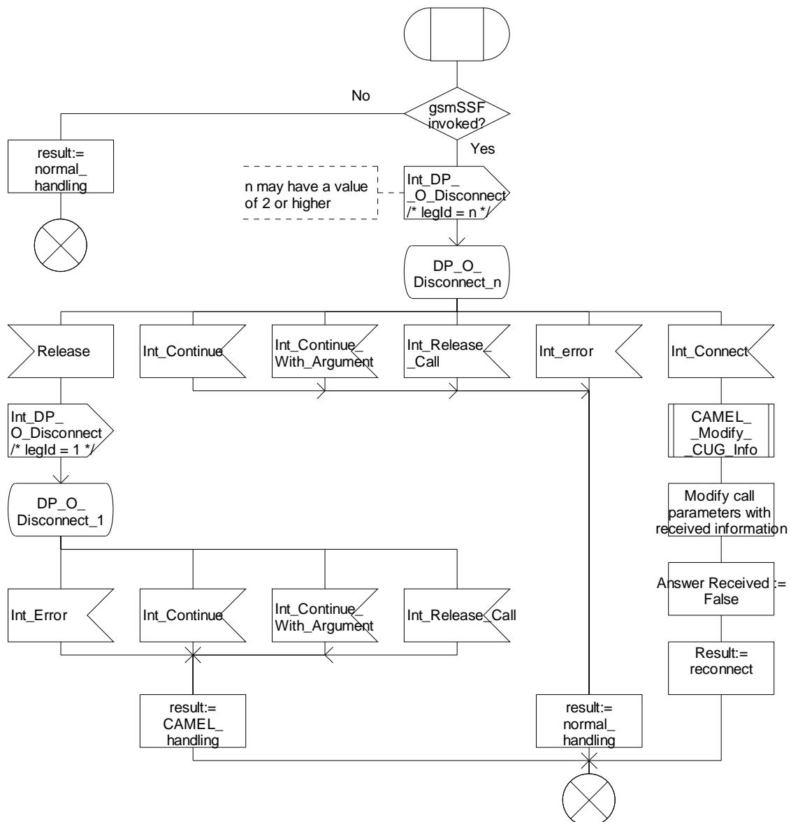
Figure 4.19-1: Procedure CAMEL\_OCH\_MSC\_DISC2 (sheet 1)
