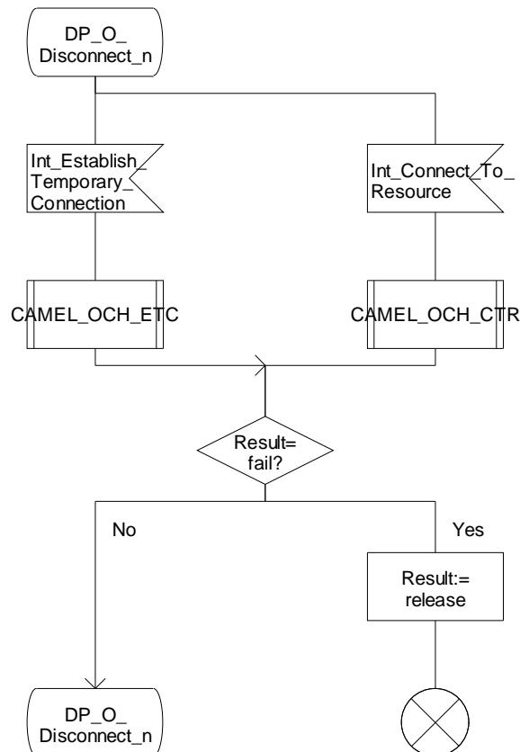
Figure 4.19-2: Procedure CAMEL\_OCH\_MSC\_DISC2 (sheet 2)
