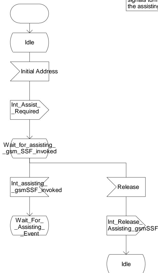
Figure 4.117-1: Process CAMEL\_Assisting\_MSC (sheet 1)
