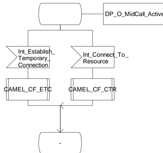
Figure 4.88-6: Procedure CAMEL\_MF\_RECONNECT\_MSC (sheet 6)
