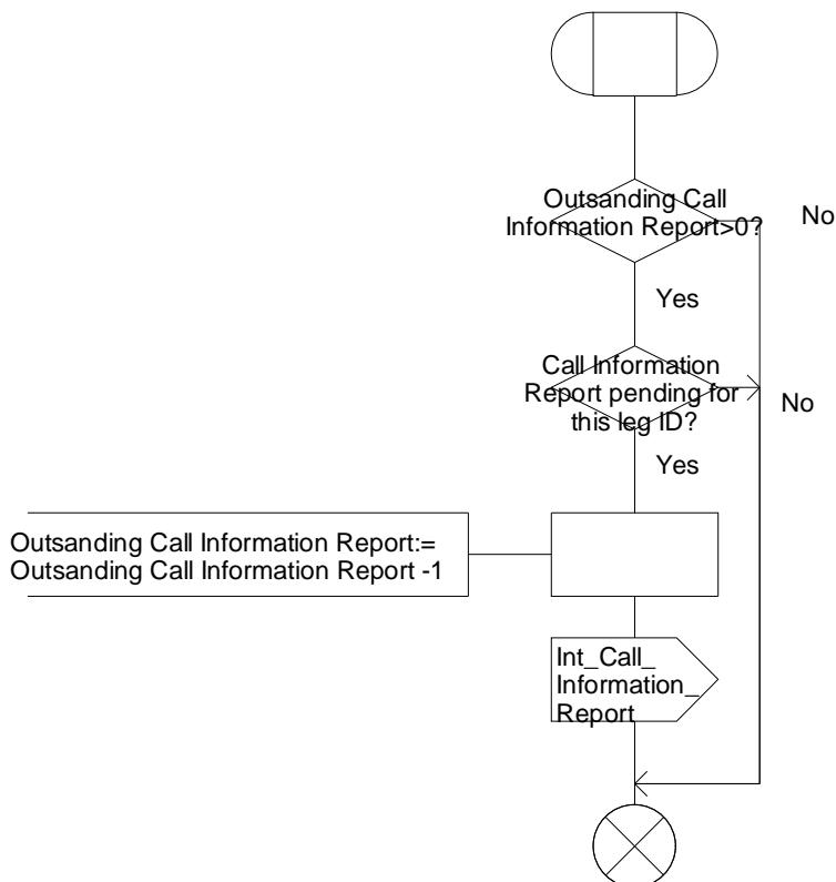
**Figure 4.107-1: Procedure Handle\_CIR\_leg (sheet 1)**
