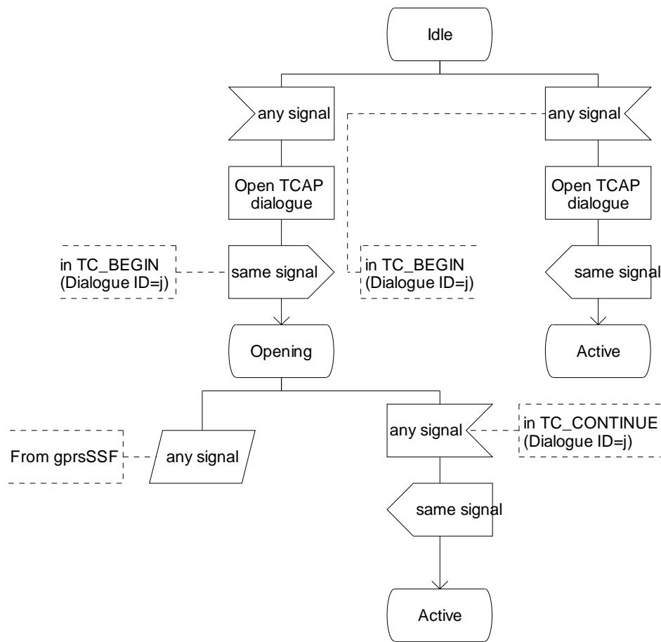
Figure 6.18-1: Process GPRS\_Dialogue\_Handler (sheet 1)
