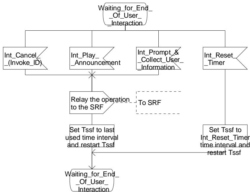
Figure 4.99-41: Process CS\_gsmSSF (sheet 41)
