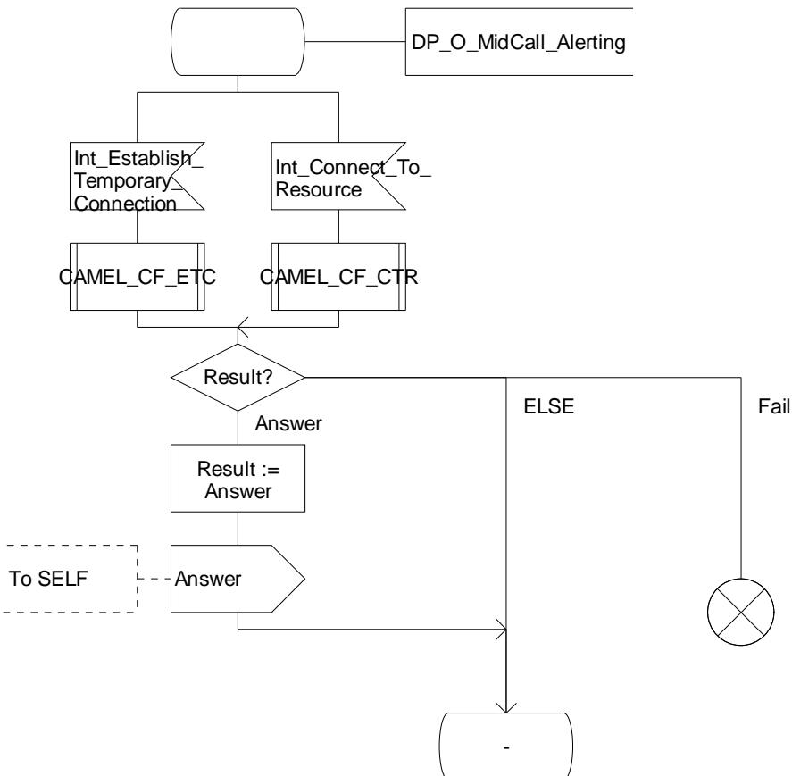
Figure 4.86-5: Procedure CAMEL\_MT\_CF\_LEG1\_MSC (sheet 5)
