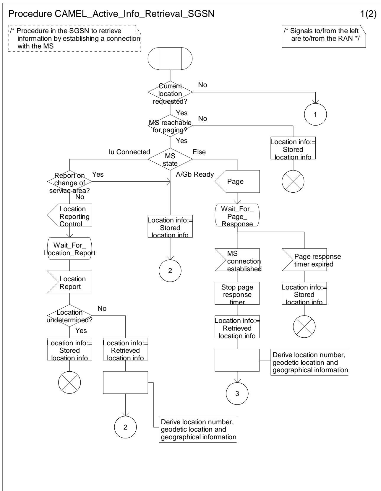
Figure 11.5-1: Procedure CAMEL\_Active\_Info\_Retrieval\_SGSN (sheet 1)
