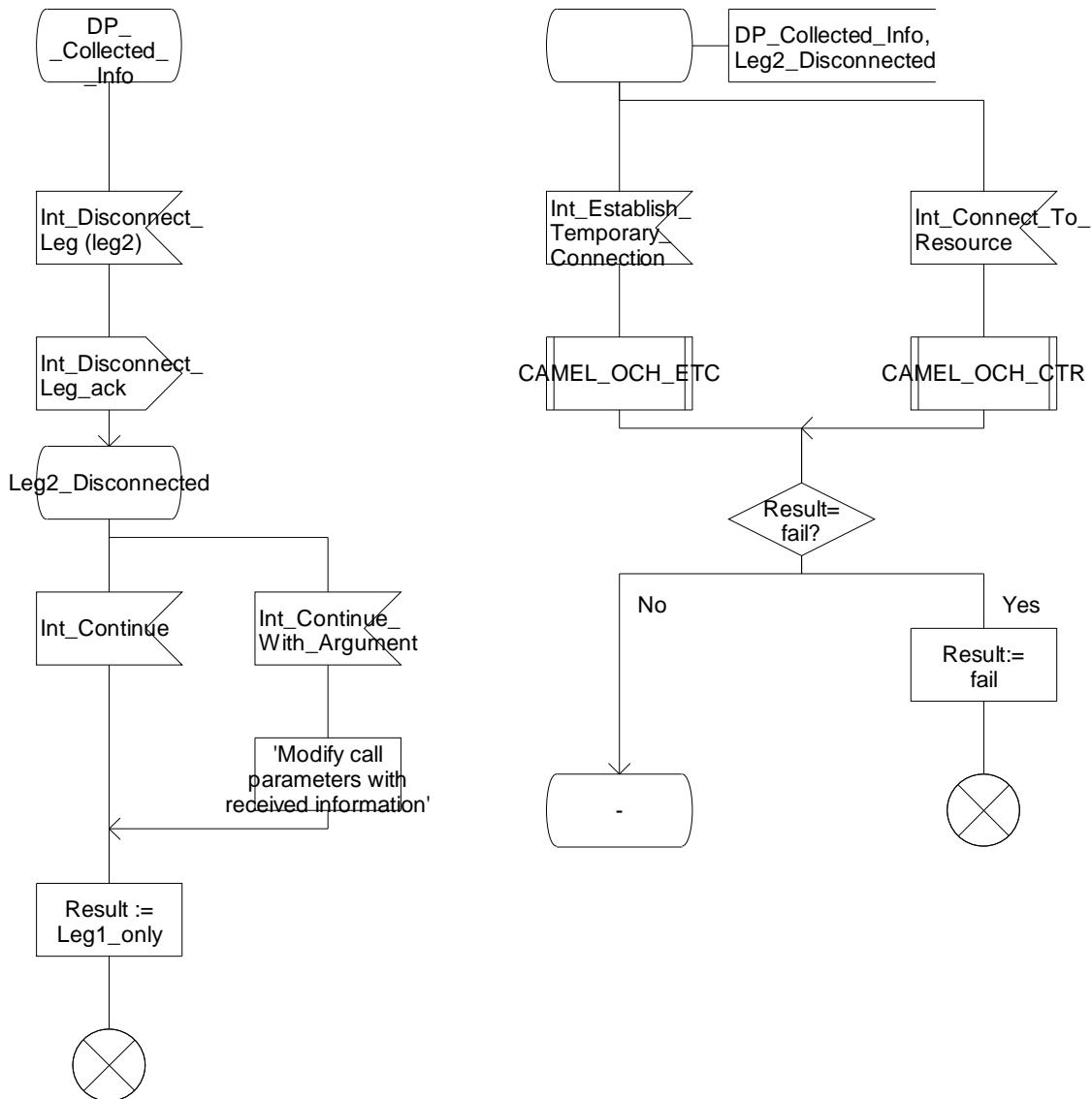
Figure 4.10-3: Procedure CAMEL\_OCH\_MSC\_INIT (sheet 3)
