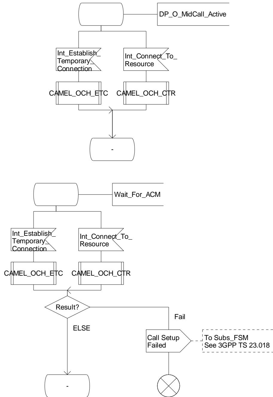
Figure 4.30-13: Procedure CAMEL\_OCH\_LEG1\_MSC (sheet 13)
