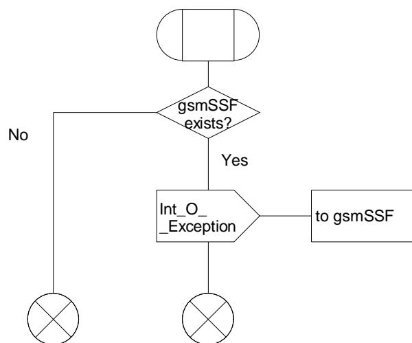
Figure 4.20-1: Procedure CAMEL\_OCH\_MSC\_DISC3 (sheet 1)
