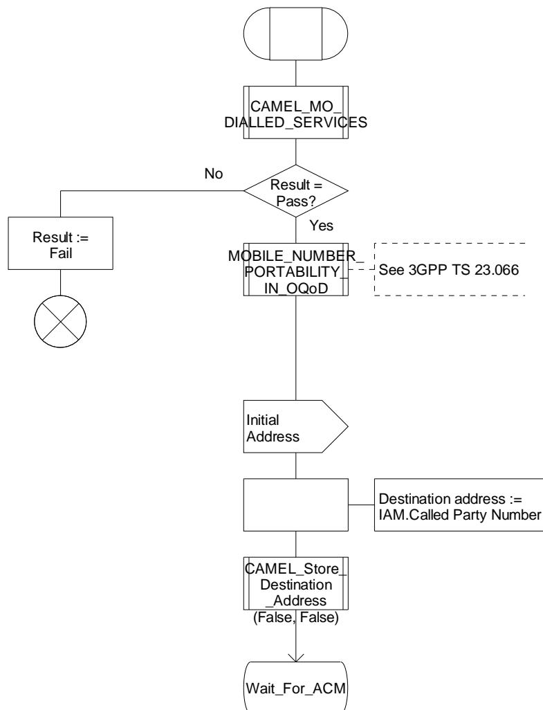
Figure 4.33-1: Procedure CAMEL\_OCH\_RECONNECT\_MSC (sheet 1)
