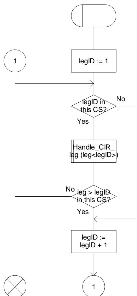
**Figure 4.106-1: Procedure Handle\_CIR (sheet 1)**
