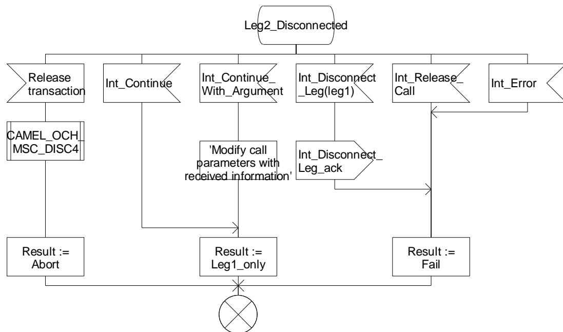
**Figure 4.13-4: Procedure CAMEL\_NDS\_MO\_INIT (sheet 4)**
