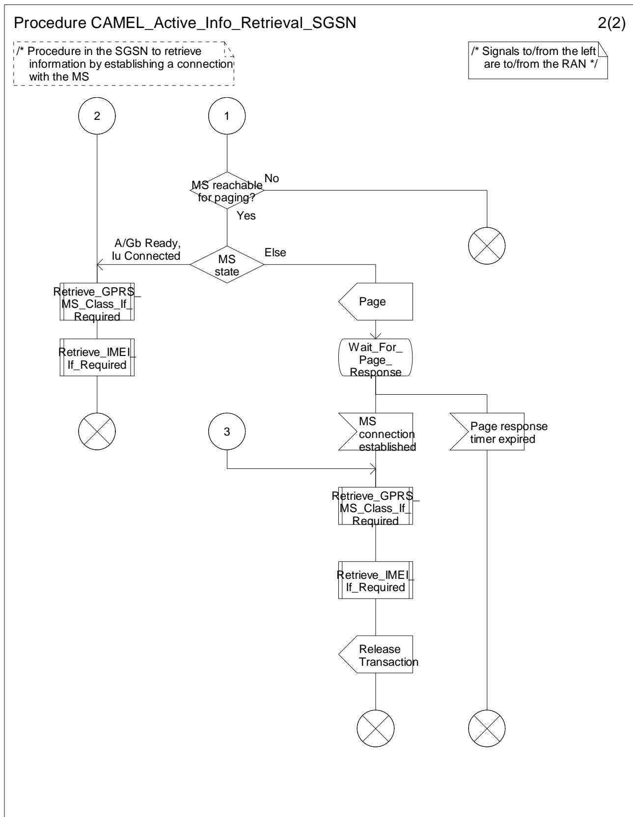
Figure 11.5-2: Procedure CAMEL\_Active\_Info\_Retrieval\_SGSN (sheet 2)
