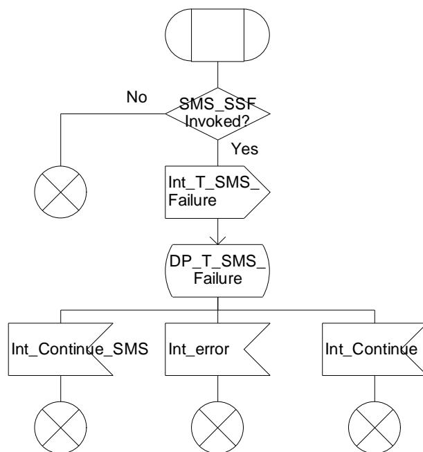
**Figure 7.11-1: Procedure CAMEL\_T\_SMS\_FAILURE (sheet 1)**
