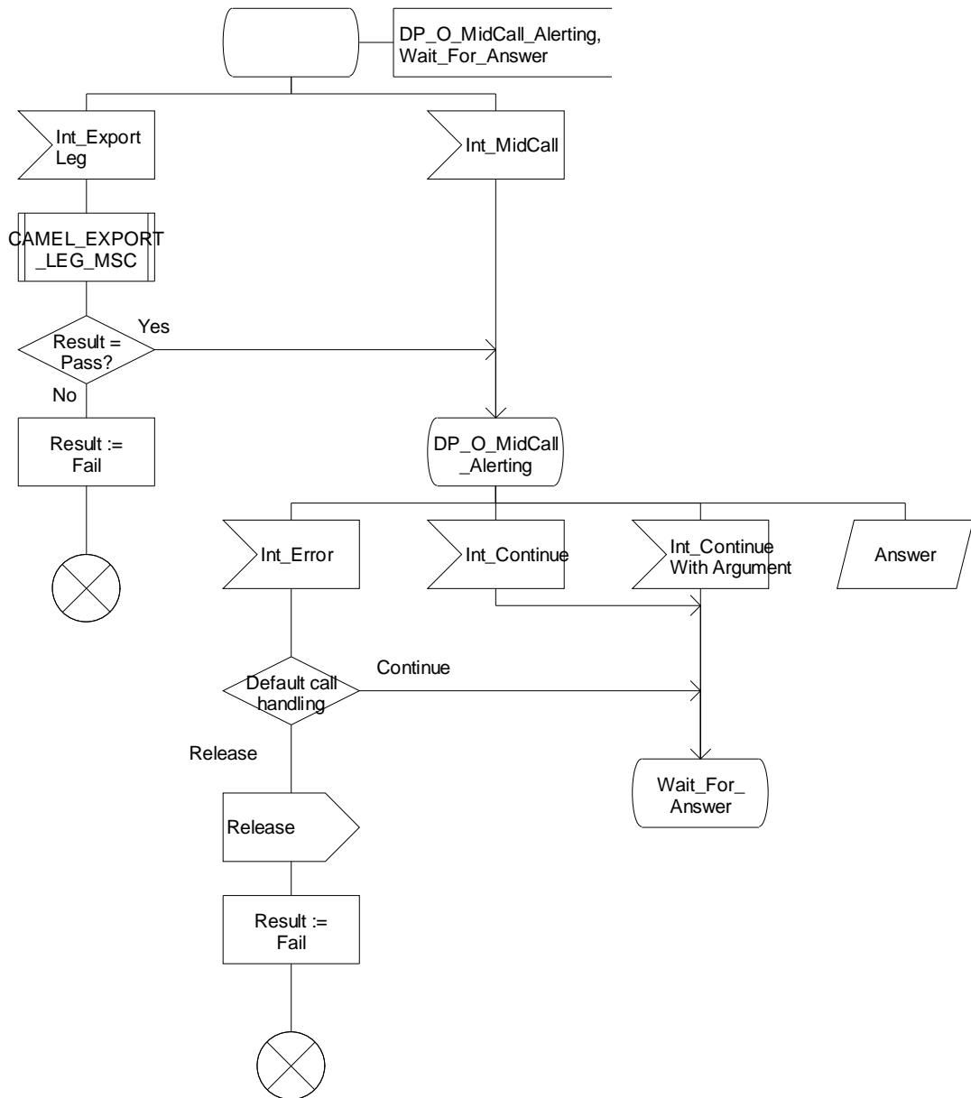
Figure 4.33-7: Procedure CAMEL\_OCH\_RECONNECT\_MSC (sheet 7)
