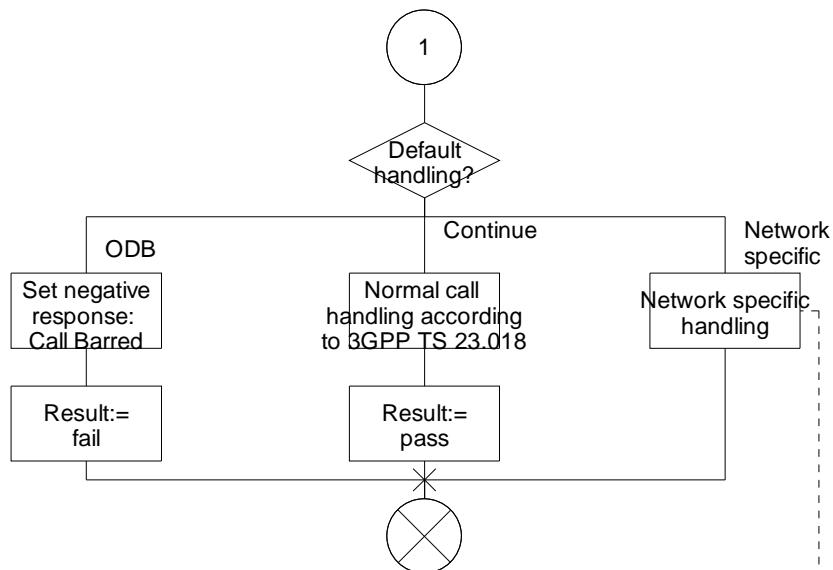
The network specific handling shall include the result of the procedure CAMEL\_HLR\_INIT (fail, pass)
