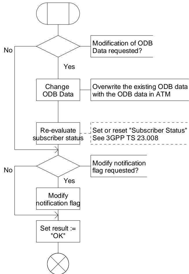
Figure 10.8-1: Procedure ATM\_Modify\_ODB\_Data (sheet 1)
