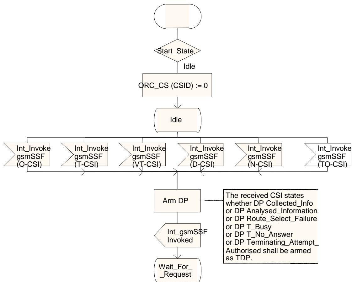
Figure 4.99-3: Process CS\_gsmSSF (sheet 3)
