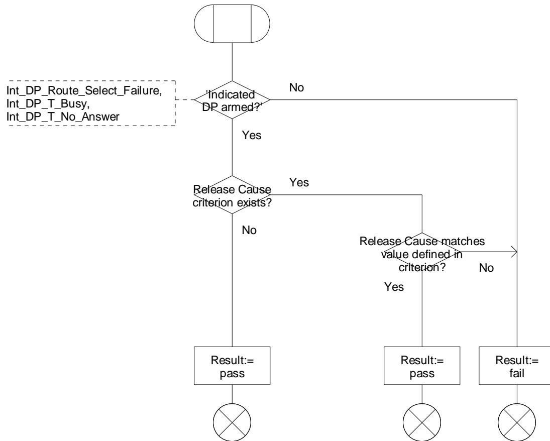
Figure 4.102-1: Procedure Check\_Criteria\_Unsuccessful (sheet 1)
