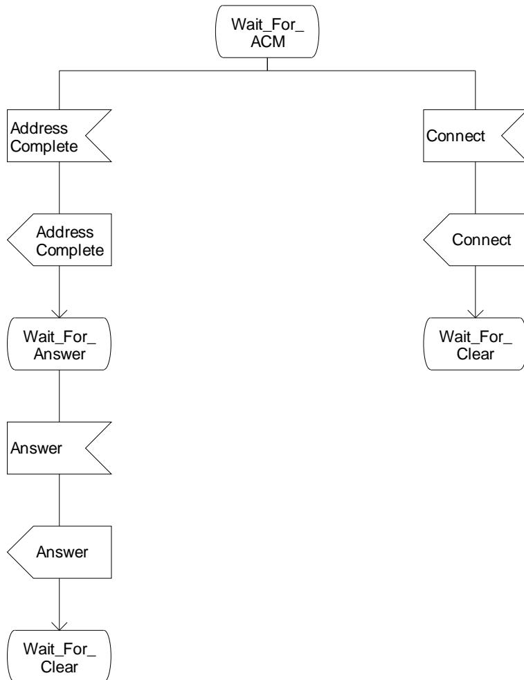
Figure 4.86-2: Procedure CAMEL\_MT\_CF\_LEG1\_MSC (sheet 2)
