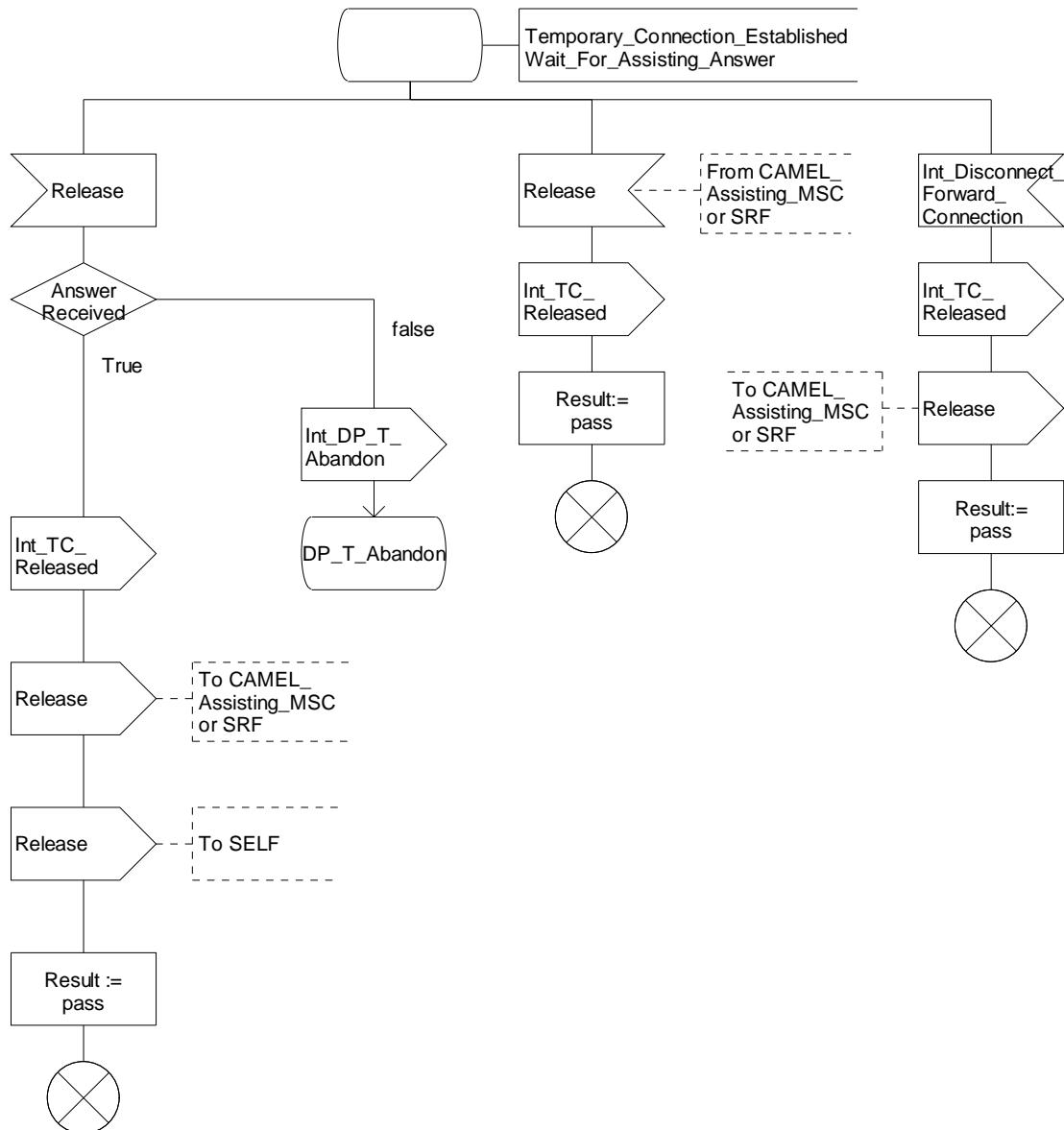
Figure 4.51-3: Procedure CAMEL\_MT\_ETC (sheet 3)
