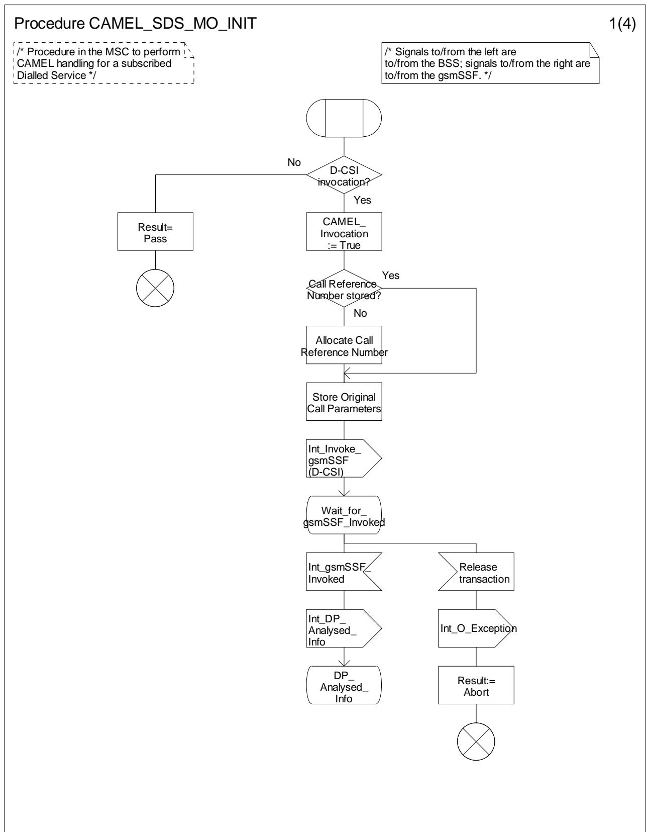
Figure 4.12-1: Procedure CAMEL\_SDS\_MO\_Init (sheet 1)
