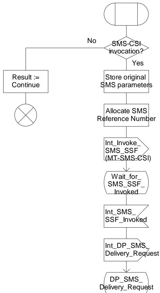
Figure 7.10-1: Procedure CAMEL\_T\_SMS\_INIT (sheet 1)
