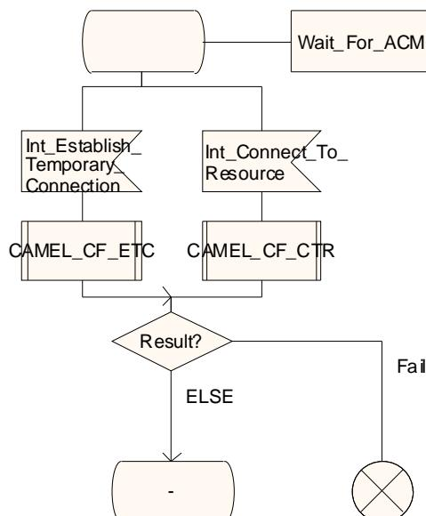
Figure 4.119D-6: Procedure CAMEL\_TOC\_LEG1\_MSC (sheet 6)
