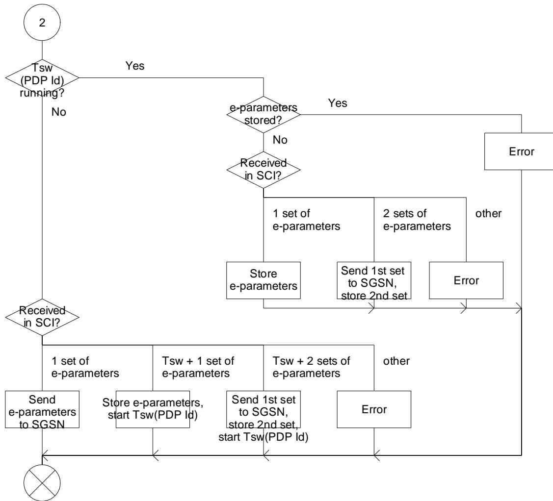
**Figure 6.23-3: Procedure Handle\_SCI\_GPRS (sheet 3)**
