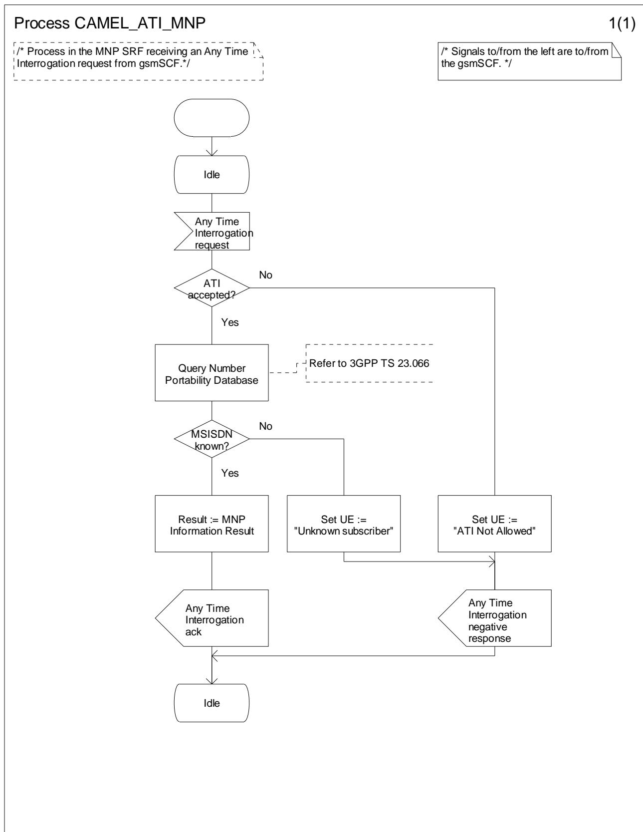
Figure 12.2-1: Process CAMEL\_ATI\_MNP (sheet 1)
