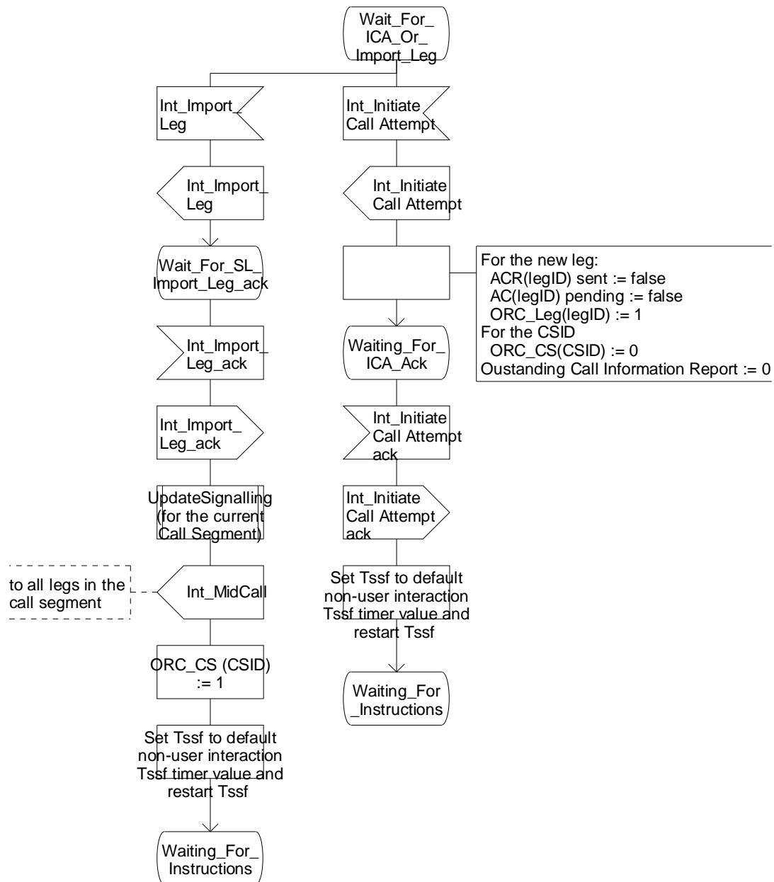
Figure 4.99-11: Process CS\_gsmSSF (sheet 11)
