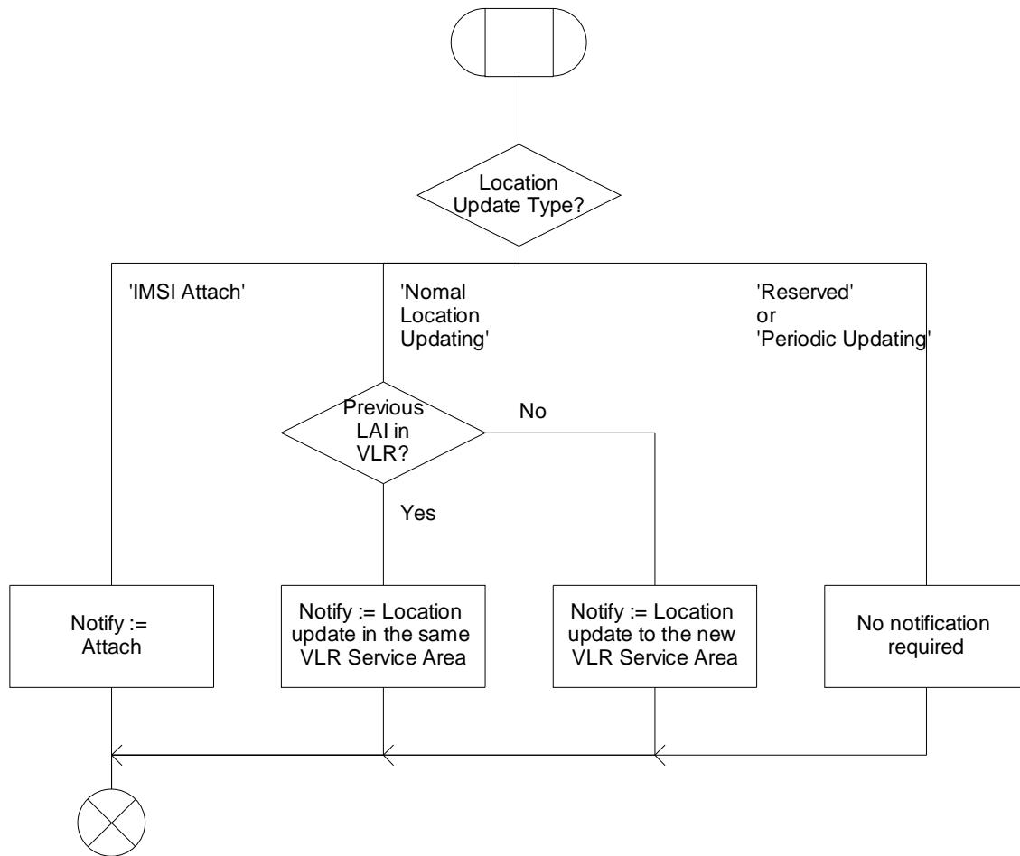
Figure 9.-1a: Procedure Set\_Notification\_Type (sheet 1)
