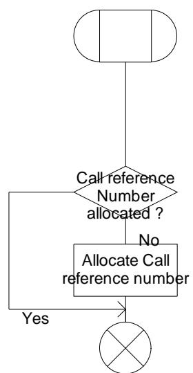
**Figure 4.41-1: Procedure CAMEL\_Set\_ORA\_Parameters (sheet 1)**
