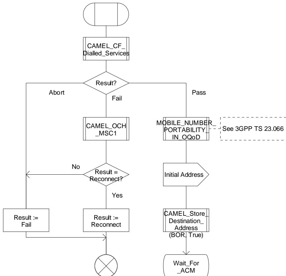
Figure 4.88-1: Procedure CAMEL\_MF\_RECONNECT\_MSC (sheet 1)
