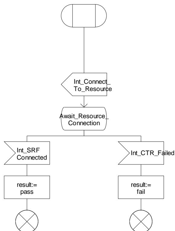
Figure 4.103-1: Procedure Connect\_To\_Resource (sheet 1)
