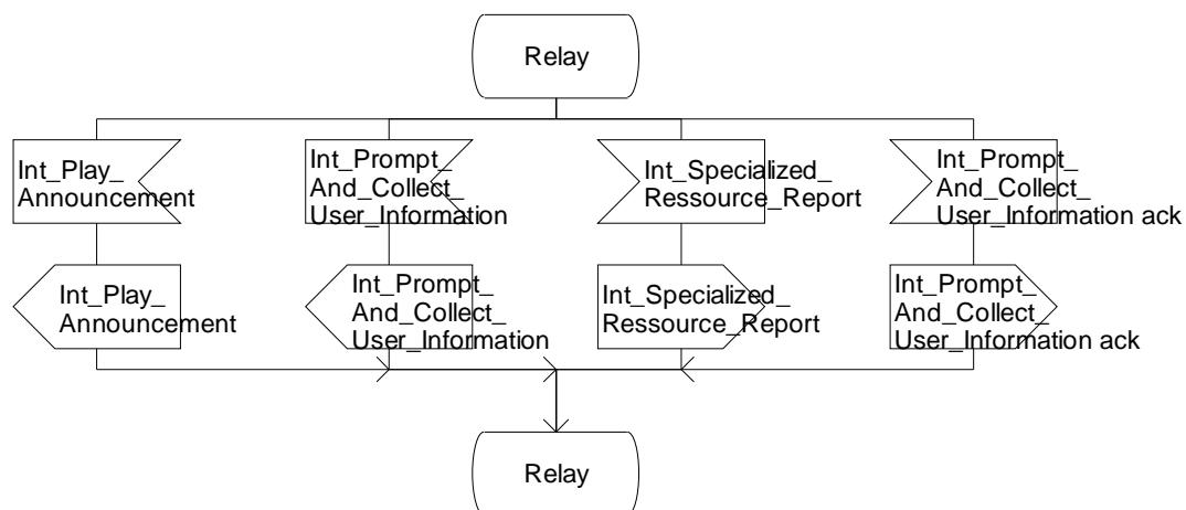
Figure 4.52-3: Procedure CAMEL\_MT\_CTR (sheet 3)
