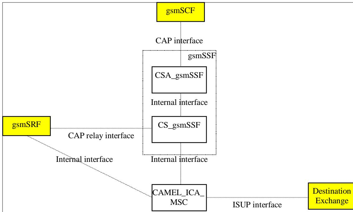
Figure 4.9-8: gsmSCF initiated call case (gsmSSF relay)
