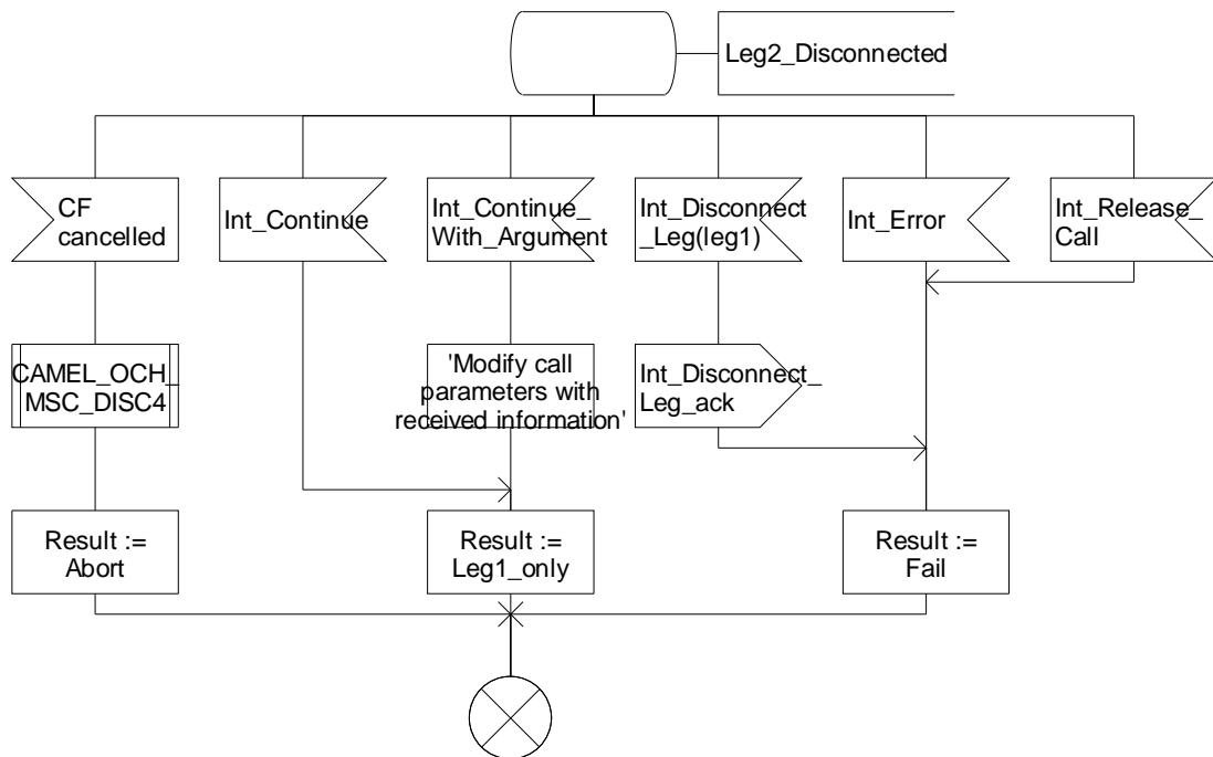
Figure 4.81-4: Procedure CAMEL\_NDS\_CF\_INIT (sheet 4)
