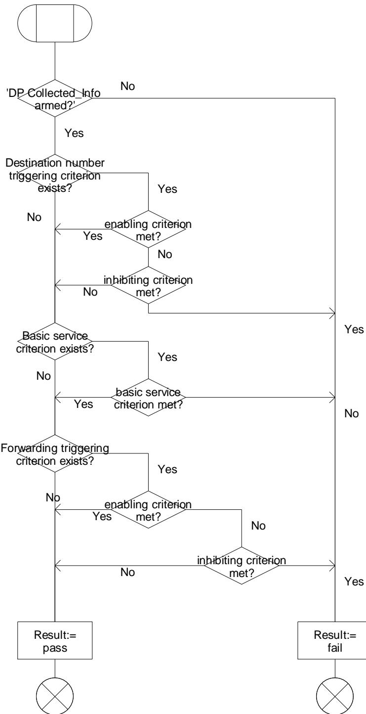
Figure 4.100-1: Procedure Check\_Criteria\_Collected\_Info (sheet 1)
