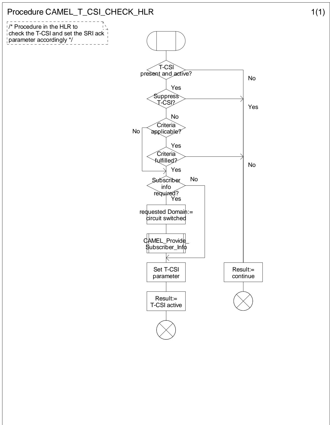
Figure 4.62-1: Procedure CAMEL\_T\_CSI\_CHECK\_HLR (sheet 1)
