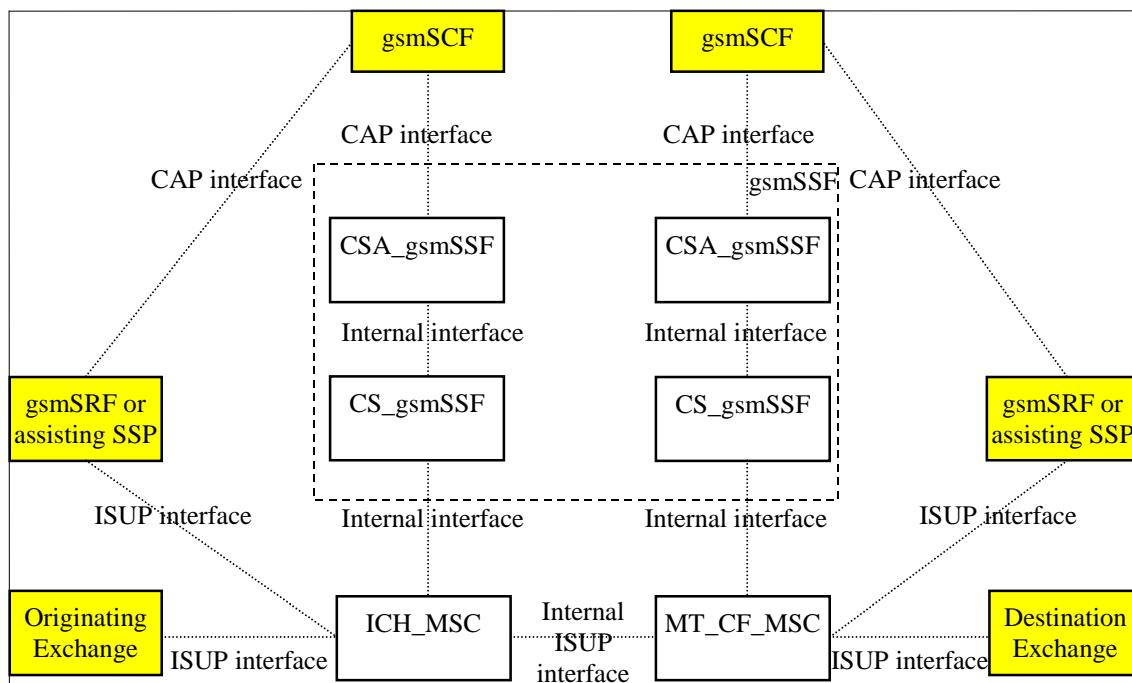
NOTE: The ICH\_MSC may also be connected via an A interface to the terminating Mobile Station
