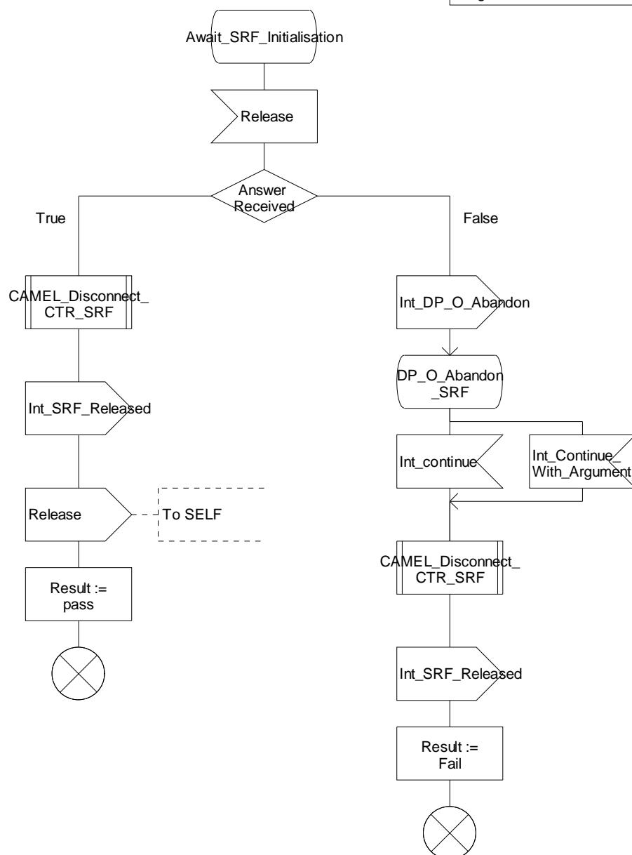
Figure 4.24-4: Procedure CAMEL\_OCH\_CTR (sheet 4)
