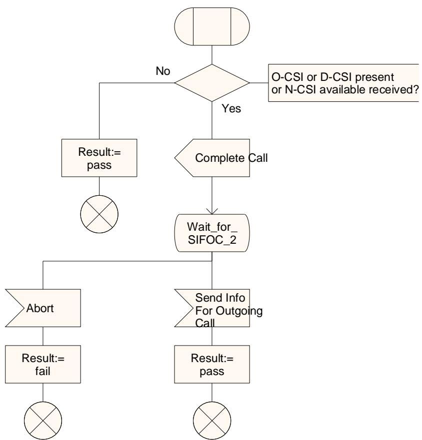
Figure 4.39-1: Procedure CAMEL\_OCH\_VLR (sheet 1)
