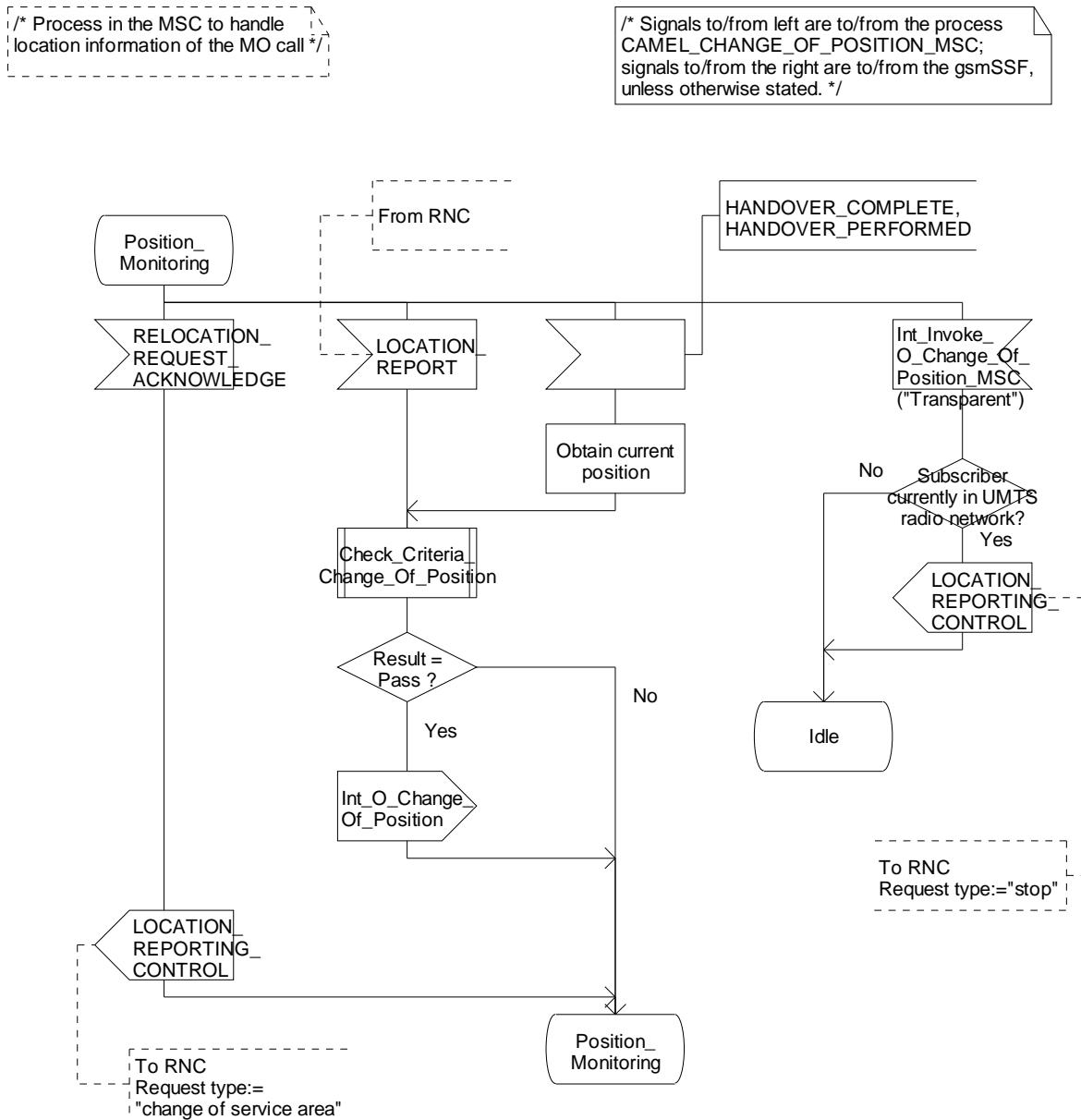
Figure 4.36-2: Process CAMEL\_O\_CHANGE\_OF\_POSITION\_MSC (sheet 2)
