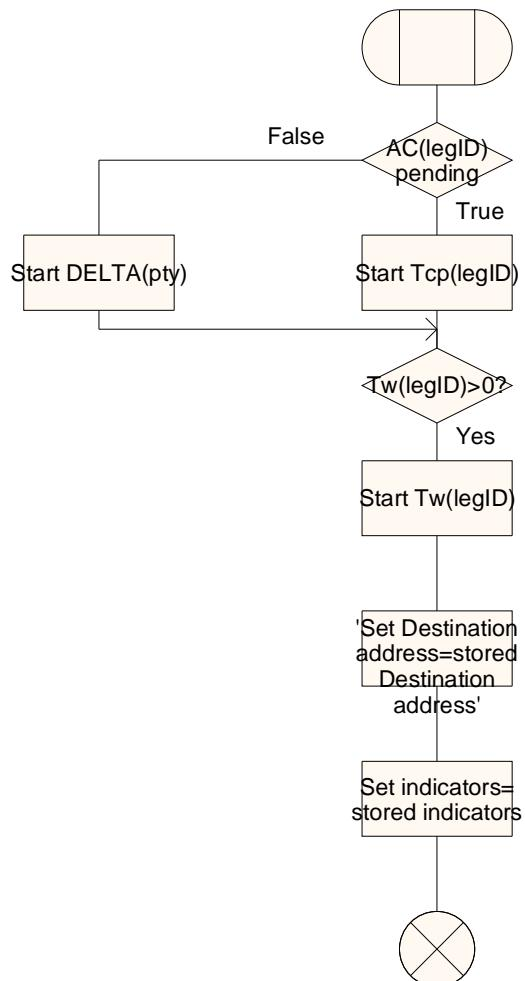
Figure 4.110-1: Procedure Handle\_O\_Answer (sheet 1)
