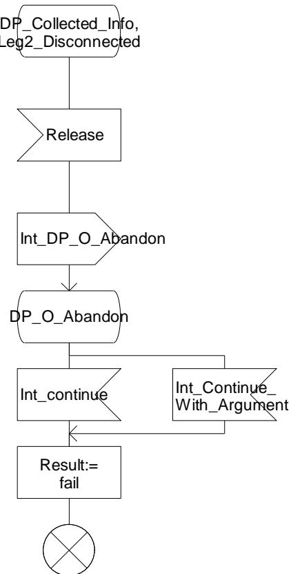
Figure 4.79-4: Procedure CAMEL\_CF\_MSC\_INIT (sheet 4)
