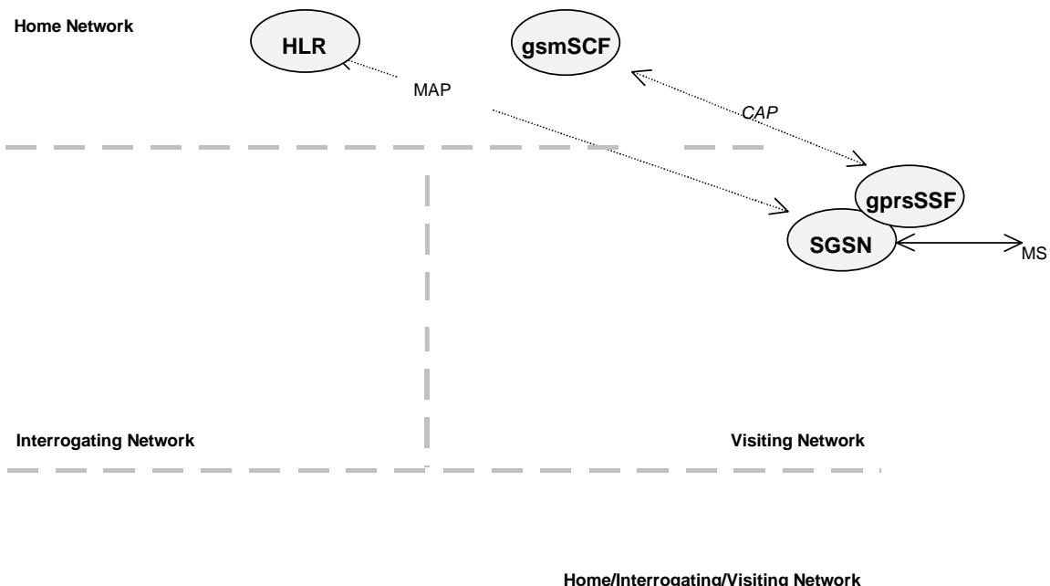
**Figure 6.1: Functional architecture for support of CAMEL**
