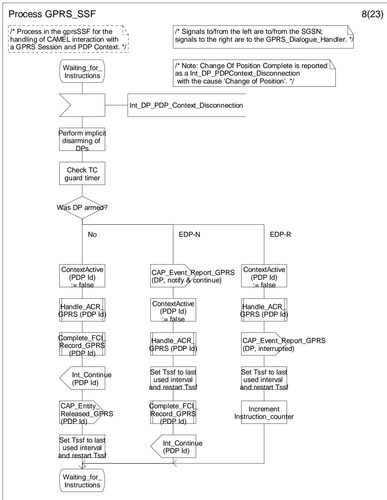
Figure 6.17-8: Process GPRS\_SSF (sheet 8)
