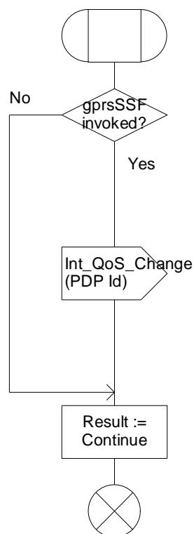
Figure 6.14-1: Procedure CAMEL\_GPRS\_Change\_Of\_QoS (sheet 1)
