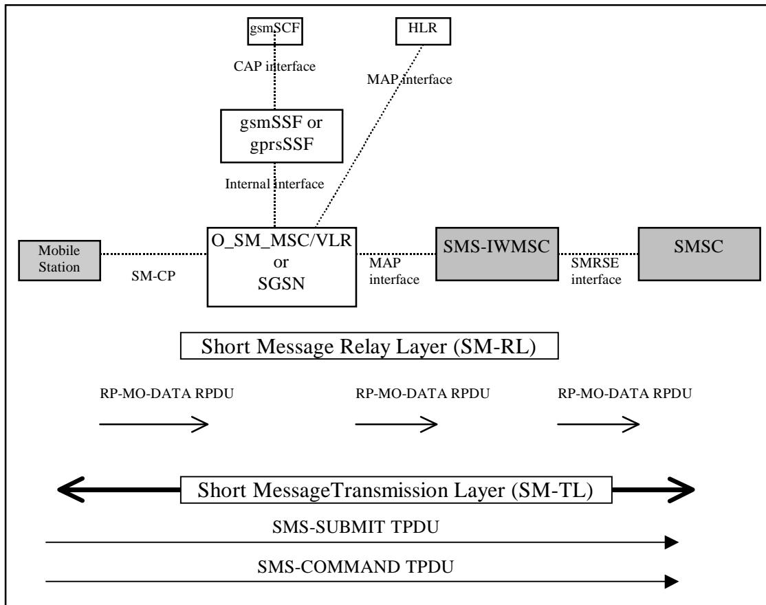
Note 1: The functional entities depicted by means of dark shaded boxes in the figure 7.4 are not affected by CAMEL interaction with MO-SMS.
