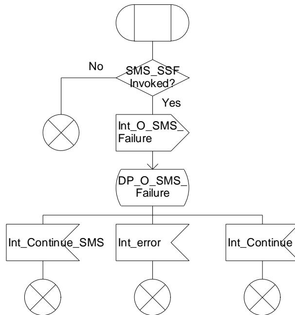
**Figure 7.7-1: Procedure CAMEL\_O\_SMS\_FAILURE (sheet 1)**
