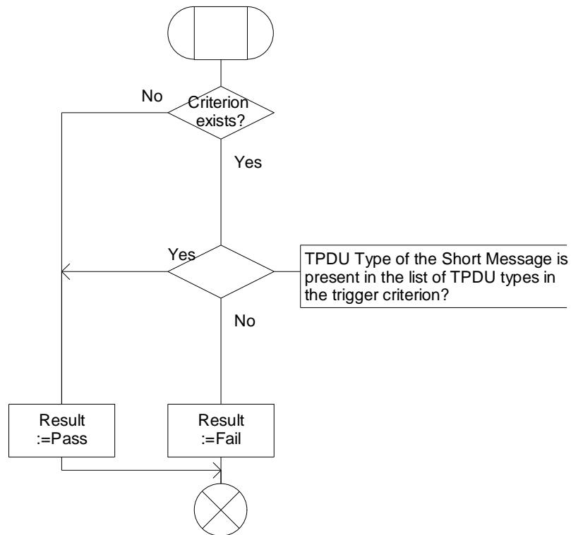
Figure 7.16-1: Procedure Check\_Criteria\_SMS\_Delivery\_Request (Sheet 1)
