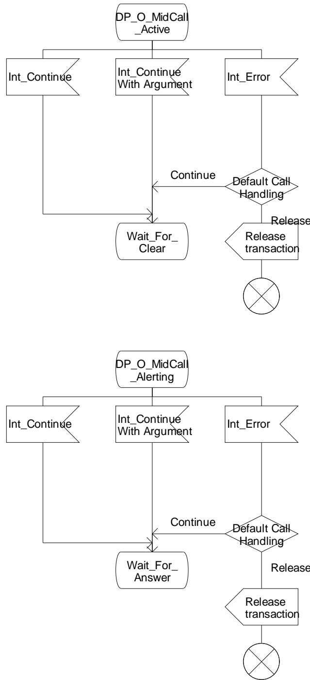
Figure 4.30-9: Procedure CAMEL\_OCH\_LEG1\_MSC (sheet 9)
