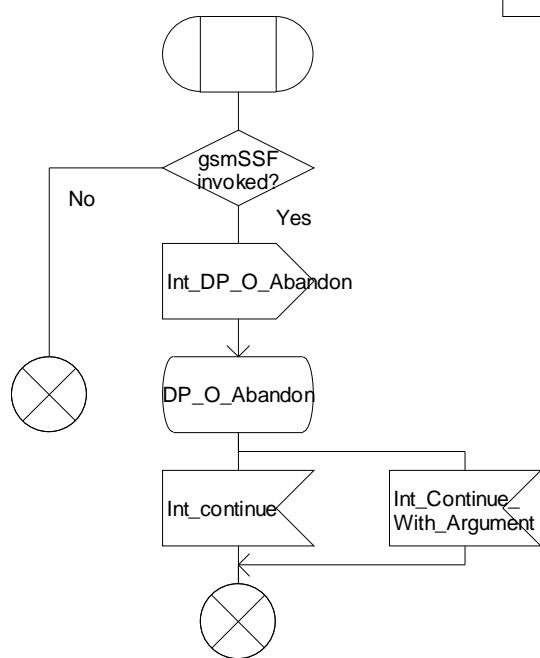
Figure 4.21-1: Procedure CAMEL\_OCH\_MSC\_DISC4 (sheet 1)
