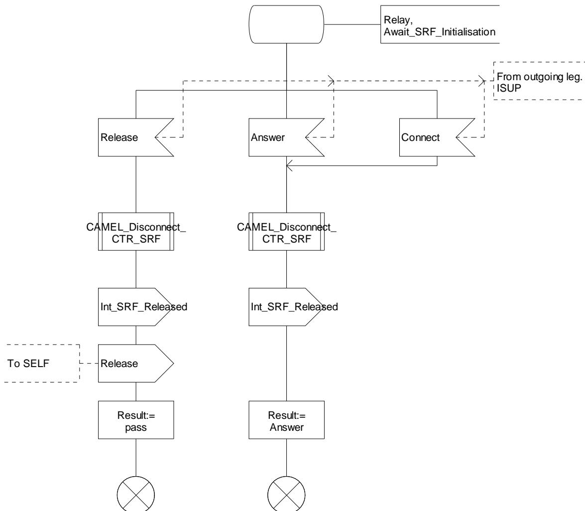
Figure 4.24-5: Procedure CAMEL\_OCH\_CTR (sheet 5)
