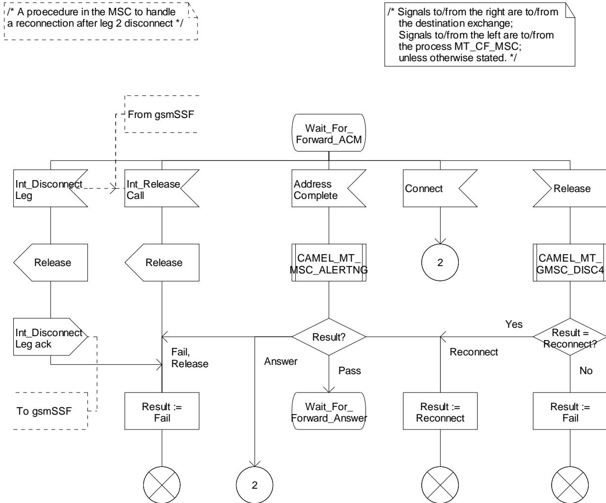
Figure 4.74-3: Procedure CAMEL\_ICH\_RECONNECT\_MSC (sheet 3)
