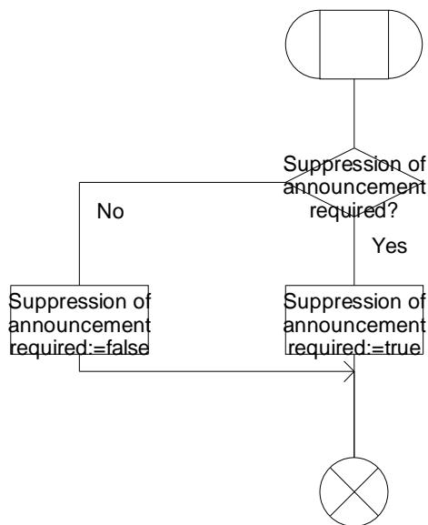
Figure 4.64-1: Procedure CAMEL\_SET\_SOA (sheet 1)
