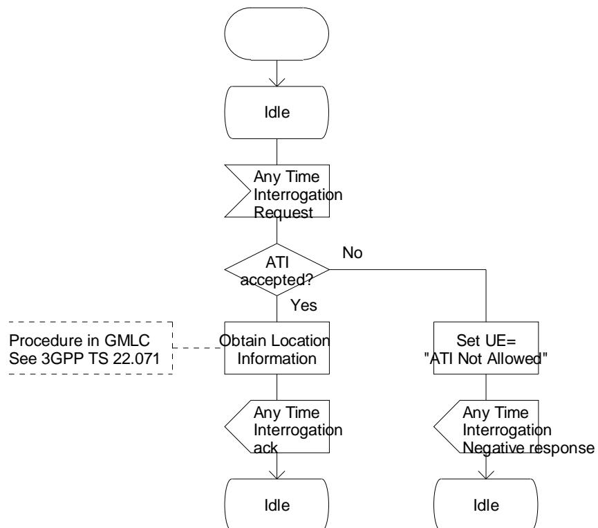
Figure 11.2-1: Process CAMEL\_ATI\_GMLC (sheet 1)
