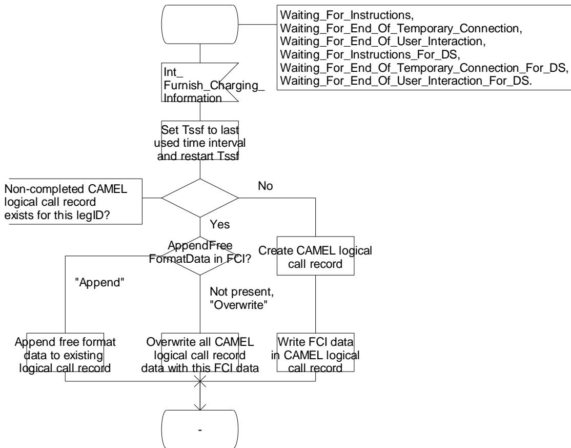
Figure 4.99-49: Process CS\_gsmSSF (sheet 49)
