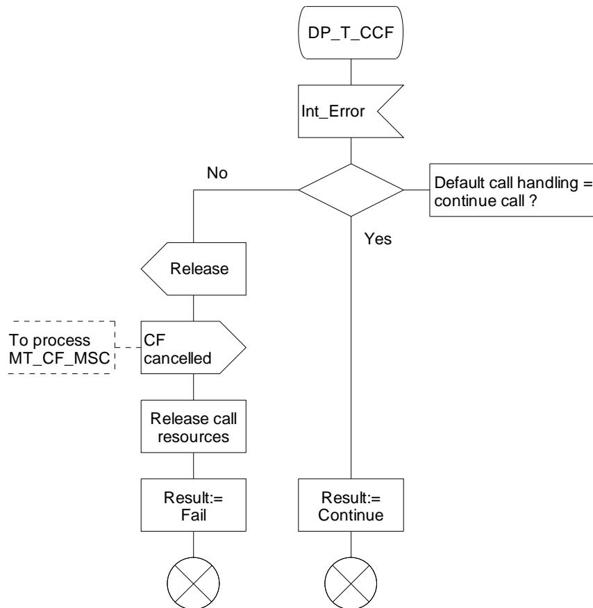
Figure 4.70-2: Procedure CAMEL\_MT\_VMSC\_Notify\_CF (sheet 2)
