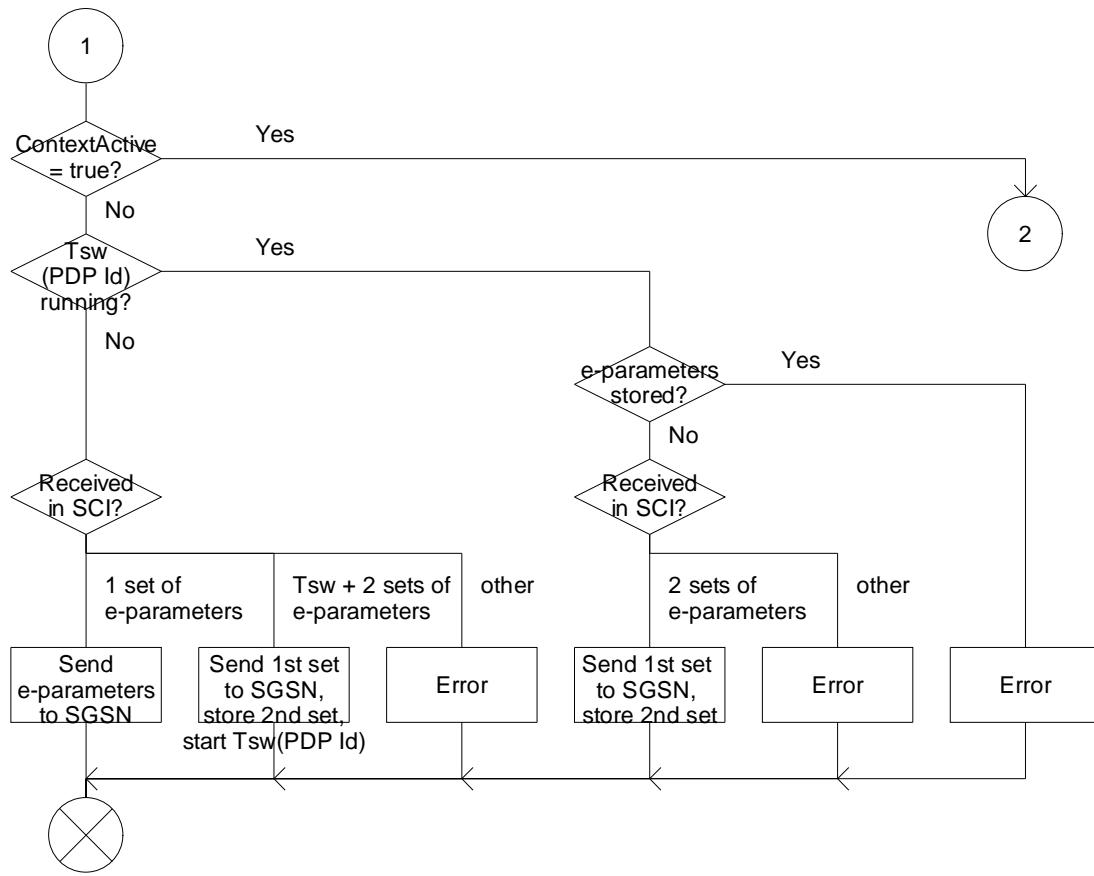
**Figure 6.23-2: Procedure Handle\_SCI\_GPRS (sheet 2)**
