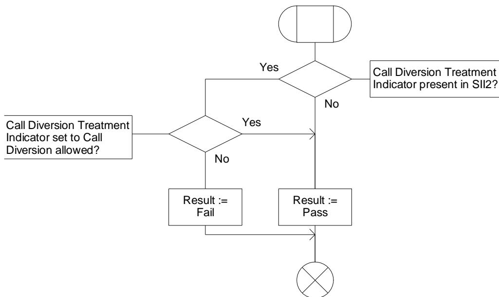
**Figure 4.63-1: Procedure CAMEL\_CHECK\_SII2\_CDTI (sheet 1)**
