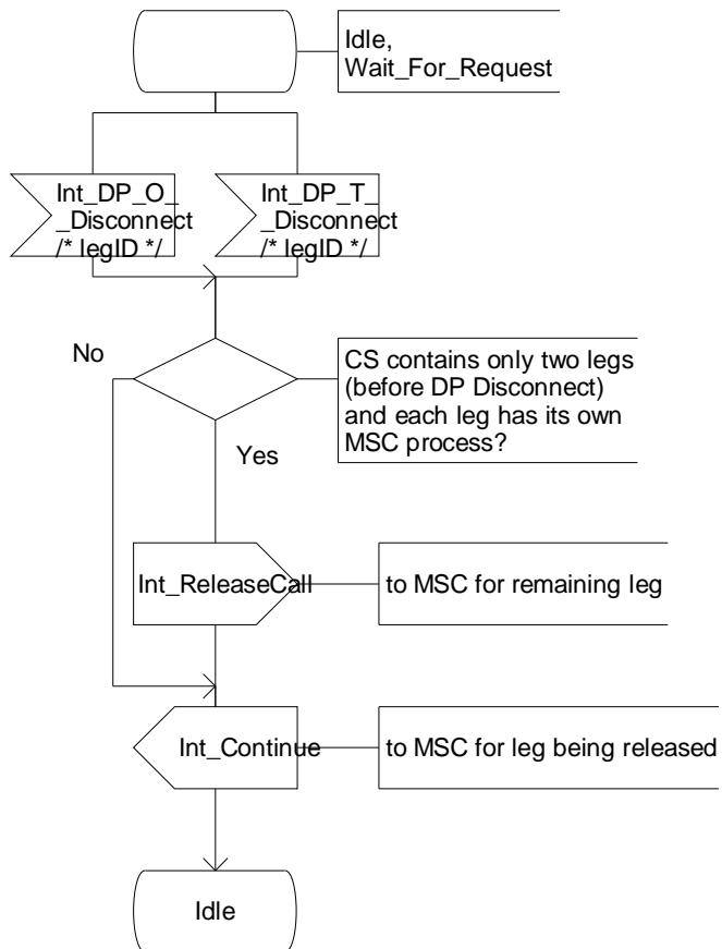
Figure 4.99-9: Process CS\_gsmSSF (sheet 9)
