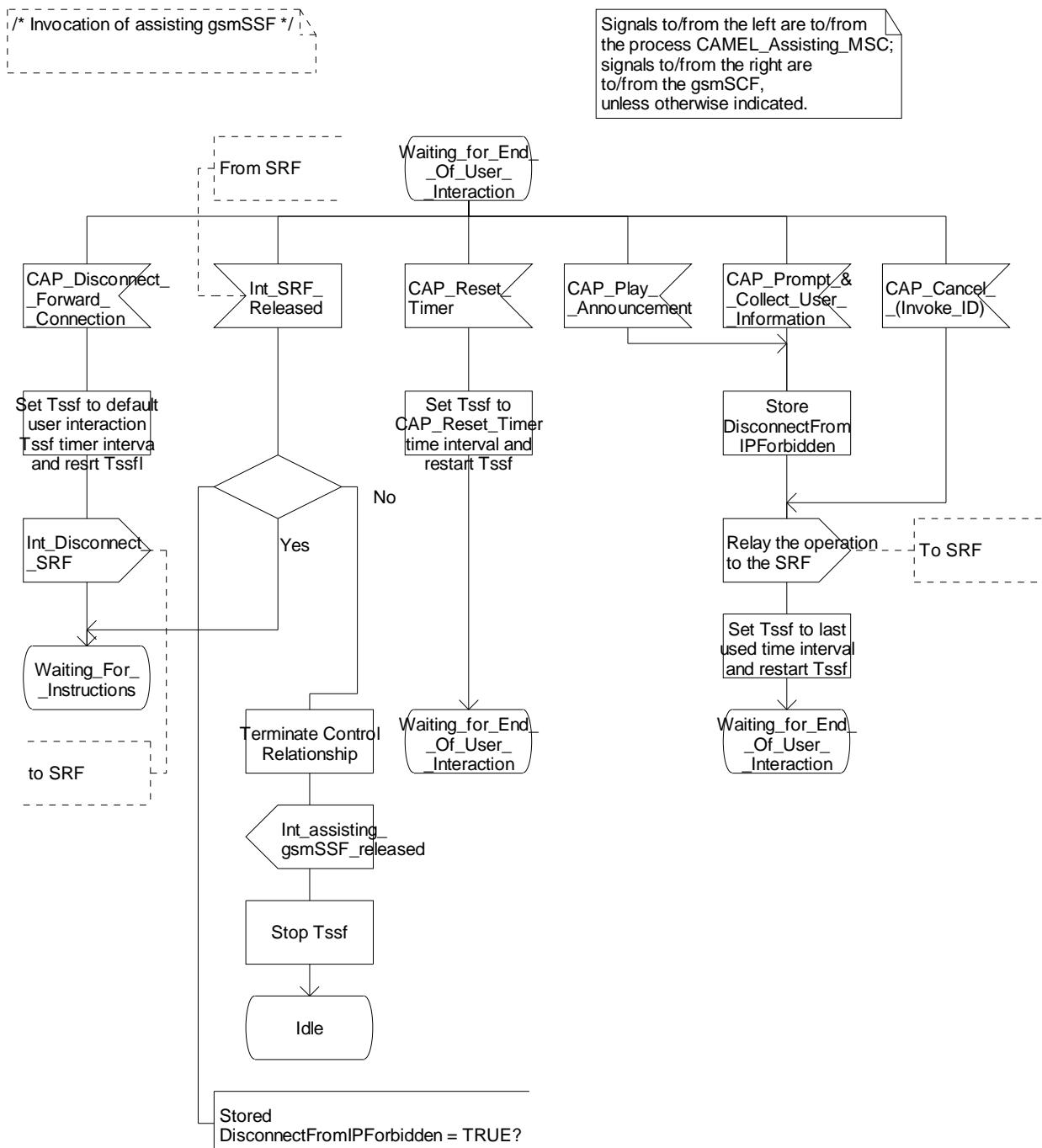
Figure 4.118-3: Process Assisting\_gsmSSF (sheet 3)
