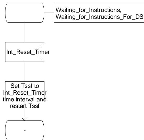
Figure 4.99-24: Process CS\_gsmSSF (sheet 24)
