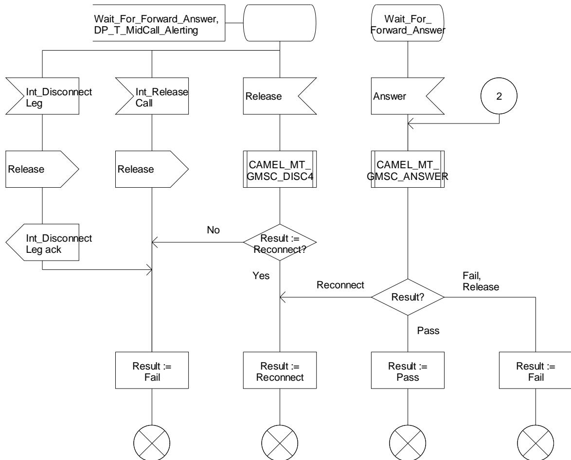
Figure 4.74-4: Procedure CAMEL\_ICH\_RECONNECT\_MSC (sheet 4)
