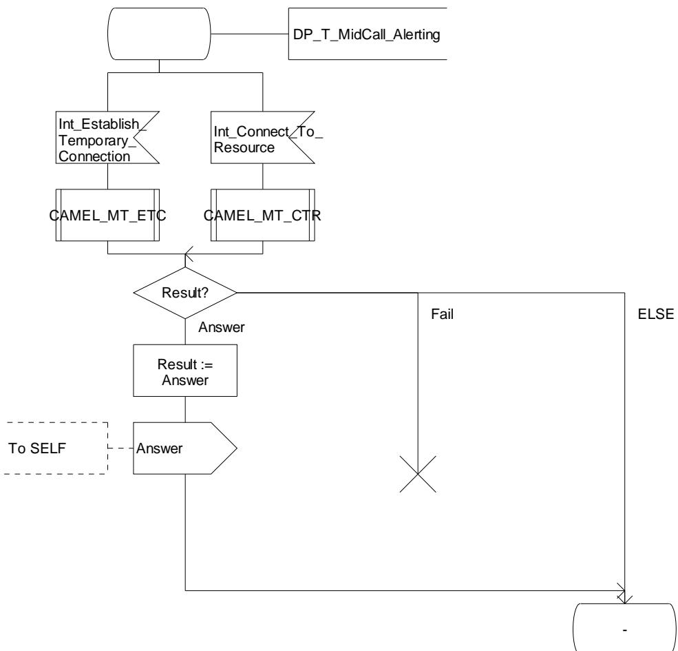
Figure 4.55-4: Process CAMEL\_MT\_LEG1\_GMSC (sheet 4)
