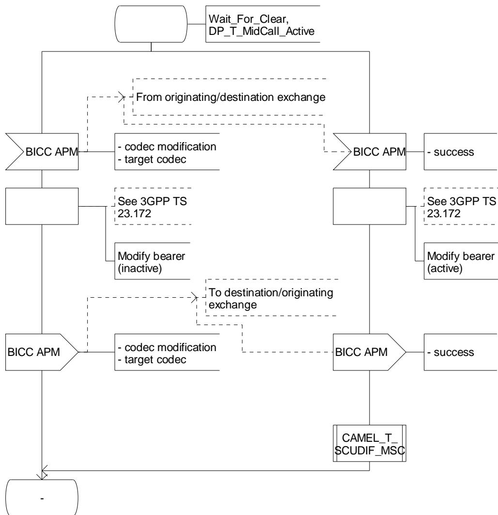
Figure 4.54-3: Procedure CAMEL\_MT\_LEG2\_GMSC (sheet 3)
