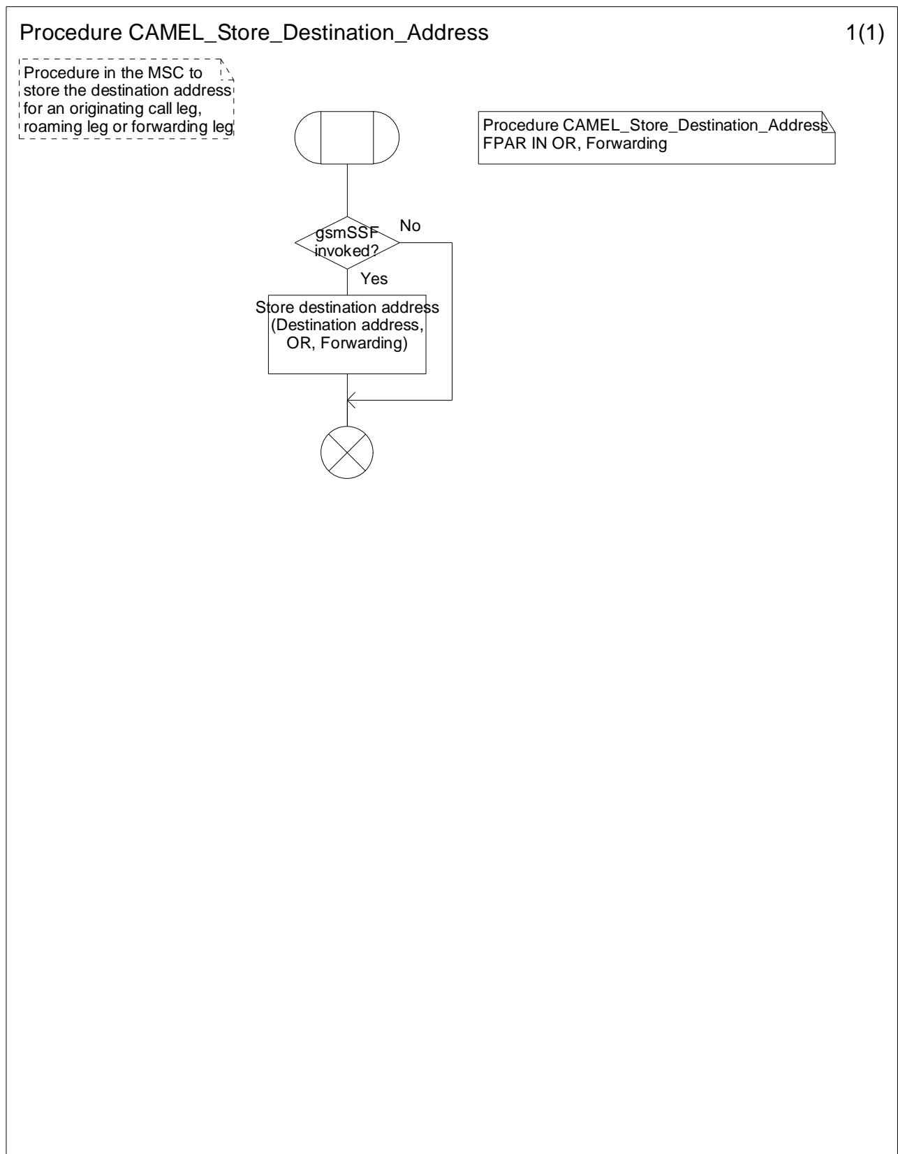
Figure 4.27-1: Procedure CAMEL\_Store\_Destination\_Address (sheet 1)
