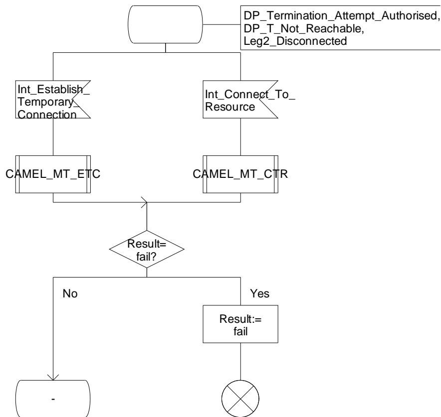
Figure 4.69-5: Procedure CAMEL\_ICH\_MSC\_INIT (sheet 5)
