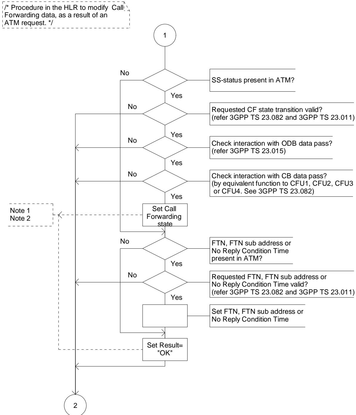
Figure 10.6-2: Procedure ATM\_Modify\_CF\_Data (sheet 2)
