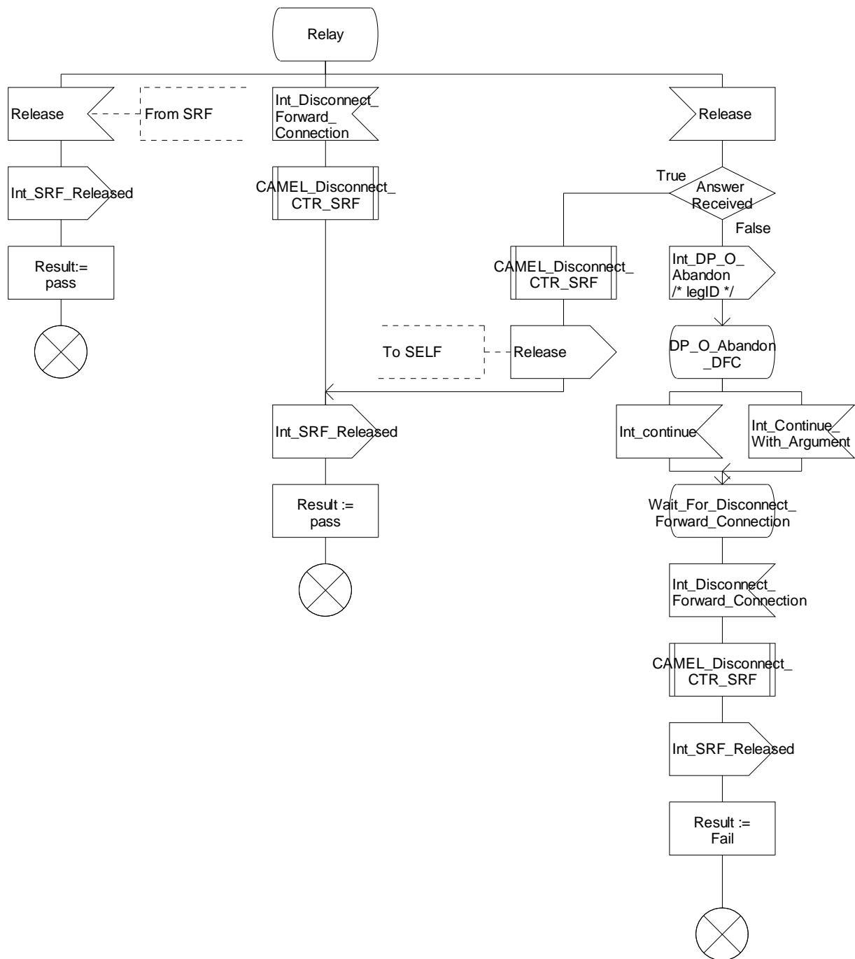
Figure 4.85-2: Procedure CAMEL\_CF\_CTR (sheet 2)
