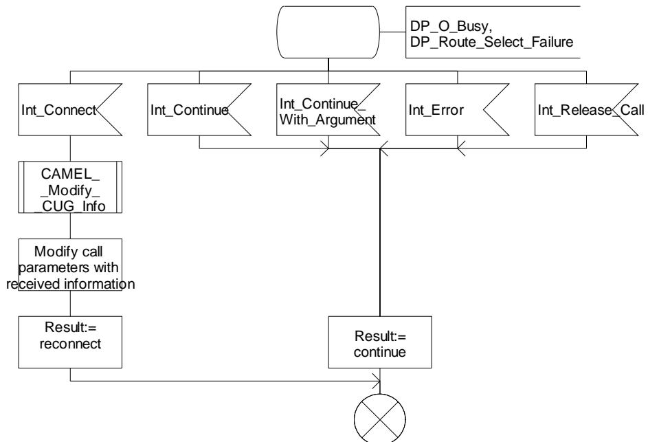
Figure 4.16-2: Procedure CAMEL\_OCH\_MSC1 (sheet 2)
