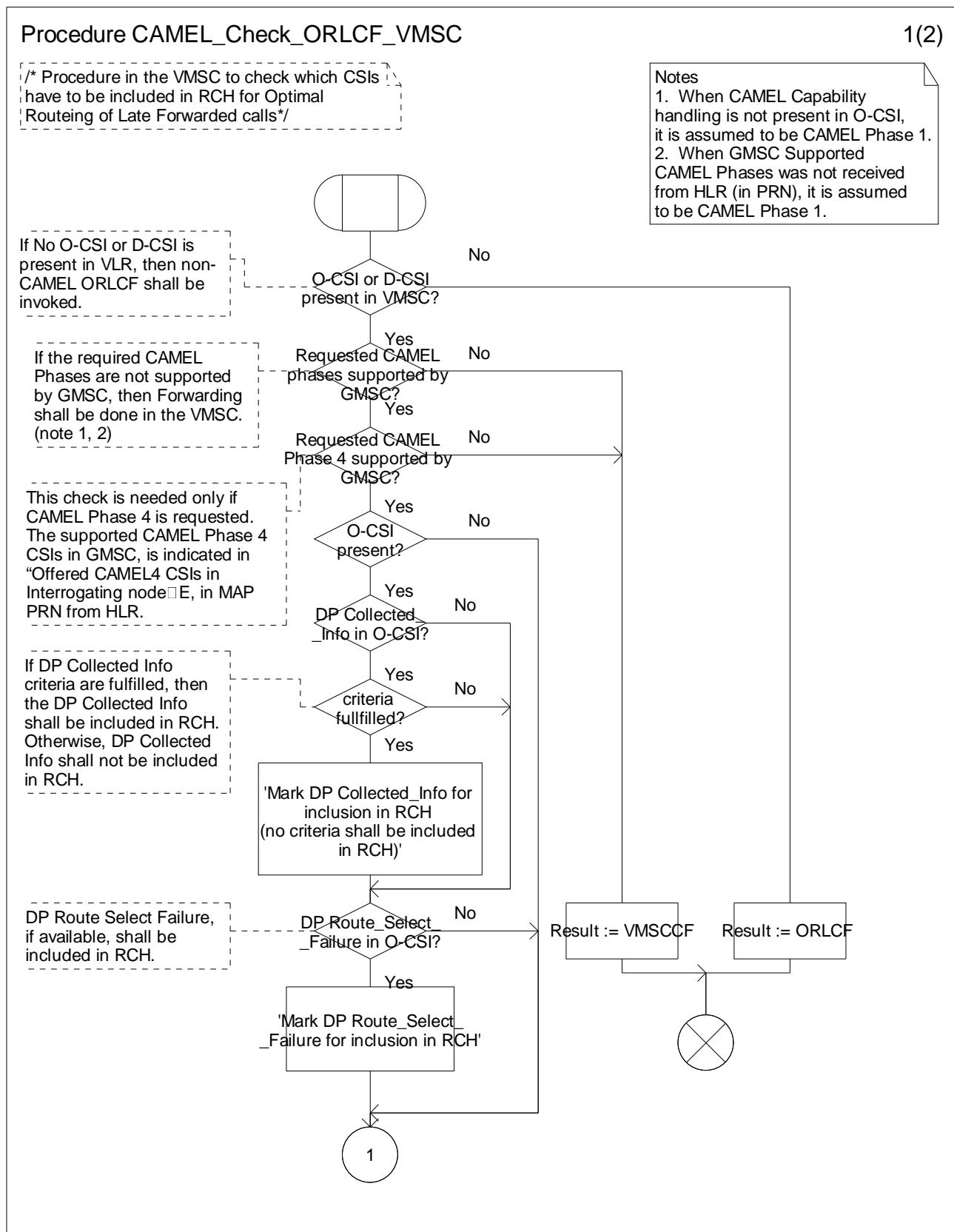
Figure 4.77-1: Procedure CAMEL\_Check\_ORLCF\_VMSC (sheet 1)
