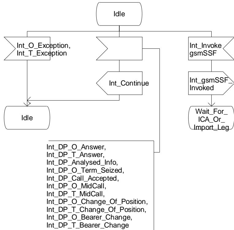
Figure 4.99-4: Process CS\_gsmSSF (sheet 4)
