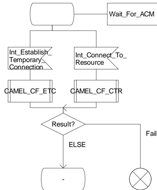
Figure 4.86-6: Procedure CAMEL\_MT\_CF\_LEG1\_MSC (sheet 6)
