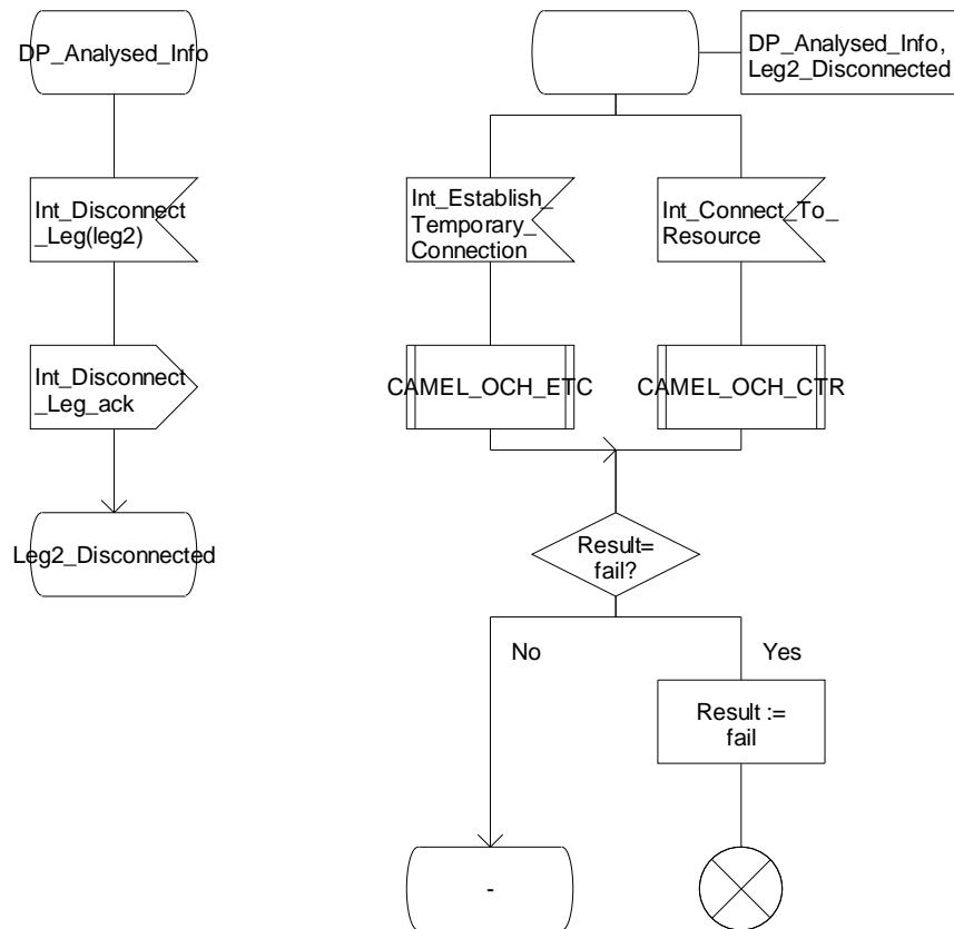
Figure 4.12-3: Procedure CAMEL\_SDS\_MO\_INIT (sheet 3)
