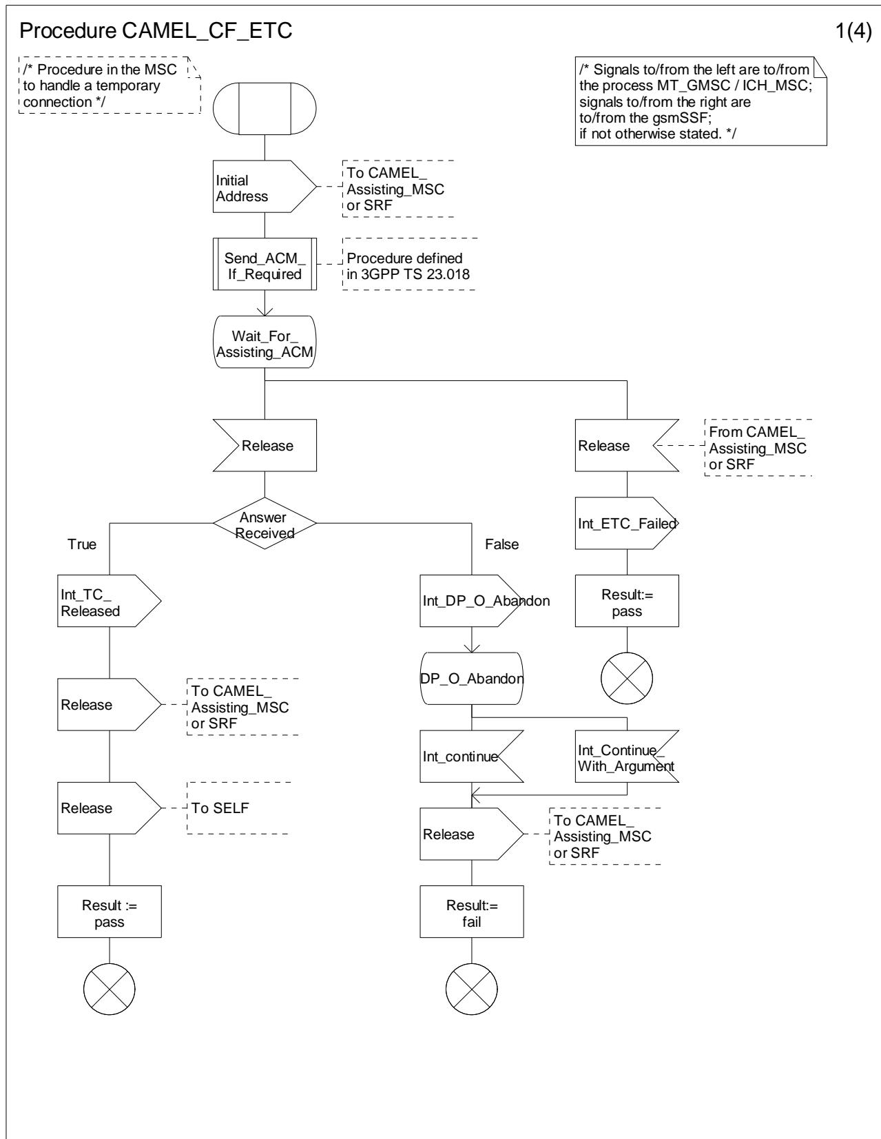
Figure 4.84-1: Procedure CAMEL\_CF\_etc (sheet 1)
