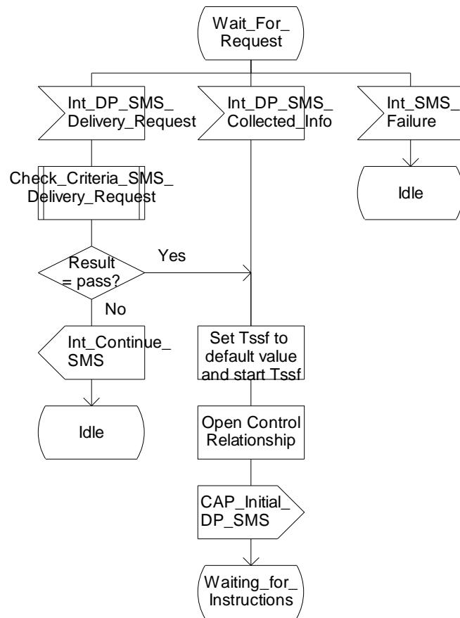
Figure 7.15-2: Process SMS\_SSF (sheet 2)
