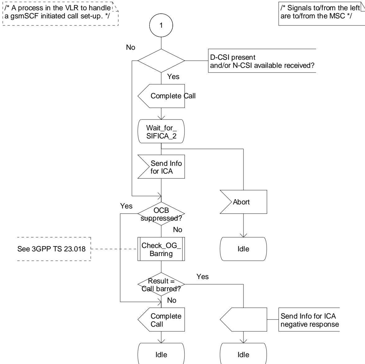
Figure 4.95-2: Process CAMEL\_ICA\_VLR (sheet 2)
