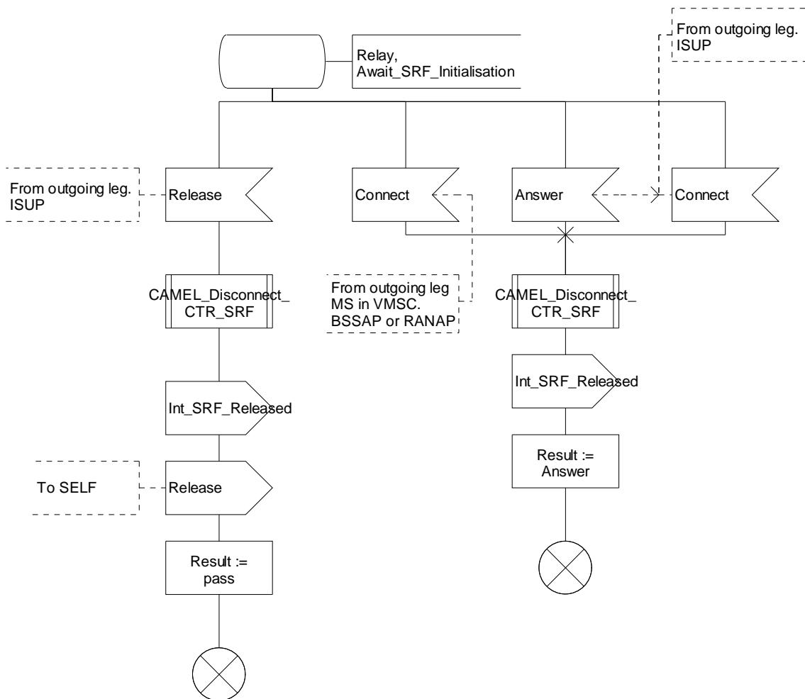
Figure 4.52-5: Procedure CAMEL\_MT\_CTR (sheet 5)
