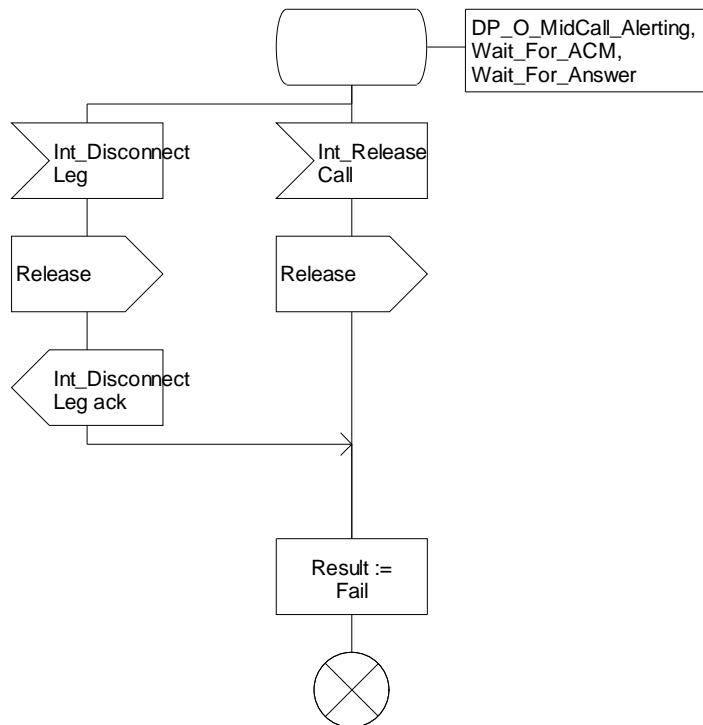
Figure 4.33-6: Procedure CAMEL\_OCH\_RECONNECT\_MSC (sheet 6)
