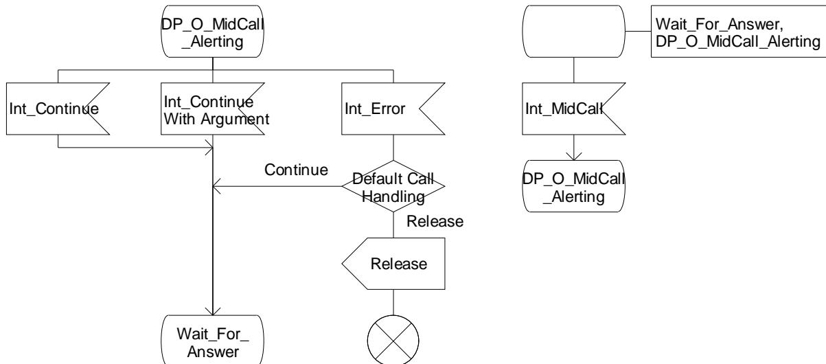
Figure 4.86-3: Procedure CAMEL\_MT\_CF\_LEG1\_MSC (sheet 3)
