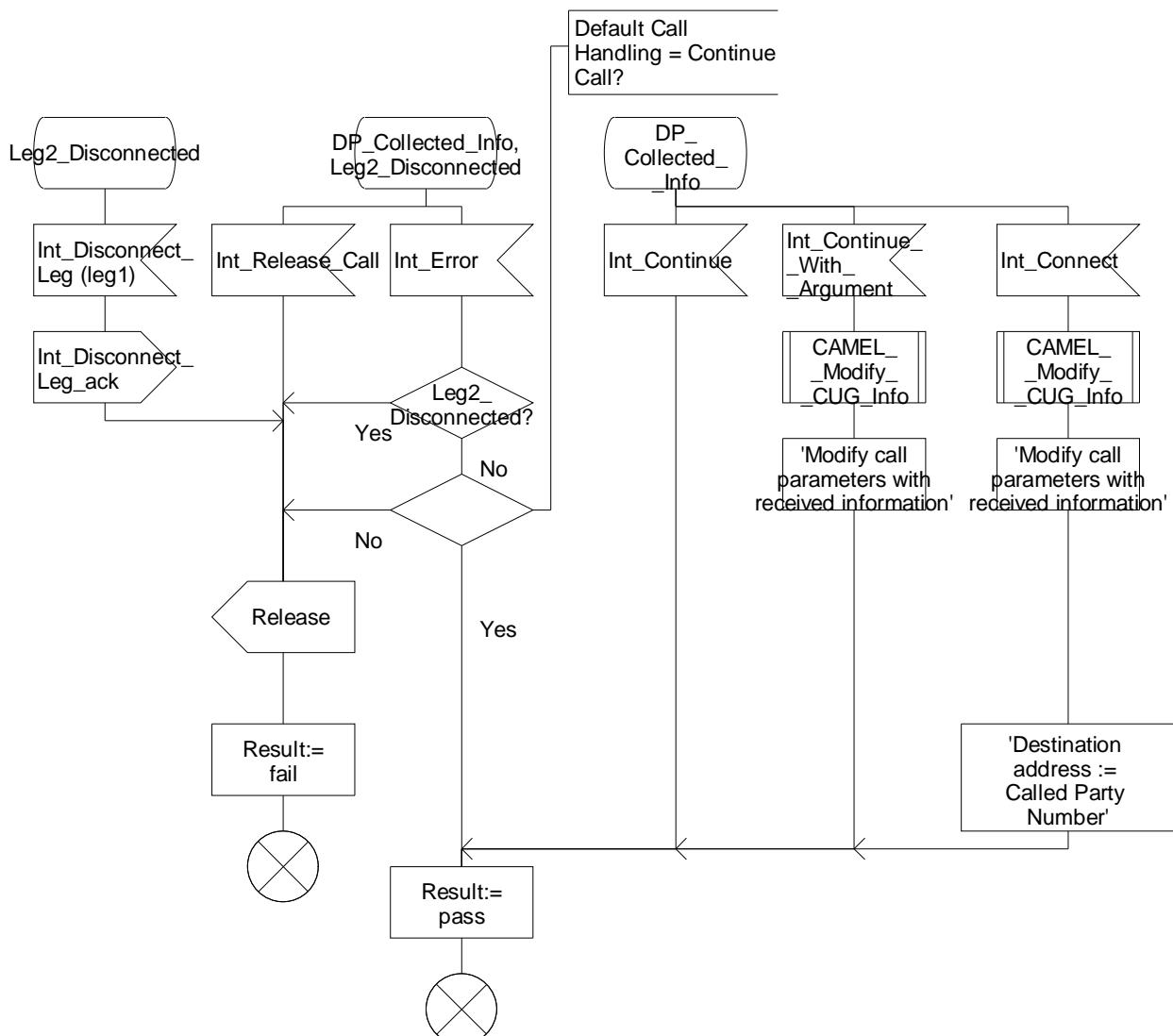
Figure 4.79-2: Procedure CAMEL\_CF\_MSC\_INIT (sheet 2)
