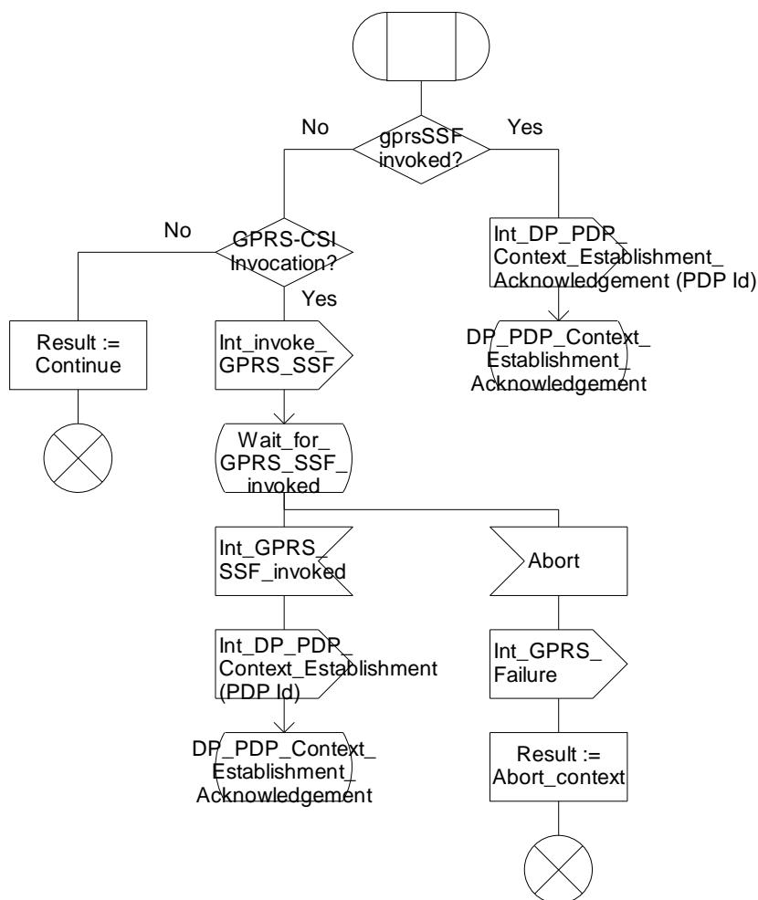
**Figure 6.13-1: Procedure CAMEL\_GPRS\_PDP\_Context\_Establishment\_Acknowledgement (sheet 1)**
