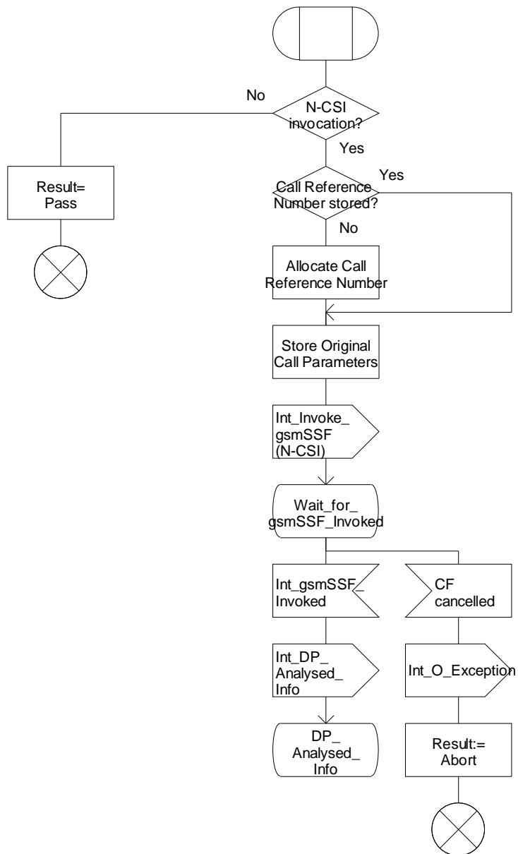
Figure 4.81-1: Procedure CAMEL\_NDS\_CF\_INIT (sheet 1)
