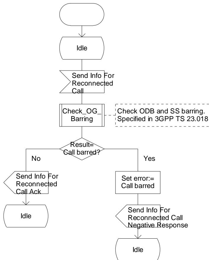
Figure 4.40-1: Process CAMEL\_Reconnected\_Call\_VLR (sheet 1)
