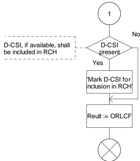
Figure 4.77-2: Procedure CAMEL\_Check\_ORLCF\_VMSC (sheet 2)
