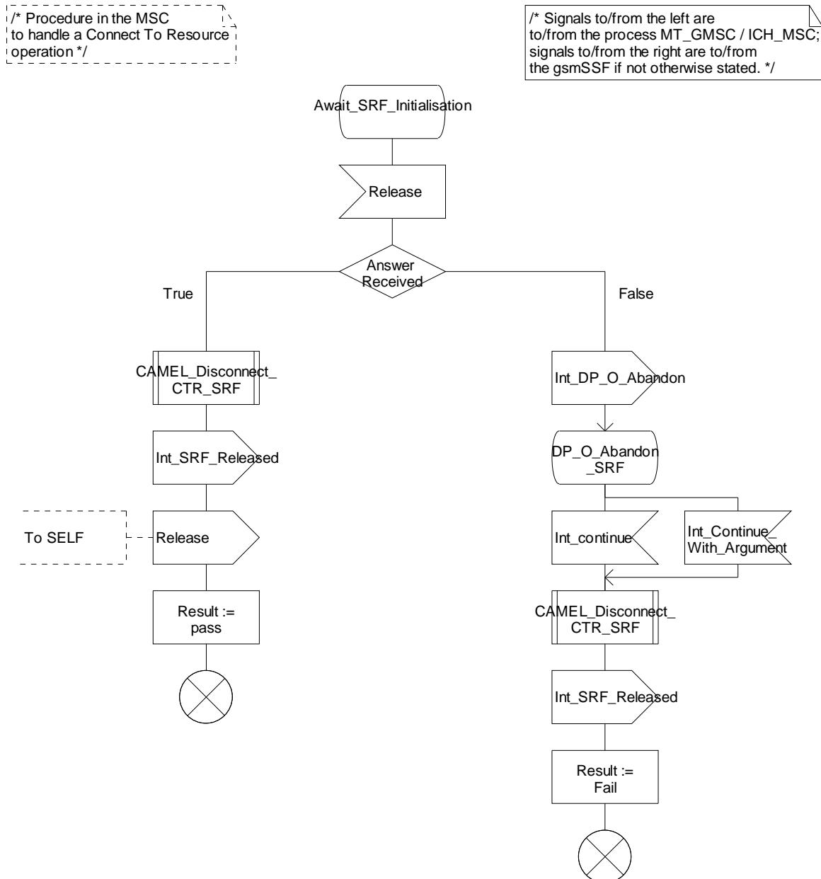
Figure 4.85-4: Procedure CAMEL\_CF\_CTR (sheet 4)
