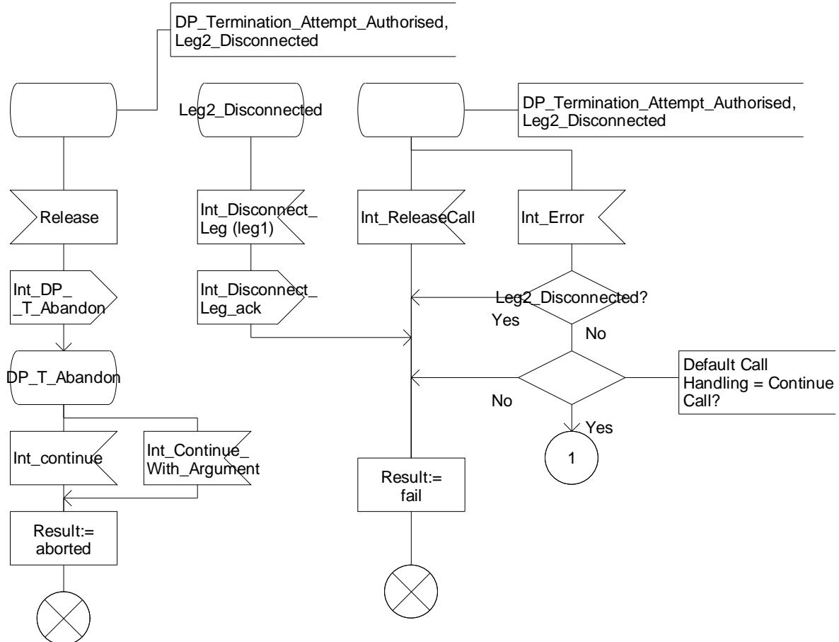
Figure 4.42-4: Procedure CAMEL\_MT\_GMSC\_INIT (sheet 4)
