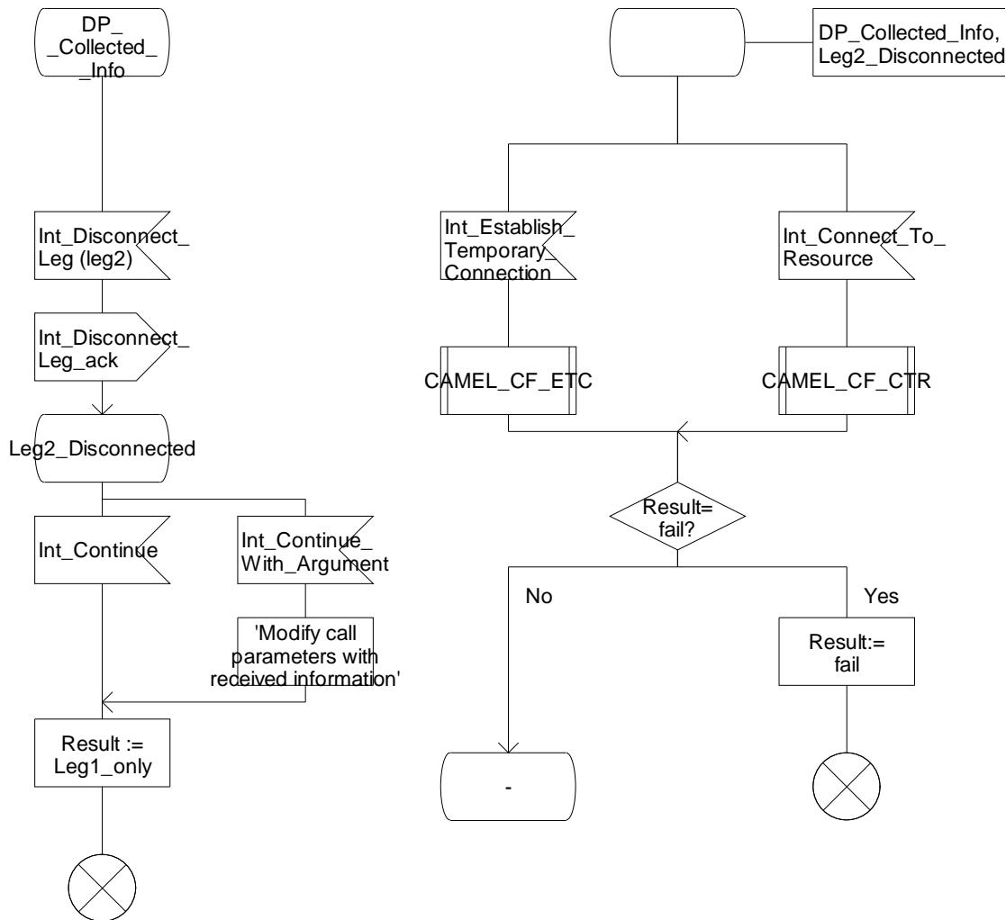
Figure 4.79-3: Procedure CAMEL\_CF\_MSC\_INIT (sheet 3)
