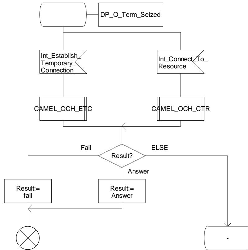
Figure 4.14-3: Procedure CAMEL\_OCH\_MSC\_ALERTING (sheet 3)
