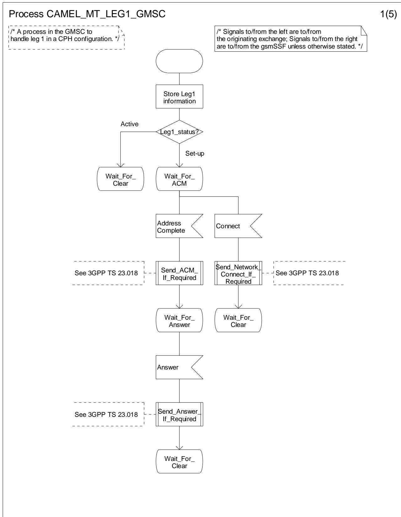
Figure 4.55-1: Process CAMEL\_MT\_LEG1\_GMSC (sheet 1)
