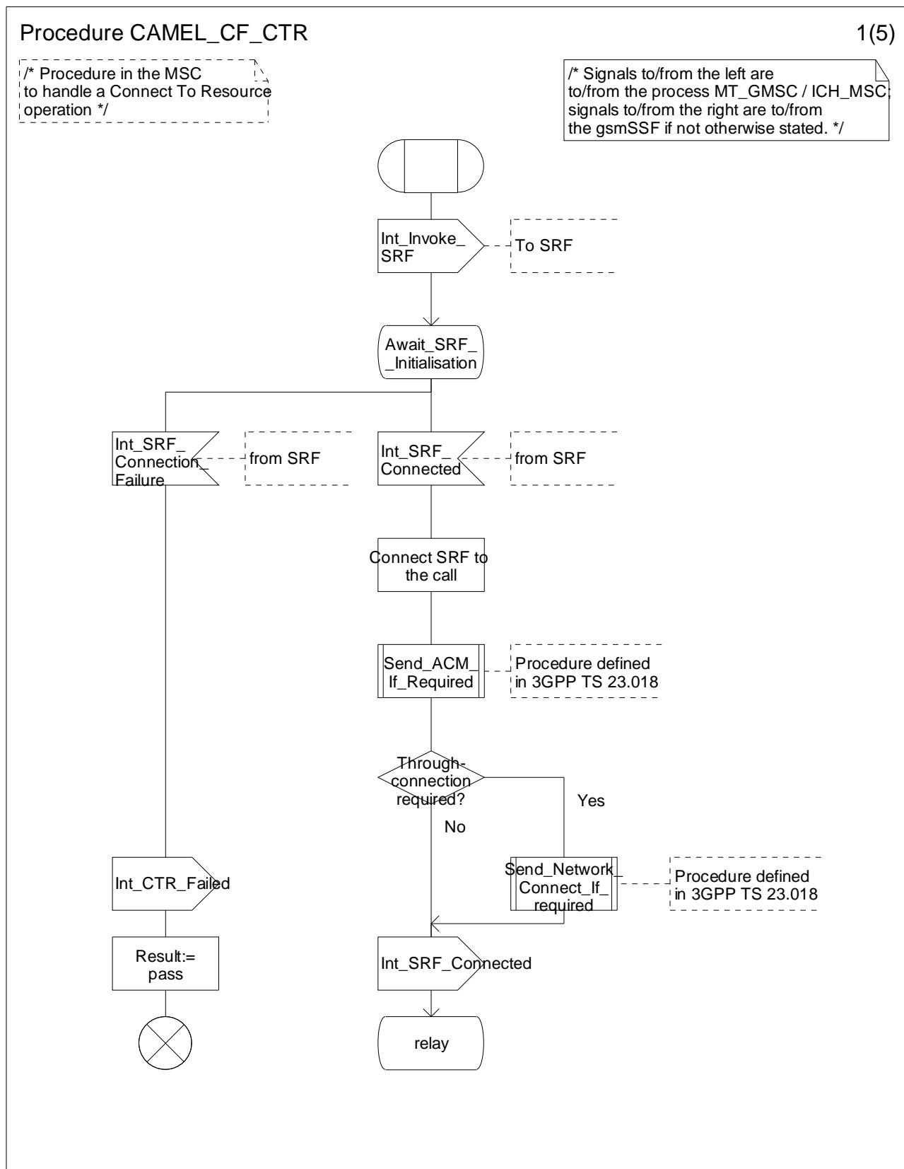
Figure 4.85-1: Procedure CAMEL\_CF\_CTR (sheet 1)
