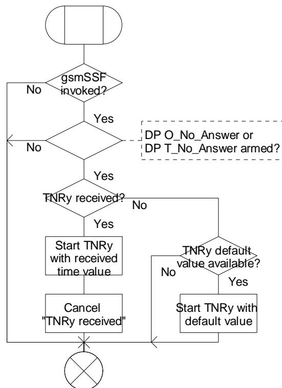
**Figure 4.25-1: Procedure CAMEL\_Start\_TNRy (sheet 1)**
