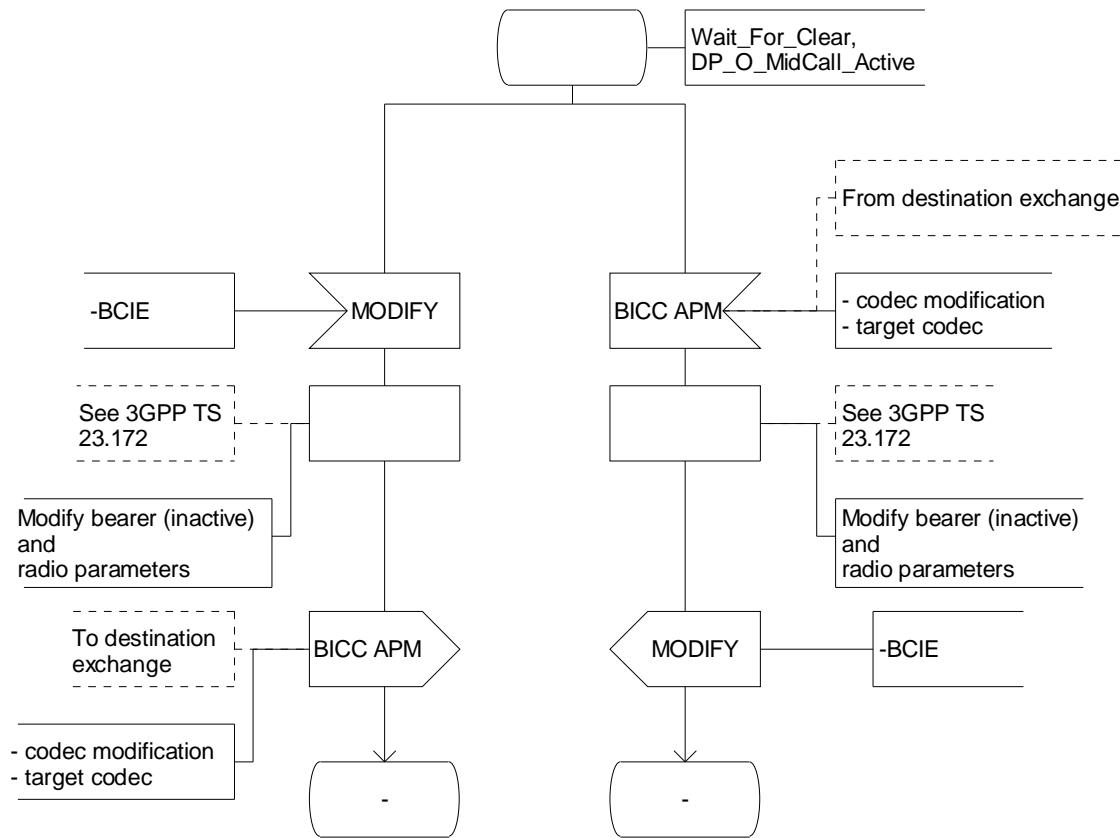
Figure 4.30-7: Procedure CAMEL\_OCH\_LEG1\_MSC (sheet 7)
