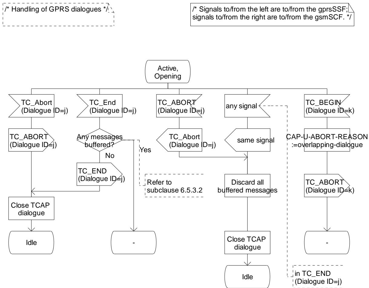
Figure 6.18-2: Process GPRS\_Dialogue\_Handler (sheet 2)
