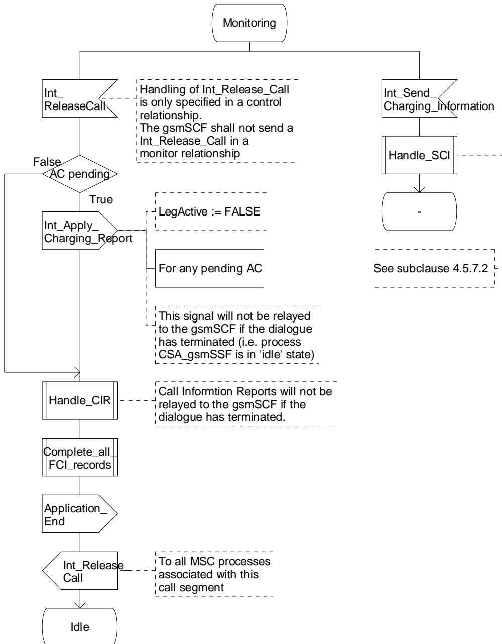
Figure 4.99-34: Process CS\_gsmSSF (sheet 34)
