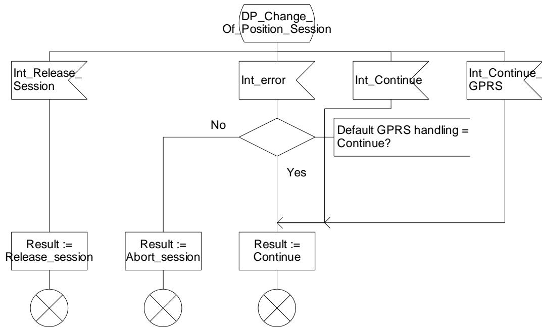
Figure 6.10-2: Procedure CAMEL\_GPRS\_Routeing\_Area\_Update\_Session (sheet 2)
