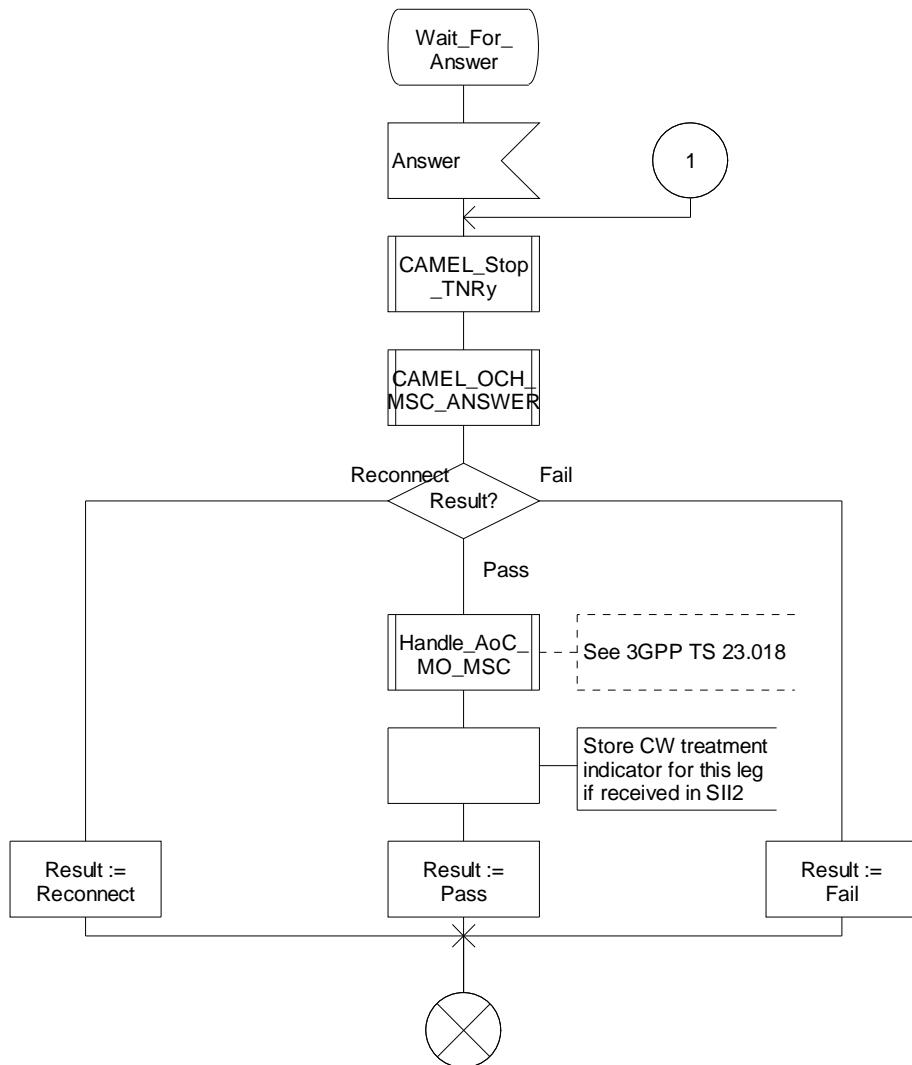
Figure 4.33-4: Procedure CAMEL\_OCH\_RECONNECT\_MSC (sheet 4)
