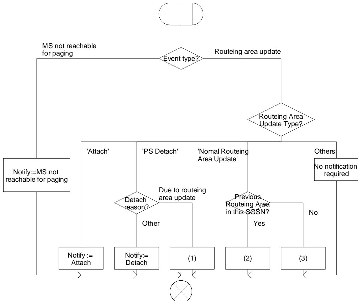
**Figure 9.6-1: Procedure Set\_PS\_Notification\_Type (sheet 1)**
