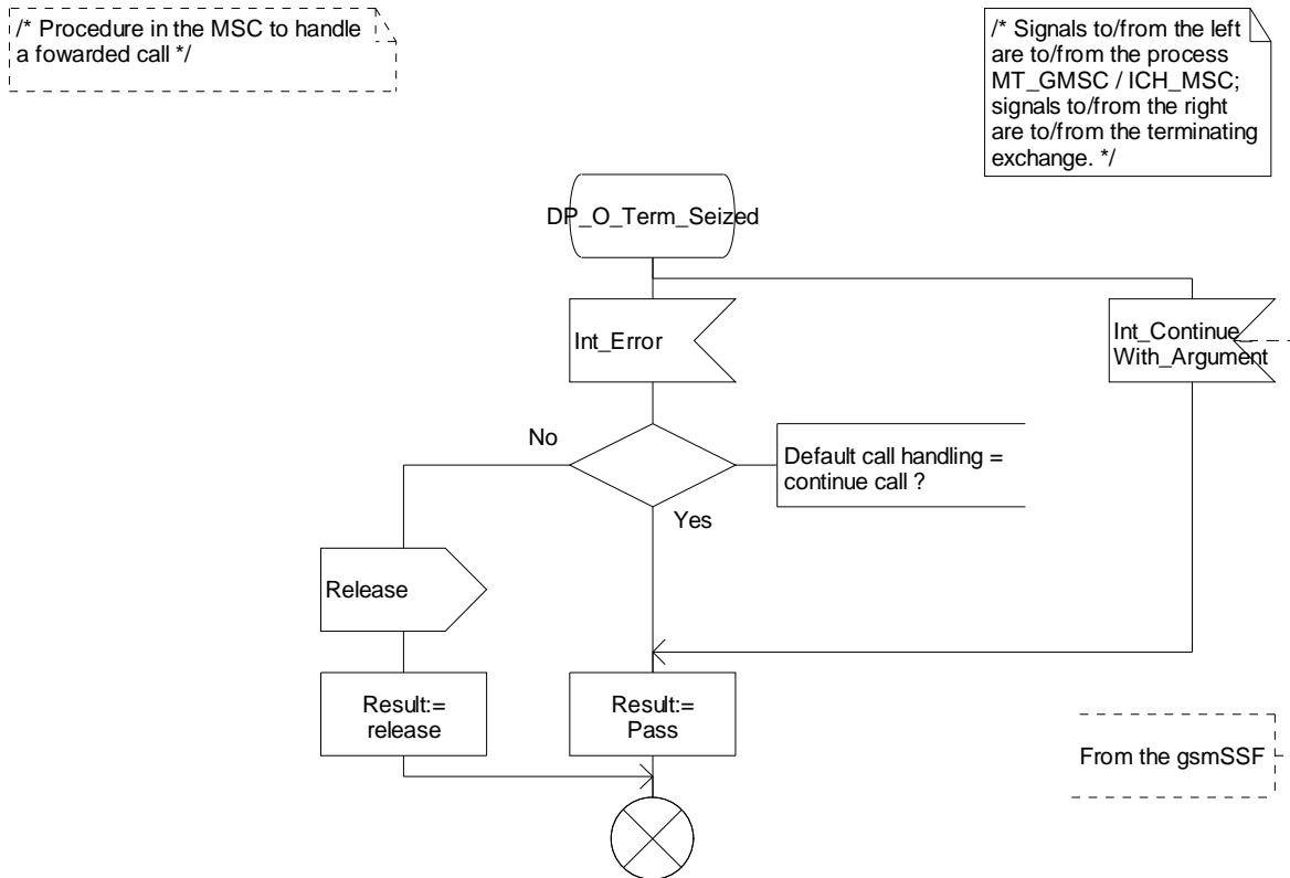
Figure 4.82-2: Procedure CAMEL\_CF\_MSC\_ALERTING (sheet 2)
