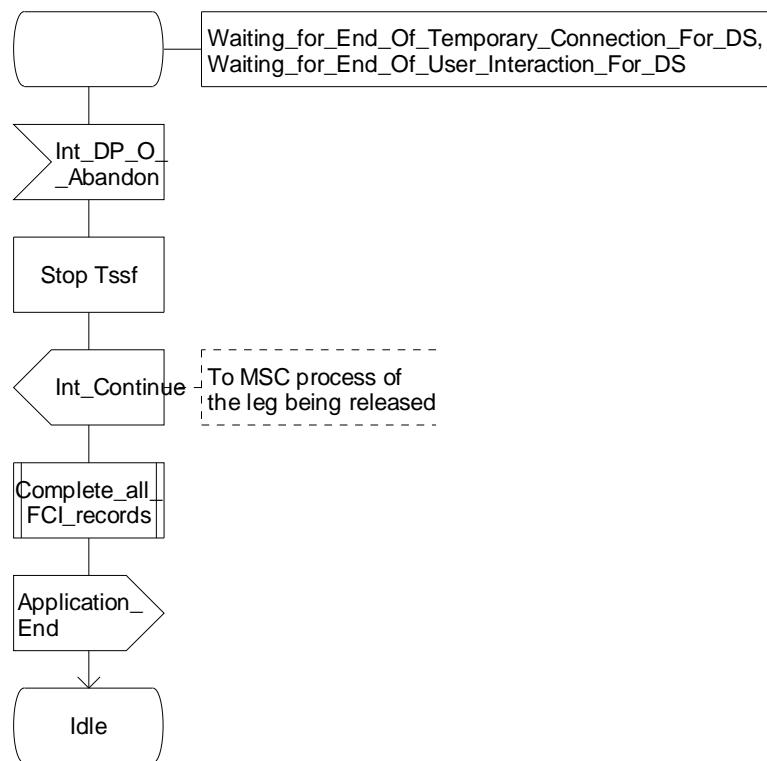
Figure 4.99-61: Process CS\_gsmSSF (sheet 61)
