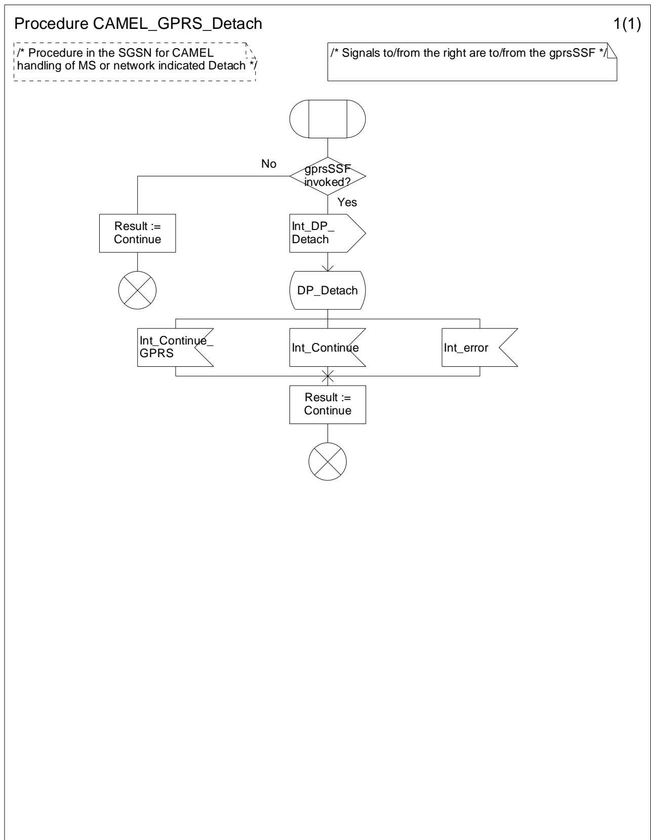
Figure 6.9-1: Procedure CAMEL\_GPRS\_Detach (sheet 1)
