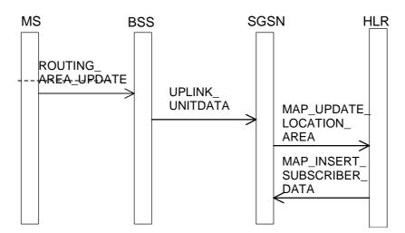
Figure 3: Signalling information required at routing area update
