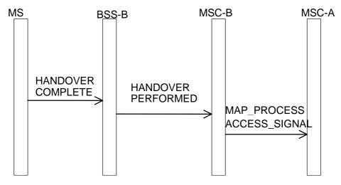
Figure 8: Signalling information required at BSS internal handover
