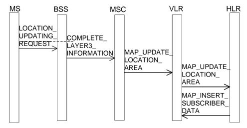
Figure 2: Signalling information required at location registration
