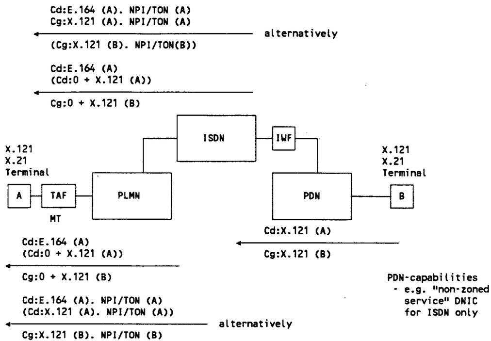
Figure 03.70/8: Interworking PDN-ISDN-PLMN (PDN "ISDN non-zoned service DNIC")
