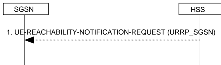
Figure 6.15-1: UE Reachability Notification Request Procedure
