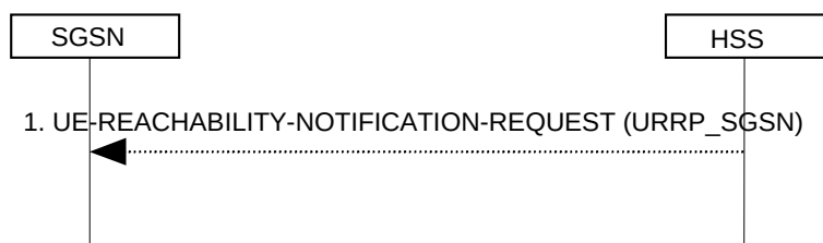
Figure 6.15-1: UE Reachability Notification Request Procedure
