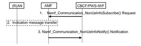
Figure 9A.2.3.2-1: Indication message transfer procedure
