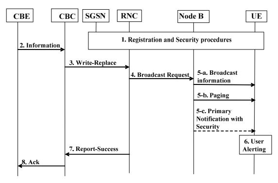
Figure 9.1.3.3-1: Warning message delivery procedure in UTRAN
