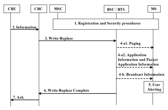
Figure 9.1.3.2-1: Warning message delivery procedure in GERAN
