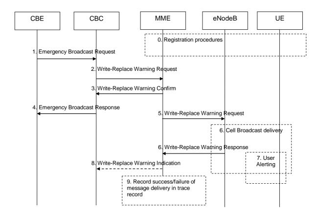
Figure 9.1.3.4.2-1: Warning message delivery procedure in E-UTRAN
