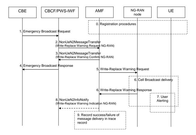
Figure 9.1.3.5.2-1: Warning message delivery procedure in NG-RAN
