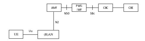
Figure B.1-1: 5GS PWS architecture with PWS-IWF
