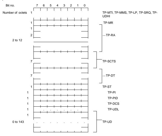
NOTE: Any unused bits shall be set to zero by the sending entity and shall be ignored by the receiving entity.
