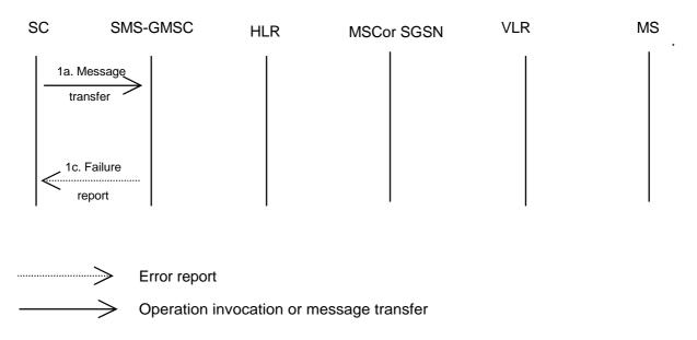
Figure 15b): Short message transfer attempt failing due to error at the SMS-GMSC
