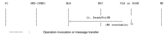
NOTE 1): In case ReadyForSM is sent by the SGSN, the reason may be MS reachable via the SGSN, or MS reachable via the SGSN and the MSC (see 3GPP TS 23.060 [27]).
