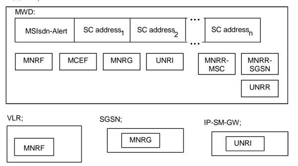
Figure 3: Example of how information on one MS can be put in relation to SC(s) in order to fulfil the requirement of Alert-SC mechanism
