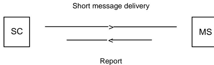
**Figure 1: The Short Message Service mobile terminated**
