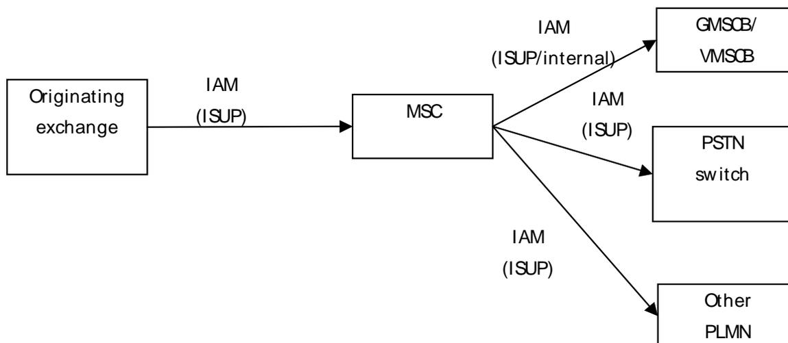
**Figure 4.3.1: Architecture for a basic trunk originated call**
