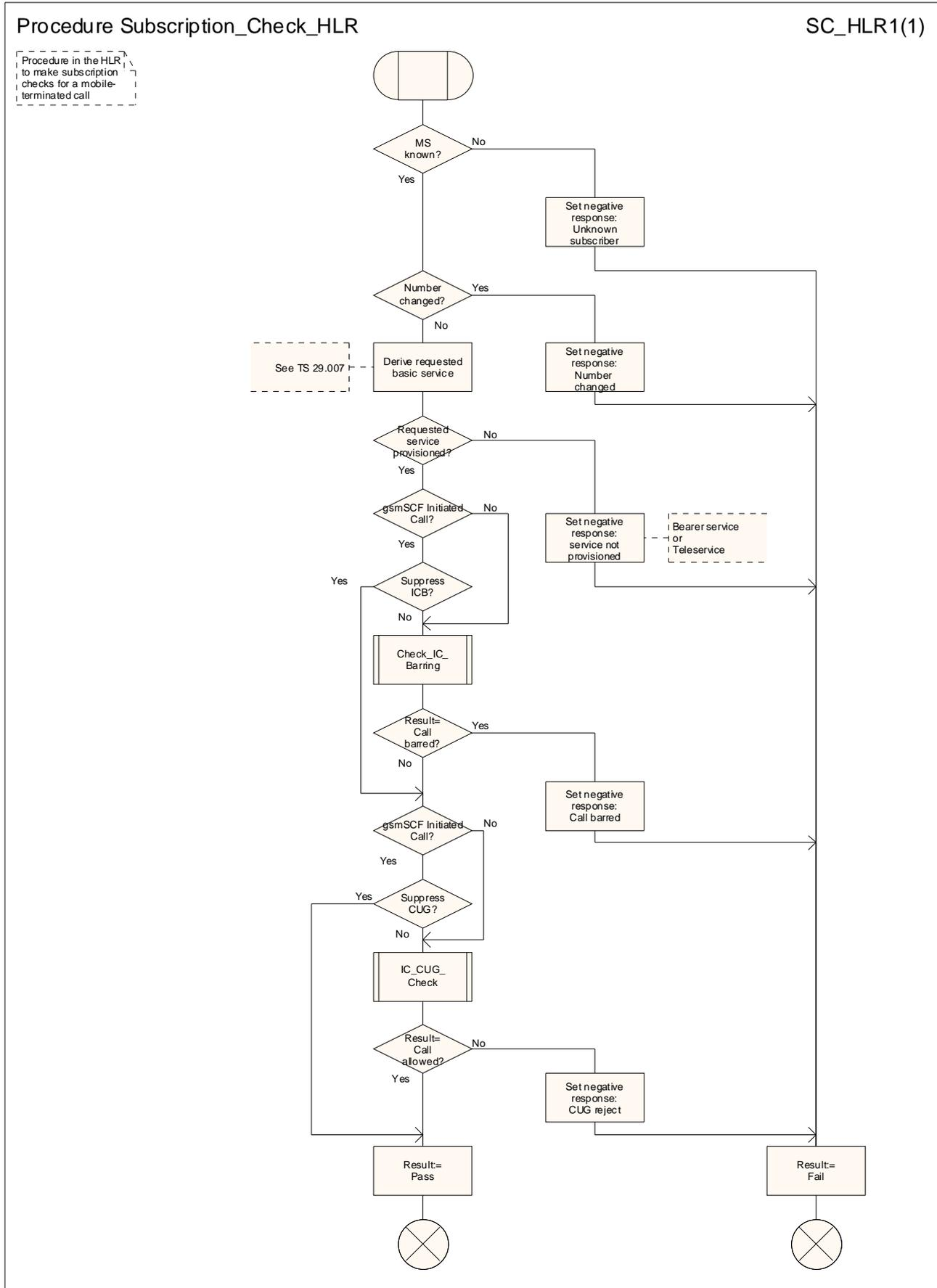
Figure 46: Procedure Subscription\_Check\_HLR
