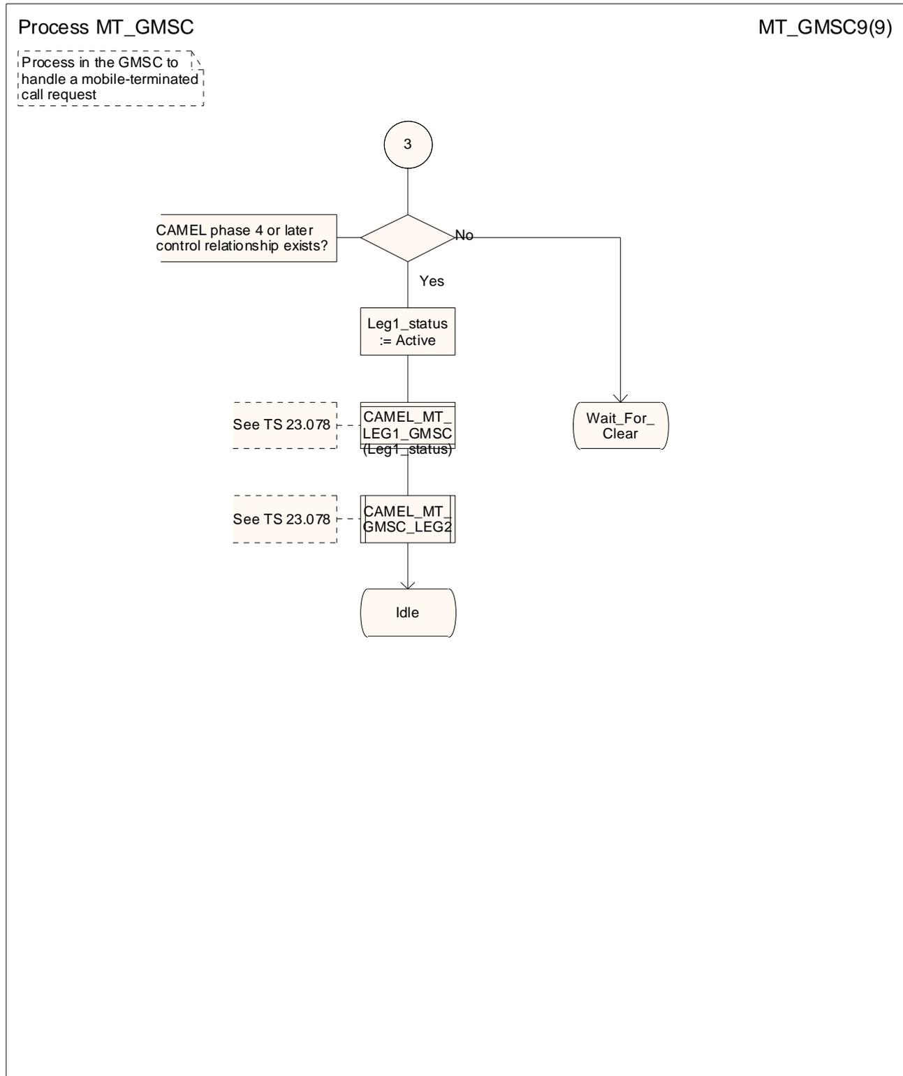
Figure 36i: Process MT\_GMSC (sheet 9)
