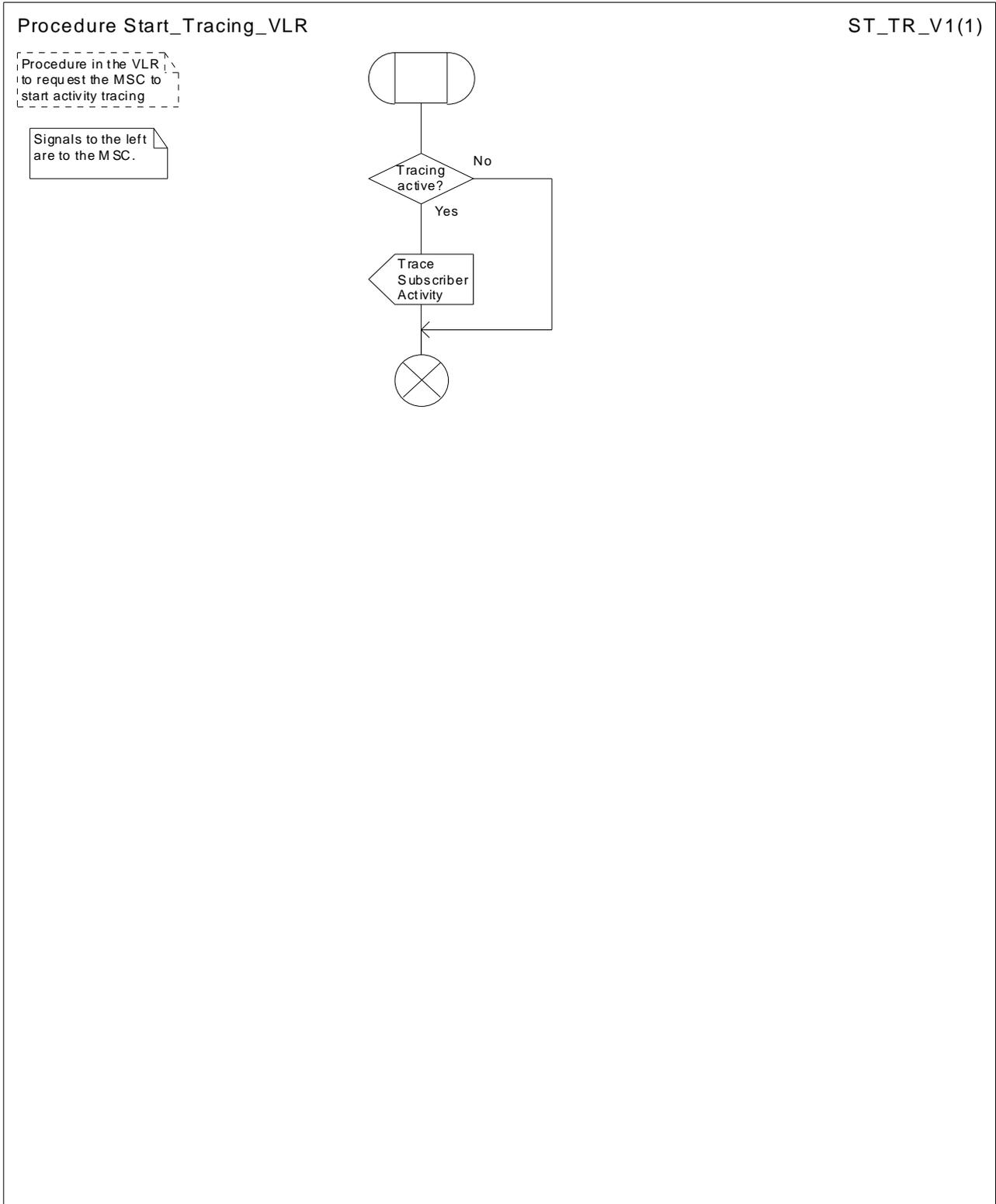
Figure 7.1.2.8: Procedure Start\_Tracing\_VLR
