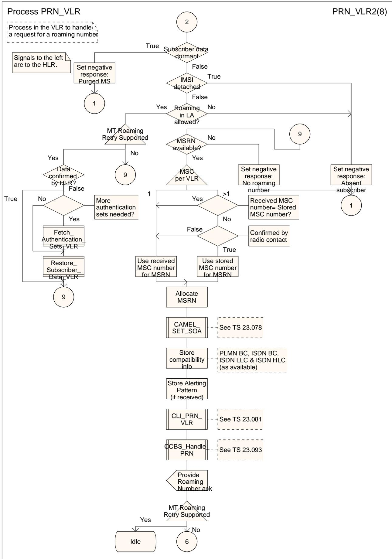
Figure 55b: Process PRN\_VLR (sheet 2)
