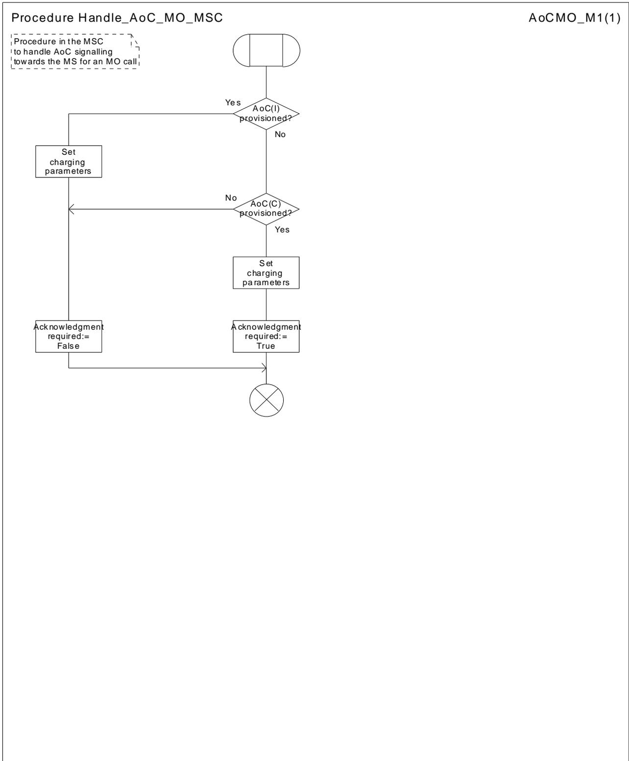
Figure 17: Procedure Handle\_AoC\_MO\_MSC
