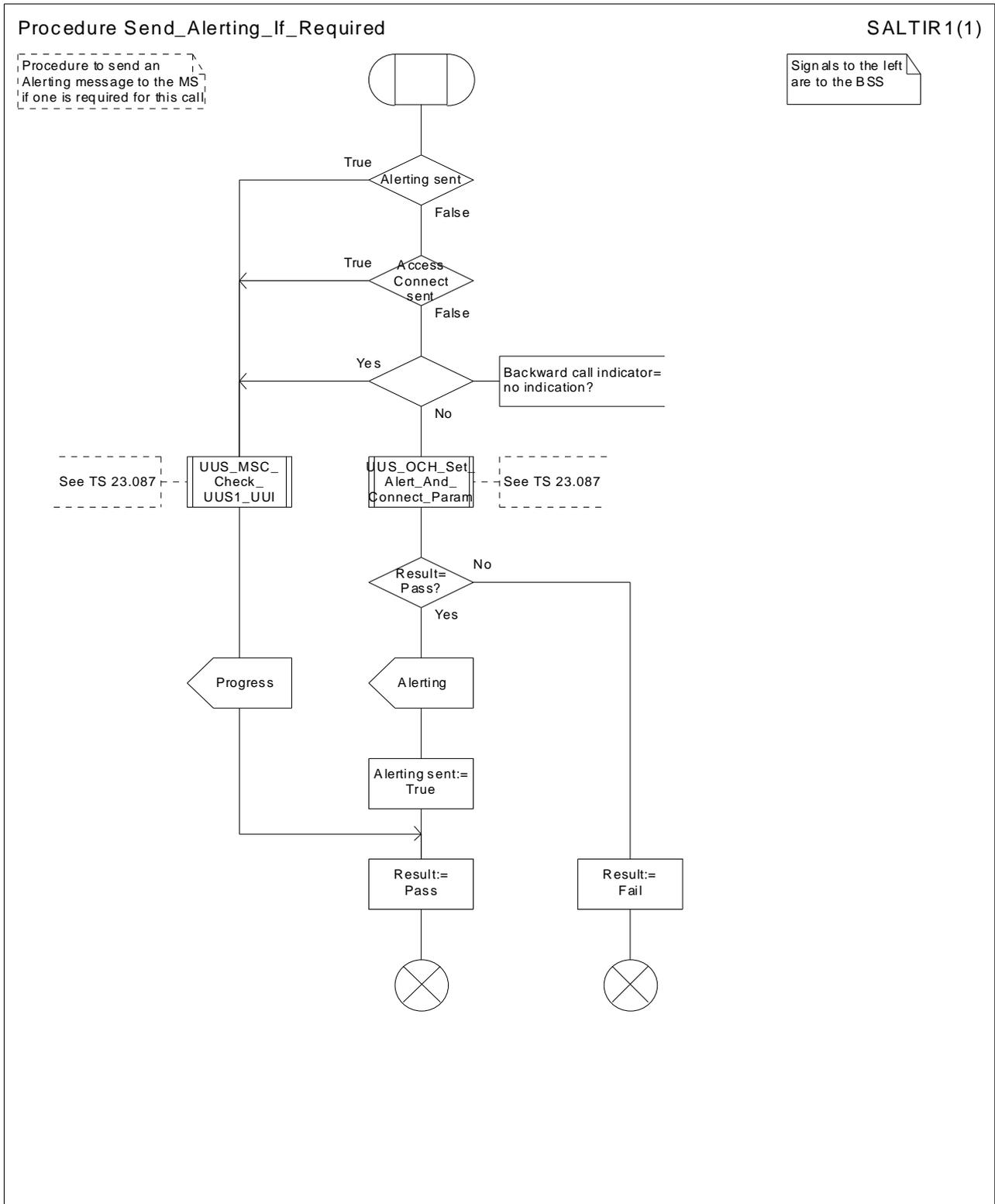
Figure 15: Procedure Send\_Alerting\_If\_Required
