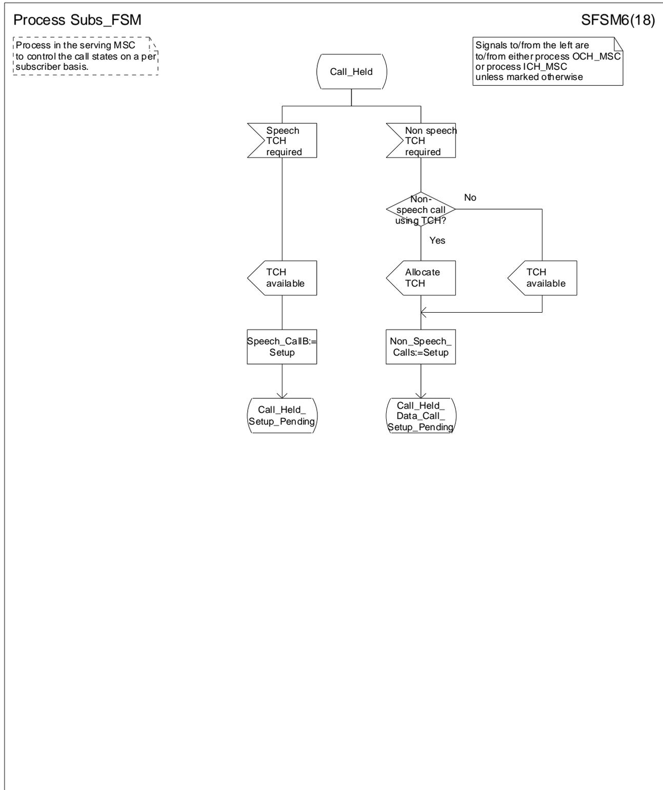
Figure 83f: Process Subs\_FSM (sheet 6)
