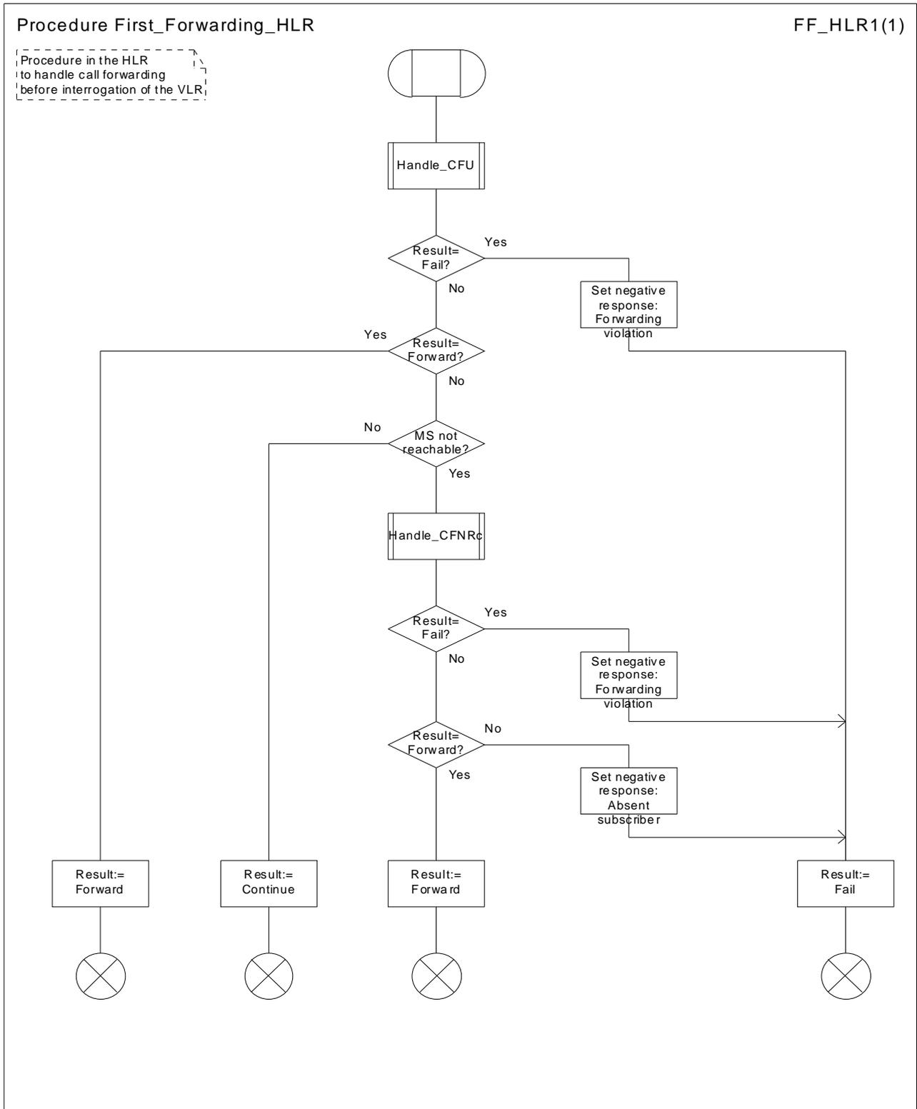
Figure 47: Procedure First\_Forwarding\_HLR
