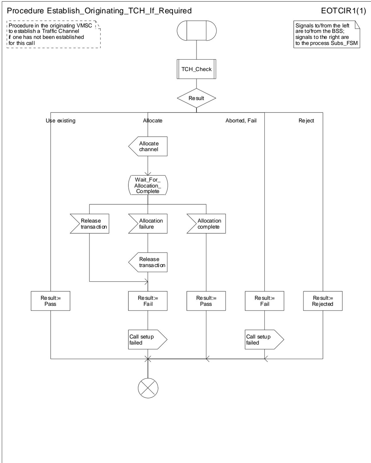
Figure 13: Procedure Establish\_Originating\_TCH\_If\_Required
