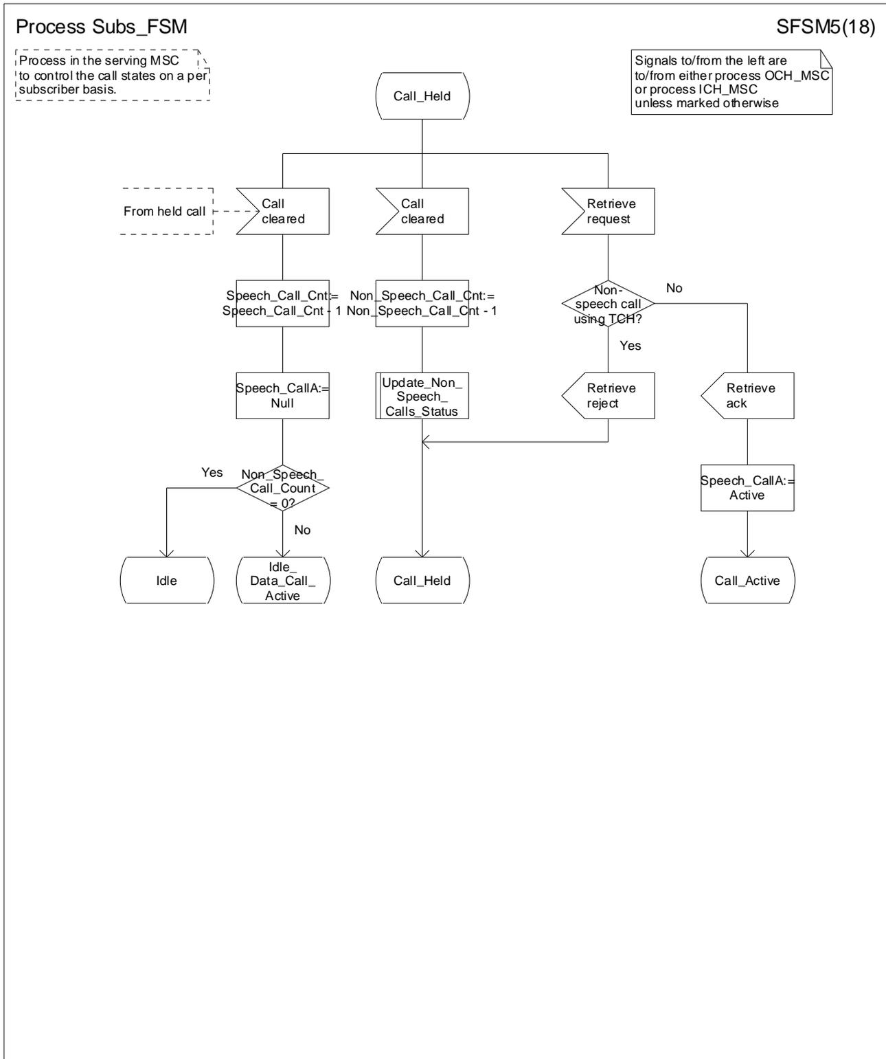
Figure 83e: Process Subs\_FSM (sheet 5)
