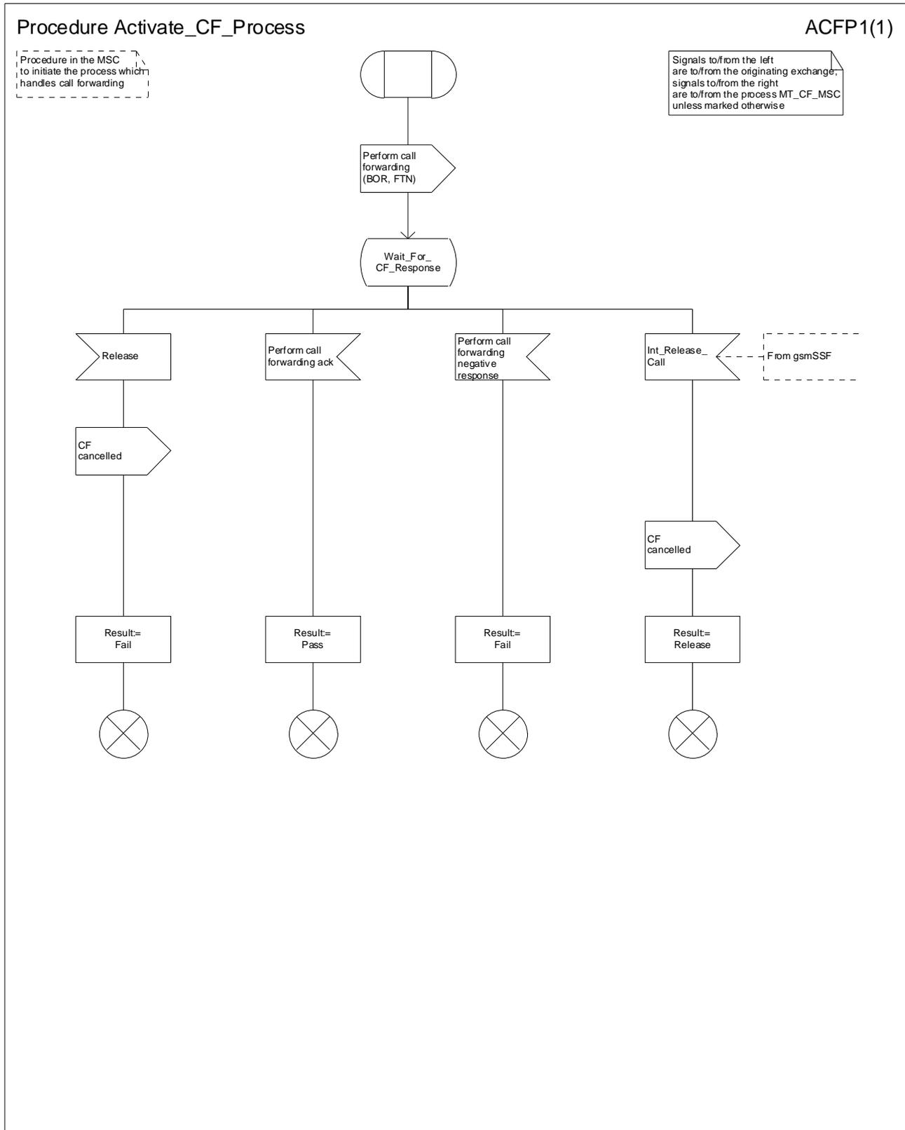
Figure 42: Procedure Activate\_CF\_Process
