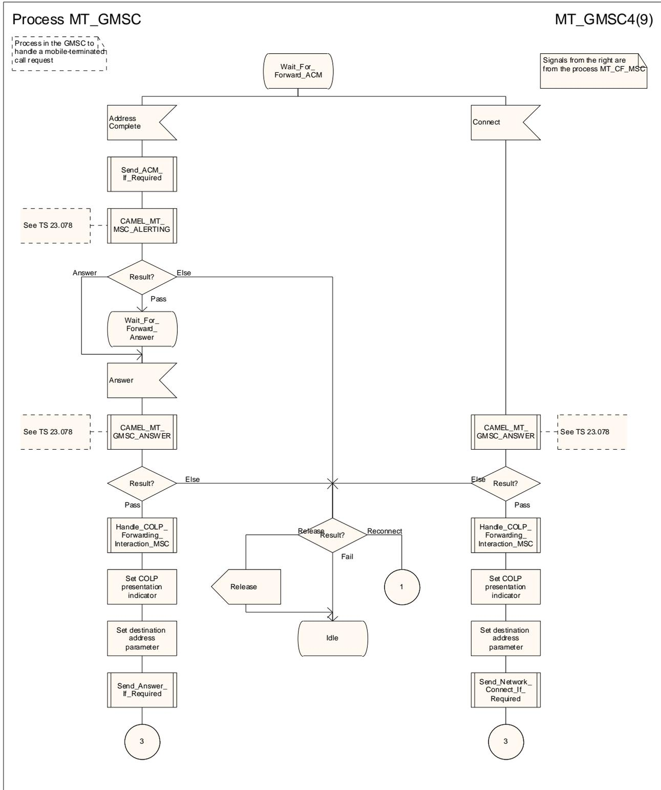
Figure 36d: Process MT\_GMSC (sheet 4)
