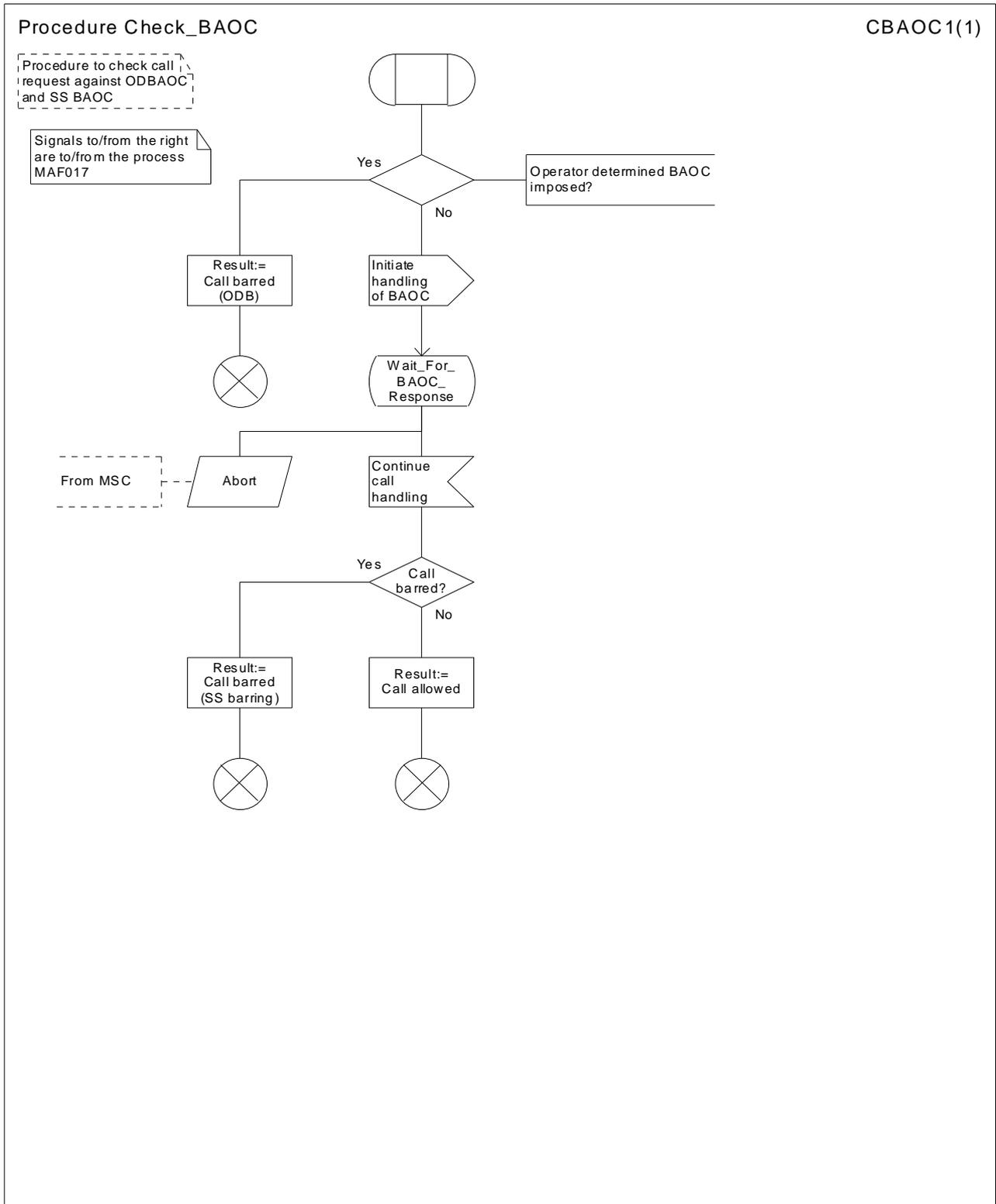
Figure 7.1.2.12: Procedure Check\_BAOC
