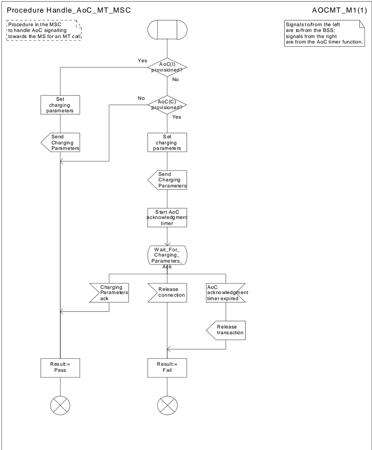
Figure 74: Procedure Handle\_AoC\_MT\_MSC
