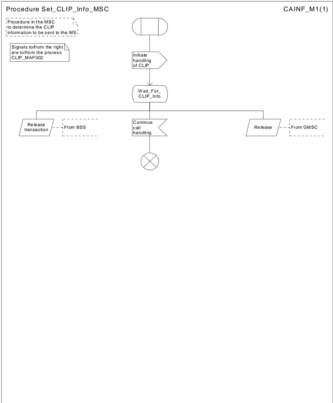
Figure 71: Procedure Set\_CLIP\_Info\_MSC
