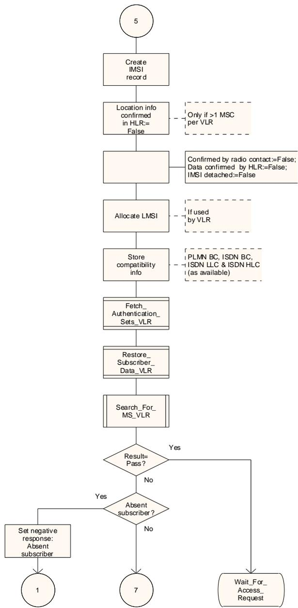
Figure 54e: Process PRN\_VLR (sheet 5)
