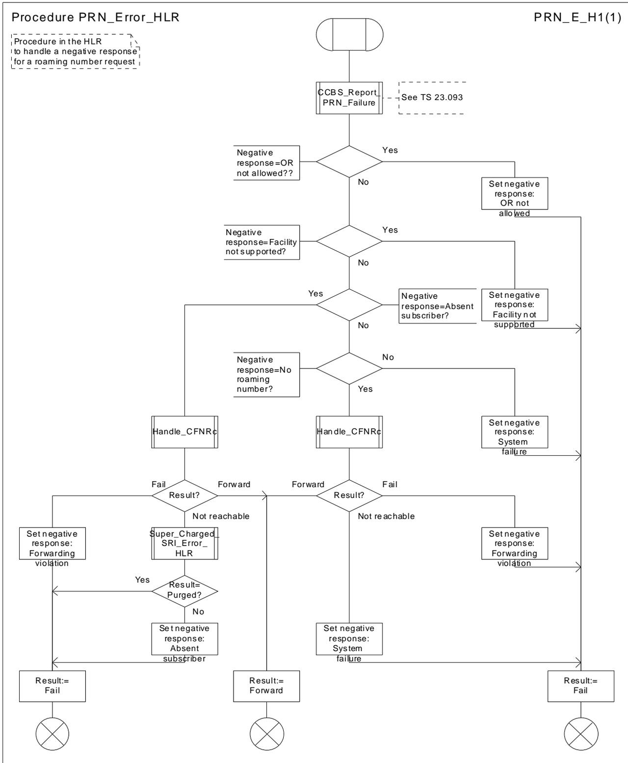
Figure 48: Procedure PRN\_Error\_HLR
