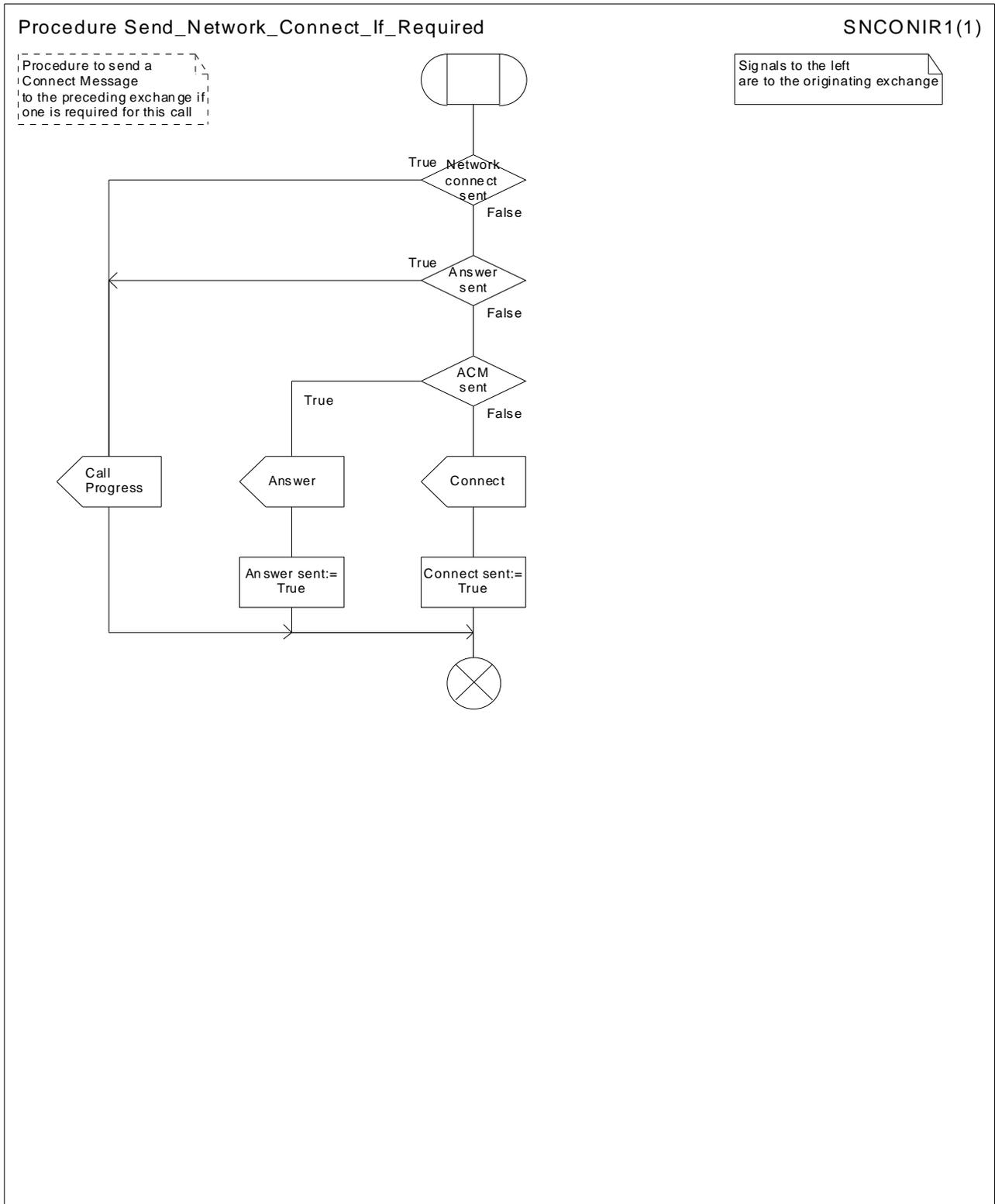
**Figure 40: Procedure Send\_Network\_Connect\_If\_Required**
