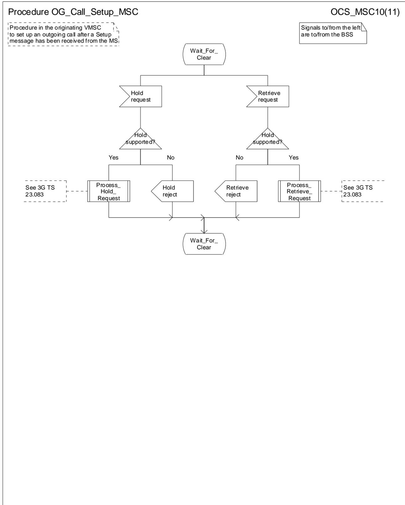
Figure 8j: Procedure OG\_Call\_Setup\_MSC (sheet 10)
