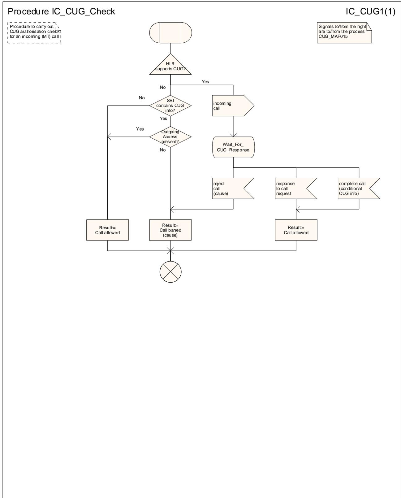
Figure 52: Procedure IC\_CUG\_Check
