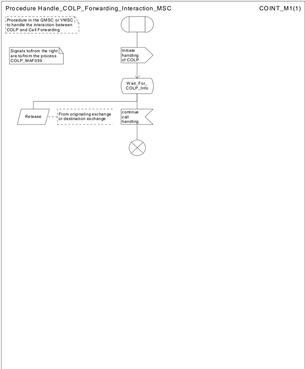
Figure 41: Procedure Handle\_COLP\_Forwarding\_Interaction\_MSC
