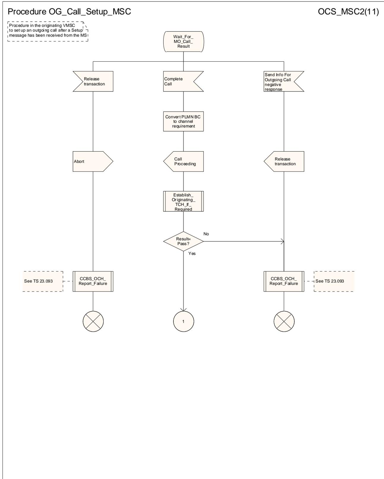
Figure 8b: Procedure OG\_Call\_Setup\_MSC (sheet 2)
