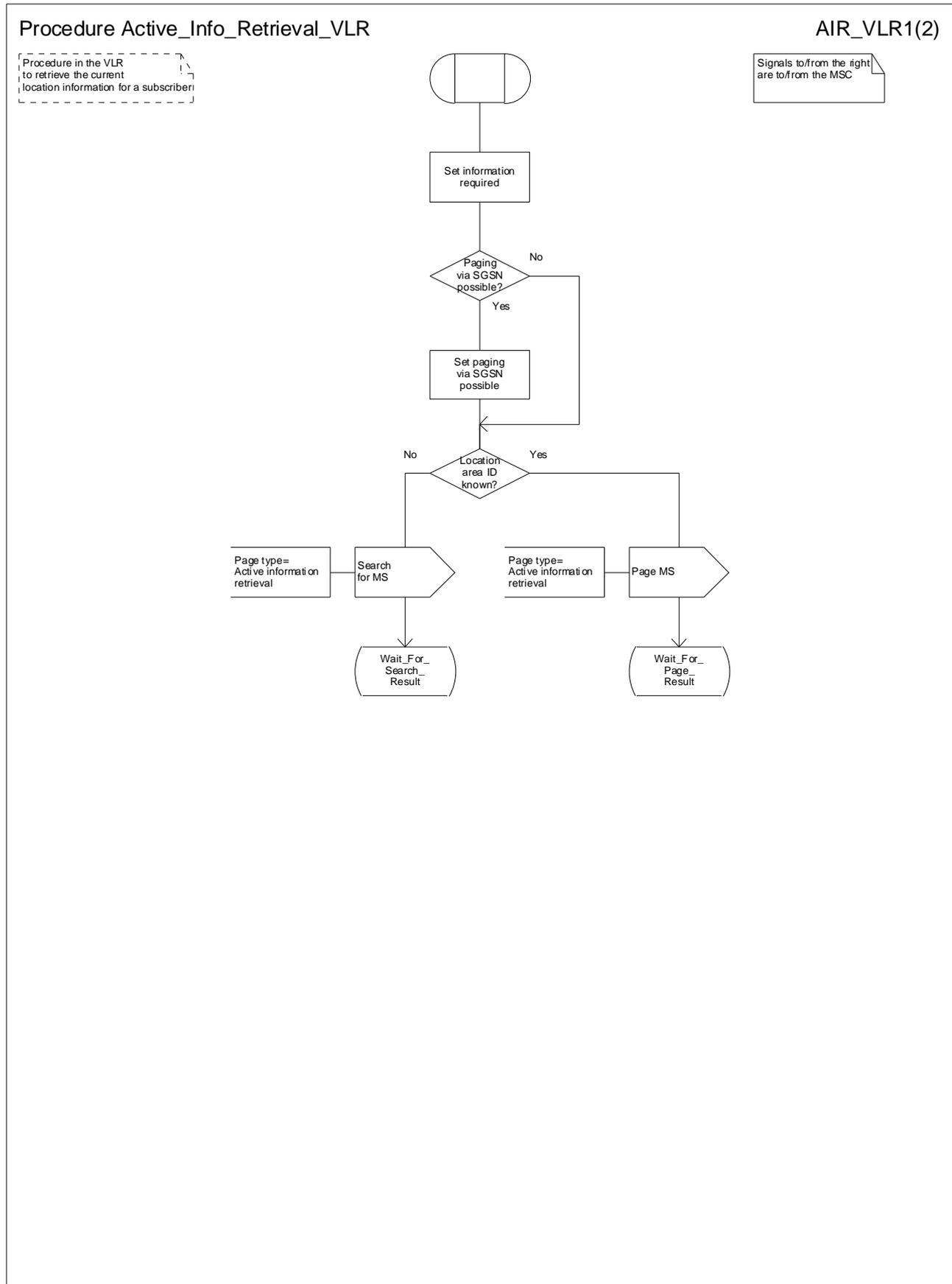
Figure 59a: Procedure Active\_Info\_Retrieval\_VLR
