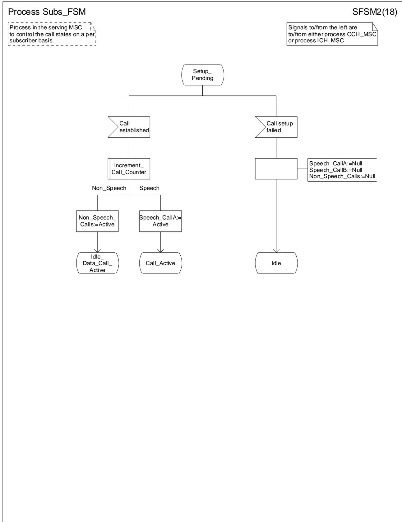
Figure 83b: Process Subs\_FSM (sheet 2)
