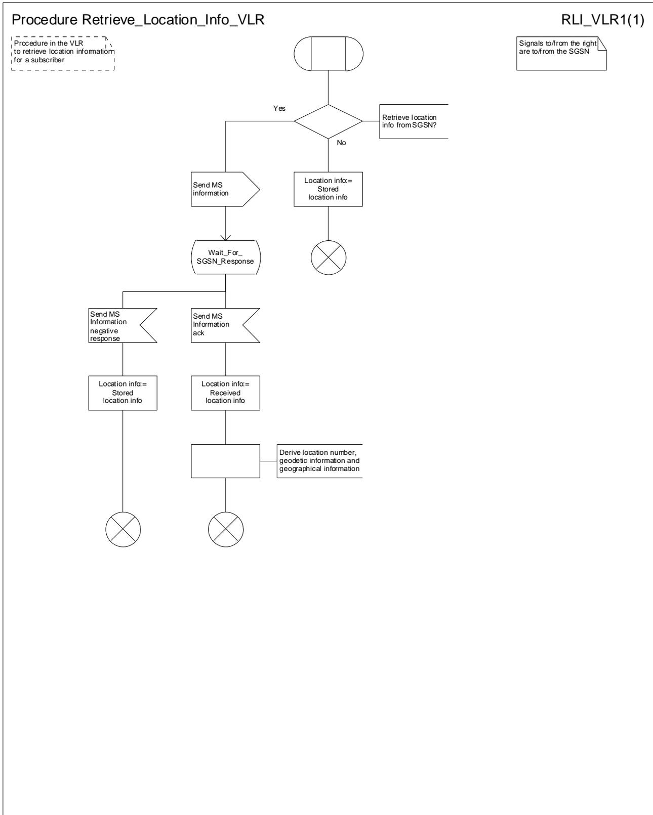
Figure 58: Procedure Retrieve\_Location\_Info\_VLR
