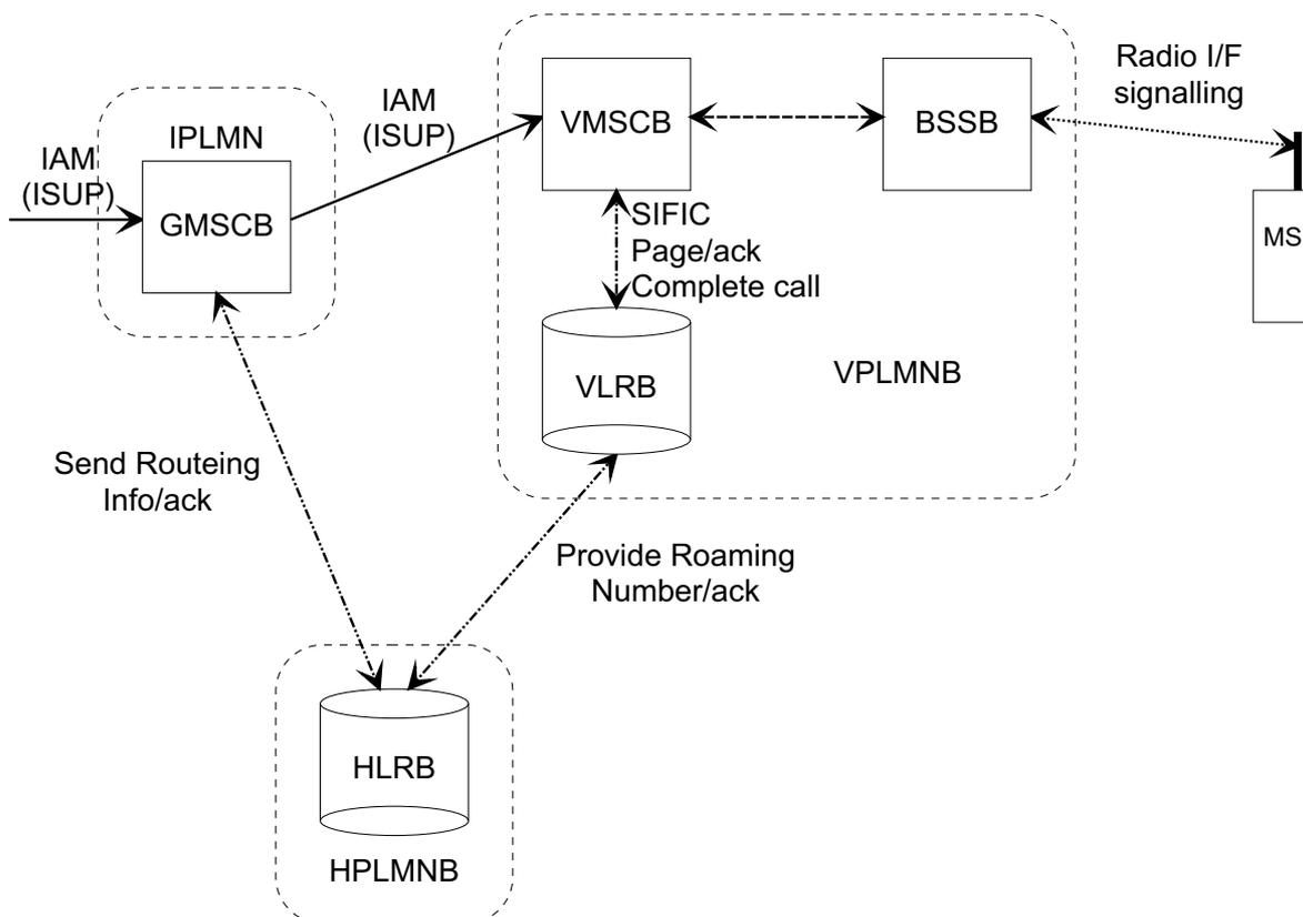
**Figure 2: Architecture for a basic mobile terminated call**
