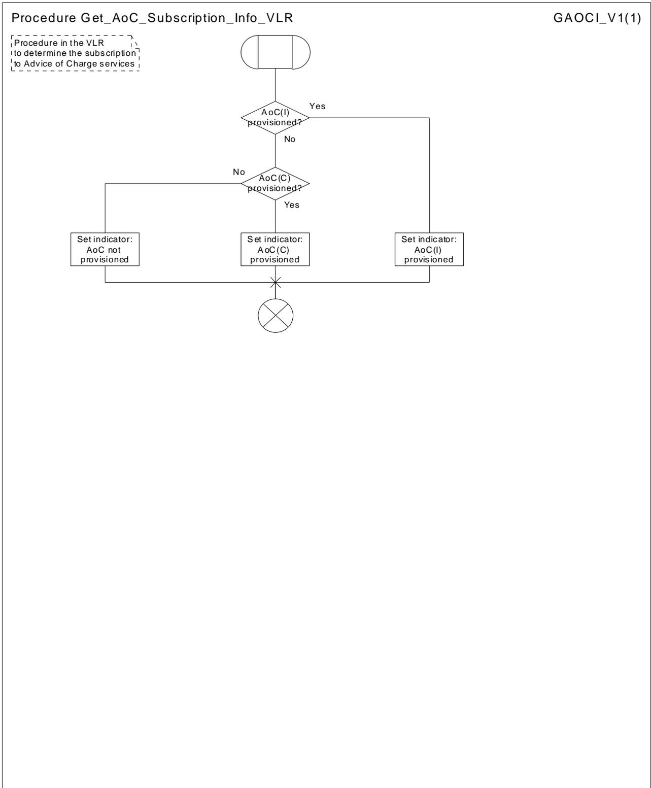
Figure 7.1.2.15: Procedure Get\_AoC\_Subscription\_Info\_VLR
