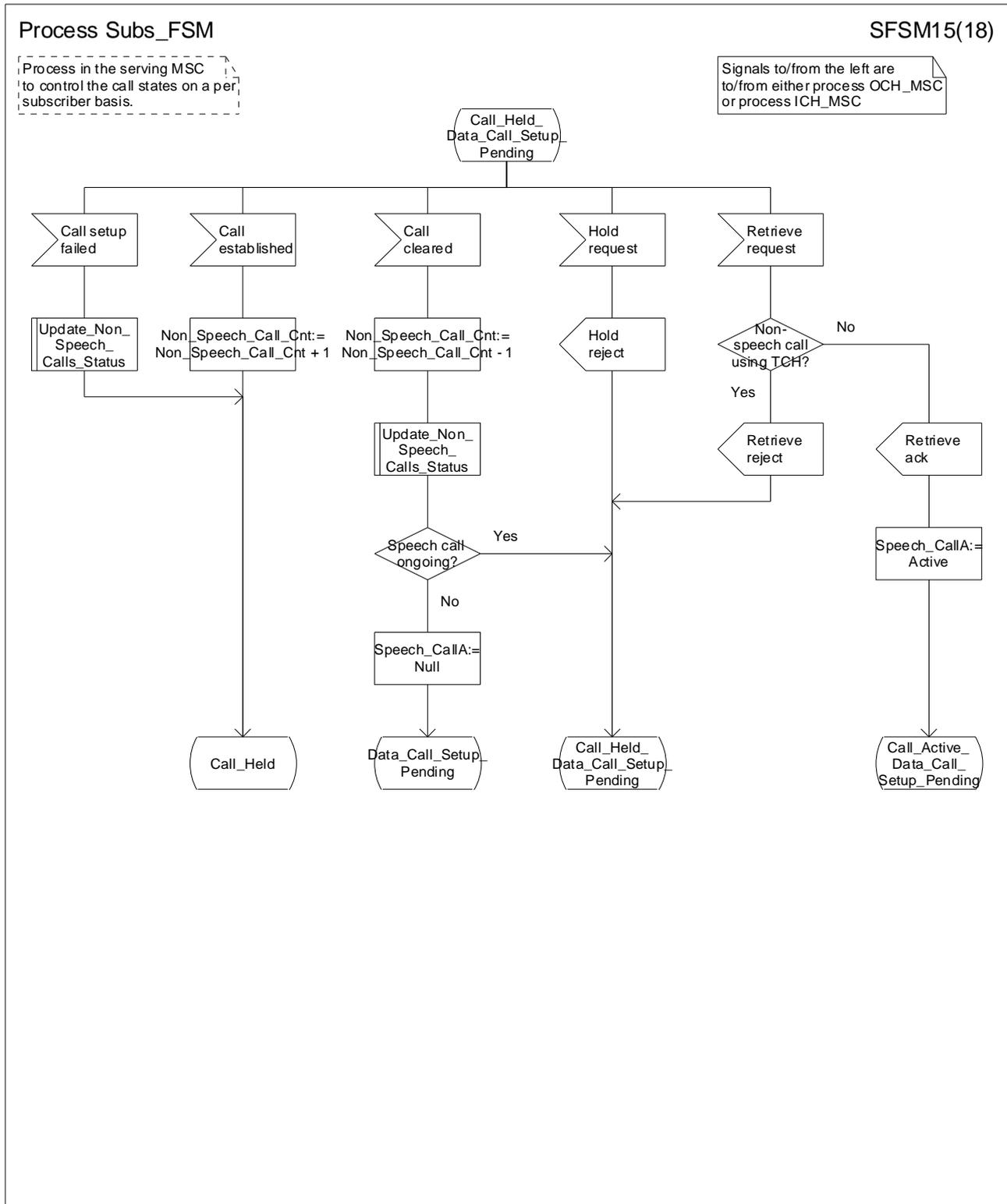
Figure 84o: Process Subs\_FSM (sheet 14)
