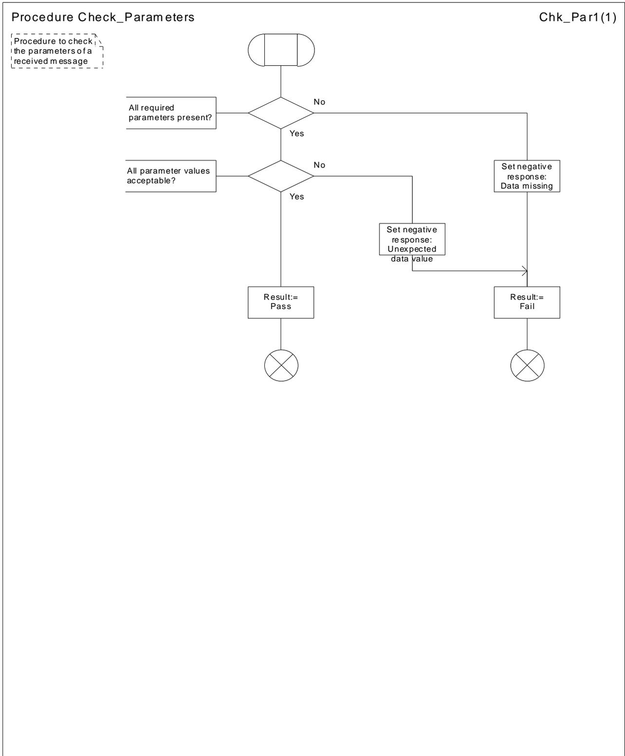
Figure 45: Procedure Check\_Parameters
