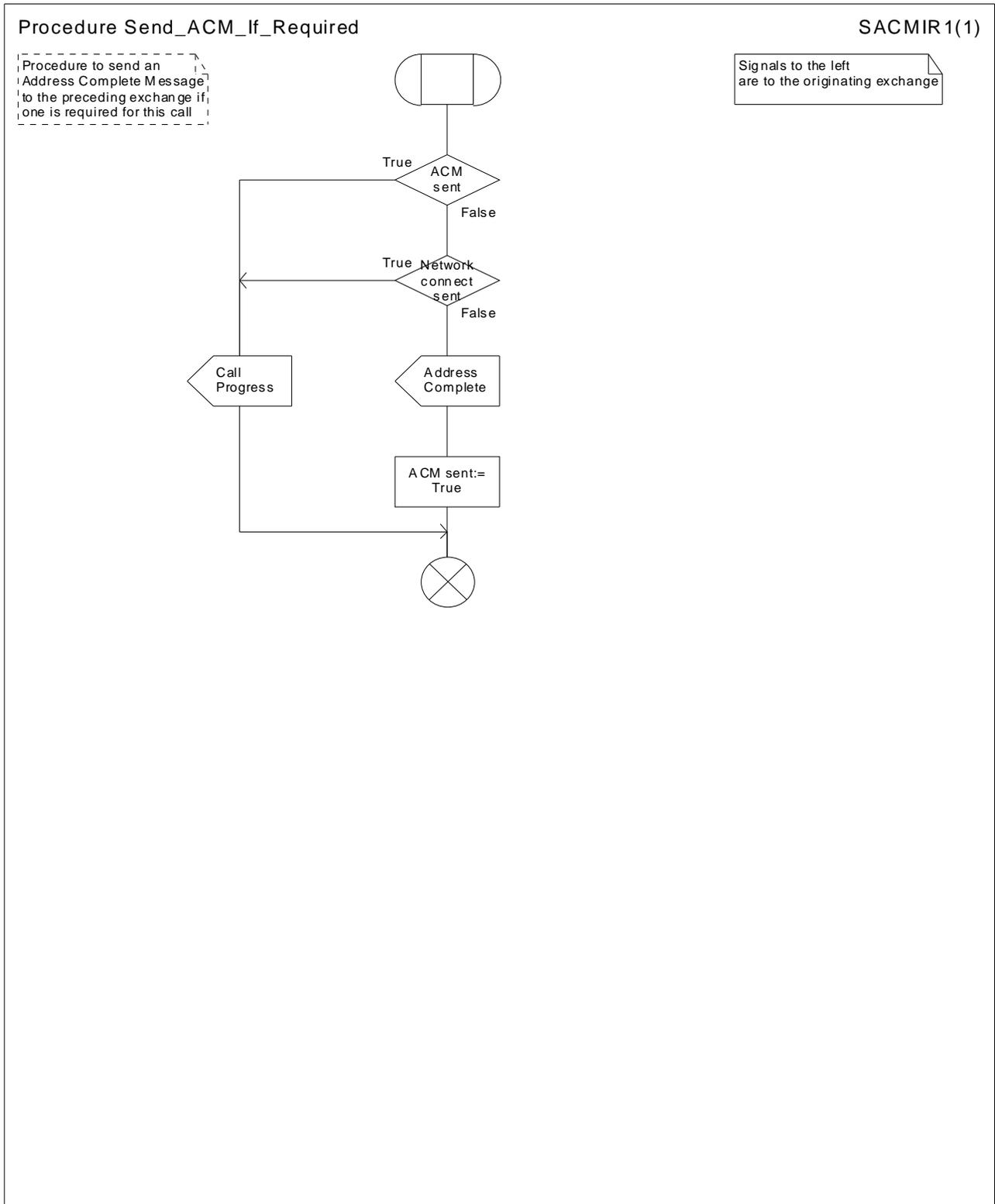
Figure 38: Procedure Send\_ACM\_If\_Required
