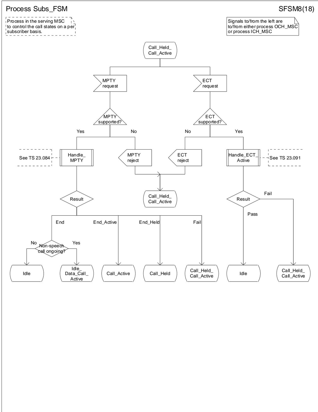
Figure 83h: Process Subs\_FSM (sheet 8)
