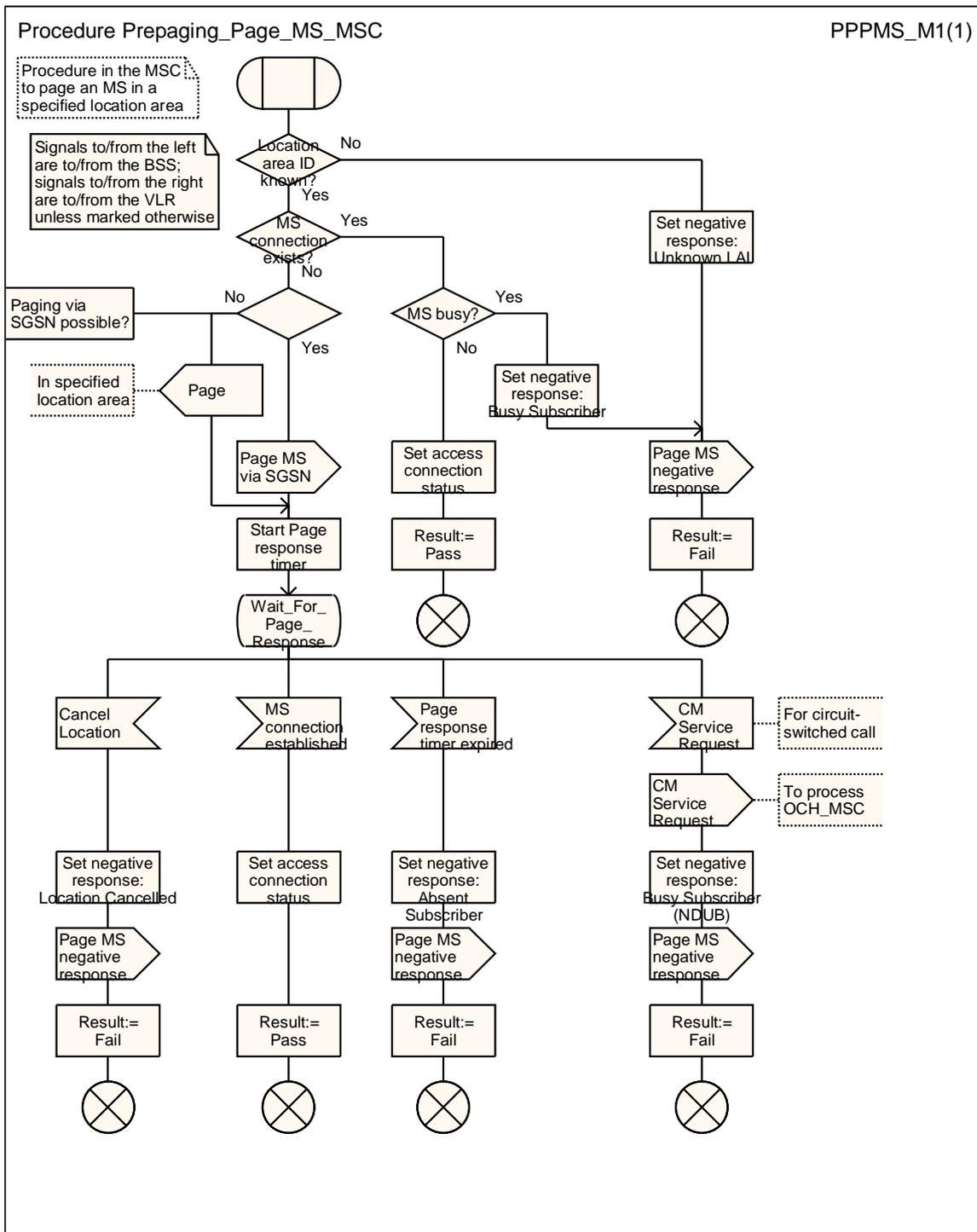
Figure 61: Procedure Prepaging\_Page\_MS\_MSC
