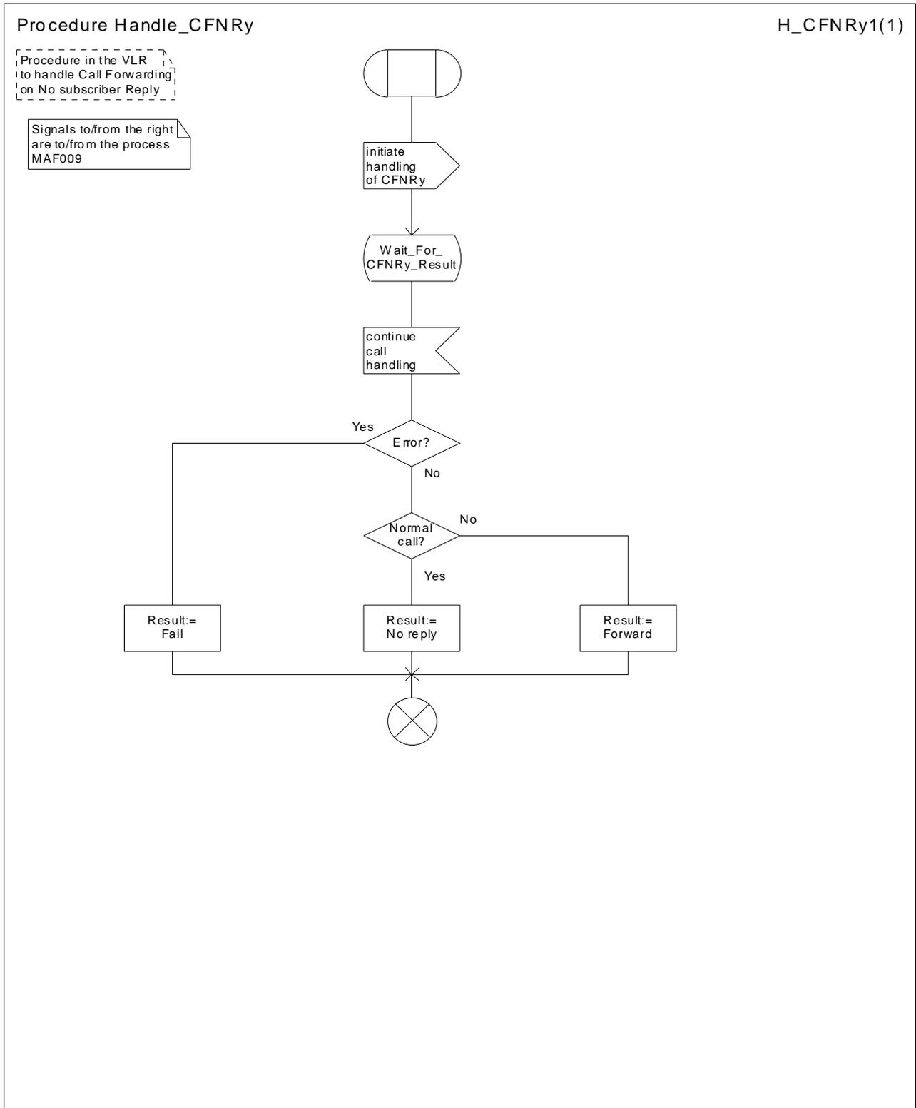
Figure 82: Procedure Handle\_CFNRy
