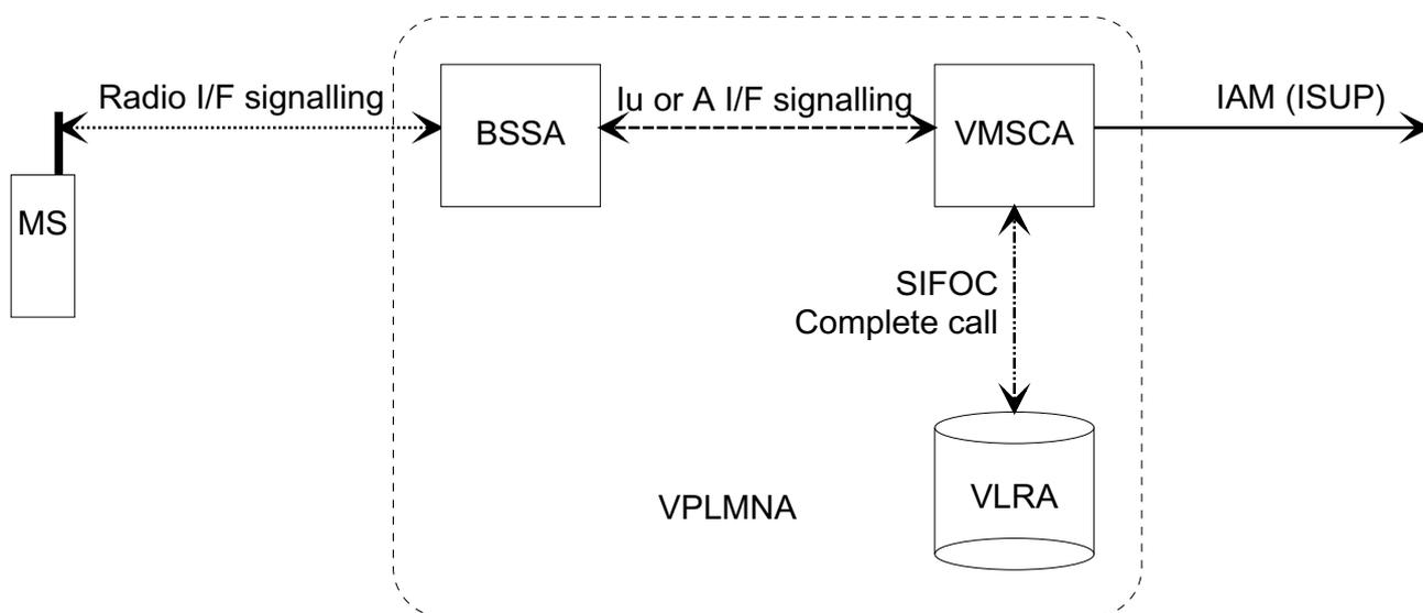
**Figure 1: Architecture for a basic mobile originated call**
