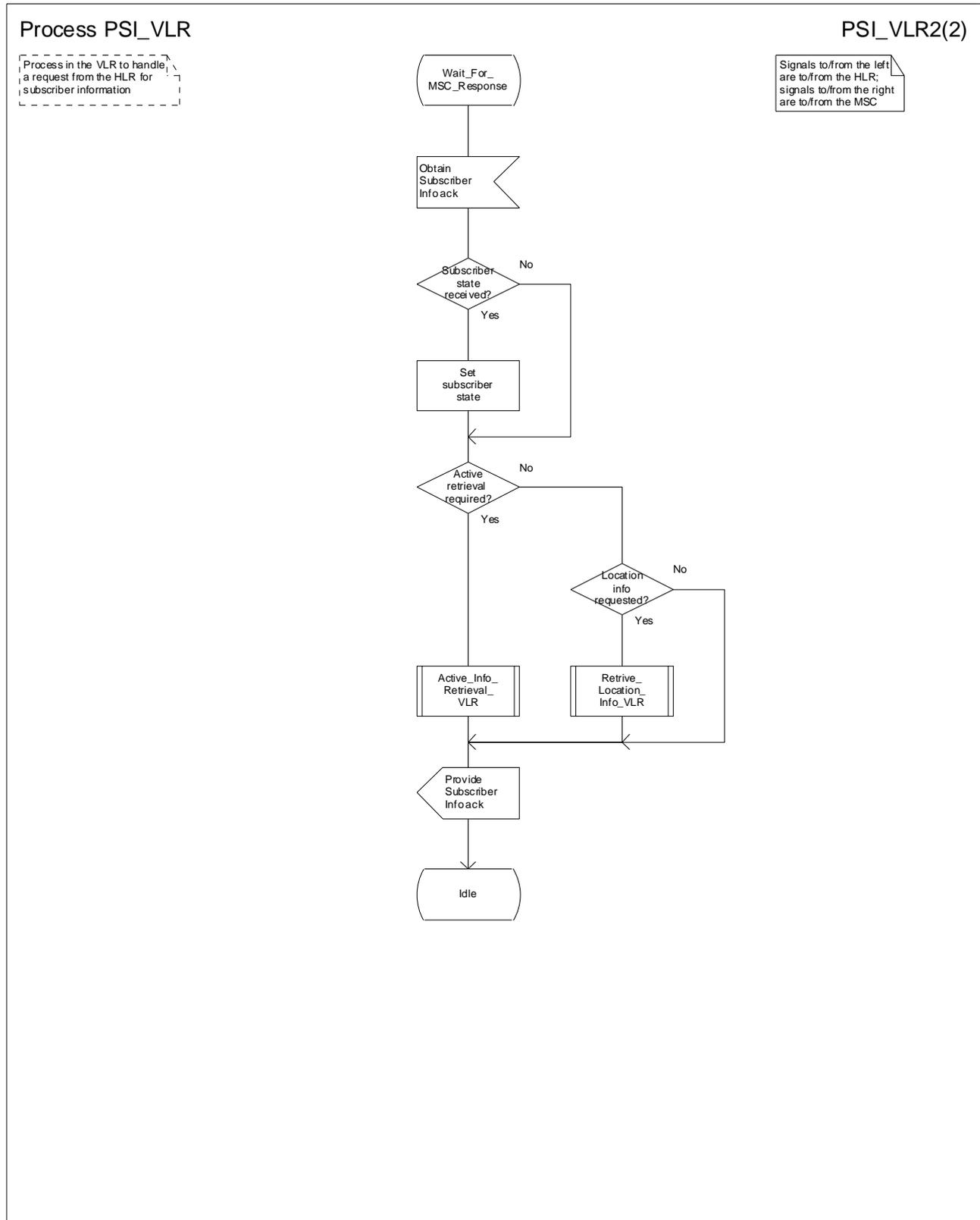
Figure 57b: Process PSI\_VLR (sheet 2)
