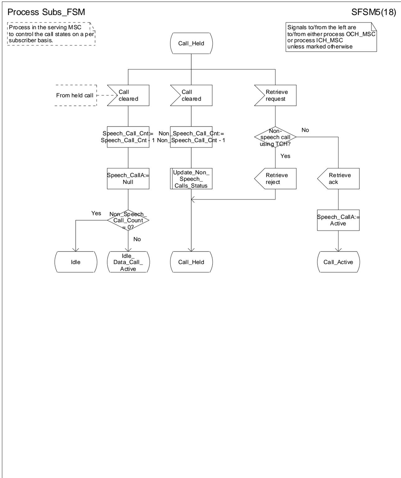
Figure 83e: Process Subs\_FSM (sheet 5)
