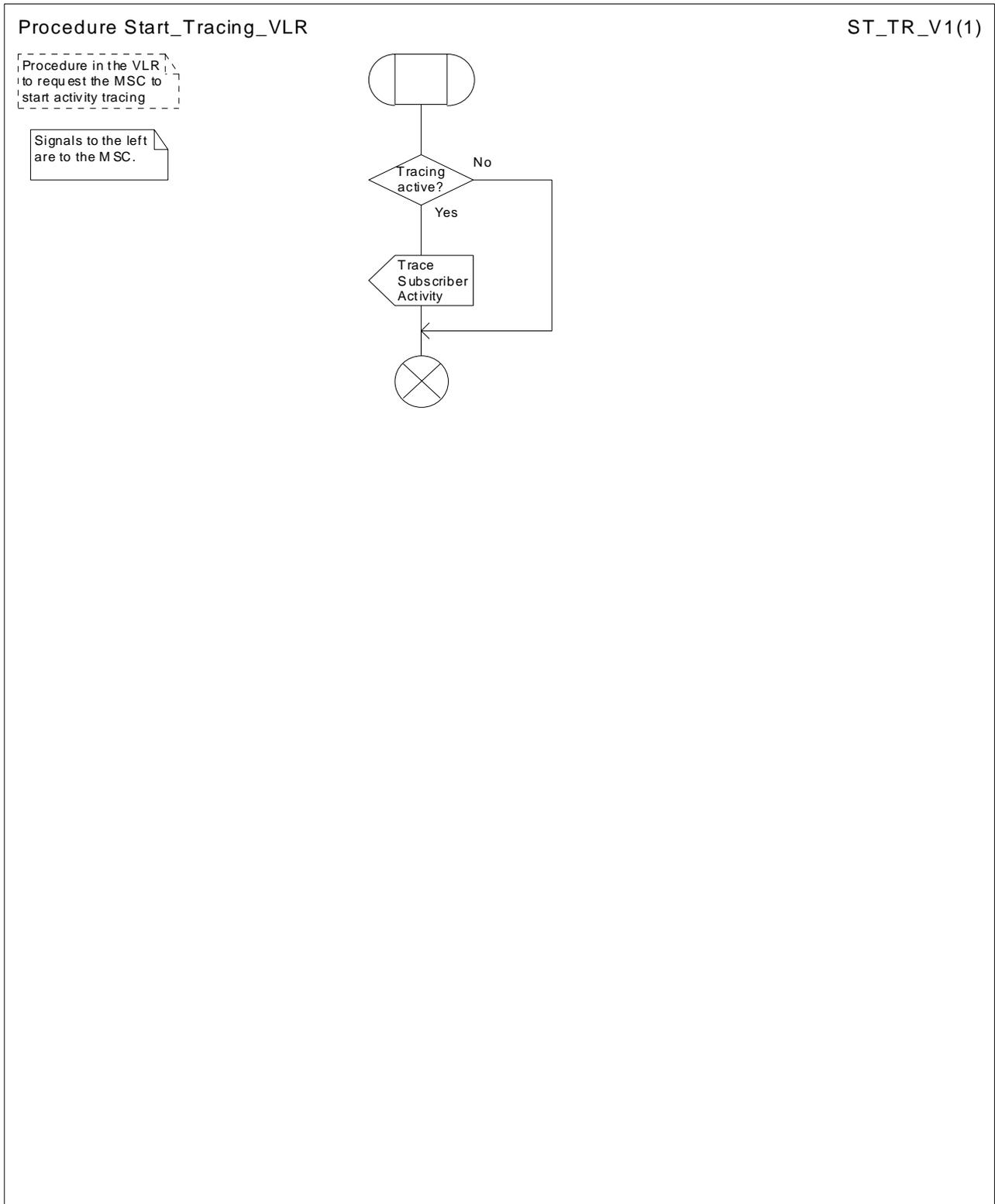
Figure 7.1.2.8: Procedure Start\_Tracing\_VLR
