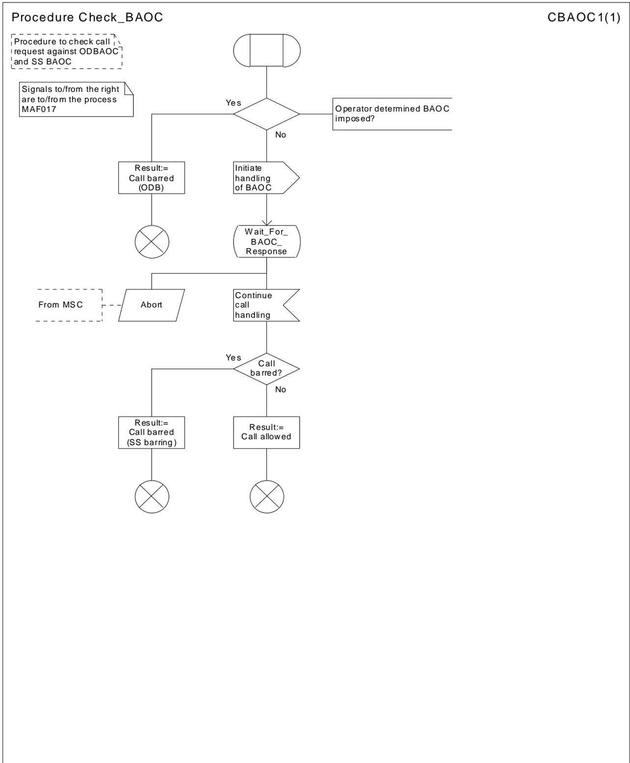
Figure 7.1.2.12: Procedure Check\_BAOC
