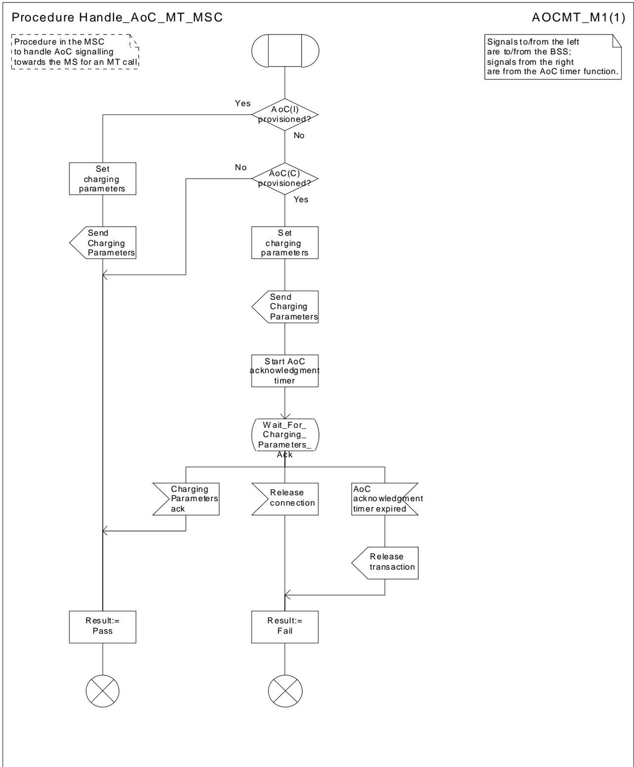
Figure 74: Procedure Handle\_AoC\_MT\_MSC
