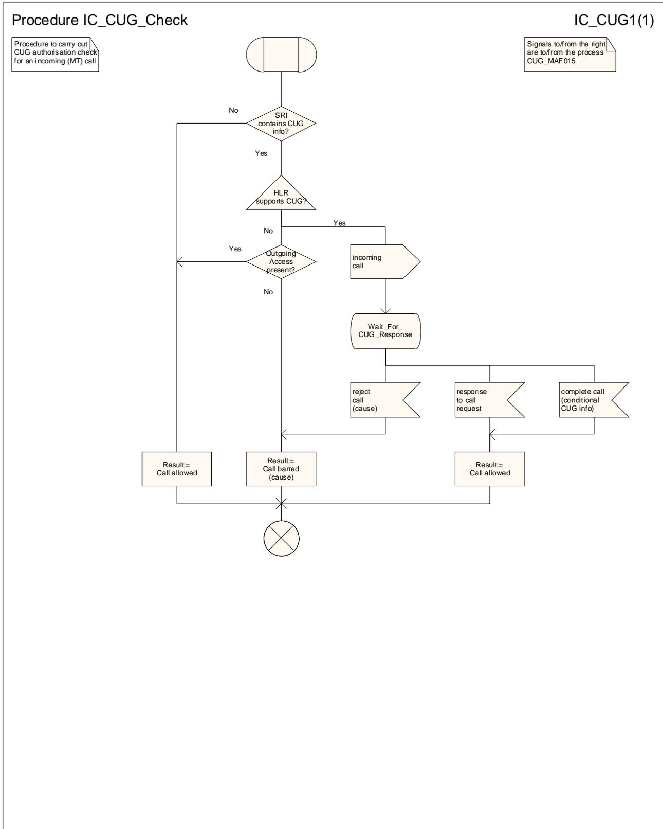
Figure 52: Procedure IC\_CUG\_Check
