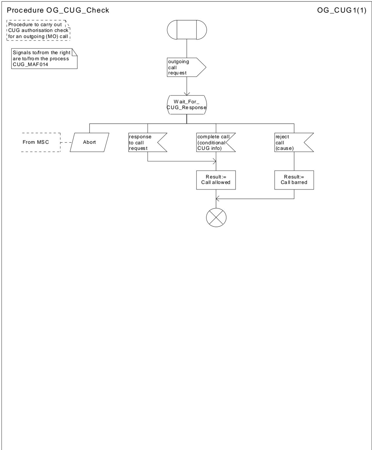
Figure 7.1.2.13: Procedure OG\_CUG\_Check
