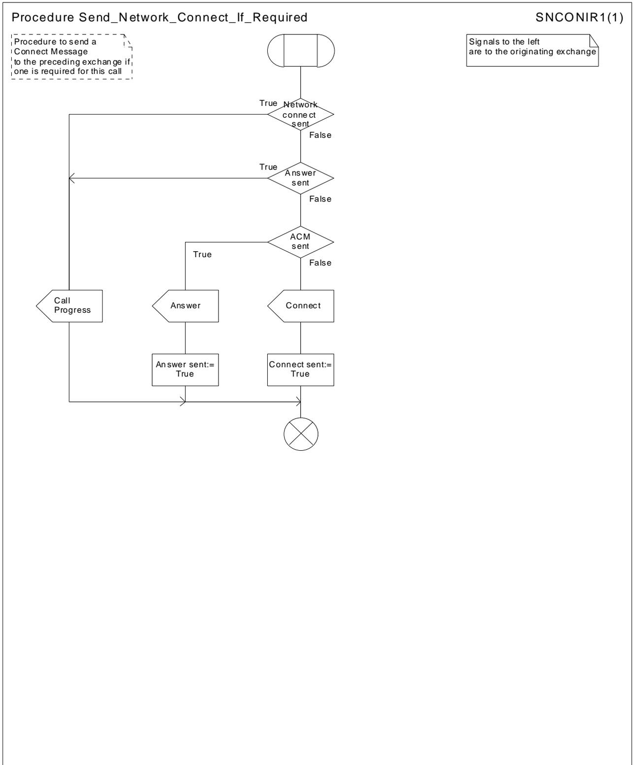
Figure 40: Procedure Send\_Network\_Connect\_If\_Required
