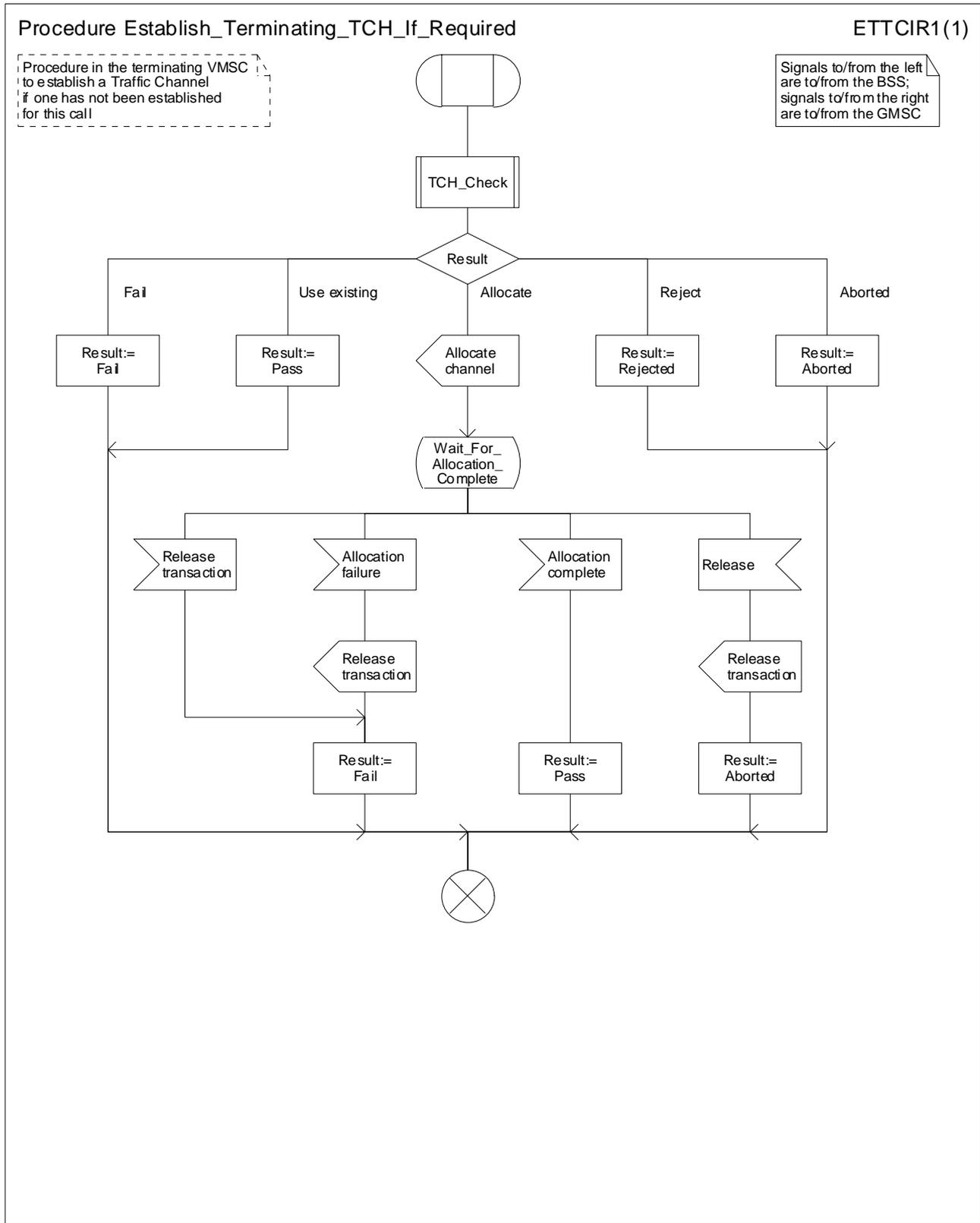
Figure 73: Procedure Establish\_Terminating\_TCH\_If\_Required
