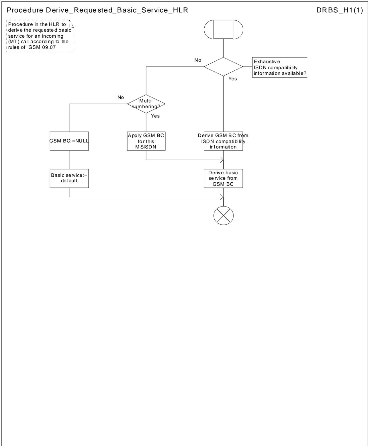
Figure 50: Procedure Derive\_Requested\_Basic\_Service\_HLR
