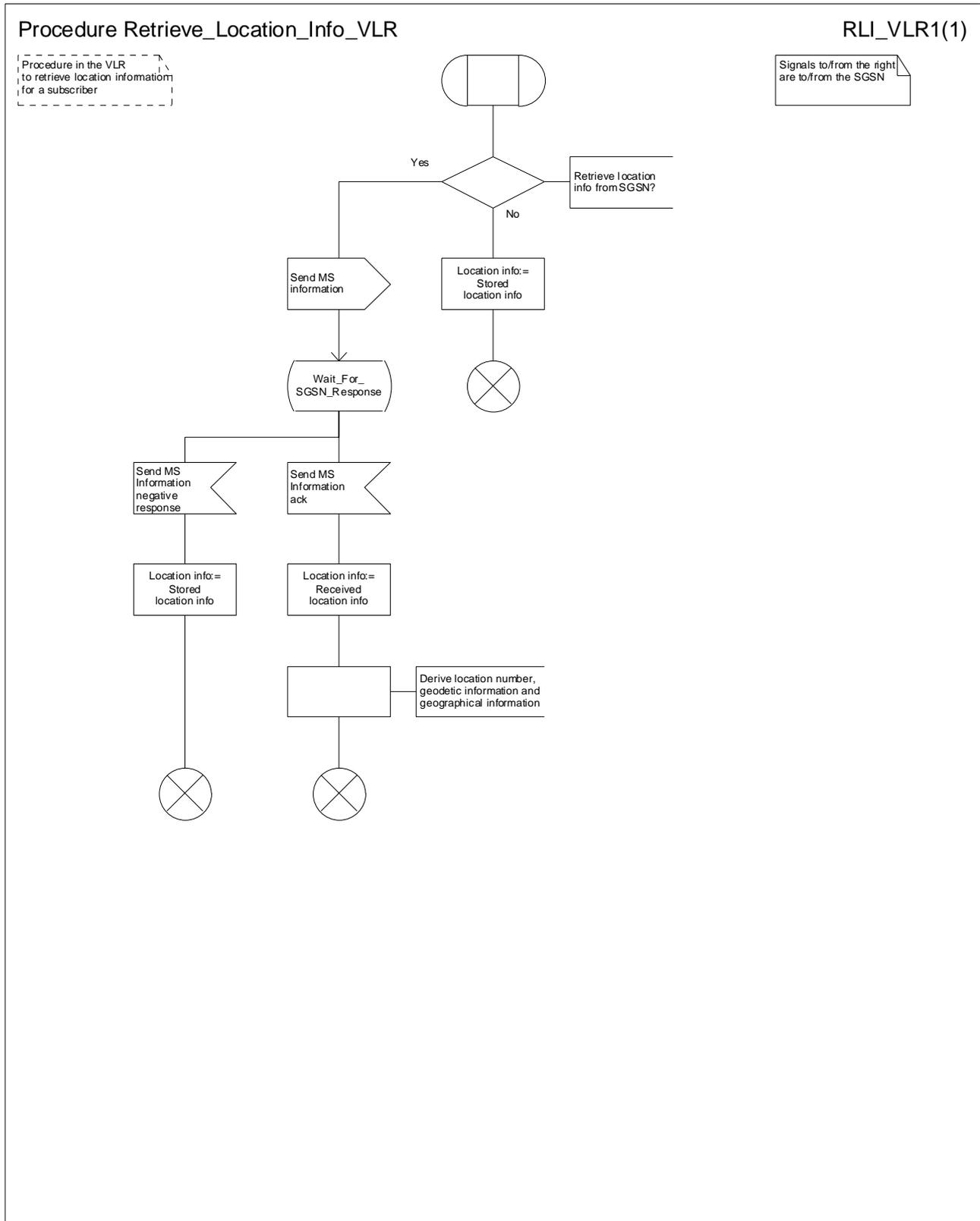
Figure 58: Procedure Retrieve\_Location\_Info\_VLR
