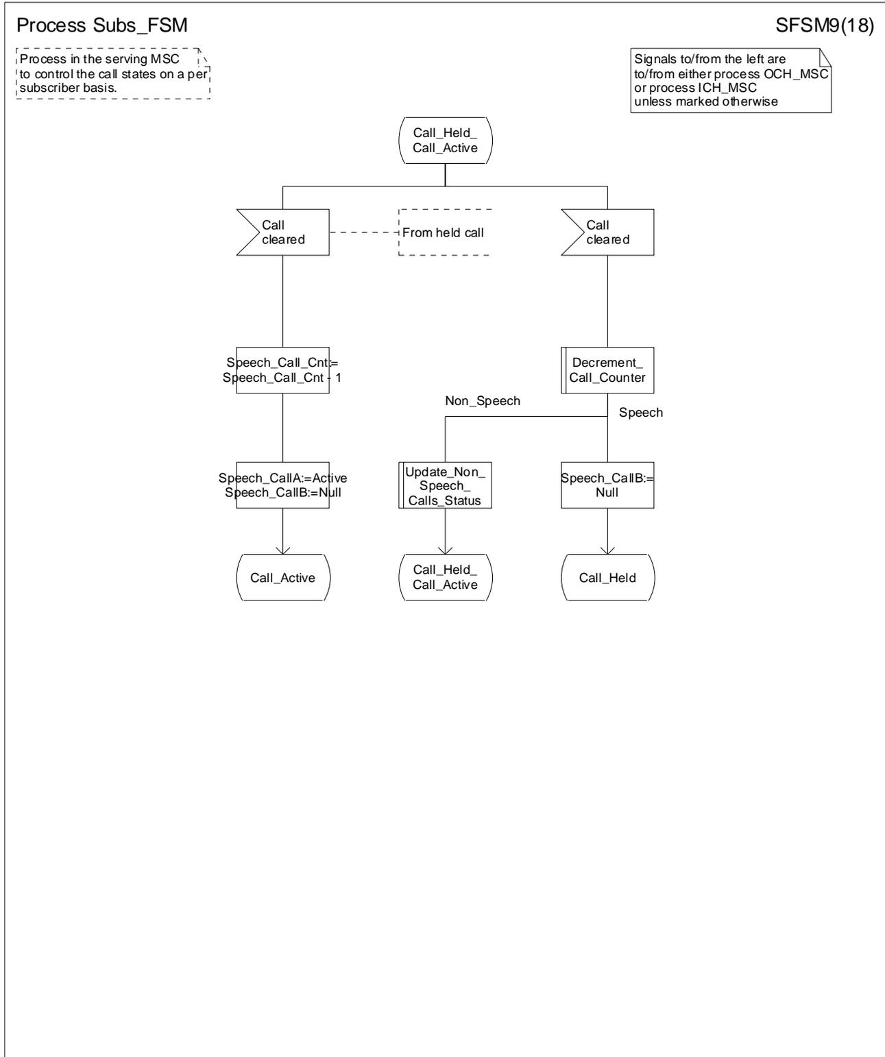
Figure 83i: Process Subs\_FSM (sheet 9)
