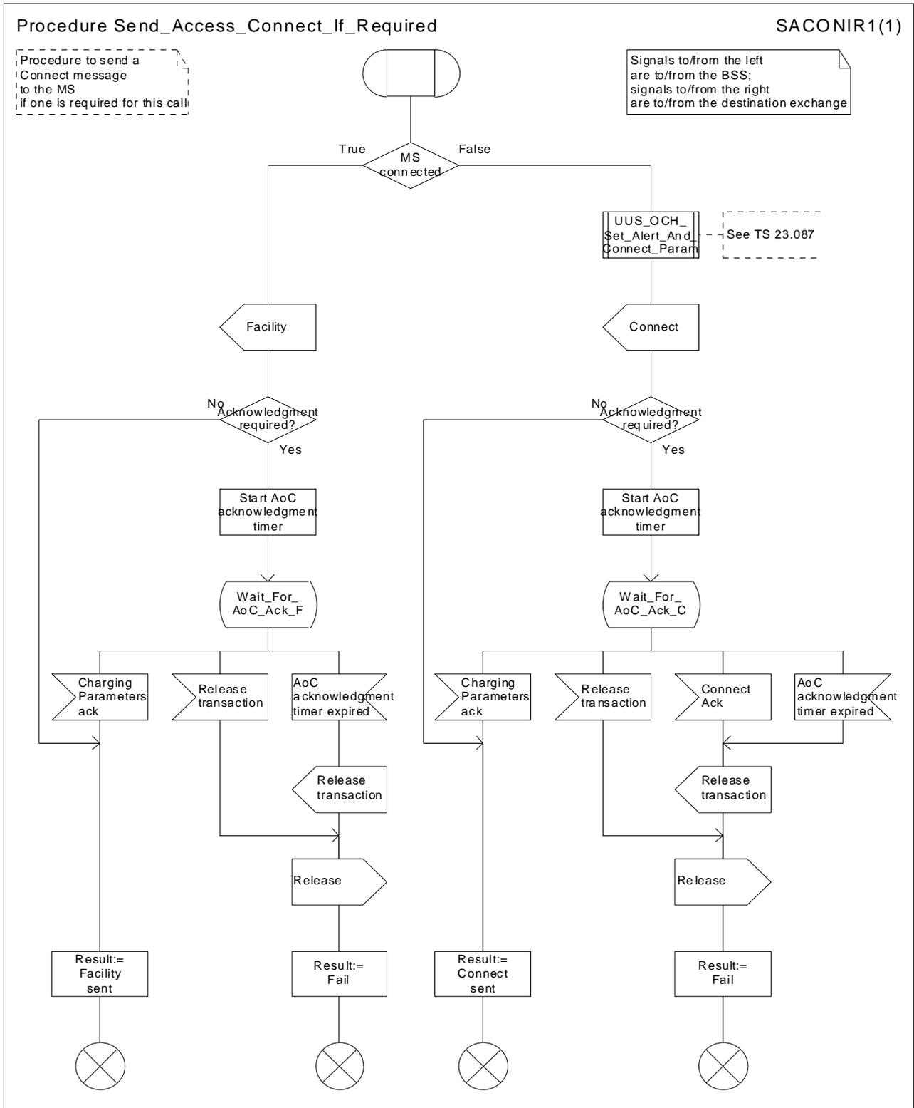
Figure 18: Procedure Send\_Access\_Connect\_If\_Required
