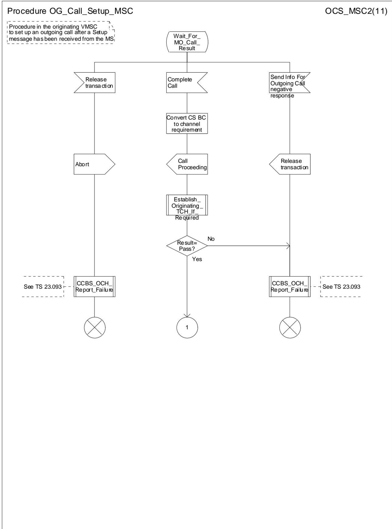
Figure 8b: Procedure OG\_Call\_Setup\_MSC (sheet 2)
