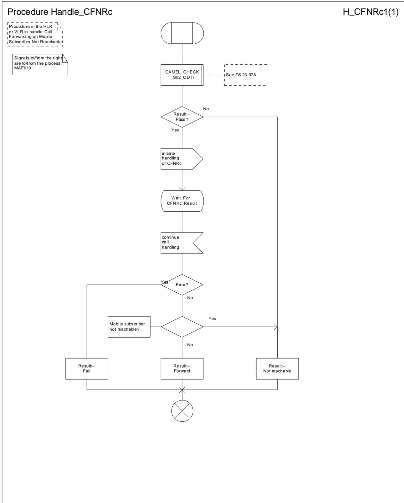
Figure 54: Procedure Handle\_CFNRc
