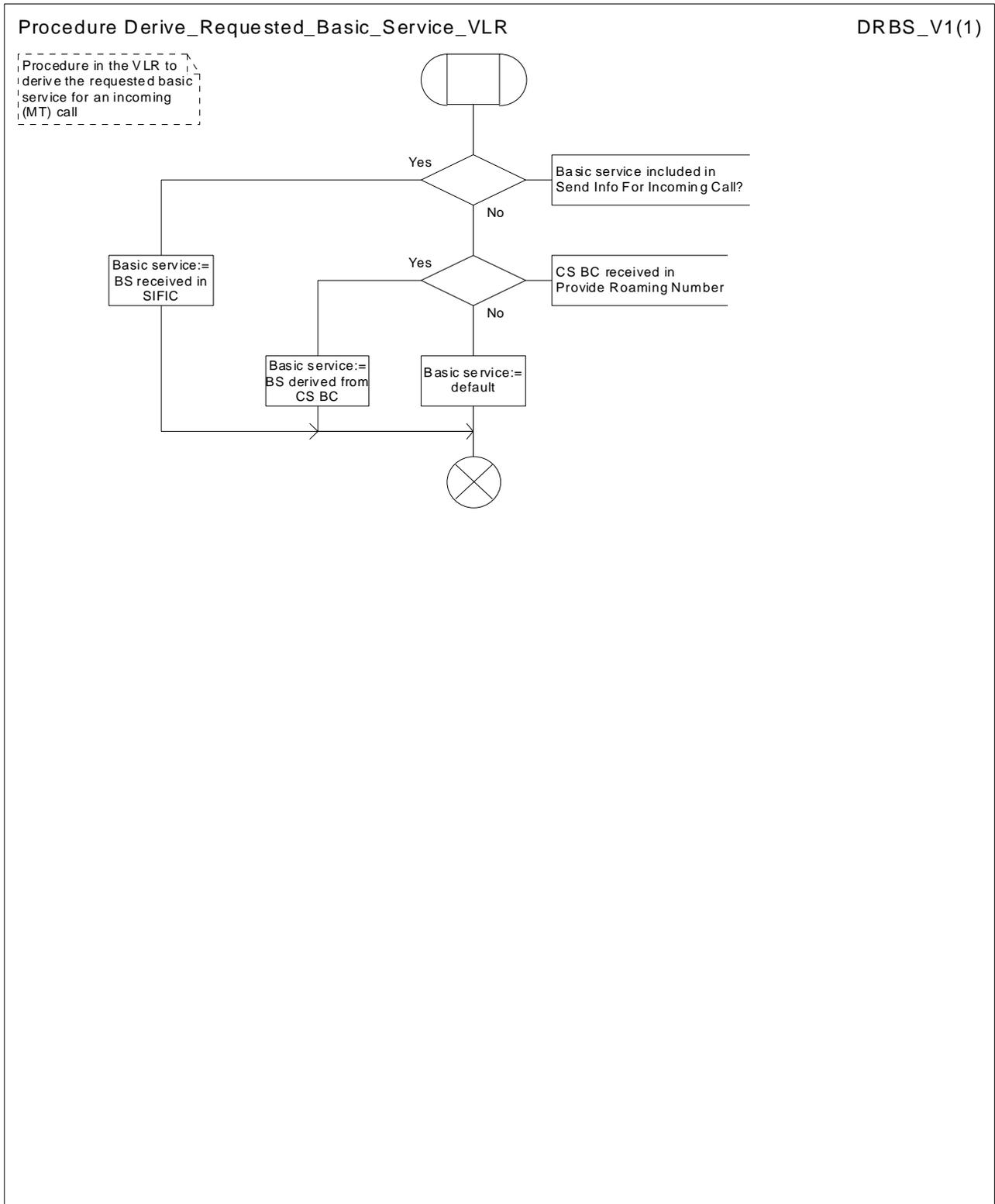
Figure 77: Procedure Derive\_Requested\_Basic\_Service\_VLR
