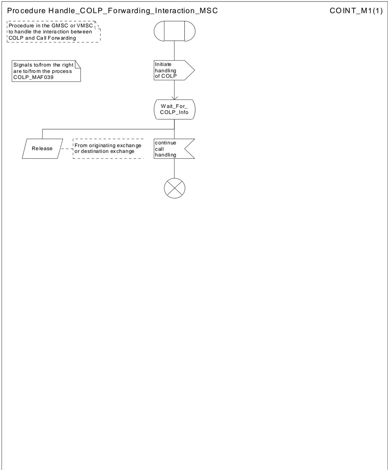
Figure 41: Procedure Handle\_COLP\_Forwarding\_Interaction\_MSC
