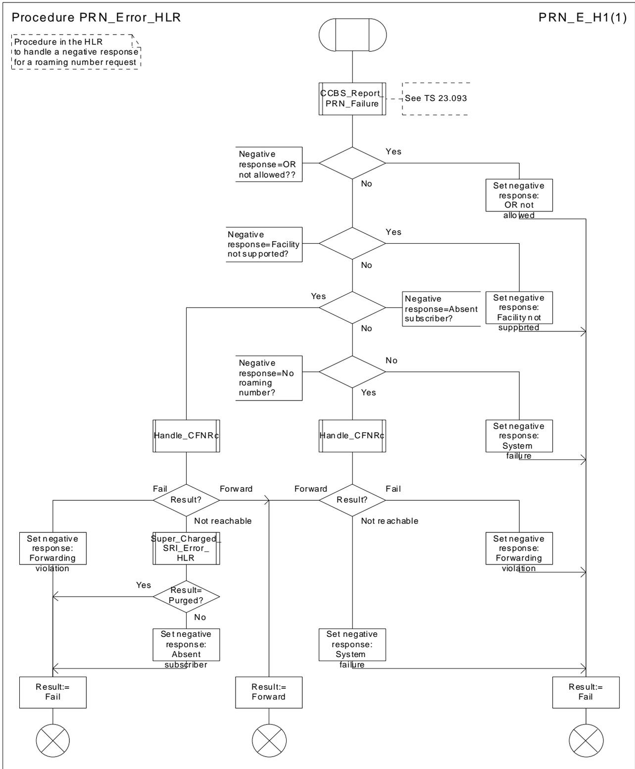
Figure 48: Procedure PRN\_Error\_HLR
