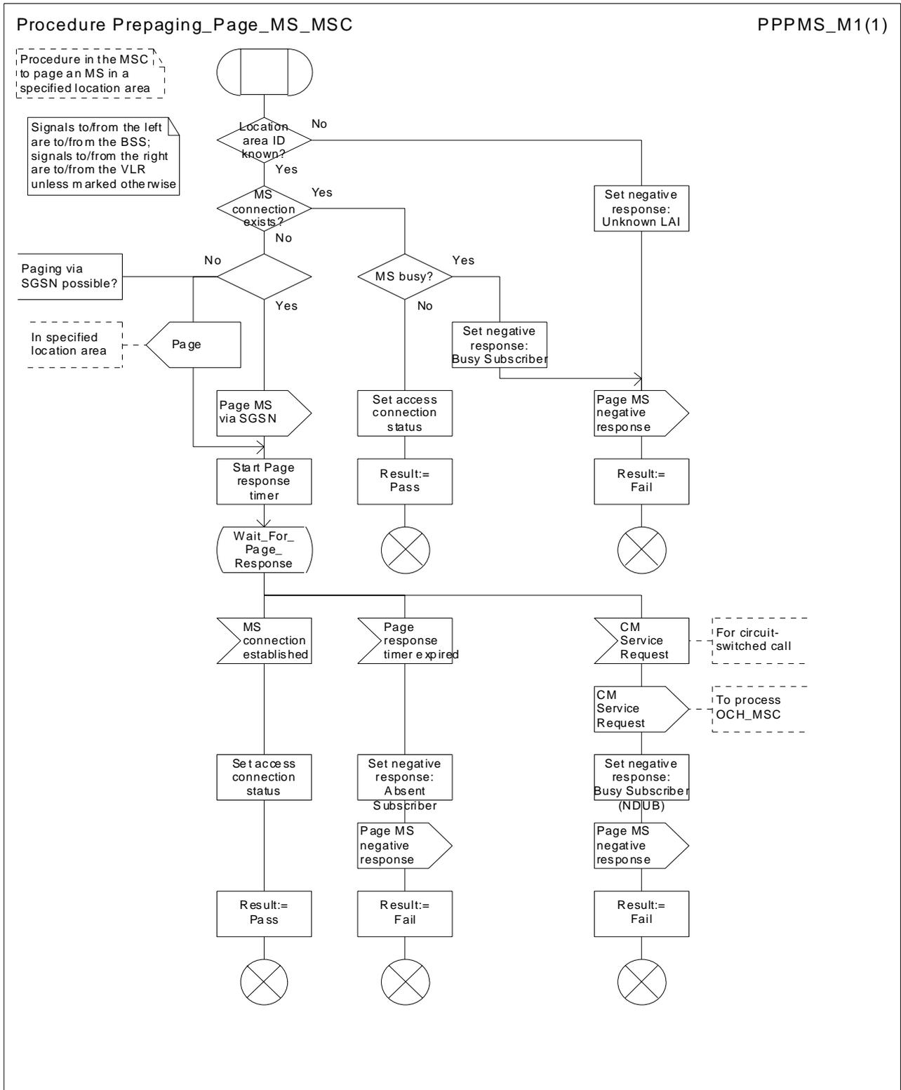
Figure 61: Procedure Prepaging\_Page\_MS\_MSC
