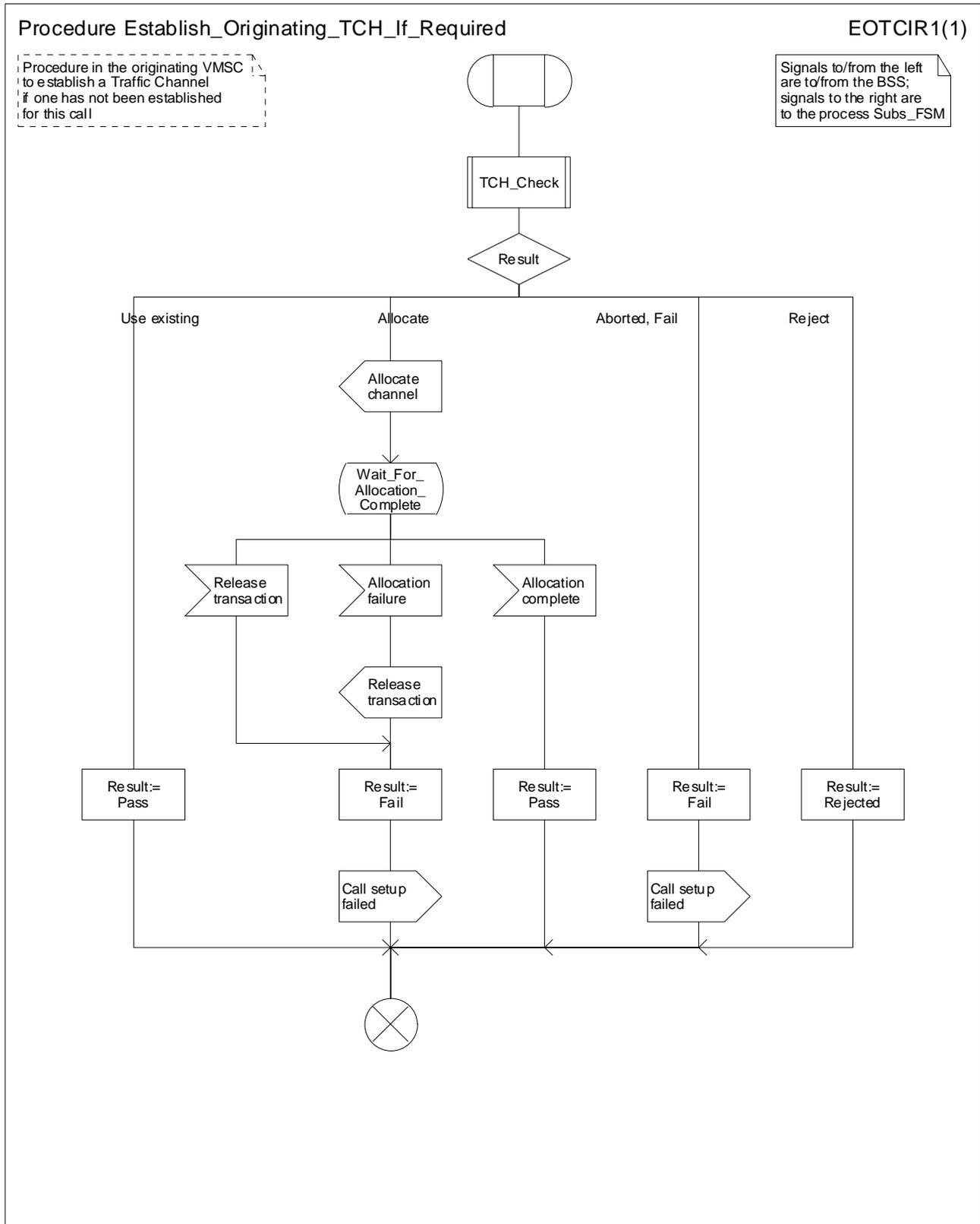
Figure 13: Procedure Establish\_Originating\_TCH\_If\_Required
