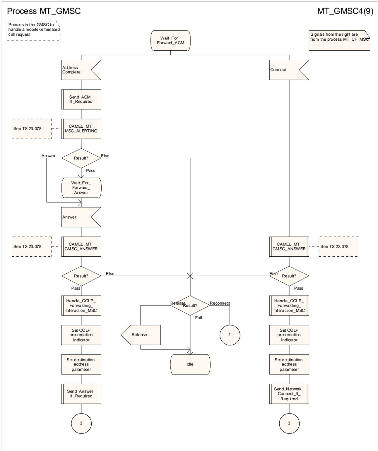
Figure 36d: Process MT\_GMSC (sheet 4)
