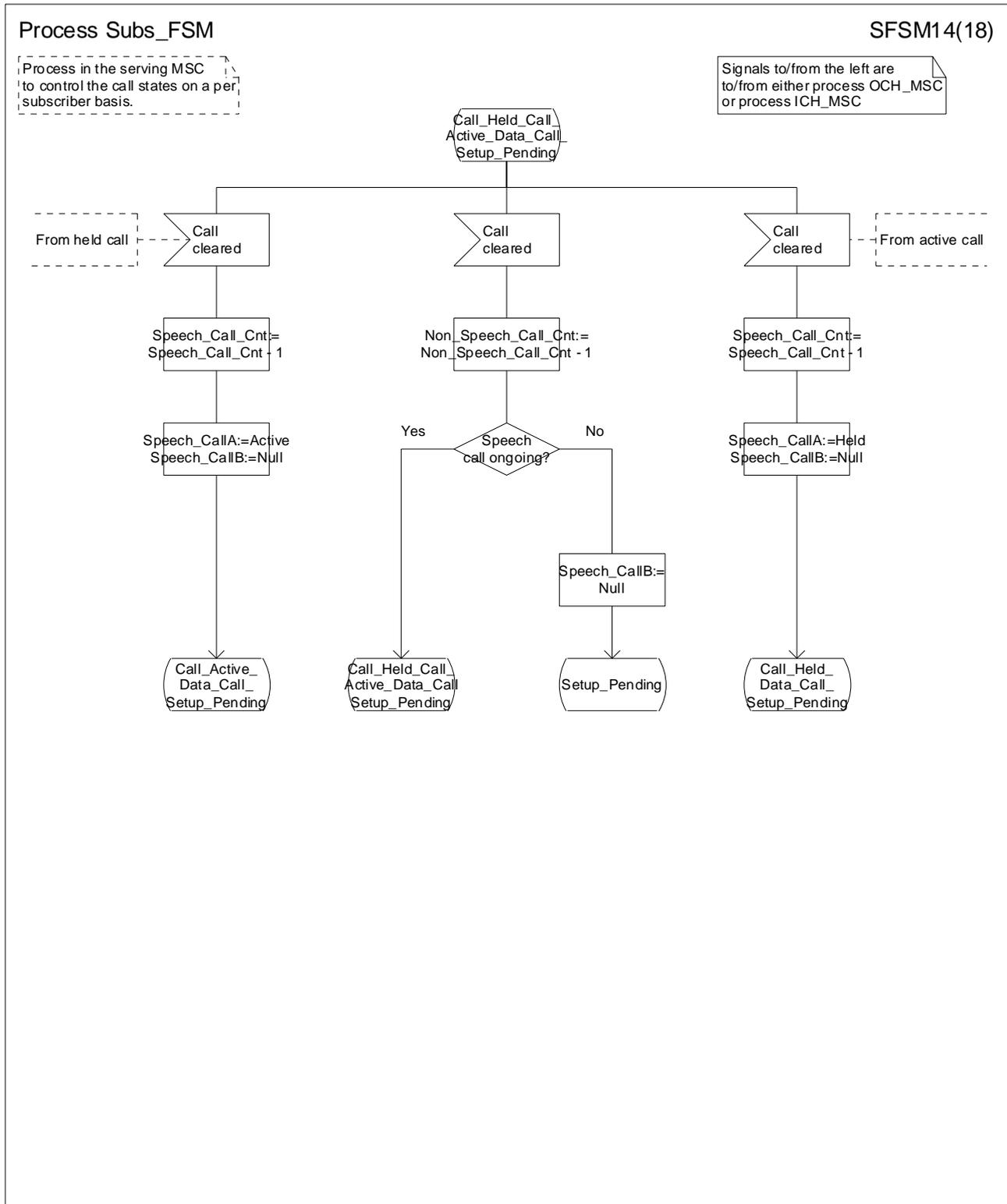
Figure 84n: Process Subs\_FSM (sheet 14)
