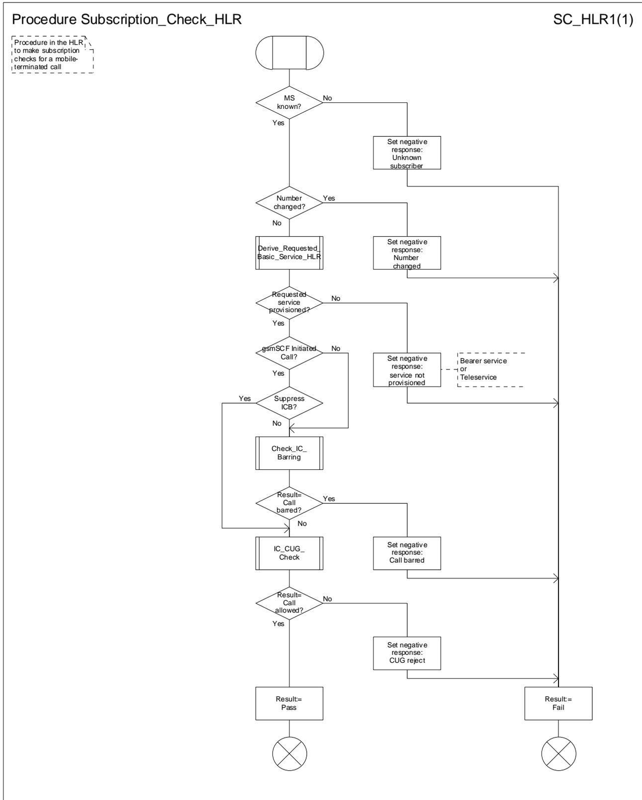
Figure 46: Procedure Subscription\_Check\_HLR
