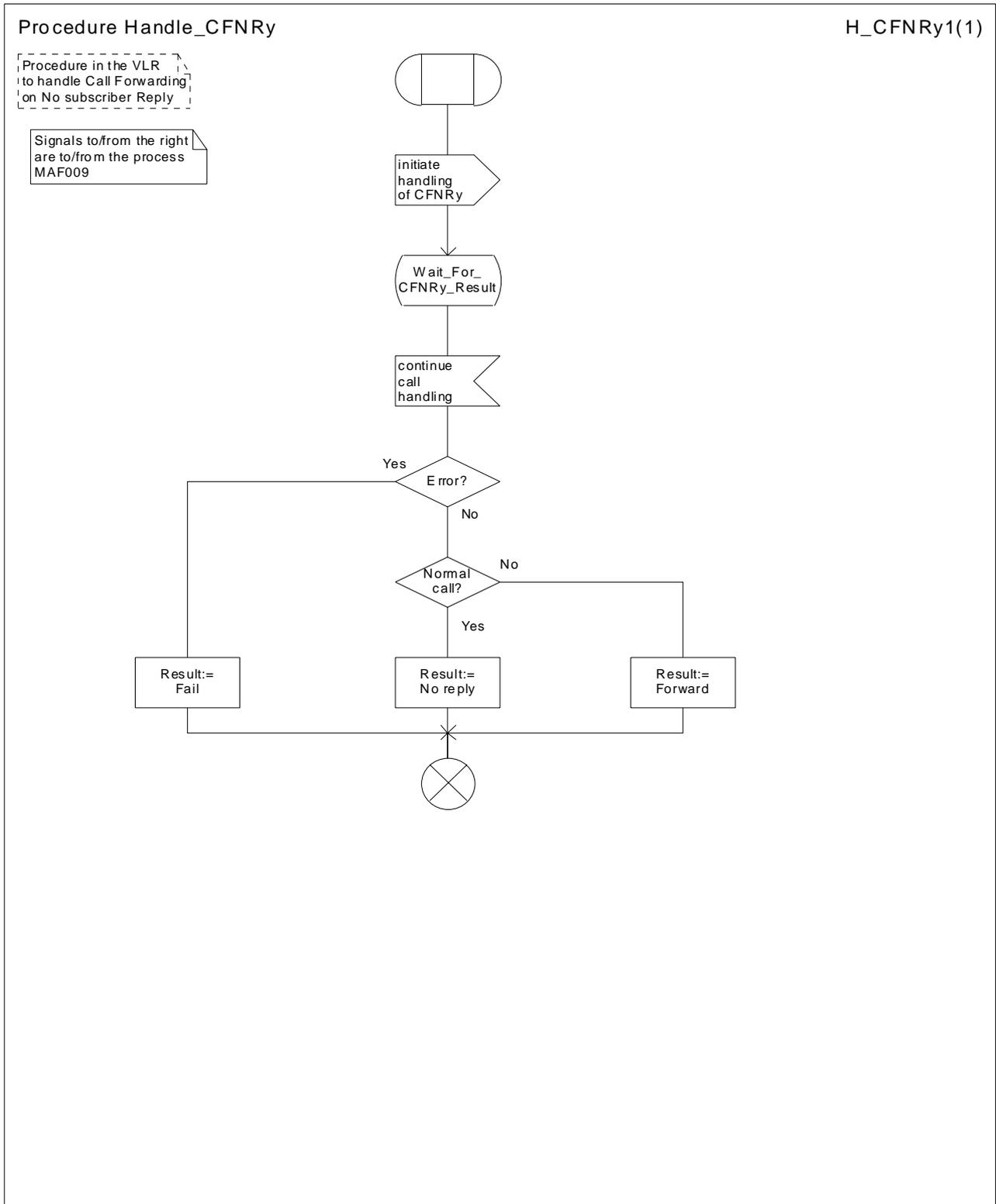
Figure 82: Procedure Handle\_CFNRy
