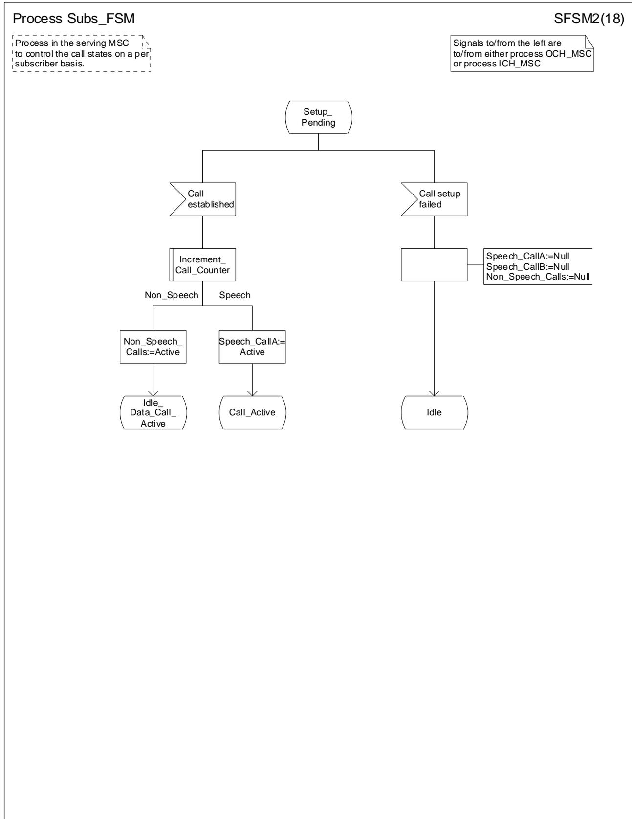
Figure 83b: Process Subs\_FSM (sheet 2)
