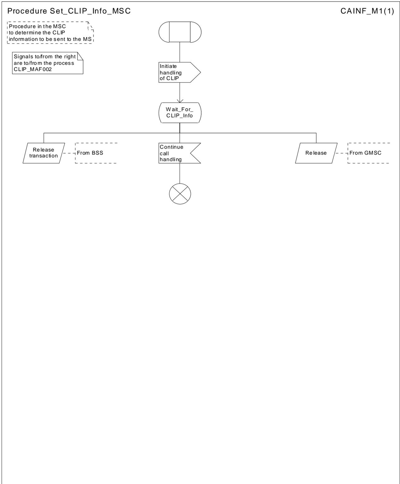
Figure 71: Procedure Set\_CLIP\_Info\_MSC
