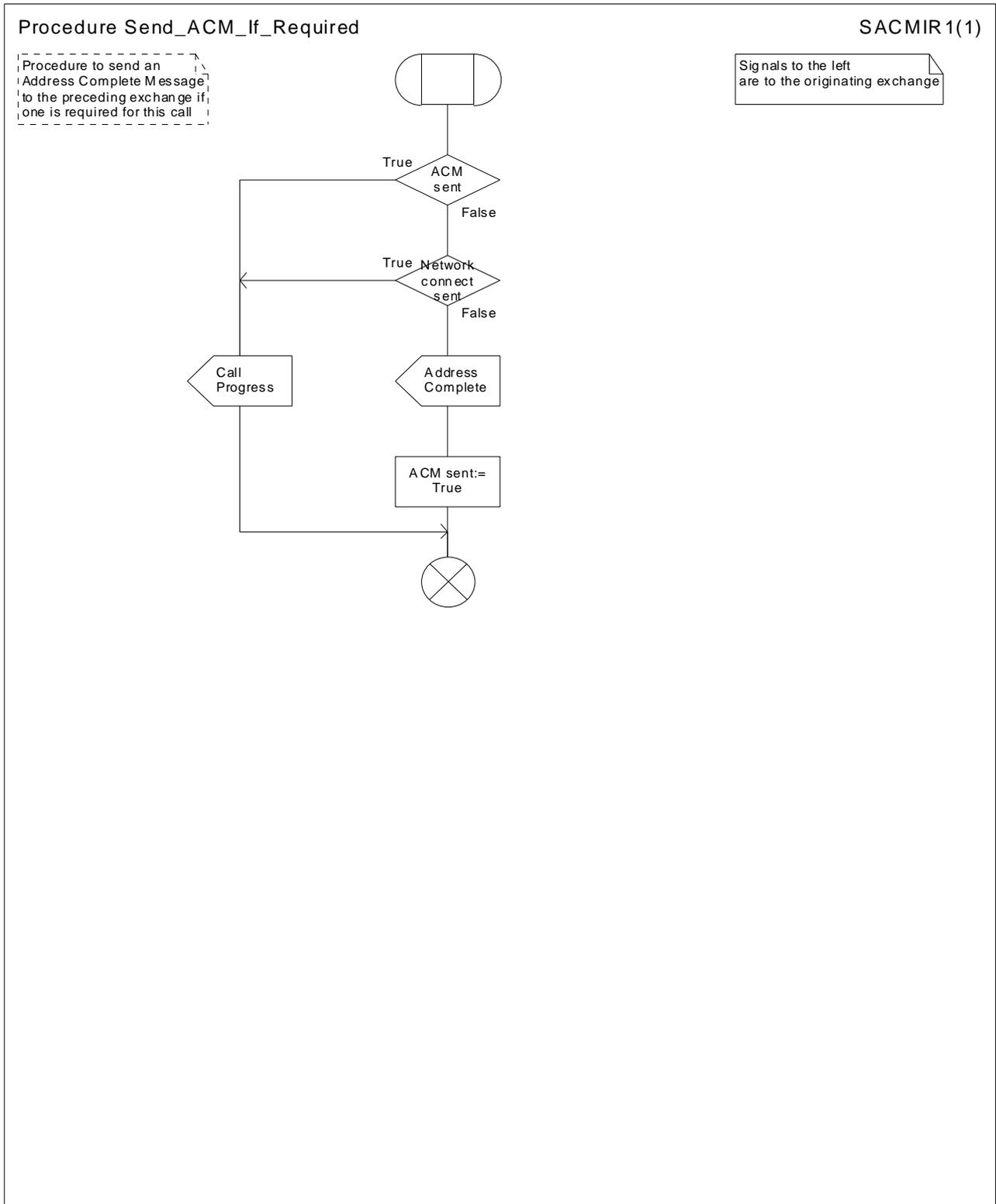
Figure 38: Procedure Send\_ACM\_If\_Required
