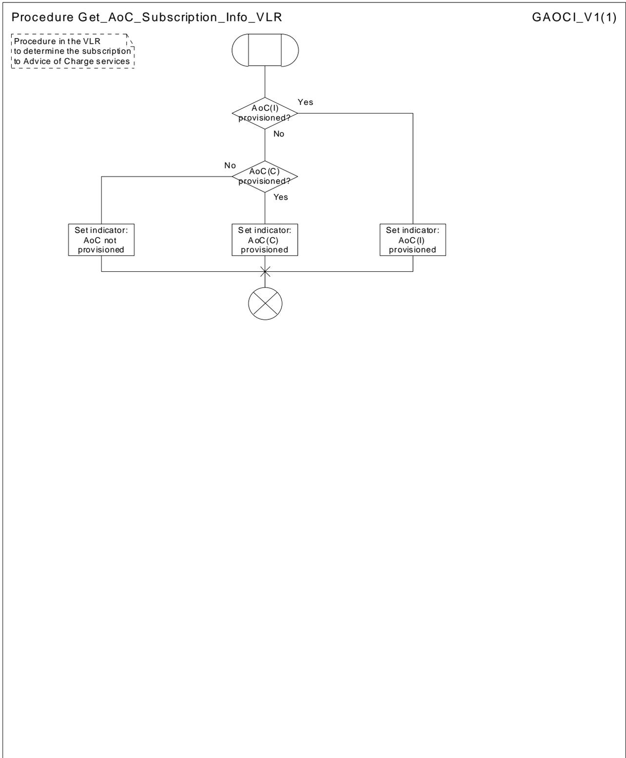
Figure 7.1.2.15: Procedure Get\_AoC\_Subscription\_Info\_VLR
