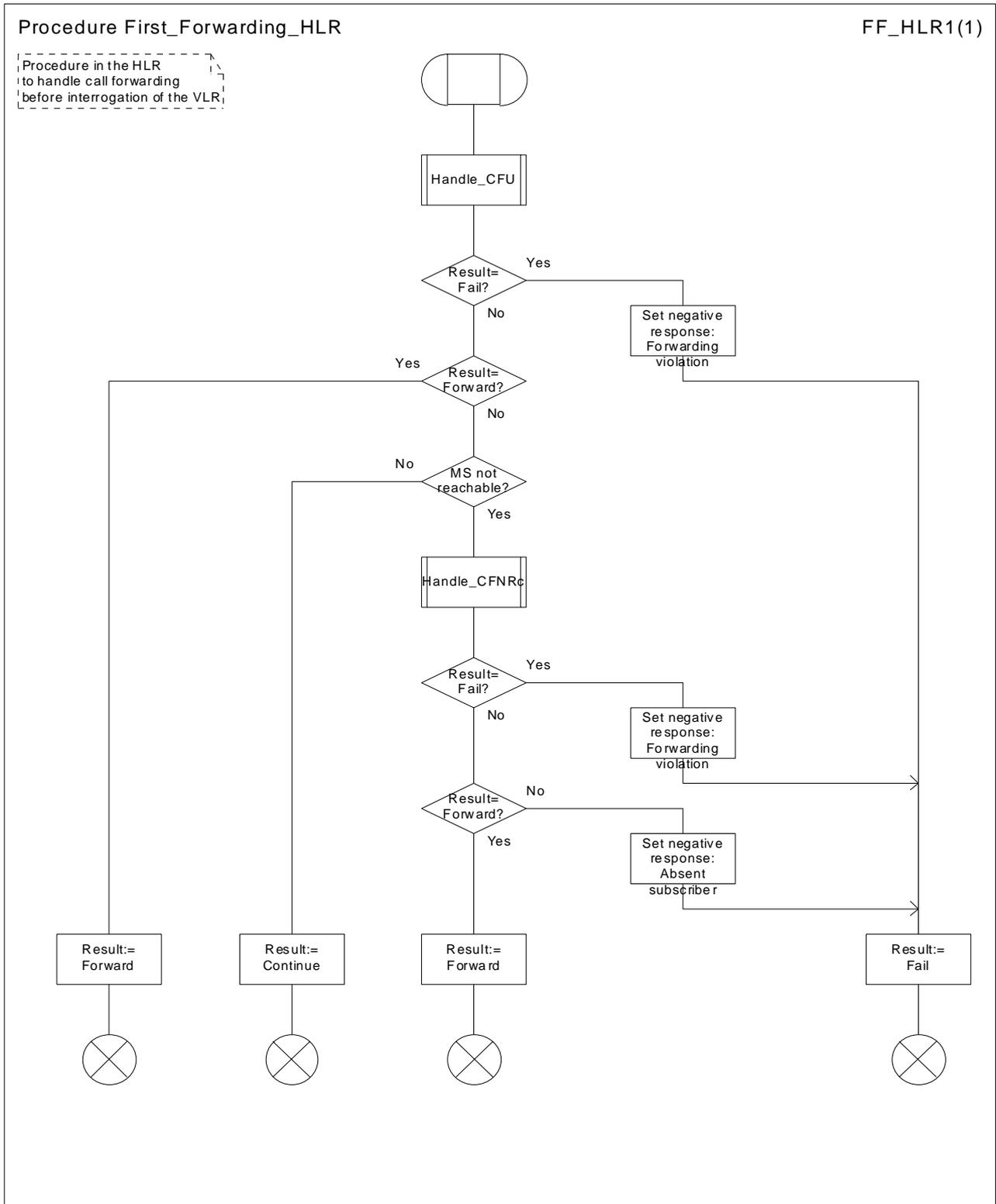
Figure 47: Procedure First\_Forwarding\_HLR
