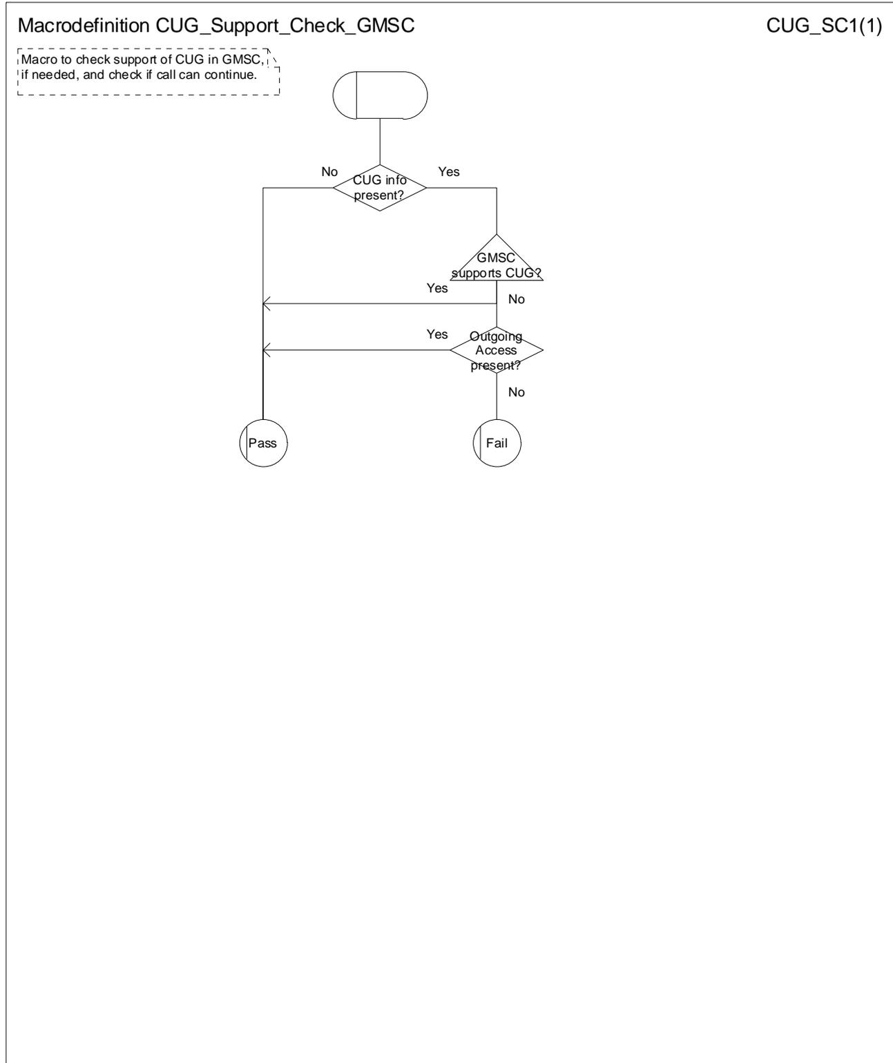
Figure 43bis: Macro CUG\_Support\_Check\_GMSC
