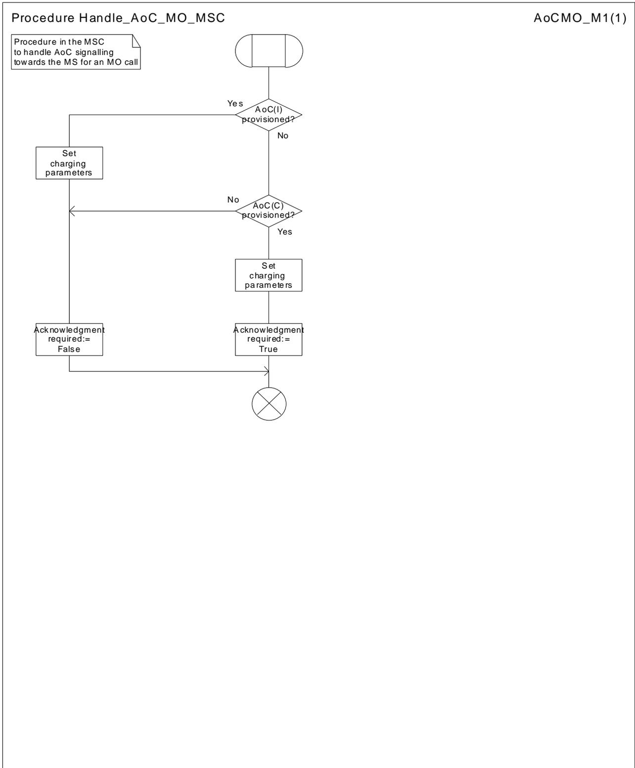
Figure 17: Procedure Handle\_AoC\_MO\_MSC
