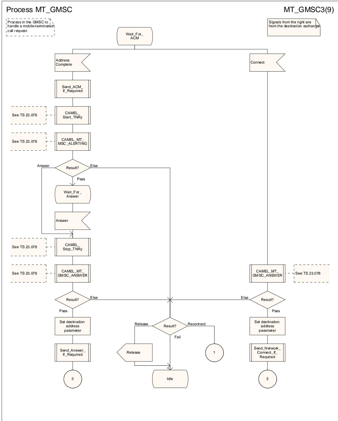
Figure 36c: Process MT\_GMSC (sheet 3)
