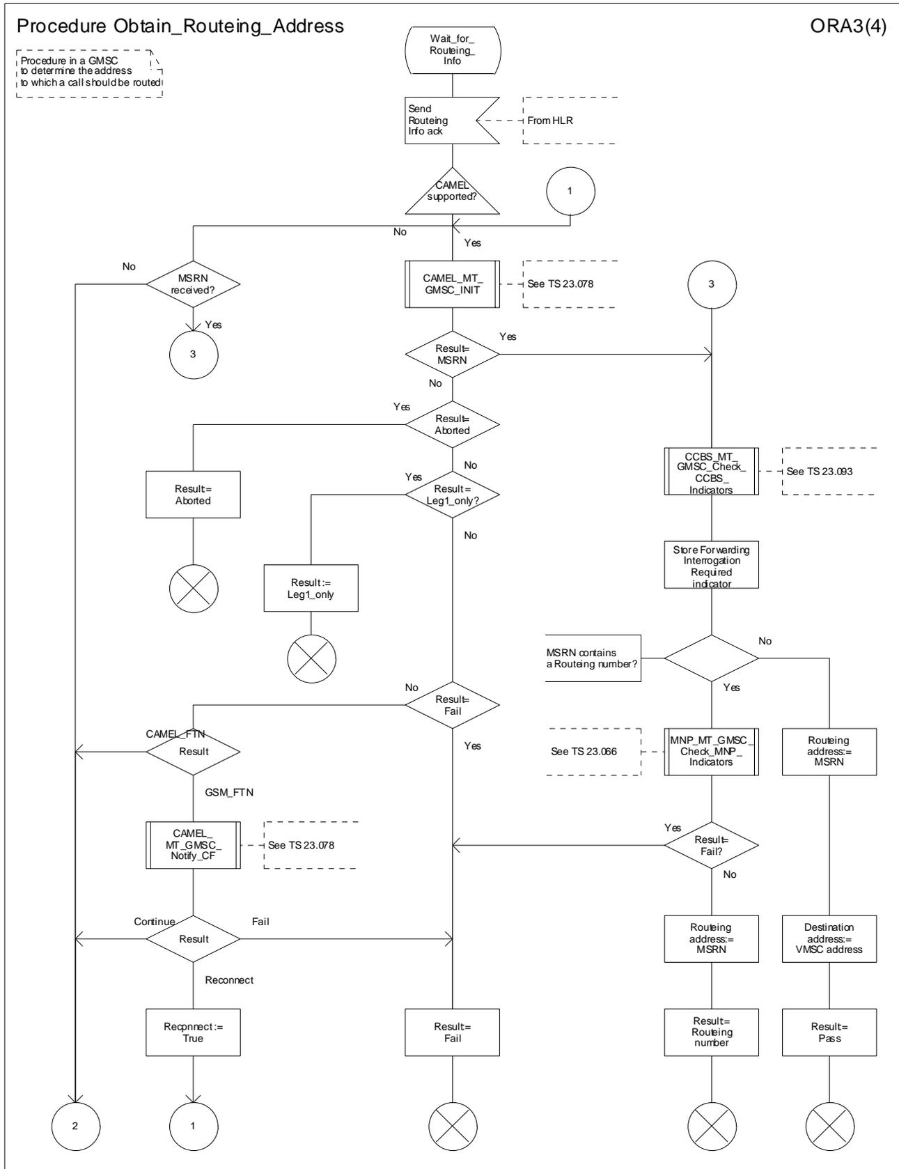
Figure 37c: Procedure Obtain\_Routeing\_Address (sheet 3)
