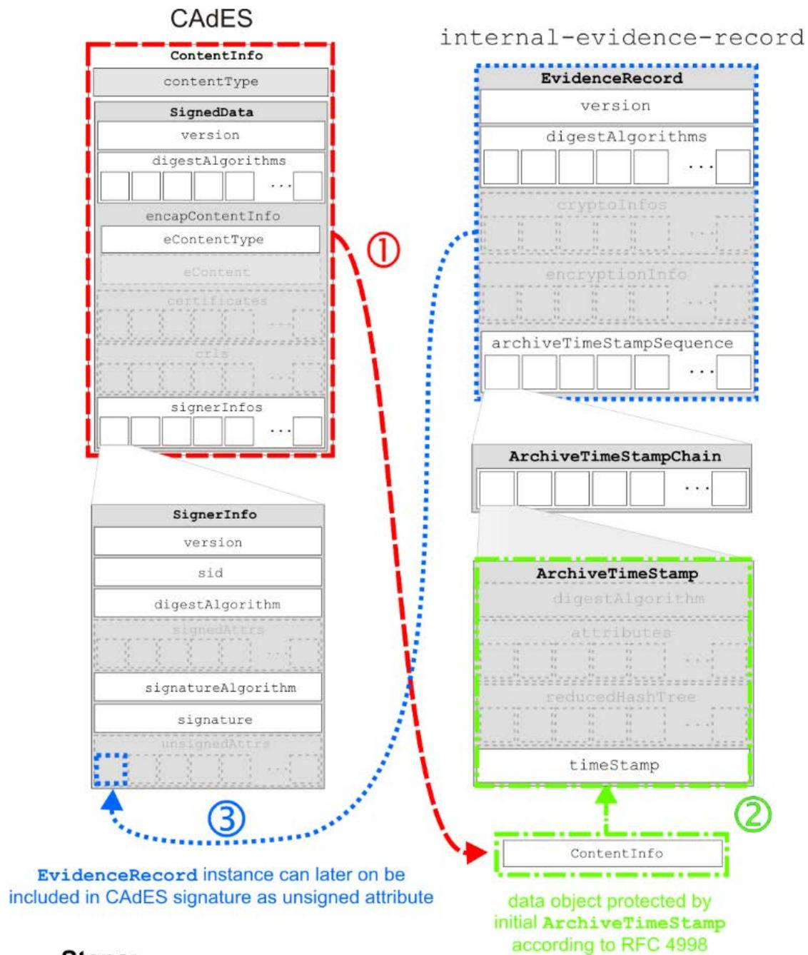
Figure 1: Illustration of internal-evidence-records attribute
