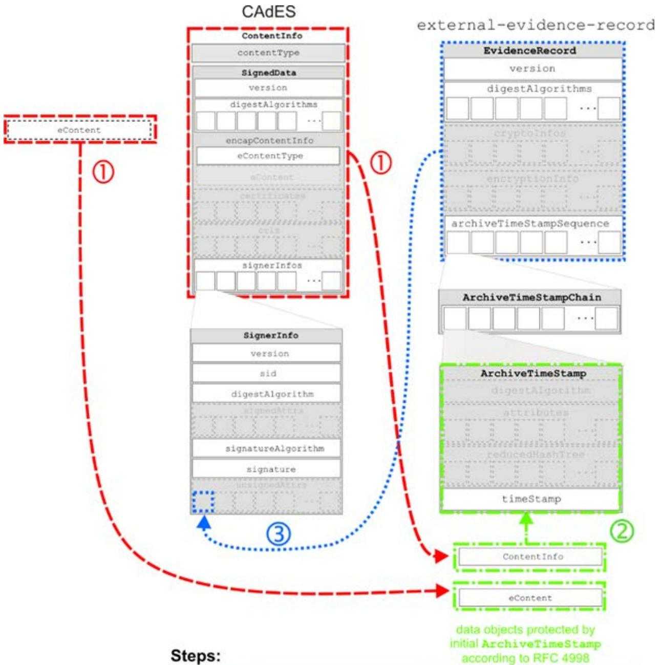
Figure 2: Illustration of external-evidence-records attribute
