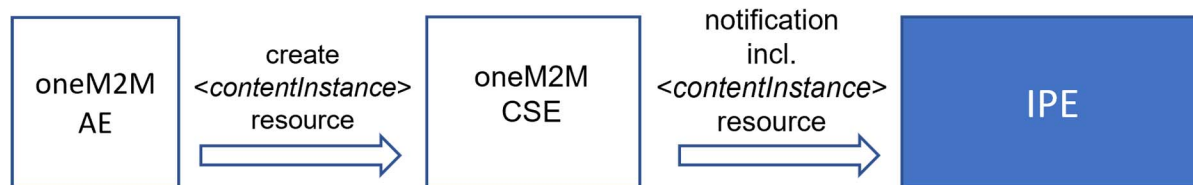
Figure 6.3.2.1-3: Message flow from AE to CSE to IPE
