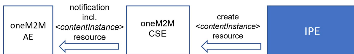
Figure 6.3.2.2-1: Data message flow from IPE to CSE to AE
