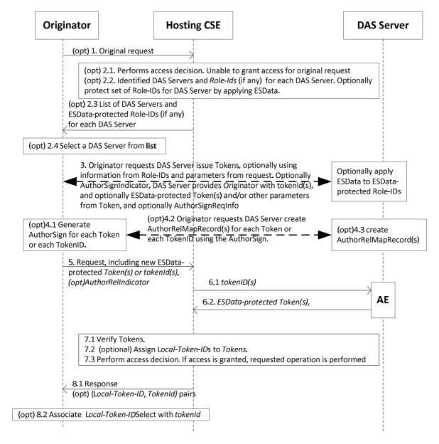
Figure 7.3.2.3-1: Message flow for Indirect Dynamic Authorization
