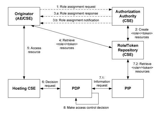
Figure 7.4.1-1: Role based access control architecture
