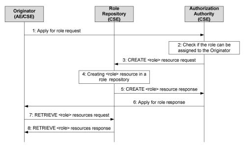
Figure 7.4.2.2-1: Procedure of role assignment
