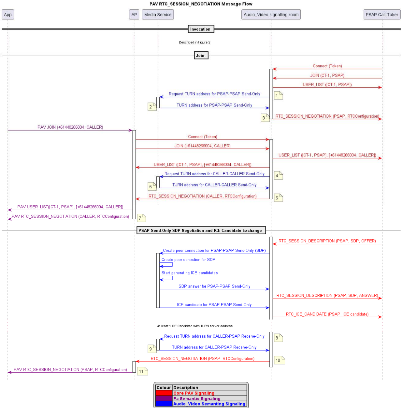
Figure 6: PAV RTC_SESSION_NEGOTIATION Message sequence diagram part 1
