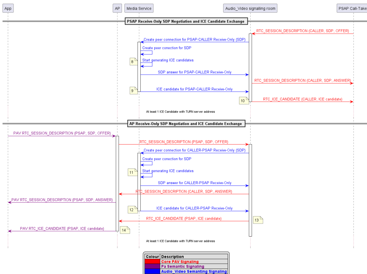
Figure 11: PAV RTC_ICE_CANDIDATE Message sequence diagram part 2
