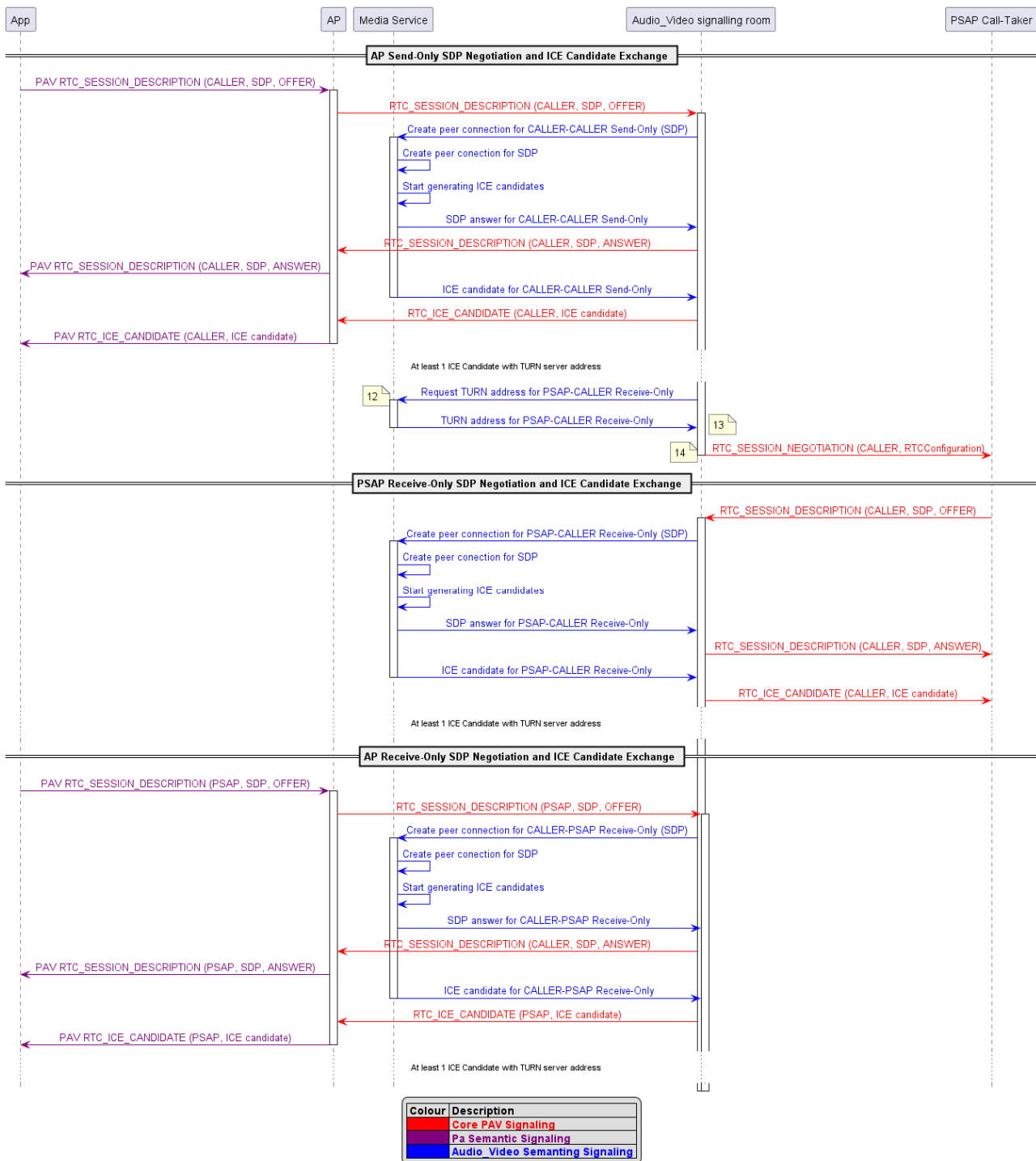
Figure 7: PAV RTC_SESSION_NEGOTIATION Message sequence diagram part 2
