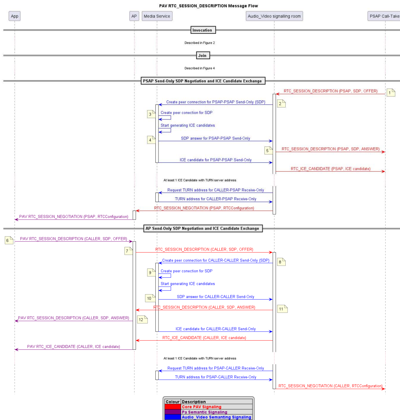
Figure 8: PAV RTC_SESSION_DESCRIPTION Message sequence diagram part 1
