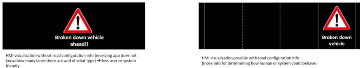
Figure B.1: New HMI options with road configuration information
