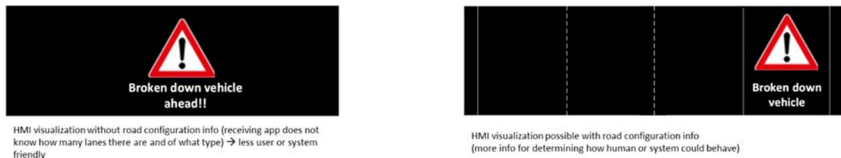
Figure C.1: New HMI options with road configuration information
