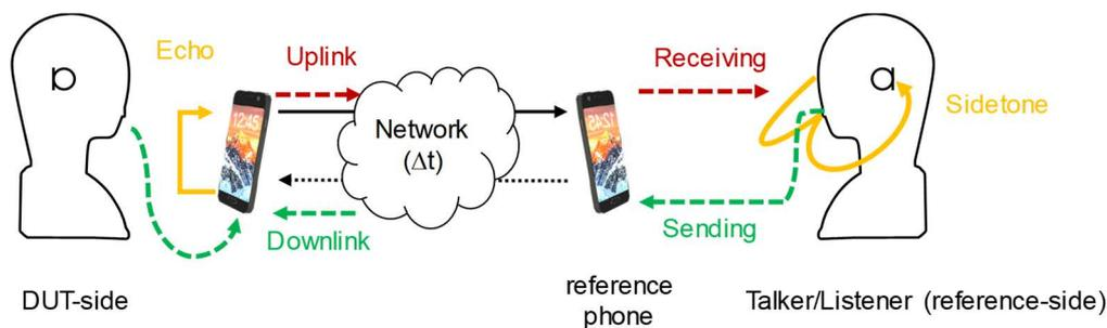
**Figure 5: Components of reference-side speech signals**
