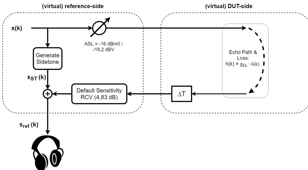
**Figure A.1: Generation of reference conditions for echo-only listening test**
