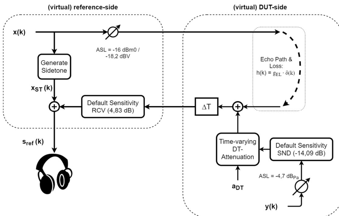
Figure A.2: Generation of reference conditions for double talk listening test
