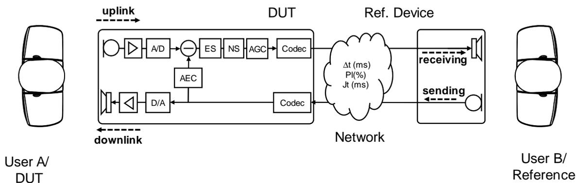
Figure 3: Simplified recording setup for generation of TPLT samples
