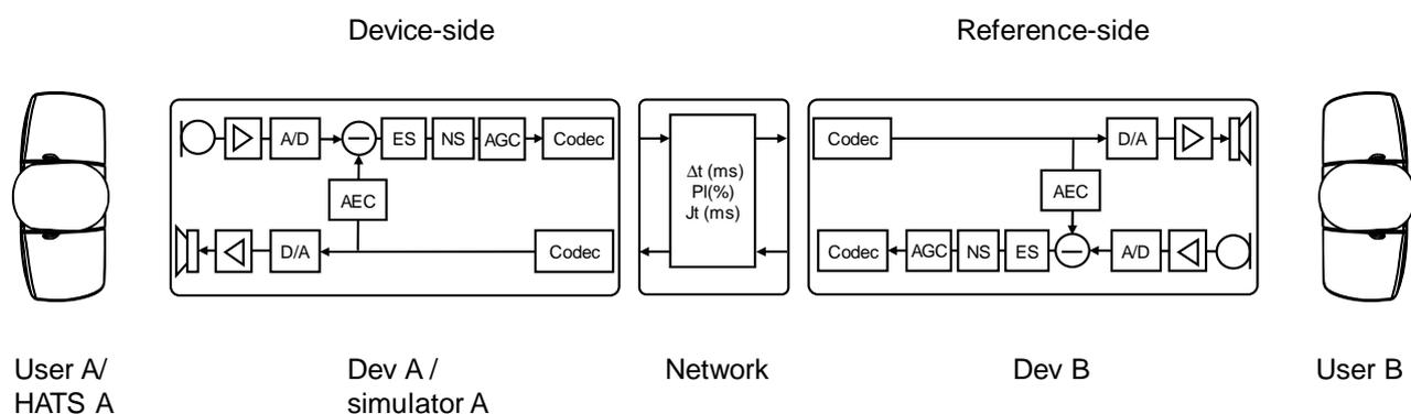
**Figure 1: Technical scheme of conversation in telecommunication**
