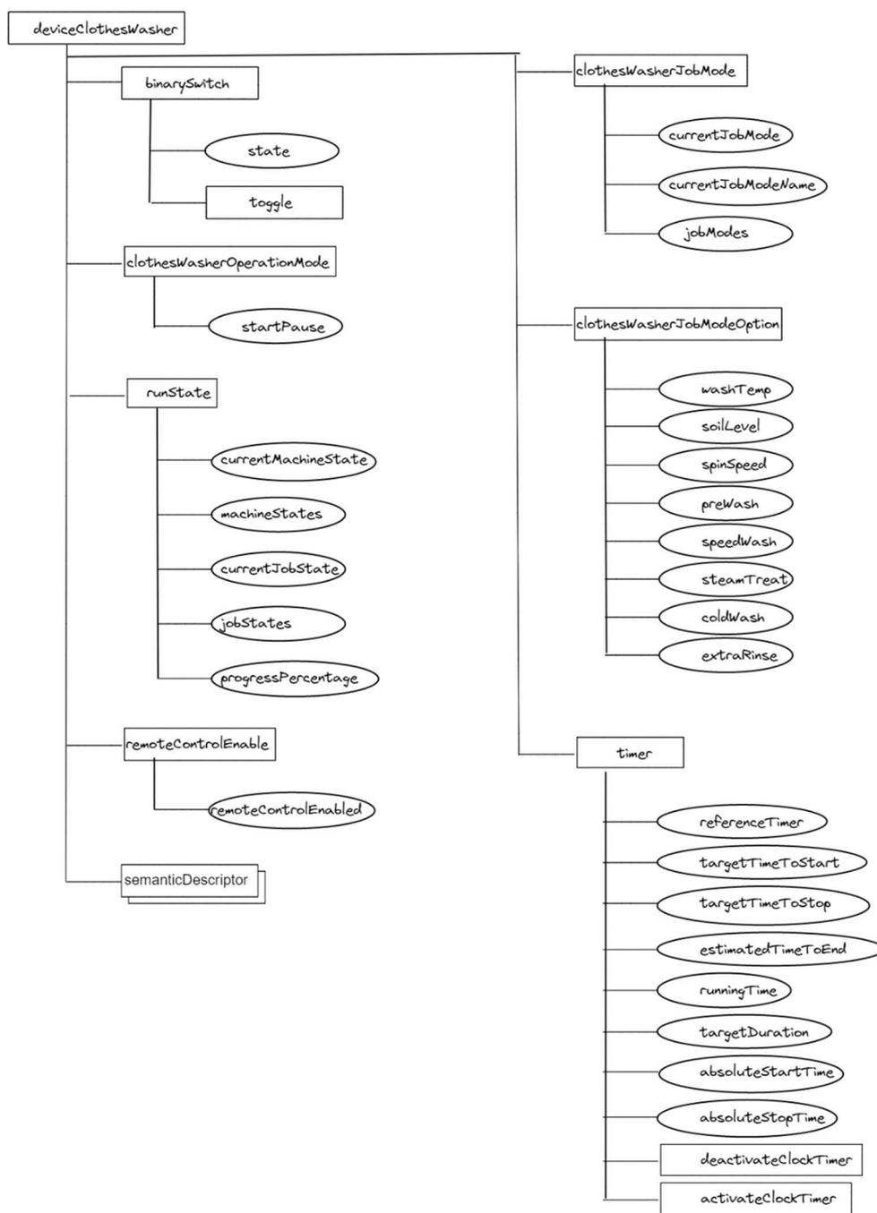
**Figure 9: SDT washing machine model**
