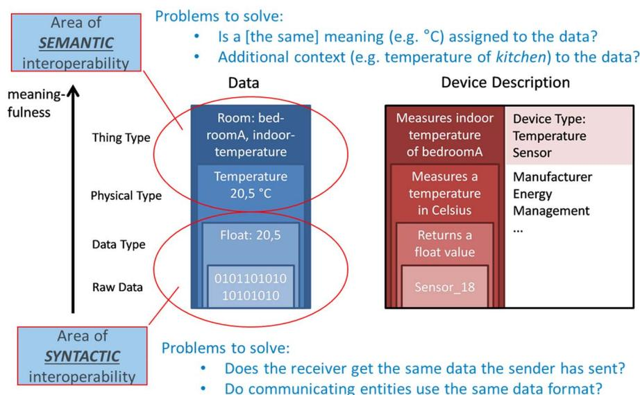
Figure 2: Meaningfulness of data from IoT devices
