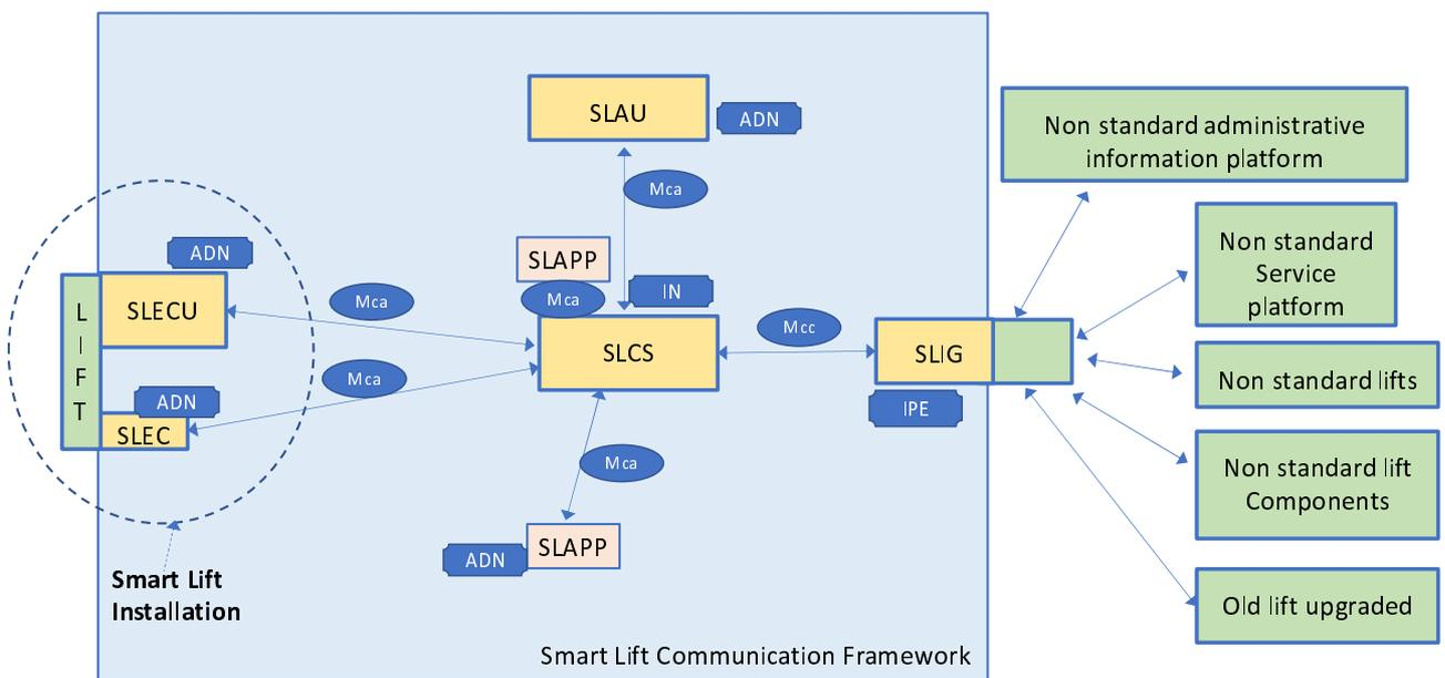
Figure 5.3-1: Smart Lift deployment cases
