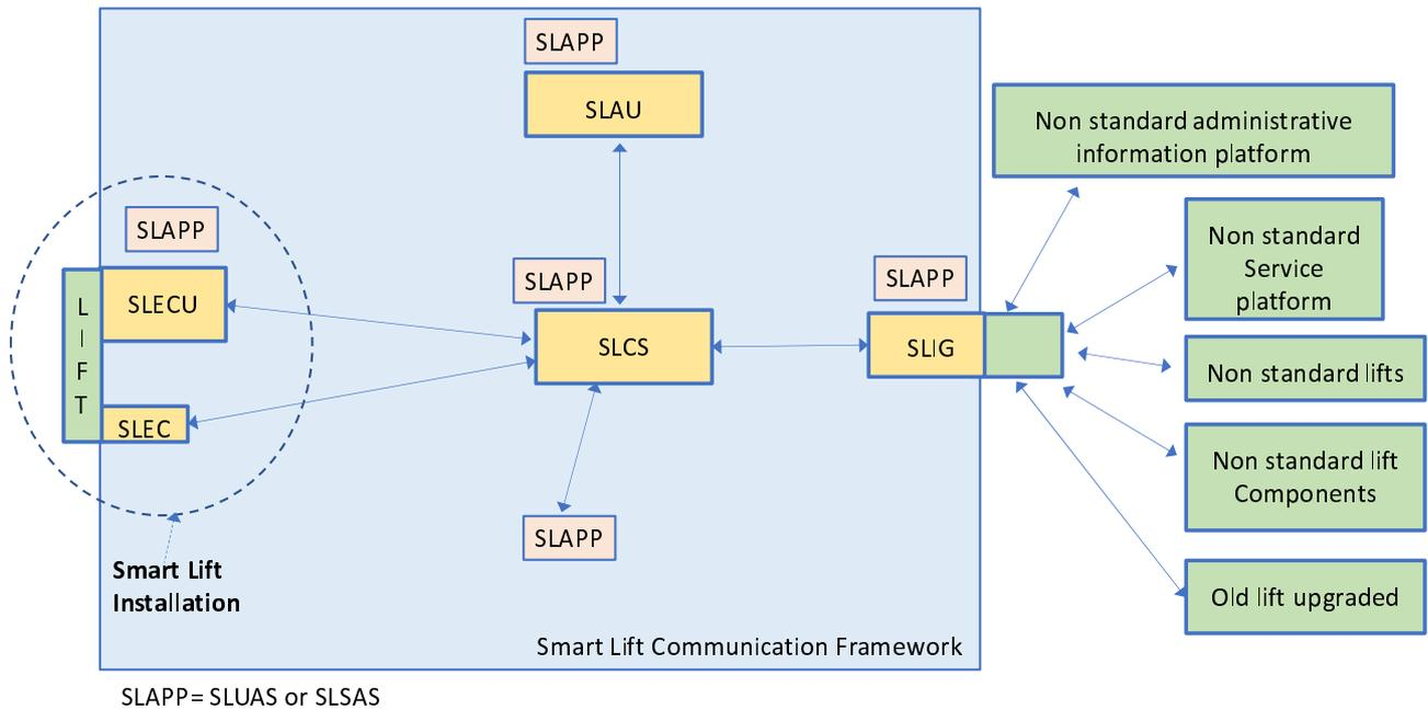
**Figure 5.1-1: Smart Lift Systems IoT Architecture**
