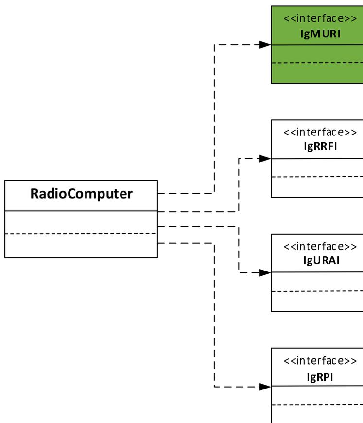
**Figure 4.2: UML class diagram for Radio Computer interfaces**
