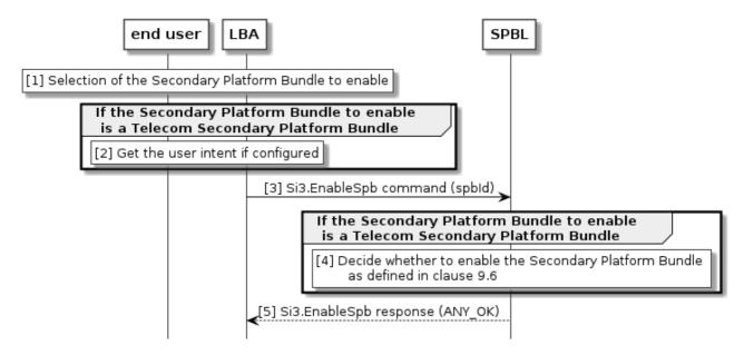
Figure 12.10: Enable Secondary Platform Bundle procedure
