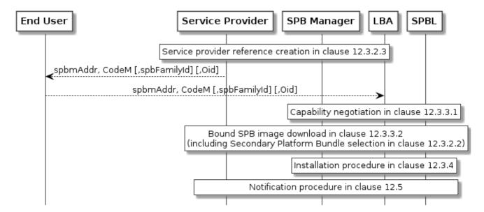
Figure 12.3: Secondary Platform Bundle provisioning procedure - case 2
