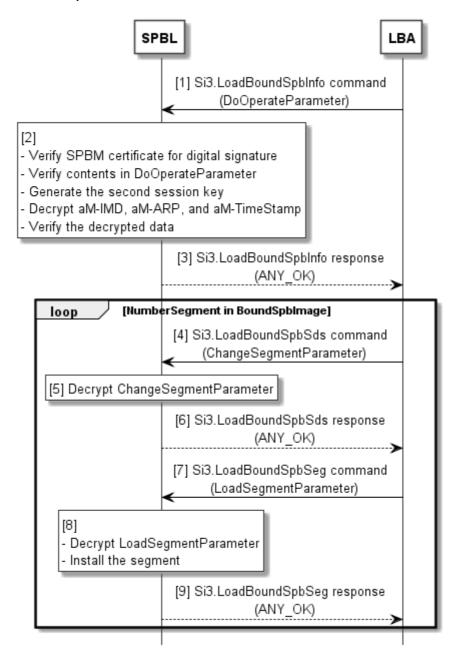
Figure 12.9: Installation procedure
