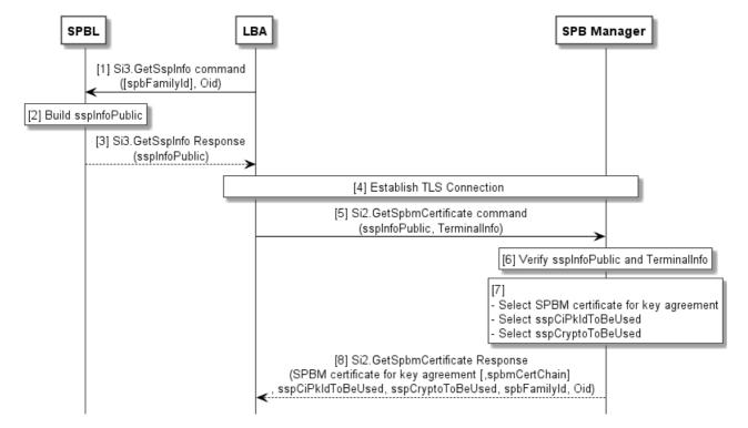
Figure 12.7: Capability negotiation procedure
