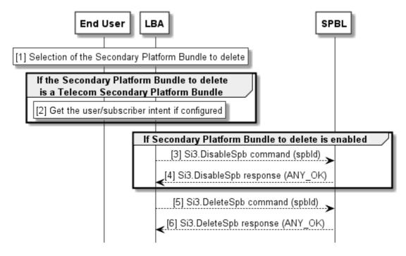
Figure 12.12: Delete Secondary Platform Bundle procedure
