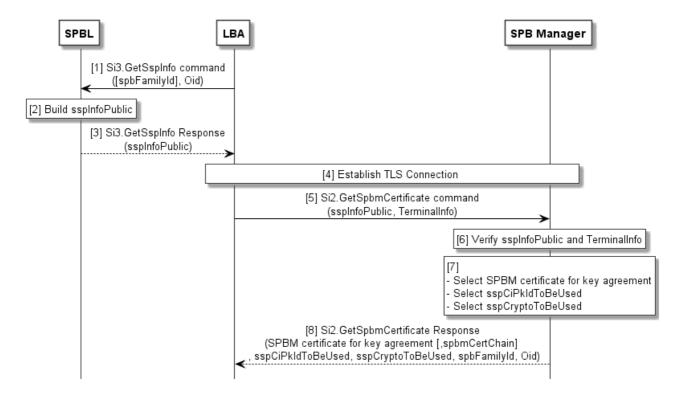
Figure 12.7: Capability negotiation procedure
