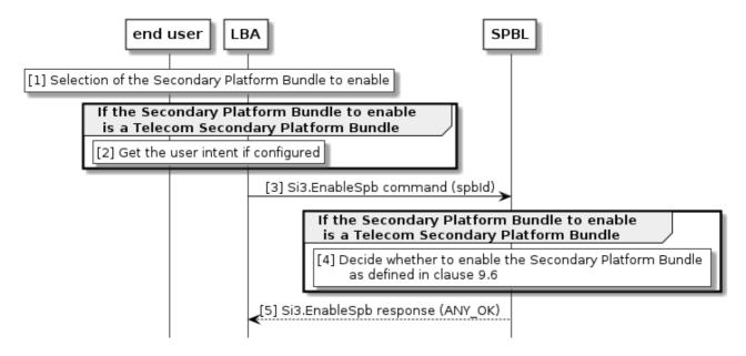
Figure 12.10: Enable Secondary Platform Bundle procedure
