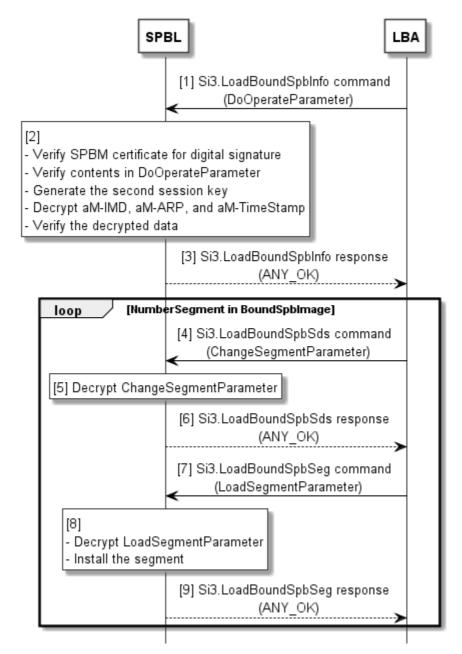
Figure 12.9: Installation procedure
