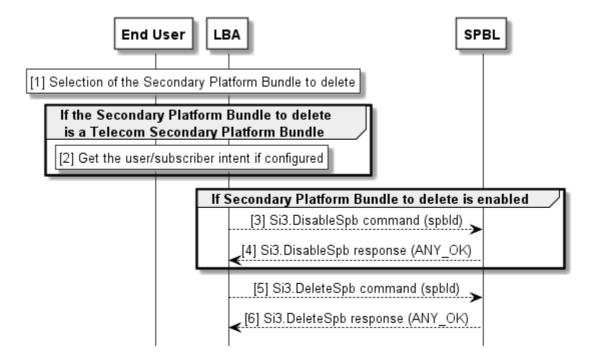
Figure 12.12: Delete Secondary Platform Bundle procedure
