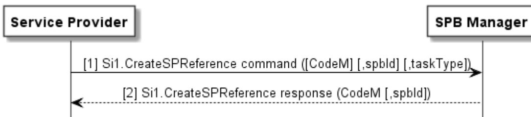
Figure 12.5: Service provider reference creation process
