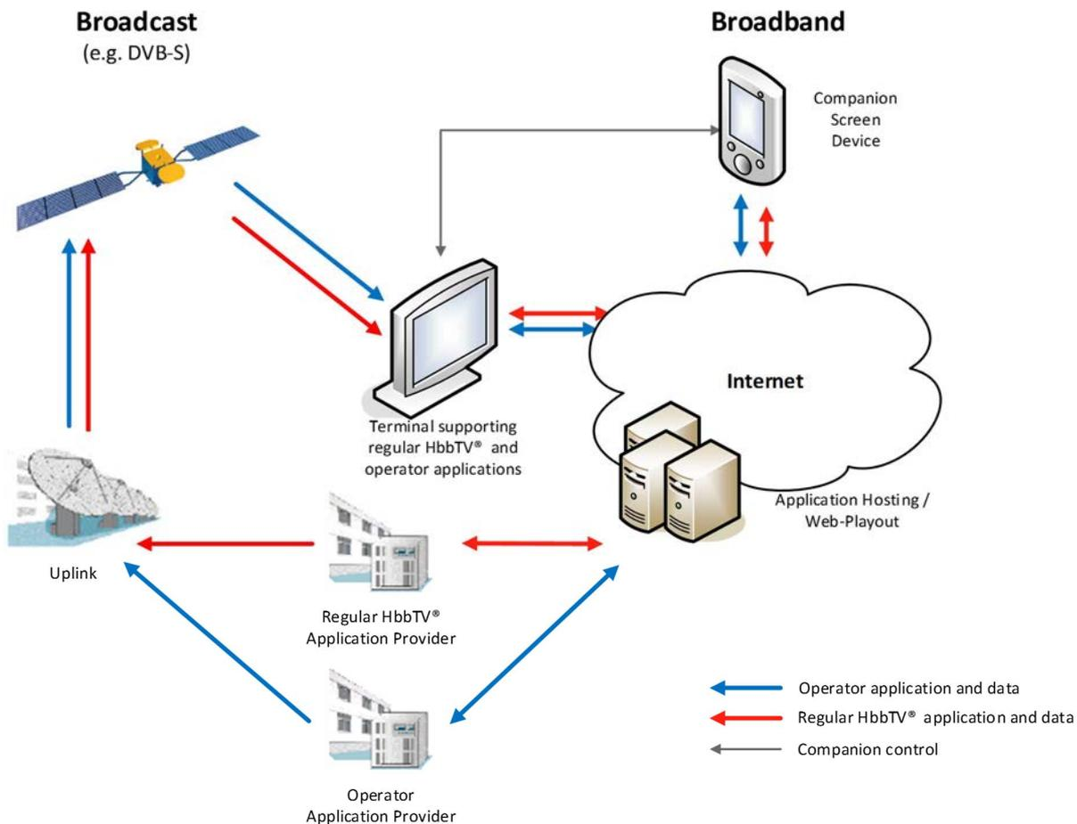
**Figure 1: System overview for an operator application terminal**
