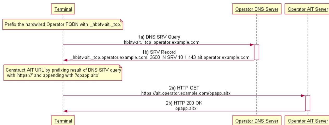
Figure C.2: Operator application discovery from hardwired FQDN
