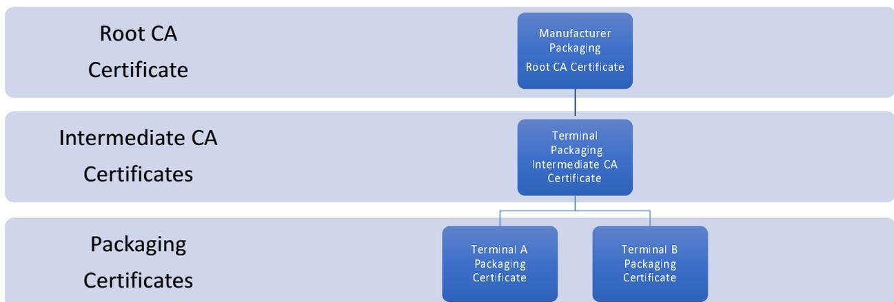
**Figure 4: Example of a Manufacturer Packaging Certificate Hierarchy**
