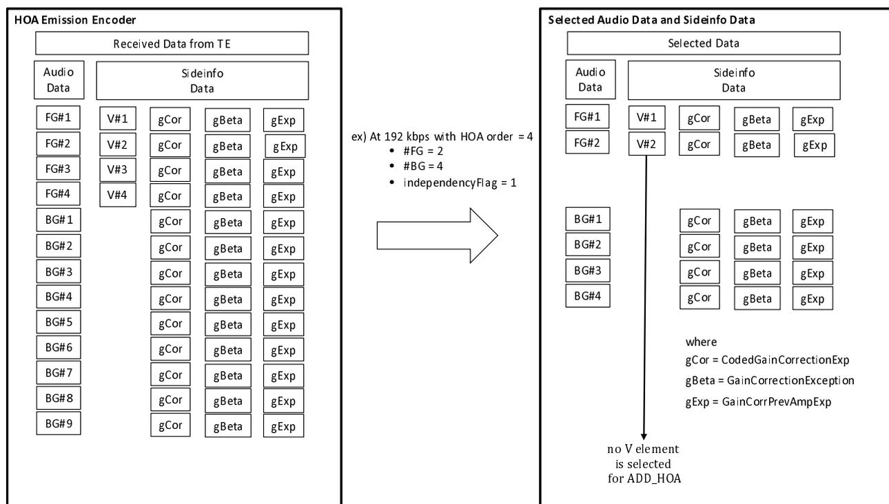
**Figure 4: Example of HOA Transport Signals and HOA Side-info selection at the emission encoder**
