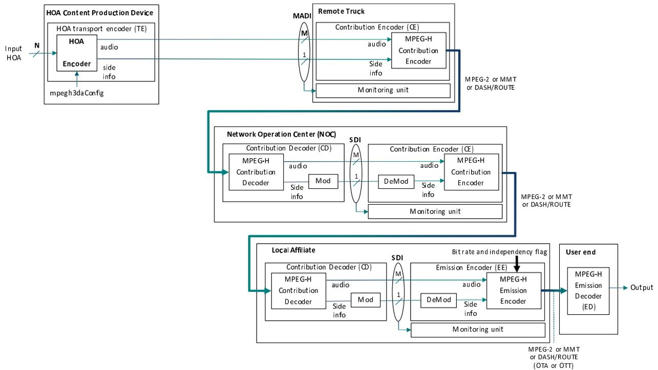
**Figure B.1: Block diagram of HOA Content Production**
