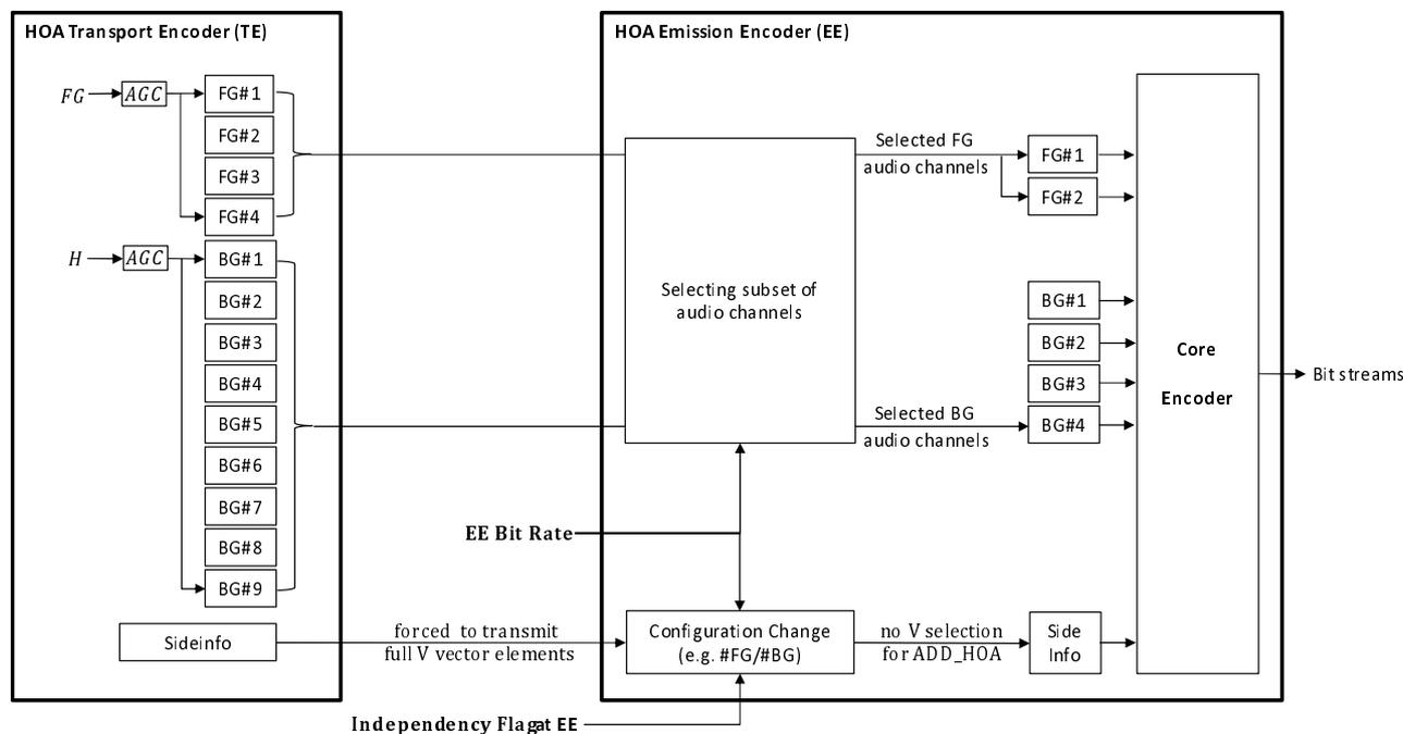
**Figure 3: HOA Transport Encoder (TE) and Emission Encoder (EE) settings**
