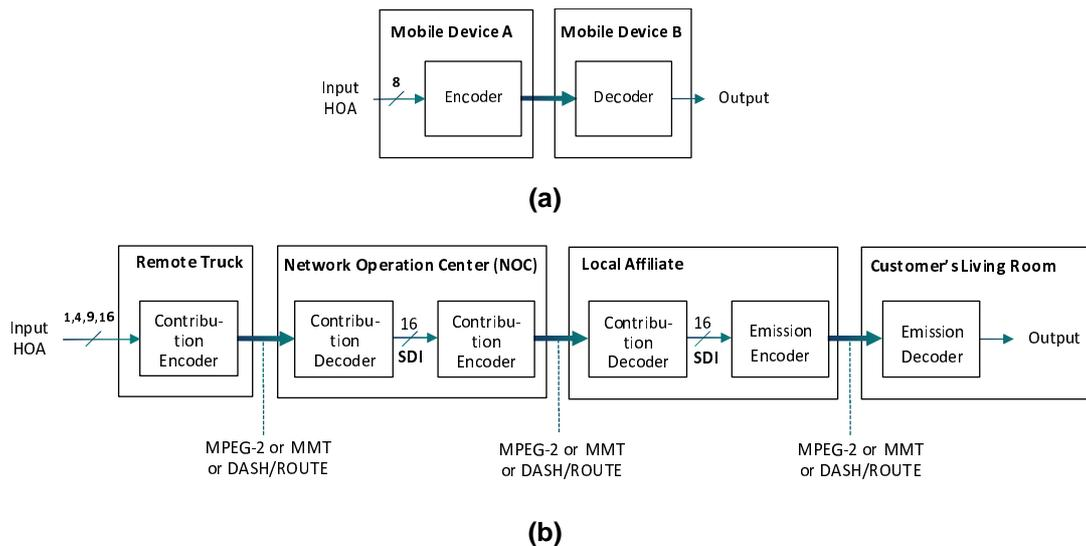
Figure 1: (a) conventional mobile devices and (b) conventional broadcast chain for order-restricted Ambisonics transport
