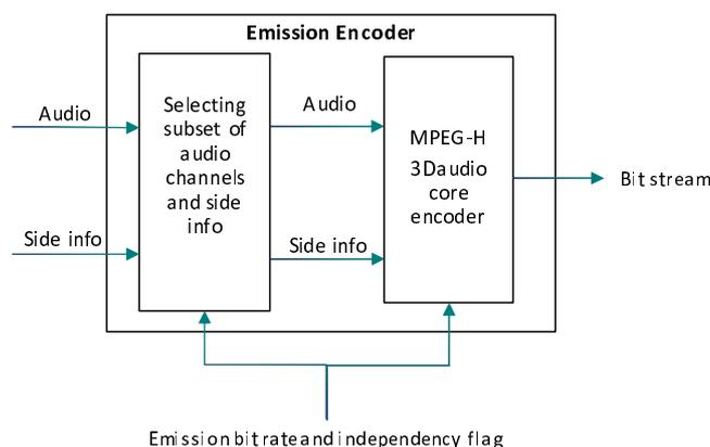
**Figure A.2: Block diagram of HOA emission encoder**
