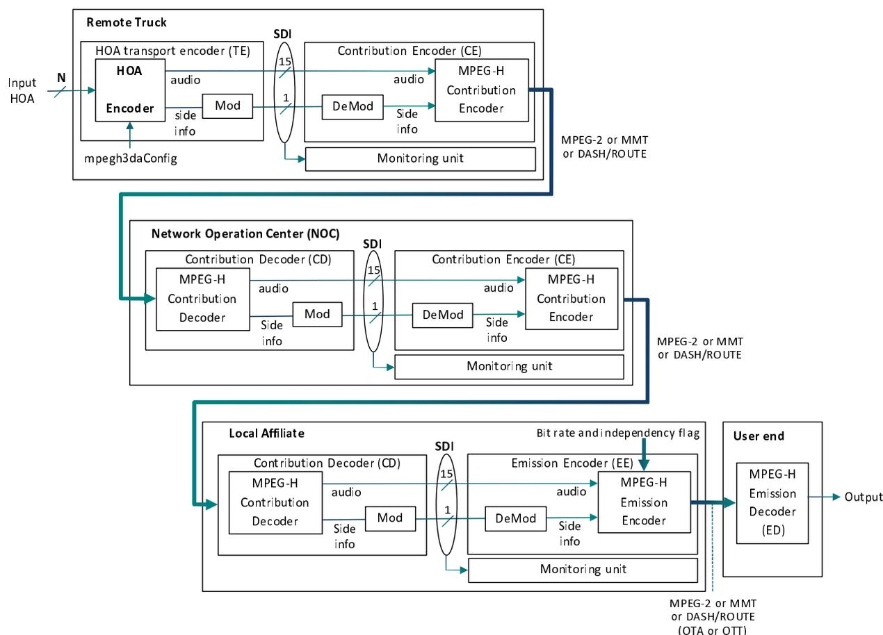
**Figure A.1: Block diagram of broadcast chain type-I that transports HOA signals (for simplicity, conversion modules from/to MPEG-2 or MMT or DASH/ROUTE are not described)**
