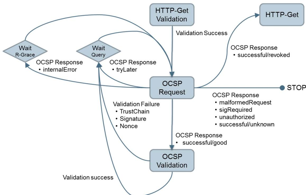
**Figure 3: State Machine Diagram - Certificate Revocation Checks**
