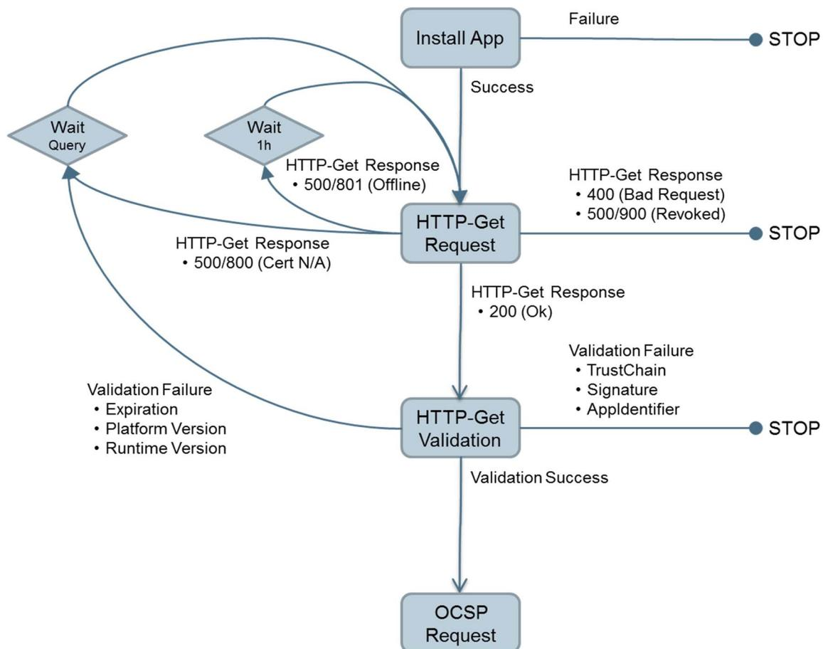
Figure 2: State Machine Diagram - Certificate Retrieval and Validation
