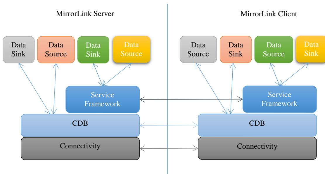
**Figure 1 Top level architecture of MirrorLink data service**
