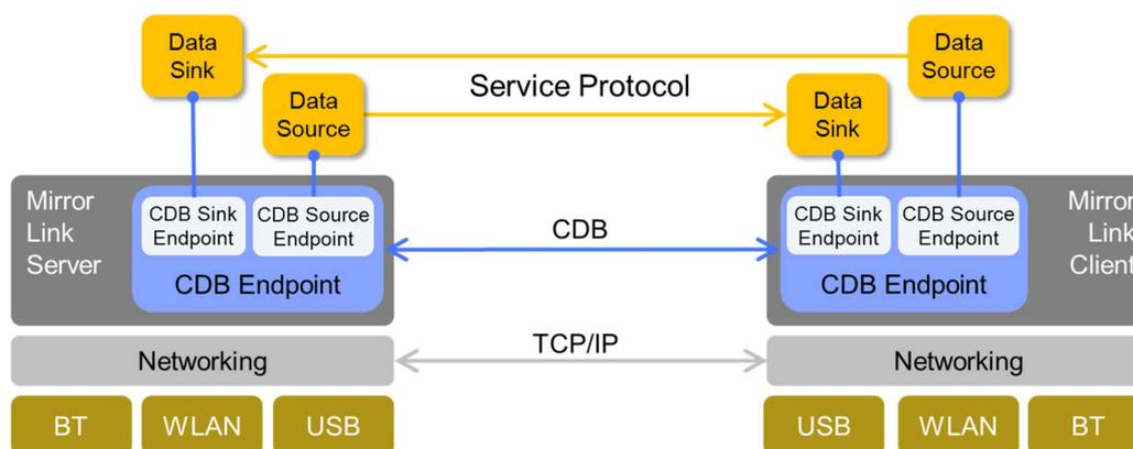
Figure 1: Common Data Bus Architecture with TCP binding
