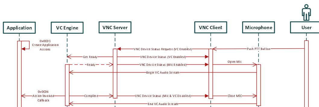
Figure 6: Message Sequence for MirrorLink Client triggered VC
