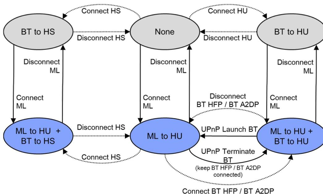
**Figure 13: Bluetooth / MirrorLink IOP States – MirrorLink Server Perspective**
