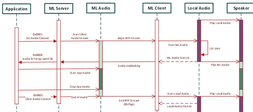
**Figure 18: Unblocking of MirrorLink Audio with presence of Local Audio**
