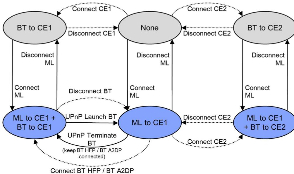
**Figure 14: Bluetooth / MirrorLink IOP States – MirrorLink Client Perspective**
