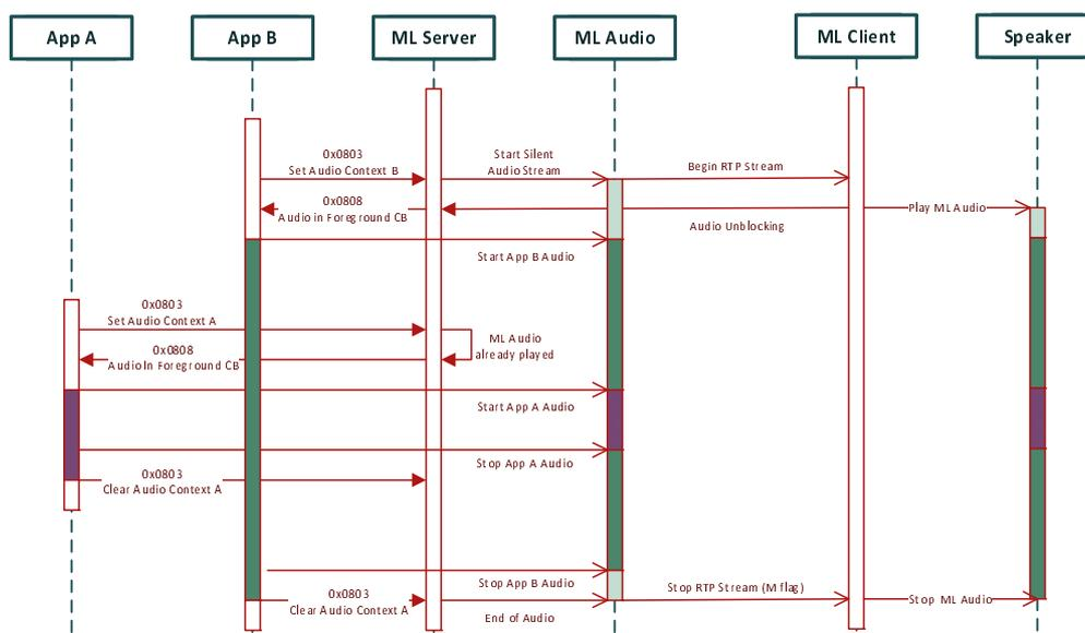
**Figure 19: Unblocking of MirrorLink Audio with presence of another MirrorLink Audio**
