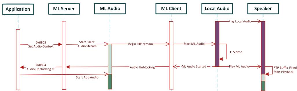
Figure 20: Impact of Initial Playback Latency in Message Sequence
