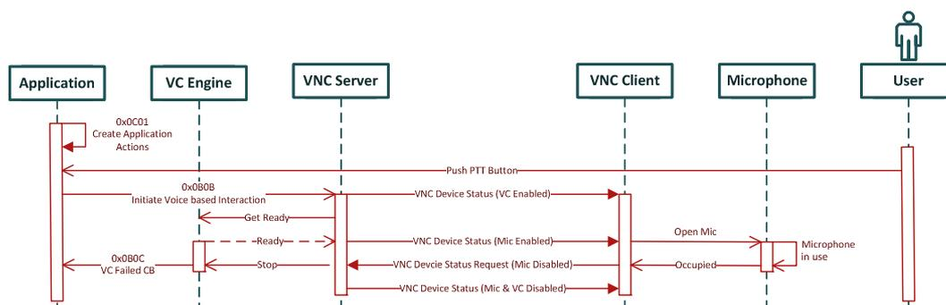
Figure 8: Message Sequence for VC with Occupied Microphone
