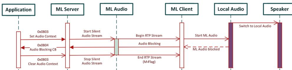
Figure 17: Blocking of MirrorLink Audio with presence of Local Audio
