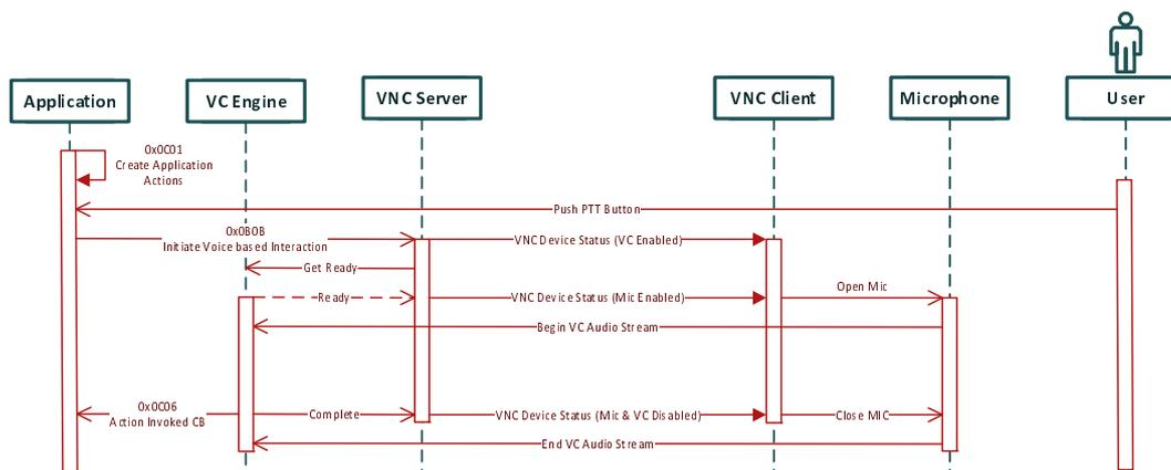
Figure 7: Message Sequence for MirrorLink Server triggered VC
